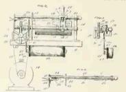
by wholly relieving the user of the burden of personally attending to operating the phonograph mechanism, supplying and removing records, adjusting the stylus, and looking after the wax cylinders from the time they are shaved, until adjusted in position on the reproducer.
