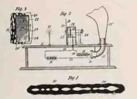
of light admitted corresponding to the sound waves. Consequently the electric undulations in the circuit, and the resultant audible vibrations of the diaphragm, correspond to the sound waves.
