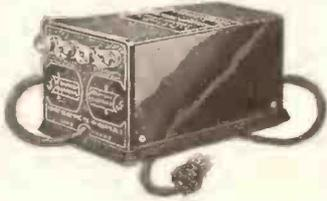
The Unitron Control enables you to draw current for both your "A" charger and "B" eliminator from a single light socket, and to control them both from the switch located on the operating panel of your radio. When you turn your set on, the "B" eliminator is thrown in and the "A" charger is cut out. When the set is turned off the reverse is accomplished.
