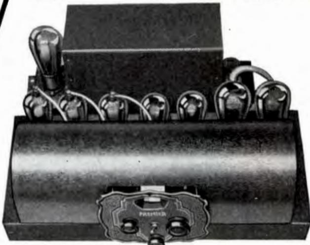
Here is the last word in Screen Grid Radio Chassis—Premier Model 724-D, using three 224-type tubes, two 227, two 245 and one 280 rectifier. Power Unit also supplies current for D. C. Dynamic Speaker.
