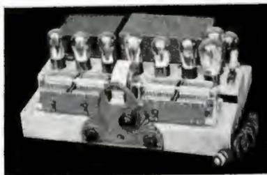
**Mandel Radio Chassis** type tubes in push-pull amplification and one type 250 rectifier tube. Receiver operates only on AC dynamic speaker.
