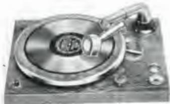
**Gordon Pick-Up and Panel Assembly** bronze. Furnished complete, with 12-inch turntable, automatic stop, speed control and extension cord. Furnished in 110 volt AC 60 cycle and also 25 cycle. Motor can be geared to run 33 r.p.m., with a 10-inch turntable for talking picture work. Gordon Electric employing counter-balanced tone arm. All metal parts, including
