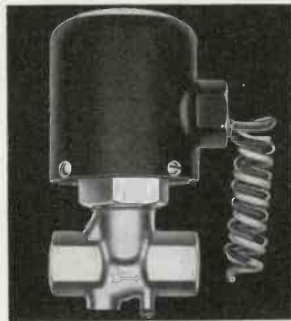
model is available with  $\frac{1}{8}$  in. orifice and the other in two orifice sizes,  $\frac{3}{16}$  in. and  $\frac{7}{32}$  in. Designed specifically for water control on water-cooled condensing units, humidifying systems and similar applications, the valves operate by the action of a movable plunger housed in a non-magnetic plunger tube surrounded by a coil. Noise and mechanical rattle are eliminated with these valves.
