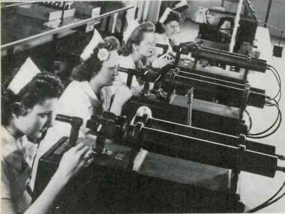
▲ **HIGH VOLTAGE** supplied by vacuum tube rectifiers clears atmosphere of dust, lint, and other air-borne dirt particles in binocular assembly room of Westinghouse, Mansfield, Ohio, plant. Girls can't wear makeup. Gun-like collimators house optical systems which check each binocular for definition of image and alignment
