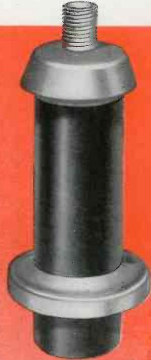
Solder-sealed entrance bushing used for larger type capacitors. Lower ring is soldered to bushing and to metal container. Upper ring is soldered to bushing and to lead brought up through bushing and hollow stud.
