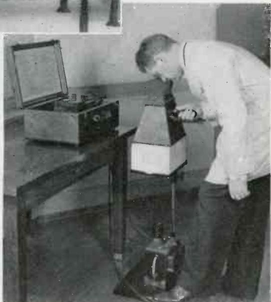
**BURNING** an evidence sample ↓ in arc of spectrograph
