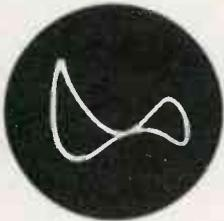
Two batches of different steel alloys became mixed. They had to be sorted quickly, positively, economically. This oscillograph pattern served to identify one alloy from the other.
