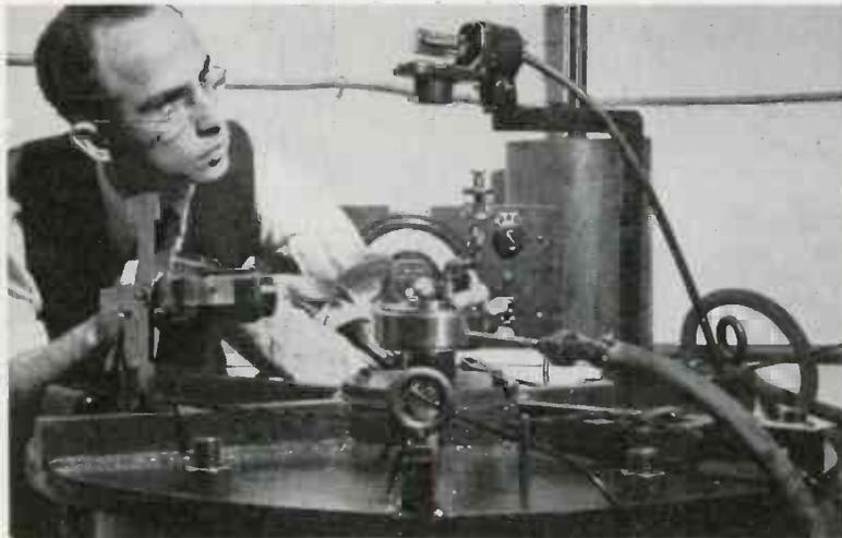
↑ **PHOTOELECTRIC** tachometer measures speed of super-charger impellers in test runs at General Electric Company. Two-faced mirror on shaft-end reflects impulses to photo-tube above, and frequency meter indicates speed of rotation. Impellers weighing as much as twenty pounds are driven to 60,000 rpm in vacuum chamber
