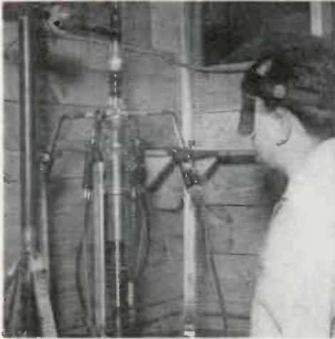
**STEM-PRESS** machine. Sealing tungsten filament rods to glass
