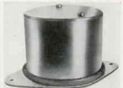
Consisting of a synchronous motor-driven timer which delivers an accurately measured time delay prior to activation of a switch mechanism, it controls plate voltage to mercury vapor rectifiers and other tube equipment.
