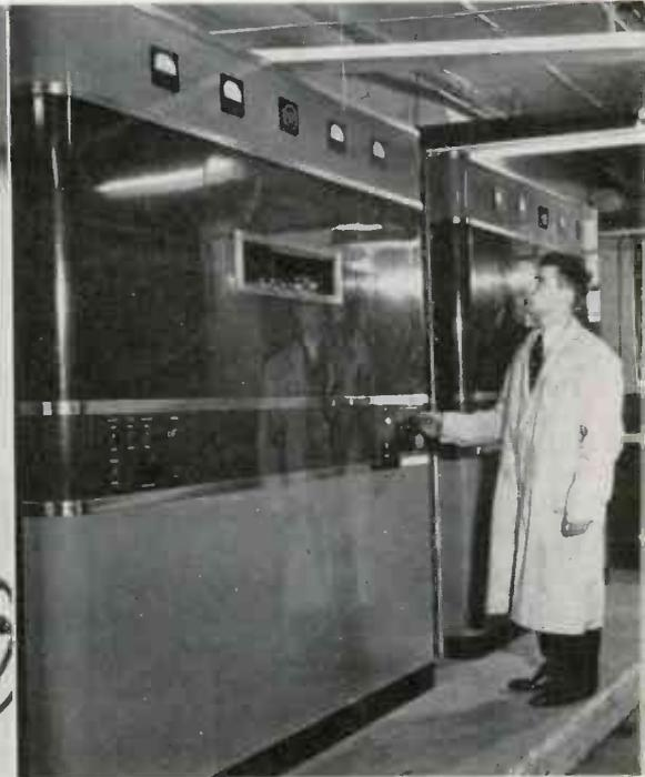
▲ **HIGH FREQUENCY** heating oscillator used in developmental work on laminated wing-spars and other components of plywood airplanes, at Dura-mold Division of Fairchild Aircraft and Engine Corp., New York City. Unit is a converted FM amplifier, with output of 15 kw at 10 mc
