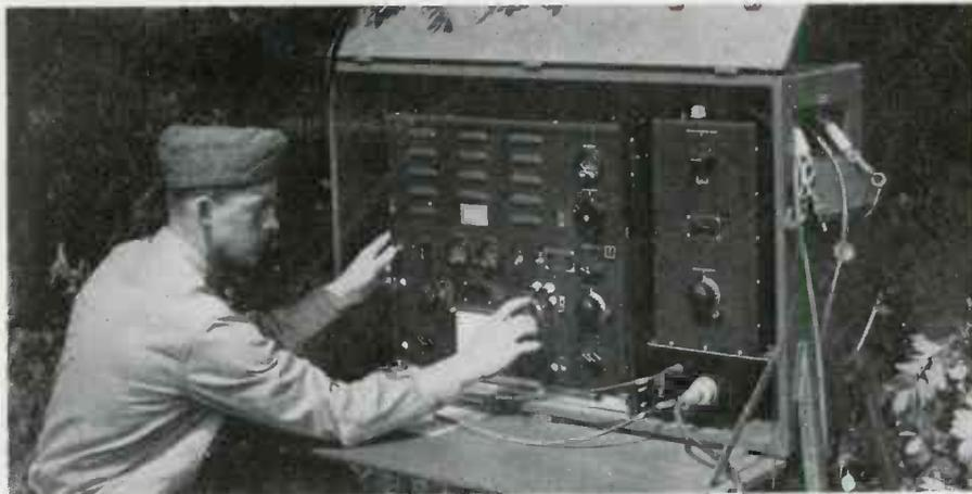
A close-up of Signal Corps' transmitter BC-191-C
