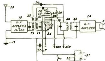
such a way as to keep amplification constant. An inverse feedback circuit deriving its potential from anode 19 may be added. The potential of control grid 20 can be supplied by a rectified output signal, e.g., if pass range adjustment for control of background noise or needle scratch suppression is desired. H. Boucke, Patents Research Corp., (F) March 29, 1940, (I) March 30, 1943, No. 2,315,043.
