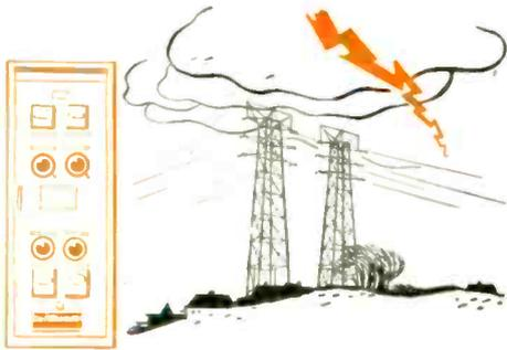
**Carrier-Current Relaying**—One of the most important electronic applications in the power transmission field. Carrier signals permit simultaneous high-speed tripping of both circuit breakers in from one to three cycles. This high-speed clearing of faults by electronic methods improves system stability and increases loads that can be carried safely.
