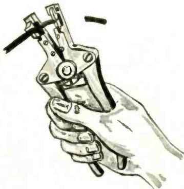
model is available with "hold-open feature" for stripping fine stranded wires. It automatically holds jaws open until wire is removed, and strips without crushing. Manufactured by Wood Specialty Manufacturing Co., Rockford, Ill.
