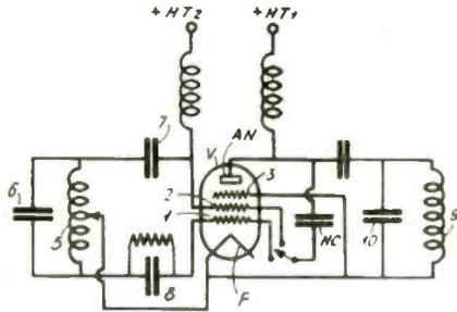
tralizing capacity NC may be inserted. The oscillations generated may be modulated by applying potentials to grid 1, grid 2 or to plate AN. Alan D'Arcy Hodgson, RCA, (F) Oct. 10, 1931, (I) March 9, 1943, No. 2,313,071.
