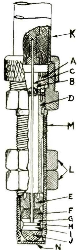
Fig. 3. A piezo pressure gage for cylinder combustion measurements
