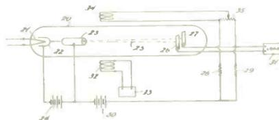
condition, the potential difference existing between plates 26 and 27 will be directly proportional to the signal. With this arrangement, no variation from the controlled means is reflected back into the signal source and comparative independence of any change in the components of the device are obtained. Other deflecting means
