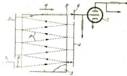
electrodes 4, 5 and collecting plate 6. A uniform magnetic field having a direction indicated by arrow H is provided. Under these circumstances, the electrons move along track P and a time delay dependent on the potential difference between deflecting electrodes 2, 3 is obtained. It is possible, with the device, to mix signals with varying time delay. G. S. P. Freeman, Electric & Musical Industries, Ltd., (F) July 5, 1941, (I) Feb. 23, 1943, No. 2,312,033.
