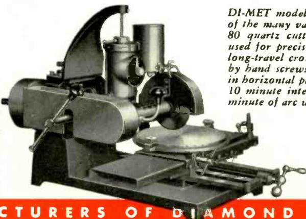
*DI-MET model 80 with HVCT-12 Rotary Table — One of the many variations of the versatile DI-MET model 80 quartz cutting machine. HVCT-12 Rotary Table, used for precision orientation of the quartz piece, has long-travel cross and through-feeds manually operated by hand screws. Table tilts to  $\pm 10^\circ$  and rotates  $360^\circ$  in horizontal plane. Vertical adjustment is graduated in 10 minute intervals, horizontal adjustment reads to 1 minute of arc with vernier.*
