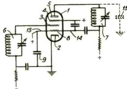
and to the output electrode via lead 14. In a preferred embodiment, cathode 2 is connected to the anode side of suction grid 8 instead of to its control grid side. G. H. P. Alma, M. J. O. Strutt and A. van der Ziel, Alien Property Custodian, (F) May 9, 1941, (I) March 30, 1943, No. 2,314,916.
