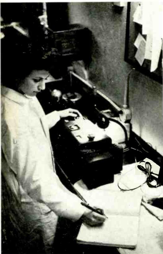
UNABRIDGED SPECTROPHOTOMETER measures light transmission of sample at all wavelengths for most accurate vitamin assays. Diagram of electronic null-point system of Beckman unit below
