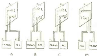
planes are at right angles to one another, and present a slope of 45° or 135° with the horizontal. In this way, the master station may communicate with any of the satellites. For stations A and B to communicate with one another, it is only necessary for station B to rotate its antennas 180° about a vertical axis. E. Gerhard, Alien Property Custodian, (F) May 31, 1941, (I) Feb. 16, 1943, No. 2,311,435.
