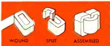
This split-core construction saves valuable man-hours because there are only 2 or 4 pieces to assemble around the windings.
