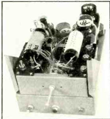
Series 20, 4 channel 1600-6000 K.C., 20 watt transmitter.
