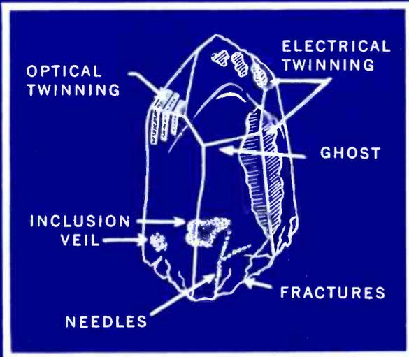
COMMON IMPURITIES IN THE MOTHER OR NATURAL CRYSTAL CAN BE DETECTED WHEN A LIGHT IS PASSED THROUGH THE CRYSTAL.
