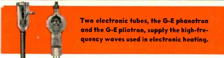
**Two electronic tubes, the G-E phanotron and the G-E pliotron, supply the high-frequency waves used in electronic heating.**
