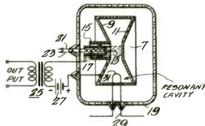
shown, the cavity electrode is maintained at a positive potential and serves as anode. Distance between cathode and effective anode must be such that the electron transit time is less than a half period. E. G. Linder, RCA, (F) June 25, 1940, (I) March 23, 1943, No. 2,314,794.
