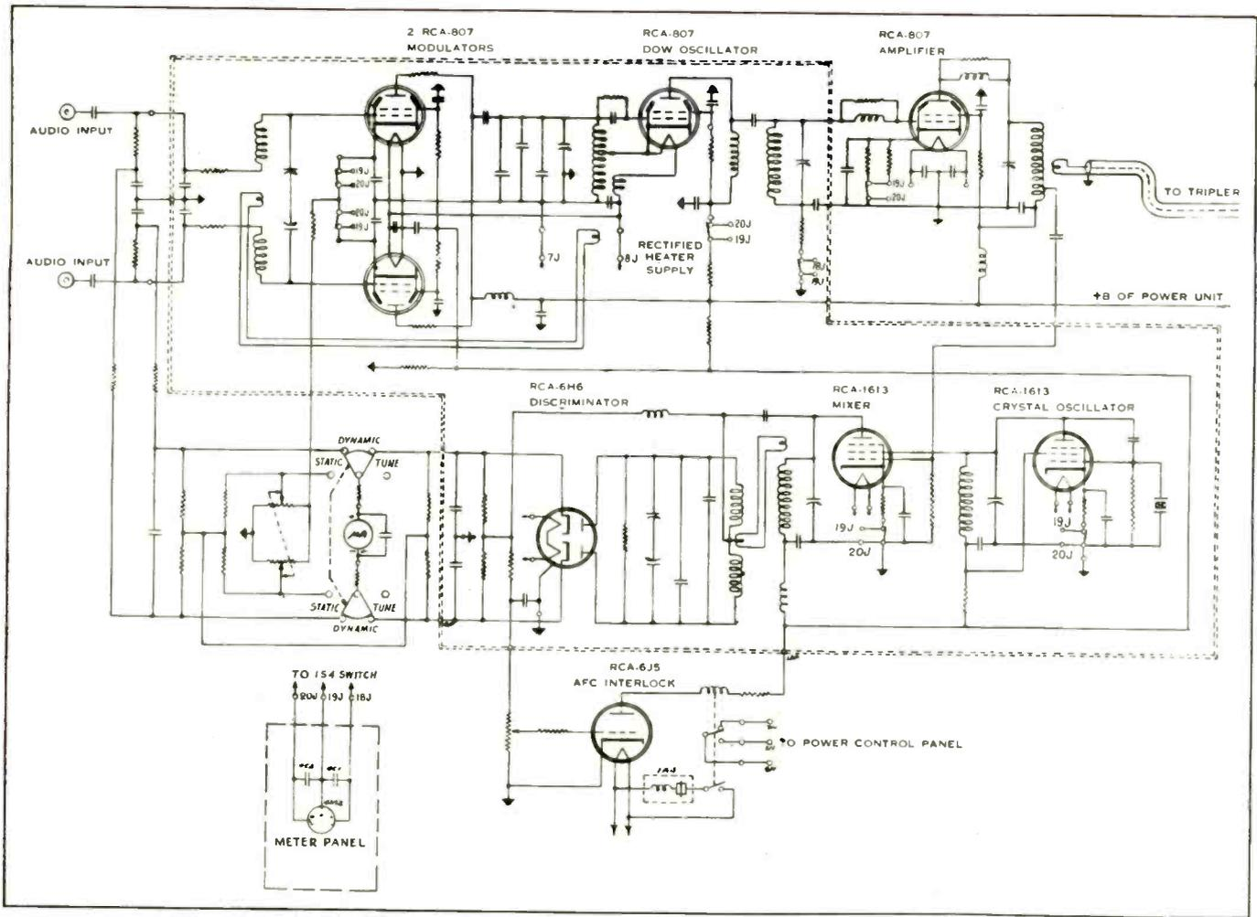
THE HEART of the system is the frequency modulated oscillator, with its automatic carrier stabilizer, all kept at a constant temperature for frequency stability
