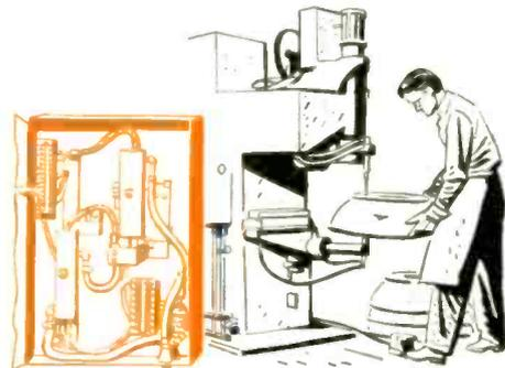
**Accurate Welding Control**—The use of small Ignitron tubes has practically eliminated mechanical contacts for resistance welding. In the Westinghouse power switch, Weld-O-Trol, action is instantaneous. Speed of current interruption is 600 or more times per minute. The two Ignitron tubes in each Weld-O-Trol are guaranteed for a year and have consistently held up for much longer periods.
