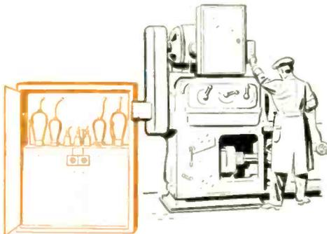
**Speed Control**—By converting a-c power to direct current with thyatron tubes, Westinghouse has developed small, compact speed control units for d-c motors without using rotating equipment for current supply. Direct current is supplied by the tubes to the armature and field of the d-c motor. Both armature and field circuits are controlled by one dial on the Westinghouse Mot-O-Trol.
