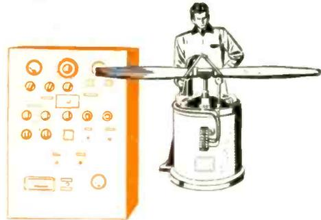
**Vibration Fatigue Tests**—Only through electronics has it been possible to build vibration testing equipment that will deliver from 10 to 10,000 cycles per second. Employing the principle of the dynamic radio speaker, Westinghouse engineers have developed vibration fatigue equipment that has opened the way for tests that could not be made with existing mechanical methods.
