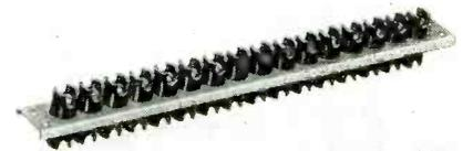
clearances and leakage distances for circuits carrying up to 300 volts, 20 amperes. Center to center distance between terminal units is  $\frac{5}{8}$  in. Maker is Curtis Development and Mfg. Co., 1 No. Crawford Ave., Chicago, Ill.
