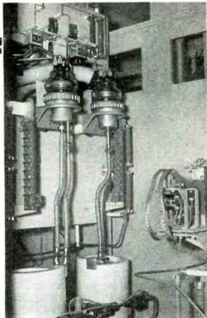
The RCA type 880 modulator tubes are capable of supplying on maximum demand about 65,000 watts audio power
