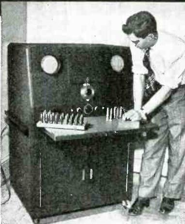
GOOD bad GOOD GOOD bad... 6,500,000 bullets, rejected because of a mix-up in copper cladding measurements, were re-sorted by the DuMont Cyclograph... 99% of them salvaged!
