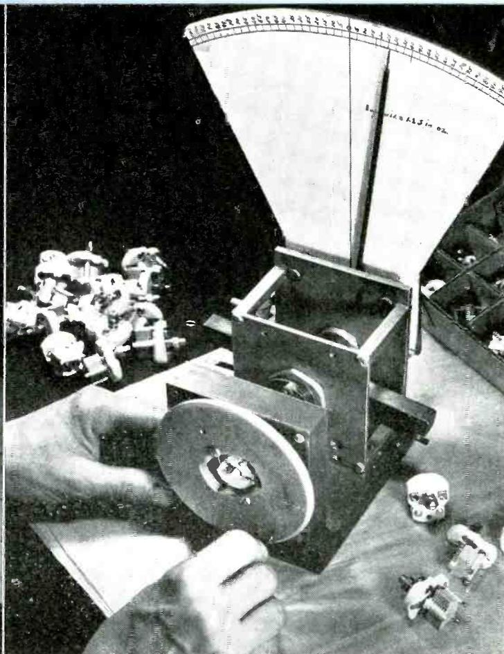
Special torque and smoothness tester for midget APC's (air padding condensers) was hurriedly improvised from old radio and condenser frames a year ago and has been in constant use ever since, testing four to five thousand condensers a day as opposed to only two hundred by old method. Condenser is plugged in at front. Spring-loaded scale reads inch-ounces torque
