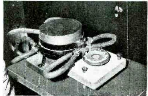
A 20-kw. Ajax-Northrup tube converter provides power for hardening sprocket teeth above. Below, 6-kw. spark-gap set hardens ordnance part in 35 seconds.
