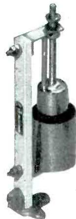
Type N neutralizing condensers in 5 sizes
