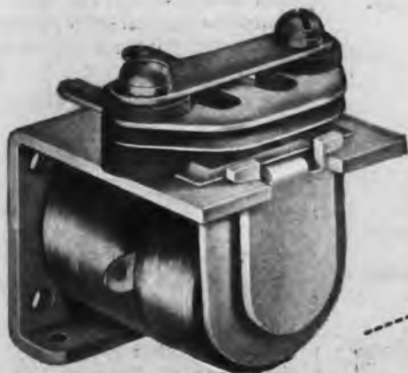
The F relay shown is a single pole, single throw normally open combination. The standard contacts carry three amperes at 24 volts DC or 115 volts AC non-inductive. Bakelite insulation is used. May be supplied on other contact combinations. Silver is standard contact material, alloy contacts can be substituted. The F is 1\ 11/32 " high, 1\ 3/16 " wide and 1\ 3/32 " long. Weight is 1\ 1/2 ounces.
