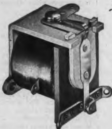
The E relay illustrated is a single pole, double throw arrangement. The standard silver contacts are capable of carrying one ampere at 24 volts DC or 115 volts AC non-inductive. Insulation is bakelite. Alloy contacts are available. Other contact arrangements may be furnished. The E is 15/16 " high, 1\ 1/16 " wide and 1\ 1/16 " long. Weight 1\ 1/2 ounces.
