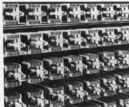
(Left to right) The operator punches the problem data on tape, which is fed into the computer. The solution emerges in the teletype receiver. Relays which figure out the problem look like your dial telephone system.
