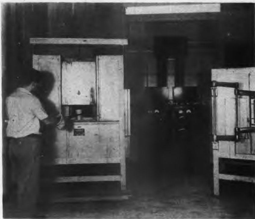
Fig. 13. High temperature firing of phosphor materials in inert atmosphere
