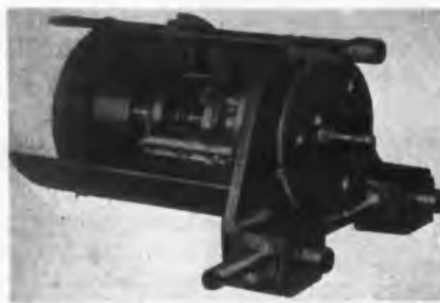
Photograph of coaxial butterfly oscillator with lighthouse tube mounting (left end) and geared rotor drive (at right end). Cross sectional view of this oscillator is shown below
