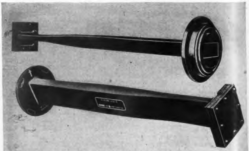
Fig. 7. Views of both ends of the wave guide. Waves coming out of the guide are reflected by flat end plate through oval holes toward parabola
