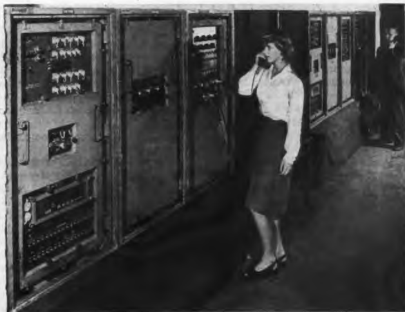
Fig. 1. Multiplexing and pulse positioning equipment is mounted in racks shown below
