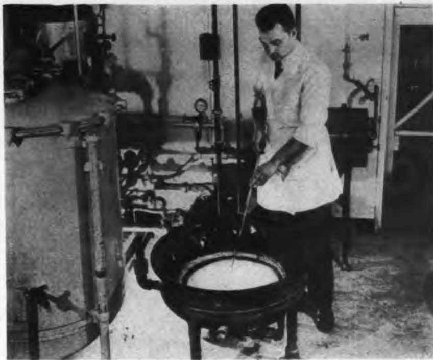
Fig. 12. Kettle being used by author to mix phosphor components
