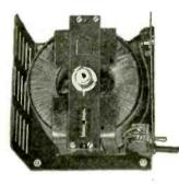
The dielectric strength of Formex magnet wire is high and stays high, during the entire life of your apparatus. For tighterpacked, lighter-weight, lower-cost coils, specify Formex magnet wire, either regular or colored. It's suitable for operation in ambient temperatures up to 105 C – also for jobs where moisture and solvent resistance are needed. Round Formex from 8 Awg to 40 Awg, ultra-fine from 41 Awg to 50 Awg, and rectangular in a full range of sizes. (Bulletin GEA-3911)
