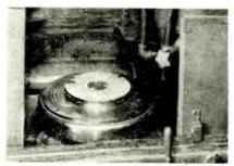
Small parts on magnetic chuck ready for grinding
