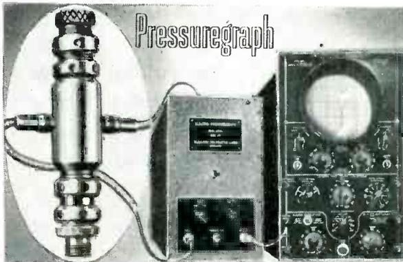
Covers wide range of engine speeds and pressures up to 10,000 p.s.i. Screws into cylinder and can be calibrated using static pressures. Vibration-proof. Accurate, dependable for frequent engine tuning. **SIMPLE OPERATION — ONLY ONE CONTROL.**
