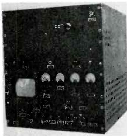
Wide range double heterodyne spectrum analyzer covering 10 to 3000 megacycles
