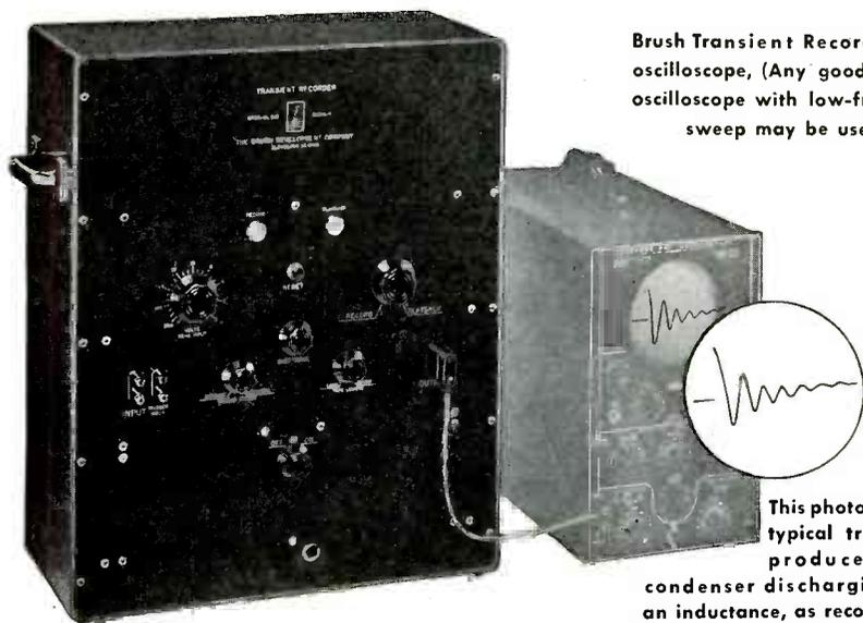
Brush Transient Recorder with oscilloscope, (Any good quality oscilloscope with low-frequency sweep may be used.)
