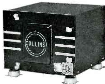
**THE 180K-1** antenna loading unit efficiently transfers the power output from the 18S-1 to any standard commercial fixed antenna. Remote controlled, pretuned operation for ten channels is provided. The nominal input impedance is 50 ohms. Weight, 10 lbs. Size, 7½" h, 10½" d, 12" l.
