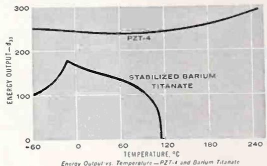
Energy Output vs. Temperature—PZT-4 and Barium Titanate
