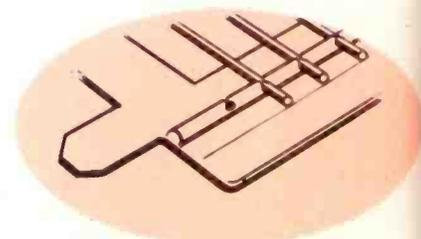
**B** Sylvania's new Framelok construction eliminates brazing and adapts the frame grid to automatic production. Grid halves are perfectly flat—free from thermal strains.
