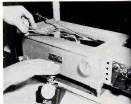
GE has developed a new copper clad glass epoxy laminate, Textolite 11558, reportedly capable of passing any dip solder specification in the industry. Here new laminate is tested in solder pot at 500° F.
