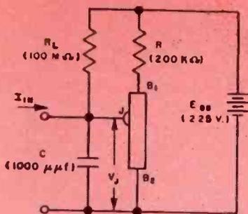
Fig. 1: This silicon double-base diode free-running oscillator was investigated.
