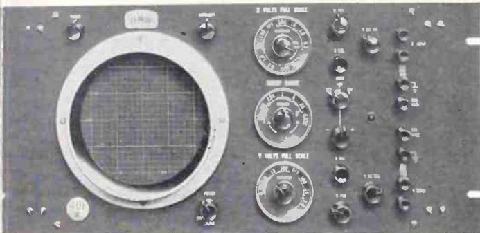
Identical in every electrical respect to its industry standard counterpart, the 401-R is physically rearranged for insertion into standard 19" relay racks. For quantitative and qualitative studies within the dc to 100 kc bandwidth, the 401-R offers important advantages in an easy-to-use configuration for panel operation. Some of these features... not available in other rack mountable units... are:
