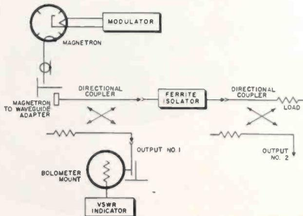
With this technique, the measured insertion loss includes the true resistive losses of the ferrite component, as well as the energy loss due to reflection at both the input and output of the isolator. It should be noted that a VSWR as high as 1.2 contributes .05 db to the insertion loss measurement. In all but very special cases, we consider an input VSWR of 1.15 as acceptable, which contributes less than .05 db to insertion loss of the ferrite device.
