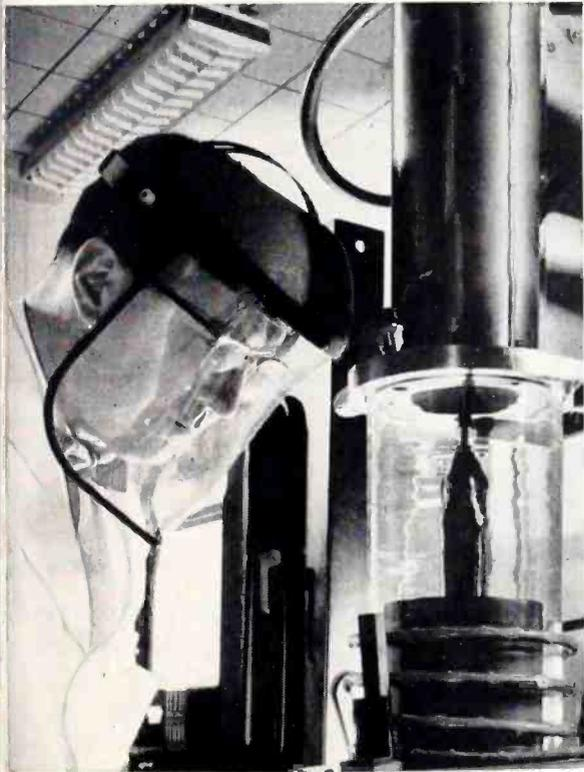
In the center of the quartz housing, a germanium crystal is being grown. A "perfect crystal lattice," it will be cut into wafers  $3/10$ ths of an inch square and less than  $1/100$ th of an inch thick to become the heart of Delco High Power transistors.
