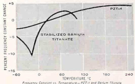
Frequency Constant vs. Temperature—PZT-4 and Barium Titanate
