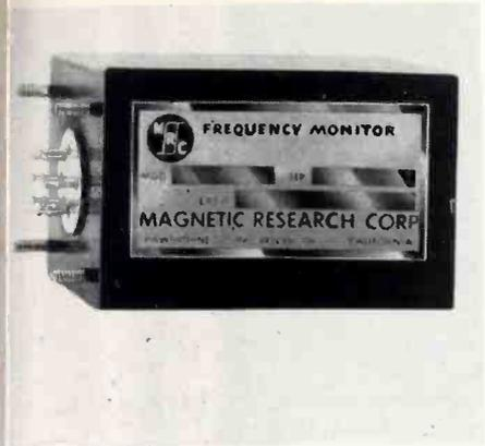
intended for telemetering instrumentation. The units produce a well filtered 0-5 vdc output voltage in response to a frequency deviation. Two representative models of the new line are the FD-400 for 400 CPS power sources and the FD-2000 for inverters operating at 2000 CPS. Frequency discriminators are available for frequencies up to 10 kc. Magnetic Research Corp., Hawthorne, Calif.
