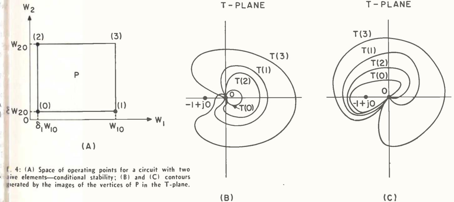
Fig. 4: (A) Space of operating points for a circuit with two active elements—conditional stability; (B) and (C) contours generated by the images of the vertices of P in the T-plane.
