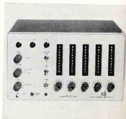
40,000 cps can be selected in 1 cps increments. If frequency is below or above limits, a light lights. Computer-Measurements Corp., 5528 Vineland Ave., N. Hollywood, Calif.
