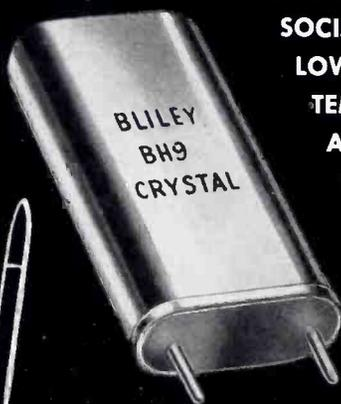
TO SOLVE THE RELIABILITY PROBLEMS ASSOCIATED WITH THE OPERATION OF LOW FREQUENCY CRYSTALS AT HIGH TEMPERATURES, BLILEY HAS DESIGNED A COMPLETELY NEW MOUNTING STRUCTURE. UTILIZING SPECIAL TECHNIQUES, THE CRYSTAL IS SUPPORTED BY A TINY SAPPHIRE ROD WHICH IS FUSED TO THE QUARTZ PLATE. THIS NEW MOUNTING STRUCTURE ASSURES RELIABLE PERFORMANCE AT TEMPERATURES UP TO 185°C. SUPPLIED FOR THE FREQUENCY RANGE 40 KC TO 600 KC— COMPLETE DESIGN SPECIFICATIONS MAY BE SECURED BY REQUESTING BULLETIN #511.
