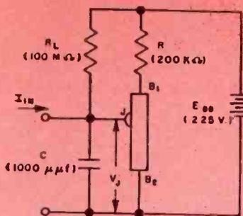
Fig. 1: This silicon double-base diode free-running oscillator was investigated.
