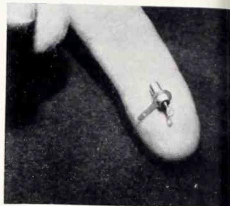
involved. It can be used for isolation purposes, electronic switching, RC timing circuits, relaxation oscillators, etc. It has high input resistance before a critical voltage is reached, at which time the new diode "breaks down" and becomes a very low resistance. Available in a wide variety of characteristics. The Victoreen Instrument Co., 5806 Hough Ave., Cleveland 3, O.
