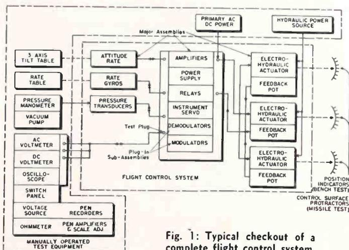
Fig. 1: Typical checkout of a complete flight control system.
