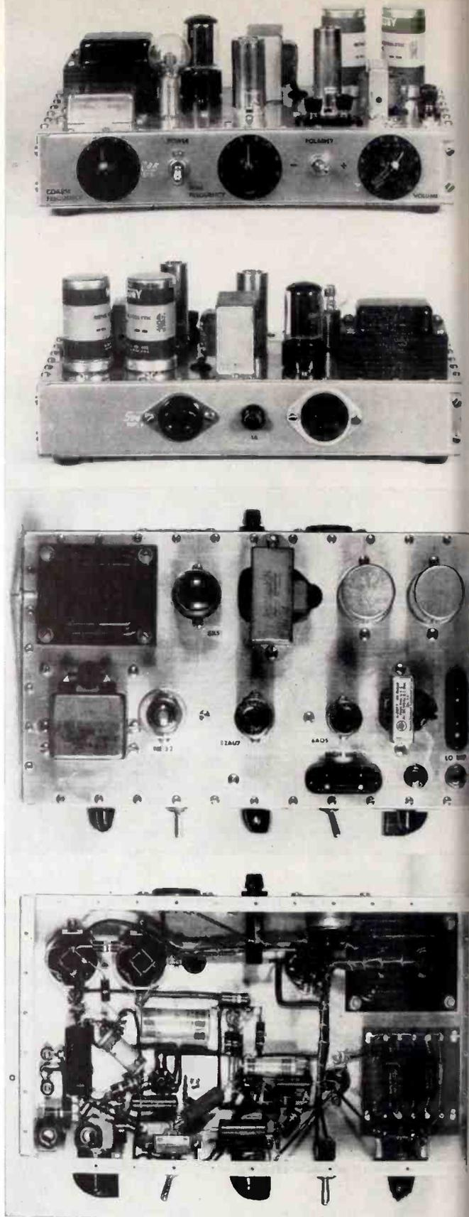
Fig. 3: The above photographs clearly indicate the location of components and controls of the prototype neon pulser. The author comments, "Major components in this pulser are substantially immortal, and should outlast the builder. The electrolytic condensers, being rated at 450 volts, and used at less than 350 volts maximum, have a life measured in years of use, and approximately two years idle."
