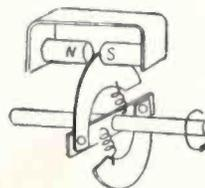
the centrifugal force, against the two springs. However, by moving outwards they penetrate more deeply inside the magnetic field produced by a permanent magnet.
