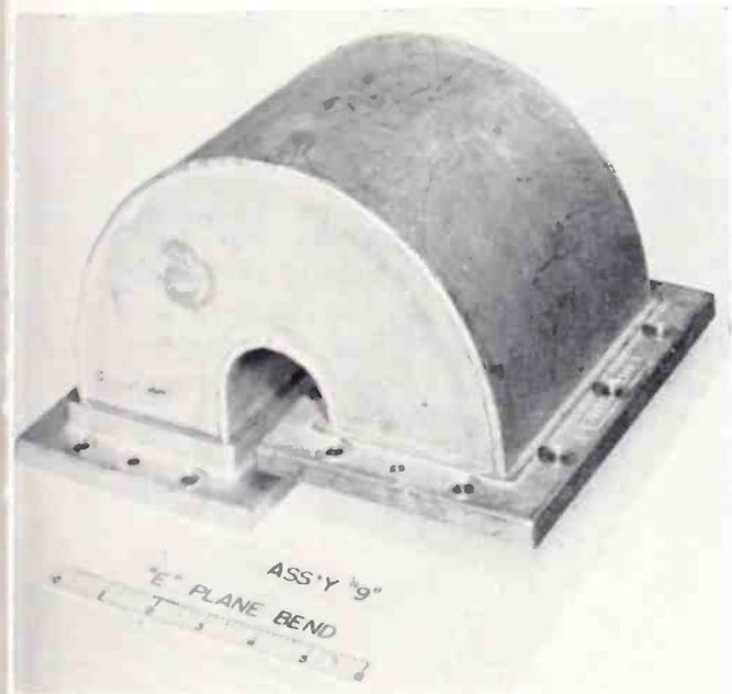
Fig. 6: Slight gaps in waveguide wall at butt welds cause no trouble.
