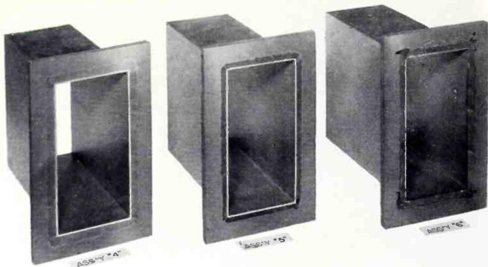
Fig. 3: Heli-arc welded at the flange face, followed by a 1/32-in. face cut.
