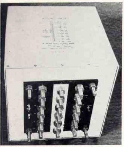
minutes. Output voltages range from 0.2 to 230 v., and performance is maintained for any condition of loading, from open circuit to 100 w. total of loads on all windings. Approximately 500 separate conductors in series and parallel combinations are assembled in a Litzendraht type cable in order to achieve the proper degree of each winding among all the others. Osborne Electronic Corp., 712 S. E. Hawthorne Blvd., Portland, Ore.
