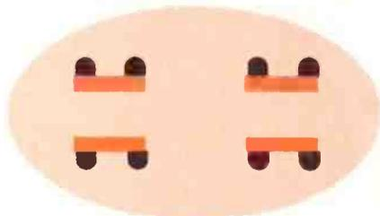
Mica slots are designed with flat alignment surface and channel index to position grids with much greater precision. Closer element spacings are possible where extra Gm is required.
