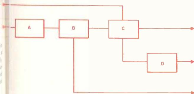
MODE 1 CONSISTS OF COMPONENTS A, B, AND C IN SERIES
