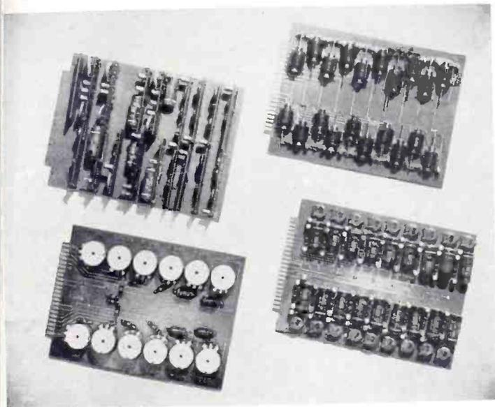
Fig. 3: These are the four basic plug-in panels used in the all-electronic digital display unit.
