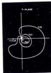
A criterion of stability is derived for calculating the stability margins of multiple loop structures. It is directly applicable to vacuum tubes, and to junction transistors in certain configurations.
