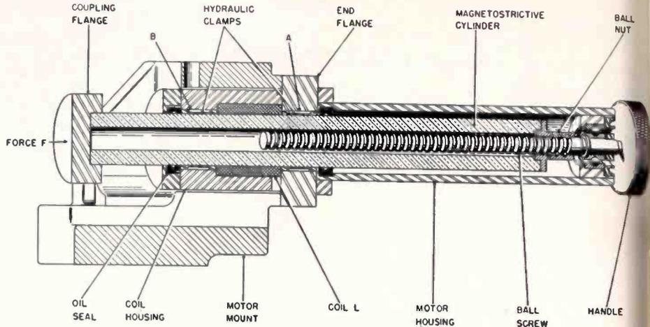
Fig. 1: The Inchworm linear actuator provides micro-inch dimensional control of delicate machine operations. One noteworthy application is in centerless grinders.
