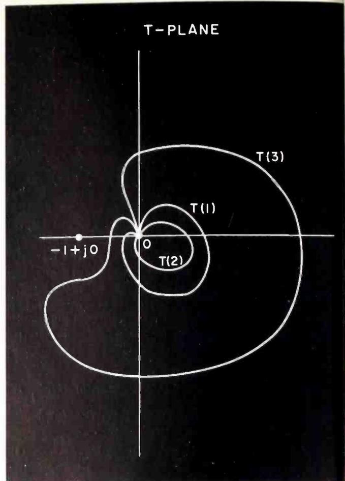
Fig. 3: Contours generated by images of vertices of  $P$  in  $T$ -plane
