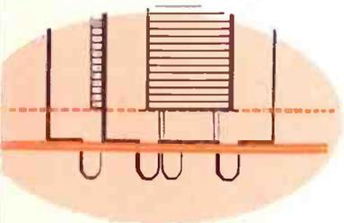
Self-alignment is accomplished in the Framelok Grid through precise control of the distance between the mica and the first grid lateral wire. These tolerances in the frame grid are held in the order of one tenth of one thousandth of an inch—considerably tighter than ordinary grid tolerances.
