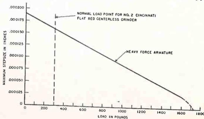
Fig. 2 (left): This is a plot of step size versus load for the new magnetostrictive motor.
