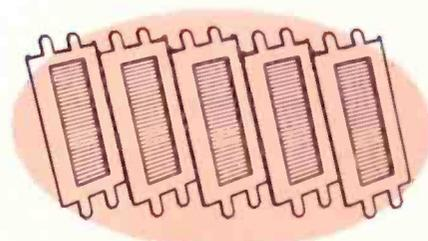
Sylvania's unique technique of frame grid construction makes it possible to duplicate grid after grid. More uniform spacings produce a more uniform electrostatic field in the tube.
