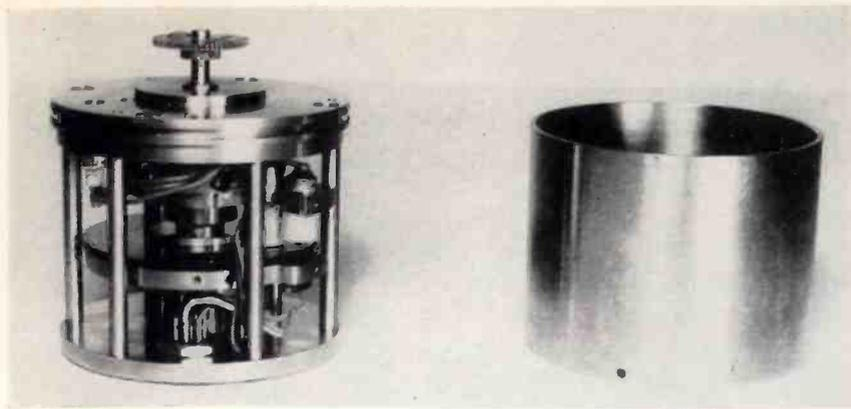
Fig. 1: The encoder with cover removed. It measures 3 inches in diameter by 2½ inches in length and weighs approximately one pound.
