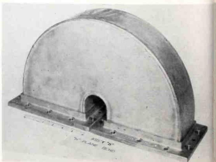
machined (lands, grooves, bolt holes) as a detail part. Whereas the flange machining for the brazed assembly must take place after the joint is made. The pre-machined flanges are considerably less costly since they can be easily done in a repetitive manner while post assembly flange machining is expensive because of the difficulty of handling and fixturing large waveguide assemblies.
