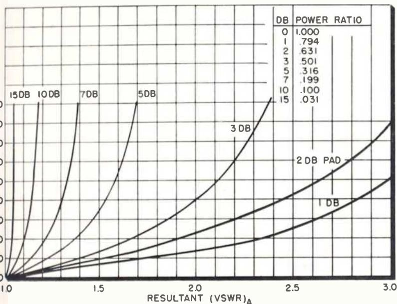
The expression  $(VSWR)_B$  in eqns. 7 and 8 would then be either the maximum or minimum value possible, depending on whether the reflections add in or out of phase. Although this analysis is more exact, eqns. 7 and 8 are sufficient for accuracies in the order of 1% when the pad VSWR is less than 1.2.
