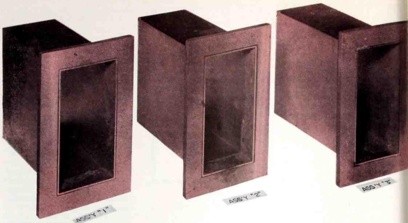
Fig. 1: These assemblies were torch brazed at the flange face.
