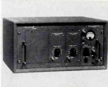
the new series features high sensitivity, reduced size and elimination of plug-ins. Model 7570 serves as a preamplifier of 1 mv. sensitivity in the 10kc to 10 MC range. Models 7571 and 7572 are heterodyne units with 10 to 110 MC and 110 to 220 MC ranges, respectively. Berkeley Div. Beckman Instruments, Inc., 220 Wright Ave., Richmond 3, Calif.
