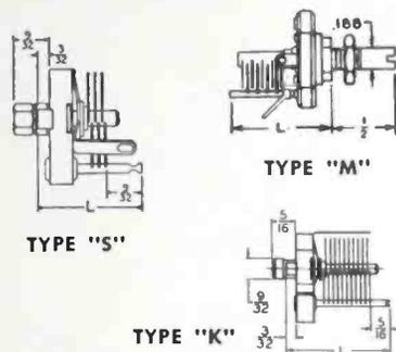
**TYPE “S” CAPACITORS**—The Type “S” Capacitor falls midway between the type “M” and “K” capacitors in physical size. Peak voltage rating 850 volts—plate spacing .013", other spacings available on special order. Square mounting studs tapped 4-40 on  $17/32$ " centers.
