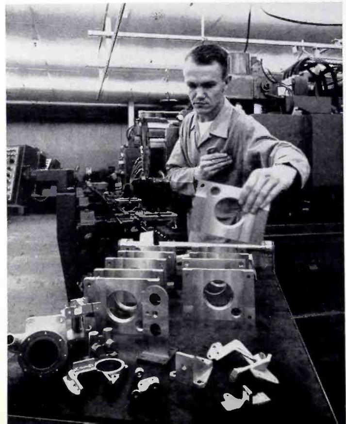
Fig 8: All the machined parts shown here can be made simultaneously on the electronically controlled line of tools developed by Hughes and the Kearney and Trecker Corp.
