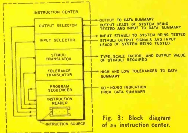
Fig. 3: Block diagram of an instruction center.
