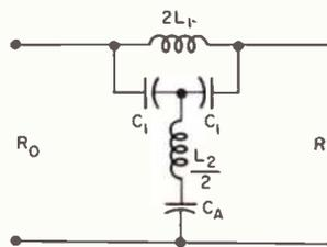
$$C_A = \frac{2C_1 C_2}{(C_1 - C_2)} = \frac{2dC_2}{(d-1)} \quad (11)$$
