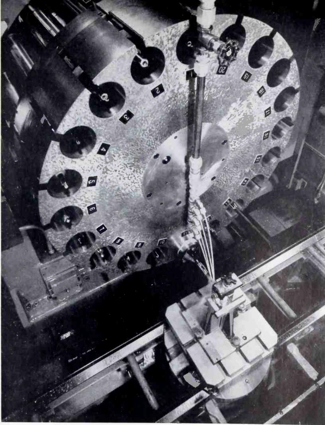
Fig. 1: Twenty different drills, taps, reamers, etc., can be set up at once on this machine. The appropriate one is chosen, positioned, and operated from punched tapes.
