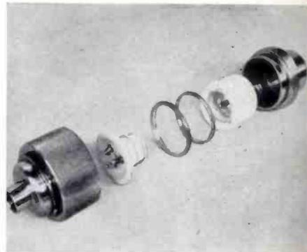
ing connector for 3 #8AWG wire, metal jacketed and mineral insulated cable. It is of special value where it may be necessary to frequently and quickly connect and disconnect large conductors. It has met environmental tests of 1,000° F., 100,000 ft. plus altitudes, 560 v. corona starting voltages and 960 v. flashover voltage. Concentric ring design eliminates alignment problems. AMP Inc., Harrisburg, Pa.
