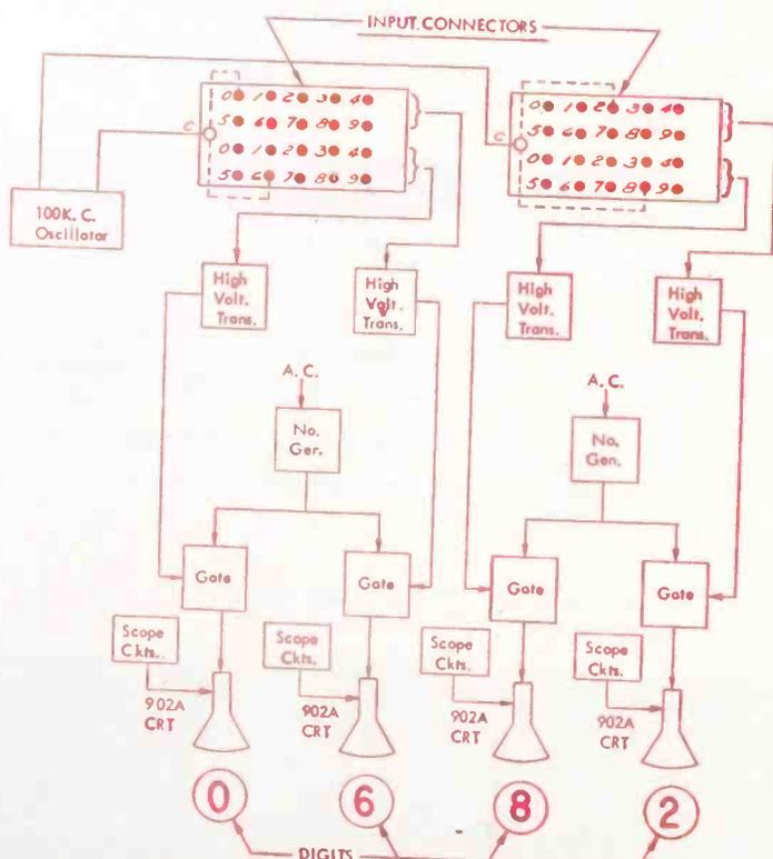
Fig. 2: Block Diagram, Hoffman digital readout Model DR-4C.
