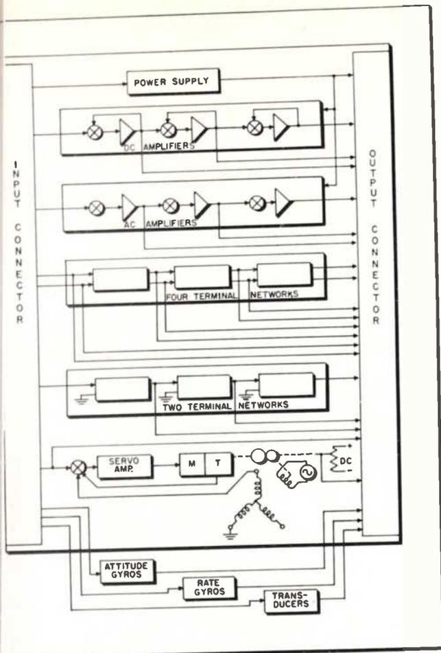
Fig. 6: Complete checkout automation requires a self-test sub-system.
