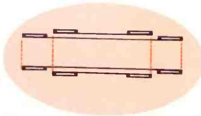
**A** Straight line geometry of grid side-rods in present grids is considerably weaker than the double-box configuration formed by frame grids. Distortion due to mount "twist" is virtually nonexistent in the frame grid structure.
