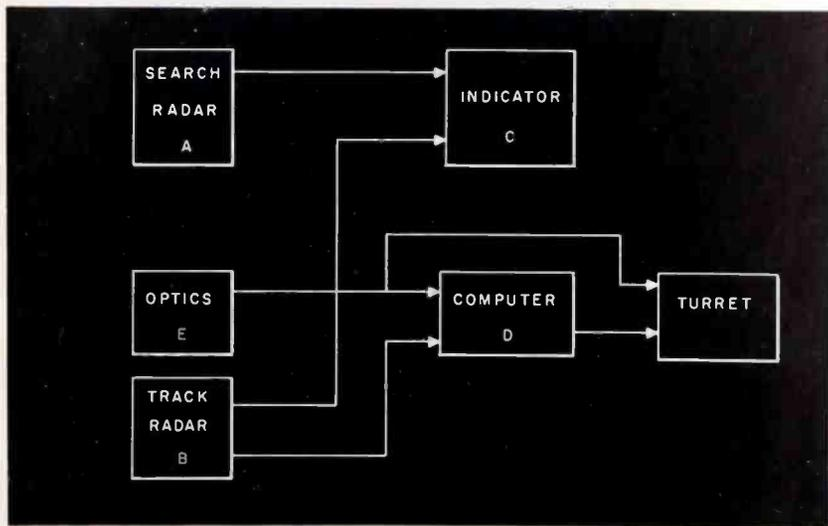
Fig. 2: Block diagram of hypothetical multi-mode fire control system.
