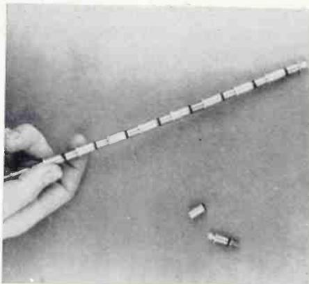
pensive threaded bushings to form simple assemblies for kilowatts of rectified power. The individual unit is sealed and threaded at each end, so it can be screwed into the bushings, or into a chassis "heat sink," or plugged into a clip holder. Unit is 1 in. long with an inverse rating of 400 v. and maximum forward current of 750 ma. Audio Devices, Inc., 620 E. Dyer Rd., Santa Ana, Calif.
