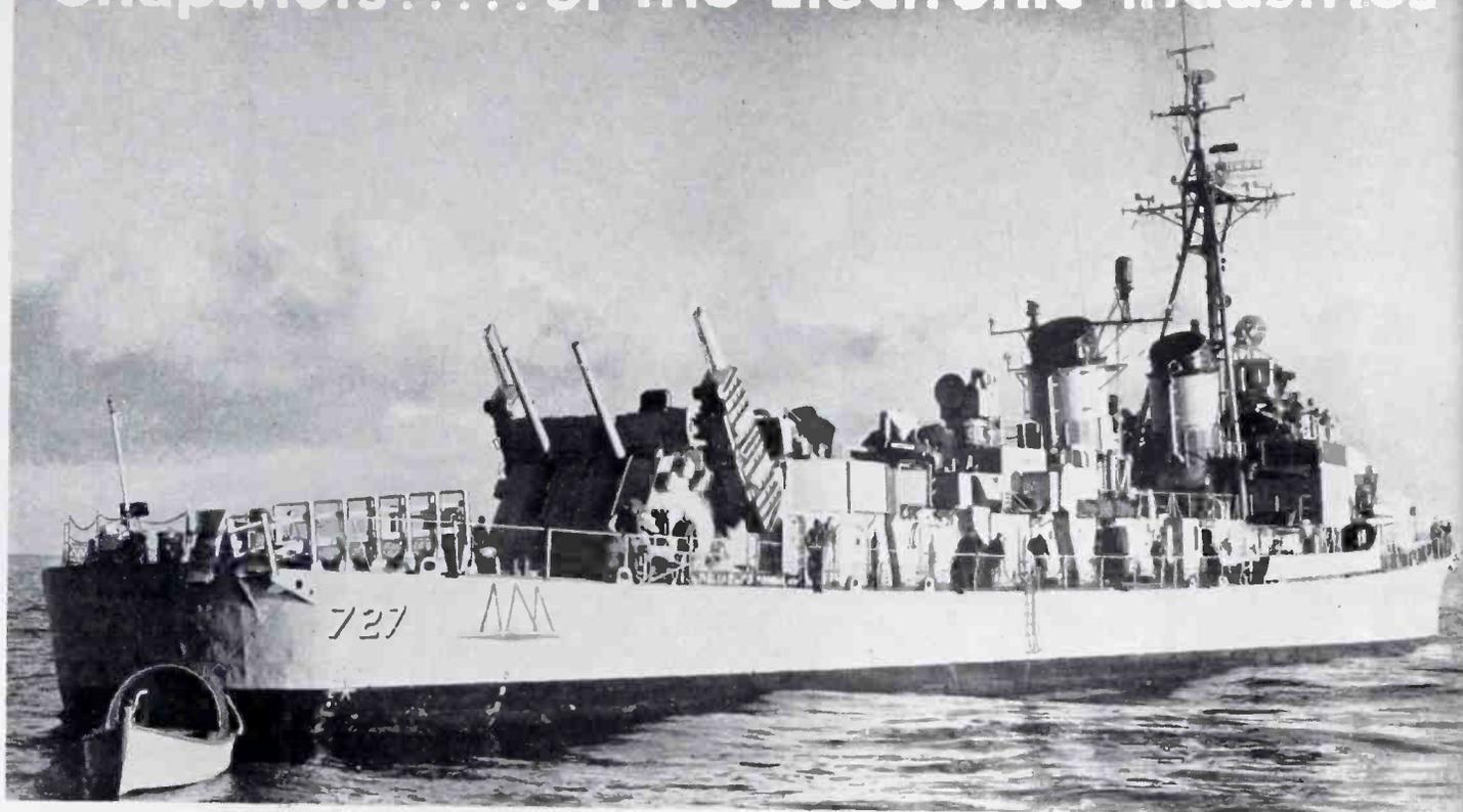
Launcher for RAT, Navy's new rocket-propelled, anti-submarine weapons system, is shown mounted on destroyer's aft 5-in. gun turret.
