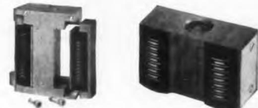
**Gap-Mounted**—Contains two head cartridges, easily removed and replaced with no close adjustment. Bracket, cartridges have lapped surfaces providing reference positions to gap perpendicularity, azimuth and contact adjustment.
