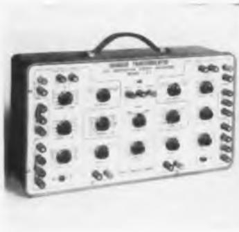
high power audio output can be simulated with the LF-1. Common or grounded emitter, base, or collector circuits may be simulated using pnp, npn, or surface barrier transistors. Built-in battery voltage supply for separate bias and load. Switch reverses polarity. Almost any external connection can be made at the 5-way binding posts provided. Sprague Products Co., North Adams, Mass.
