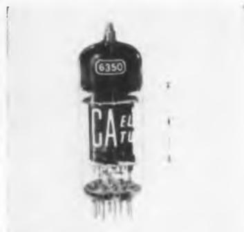
other "on-off" control equipment is available. The 6350 maintains its emission capabilities even after long periods of operation under cut-off conditions. Balance of cut-off bias between the two units of the tube is closely controlled during manufacture. It has separate terminals for each cathode and a mid-tapped heater for a 6.3-volt or 12.6-volt supply. Radio Corporation of America, Harrison, New Jersey.
