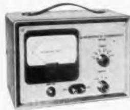
**WV-84B Ultra-Sensitive DC Microammeter**—popular choice for industrial, chemical, and general laboratory applications. Designed to measure currents from 0.0002 to 1000 microamp. Can be used as ohmmeter to measure resistance in the order of billions of ohms. Self-contained batteries permit use for field applications. Low current drain tubes extend battery life; meter protected from accidental overloads. \$110.00\* (less batteries)
