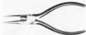
"dead" soft wire cleanly. The shear blade is removable and may be easily replaced if it becomes worn. The reverse side has a milled section behind the knife so designed that when the wire is cut, it is held in position and a turn of the hand forms a hook in one operation. Furnished standard with self-opening coil spring. Mathias Klein & Sons, 7200 McCormick Rd., Chicago 45, Ill.
