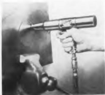
tic materials are involved. Tests were made on hard thermo setting and thermo plastics as well as on rigid "Vinylite," cellulose acetate, polystyrene, fiberglass reinforced plastics, and "Plexiglas." Operating speed and cutting stroke of the saw are easily adjusted. Only two moving parts means long saw life. Air-Speed Tool Co., 1502 W. Slauson Ave., Los Angeles, Calif.
