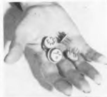
hermetically sealed to 95% Al<sub>2</sub>O<sub>3</sub> by brazing with silver, copper or nickel gold. The new line of solid pin headers is expected to find application where high reliability, exceptional uniformity and severe environmental conditions are encountered. General Ceramics Corp., Kearsbey, N. J.
