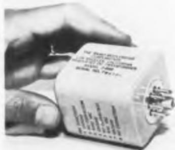
in epoxy resin and sealed. Operates over ambient temperature range of  $-55$  to  $71^{\circ}\text{C}$ . Unaffected by extremes of shock and vibration. Package operates on 24 to 32 vdc. input and delivers 900 vdc. at 30  $\mu\text{a}$  within 3%. Output ripple is regulated within 3 v. peak to peak. The entire unit is integrated in a 2 x 2 3/4 in. package. The Ramo-Wooldridge Corp., P. O. Box 8405, Denver 10, Colo.
