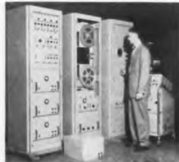
ity to record as many as seven channels, up to 2½ MC on each channel, simultaneously, on ½ in. tape. Minnesota Mining & Mfg. Co., 11701 Mississippi Ave., Los Angeles 25, Calif.
