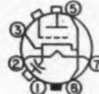
UHF triode (disk-seal type) with internal capacitor. Tube terminals added as shown where desired
