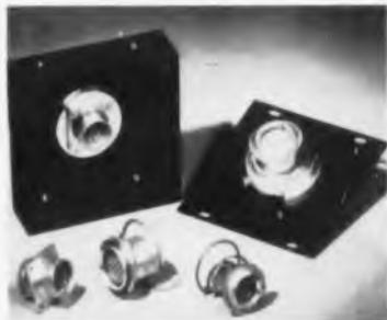
DM6502 plugs mate with receptacles to provide self-aligning connectors that are environmentally sealed. They mate with DM9606 square flange receptacles in 7, 19, 37 and 61-pin arrangements and with DM5600 miniature hermetic receptacles in 7, 19 and 37-pin arrangements. Plugs meet applicable AN "E" requirements and the latest revision of MIL-C-5015 requirements. Deutsch Co., 700 Avalon Blvd., Los Angeles 3, Calif.
