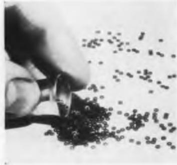
signal and fast switching speed for a low-drive core. HCA-222M1 core is made of a special ferromagnetic spinel. Functioning in a coincident current memory, it will produce an undisturbed "1" output signal of 64 mv. peak, a disturbed "0" output signal of 8 mv. peak and a switching time of 2.1 sec. when subjected to a typical driving current of 400 ma. RCA, Camden 2, N. J.
