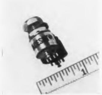
Mechanical Specs.: 1 piece machined metal case; stainless steel shaft; self-contained locking device; mechanical rotation, 330° nominal; size, 1/2 in. dia. x 5/16 in. Electrical Specs.: heat dissipation, 2 w. at 60° C; voltage breakdown, 1,000 vdc; electrical angle, 325° nominal; resistance tolerance, ±5%. Ace Electronics Associates, Inc., 99 Dover St., Somerville, Mass.
