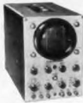
**WO-91A-5" Oscilloscope**—4.5-Mc scope, choice of wide-band or high-sensitivity operation for waveshape observation and measurement, signal tracing and alignment of chrominance circuits and wide-band amplifiers—voltage-calibrated, frequency-compensated, vertical-input attenuator and calibrated graph screen make possible direct voltage readings as easily as with a VTVM. \$239.50\*
