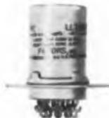
relay remains in "energized" position indefinitely without consuming power. As an overload relay it can be electrically reset from a remote position. Contacts can be closed by one circuit and opened by another. It has many applications in fail-safe circuits. Its small size, light weight and hermetically sealed enclosure make possible its use in airborne and other equipment. Either coil may be energized continuously without damage to the relay.
