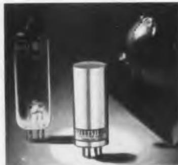
shock, are now in production. The 6X4, a direct replacement for the 6X4 full-wave high vacuum rectifier tube, features an output of 85ma. dc maximum, an input of 400 v. RMS., and a max. peak current of 225 ma. Maximum PIV is 1250 v.; the voltage drop 6 v. at 70 ma. International Rectifier Corp., 1521 E. Grand Ave., El Segundo, Calif.
