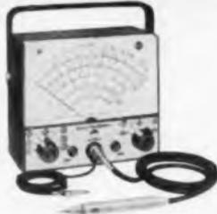
**RCA WV-98A Senior VoltOhmyst**...time-proved performance, "workhorse" of the VoltOhmyst line. Large, easy-to-read wide-vision meter (6½" w). Features: direct peak-to-peak readings of complex waveforms, accuracy of ±3% full scale on both ac and dc voltage measurements. Complete with sturdy single-unit WG-299C DC/AC Ohms Probe and Cable, ground cable, alligator clip, clip insulator, instruction booklet. \$79.50\*
