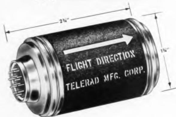
This miniature acceleration operated switch is designed for missile applications requiring positive switch functions at first motion, during, or after boost. Versatile locking arrangement permits cycling or recycling of switch during various phases of flight (requires 30 watt signal). It is conservatively rated and is designed for expendable one-time use.
