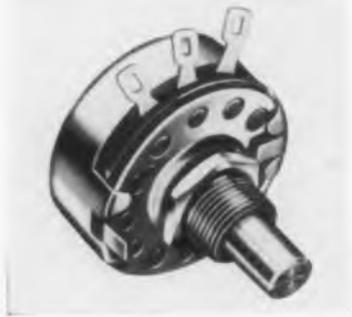
A, B, S, and DB resistance rotation characteristic tapers in nominal values up to a maximum of 5.0 megohms total resistance. Also available with integrally molded terminals at standard 35%, 50%, and 65% of effective shaft rotation. Type K controls can be furnished in single, dual, and triple units, with plain or lock bushings. Allen-Bradley Co., 136 W. Greenfield Ave., Milwaukee 4, Wis.
