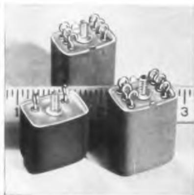
Typical transformer units using sub-miniature magnetic core laminations.
