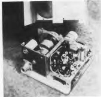
single unit. It occupies 67 cu. in. The new units transmit in the 215-235 MC range with frequency stability of  $\pm 0.01\%$  up to 71° C. Higher frequencies are possible with minor modifications. Basic unit also can be modified to operate at power outputs as low as 25 w. Integral "heat sink" provisions are suited to missile requirements. Texas Instruments Incorporated, 6000 Lemmon Ave., Dallas 9, Tex.
