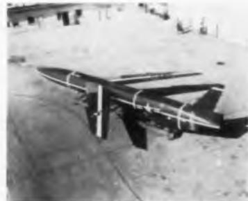
Robot-plane like, the Air Force's SNARK is sub-sonic, with a range of 6,000 miles.
