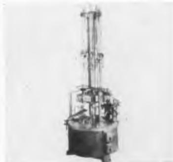
ened and ground to insure accuracy. Cutting knives are motor operated. Can be equipped with automatic tubing feed. Kahle Engineering Co., 1400 7th St., N. Bergen, N. J.
