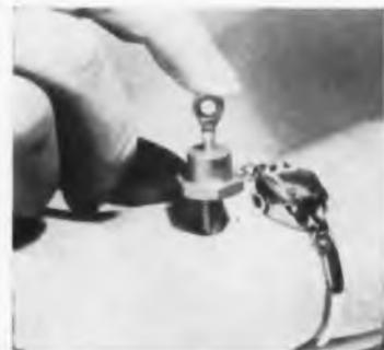
ings of 50, 100, 200, and 300 volts. Maximum leakage current rating on the rectifiers is 5 milliamperes. General Electric Semiconductor Products, Electronics Park, Syracuse, N. Y.
