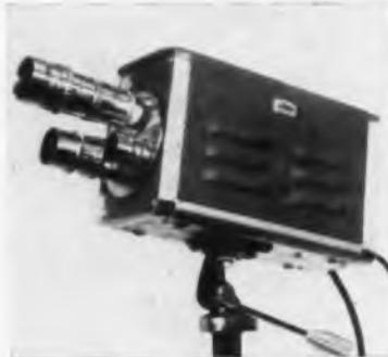
control unit. With optional 3 lens turret, the camera produces bright, clear pictures with light levels as low as ten or 15 foot candles, and usable pictures with even less light. The basic camera measures 5 x 7½ x 12 inches and weighs 12 lbs. Complete closed-circuit television systems, incorporating the TC-100, are available. DuMont Laboratories, Inc., 750 Bloomfield Ave., Clifton, N. J.
