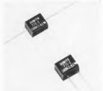
Riteohm precision resistor line. They employ no wire for the resistance element. Resistance range available is 100 ohms to 300 K ohms. Standard tolerance  $\pm 1\%$ , but tolerances can be supplied. Reactance is low due to the absence of wire coils. Consequently, these units can be used in high frequency and pulse circuits for which wire wound units are unsuitable. Ohmite Manufacturing Co., 3657 Howard St., Skokie, Ill.
