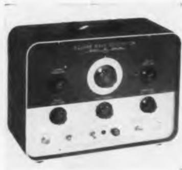
a convenient source of ideal square waves for checking the performance of audio and video and components, as well as cathode-ray oscilloscopes. Some of the features are: fast rise time, wide frequency range, control of square wave symmetry, two output impedances and accommodates synchronizing signals (step selection of 18 frequencies is provided). Measurements Corp., Boonton, N. J.
