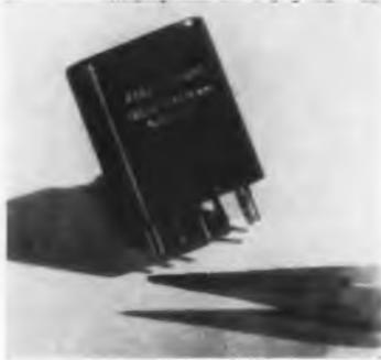
R600 (dpdt) and RS600 (spdt), these relays will withstand shocks of 50 G and vibration up to 2000 cps at 20 G. Contacts are rated at 2 a. resistive, 28 vdc or 115 vac. Continuous operation is possible throughout a temperature range from  $-65^{\circ}\text{C}$  to  $+125^{\circ}\text{C}$ . Conform to or exceed Mil. Specs MIL-R-5757C. Iron Fireman Electronics Div. 2838 S.E. 9th Ave., Portland 2, Ore.
