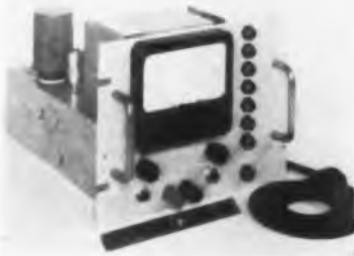
The automatic ohmmeter features automatic range switching, visual indication of resistance at the output terminals, simple readout, and fast response. Range switching is accomplished by a servo loop which selects the correct range to insure a meter indication at mid-scale for any resistance value. The selected multiplier is clearly indicated by a light. Kearfott Company, Inc., 1378 Main Ave., Clifton, N. J.
