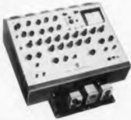
**WT-100A Electron-Tube MicroMhoMeter**—Accuracy suited for electronic equipment manufacturers and research, development, and maintenance groups. Precision tube testing under actual circuit conditions. Built-in "shorts" test; burnout-protected meter; regulated power supplies for AC voltages; measures transconductance up to 100,000 micro-mhos in 6 ranges. \$949.00\*
