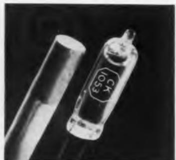
the full scale life of the tube may be varied by means of the anode current used. Shelf life is 2 years or more. Raytheon Manufacturing Co., 55 Chapel St., Newton 58, Mass.
