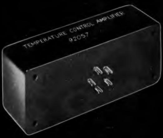
A sensitive differential magnetic amplifier for use in controlling the temperature of gyro housings and similar airborne devices. Responds to variations in resistance of a wire type sensor. Includes fail safe feature by reducing output when sensor resistances change abnormally high or low. Operates directly from 115 volt, 400 cps supply. Time response less than 0.5 sec. to a 1 ohm step.
