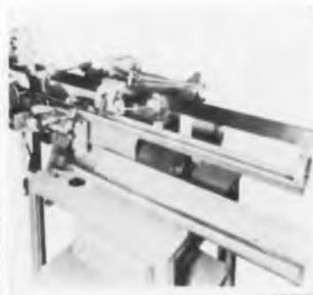
easily attached to the CS-6 machine without drilling a hole. It is recommended that a wire straightener be mounted ahead. Artos Eng. Co., 2757 S. 28th St., Milwaukee 6, Wis.
