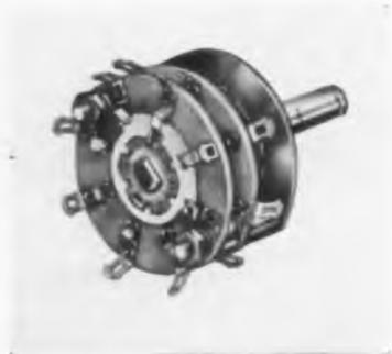
position wafers, with the latter providing up to 18 insulated contacts. Standard shaft diameter is ¼ in., but 5/32 in. and ¾ in. shafts are also available. Solid rivets fasten clips to the switch sections. Silicone fibre glass, meeting specification MIL-997 type GSC, is used for the switch stator. The rotor is punched from KEL-F. Oak Mfg. Co., 1260 Clybourn Ave., Chicago 10, Ill.
