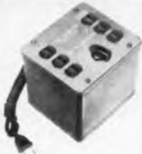
**WP-25A TV Isotap**—Speeds up servicing, prevents damage to test equipment, minimizes shock hazards. May be used as high-medium-low-voltage isolation transformer or autotransformer for testing TV receivers at various settings of line voltage. Supplies outputs of 130, 115, and 105 volts at maximum load. Tapped to match line voltages from 105 to 130 volts in six steps. \$22.00\*
