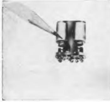
der shocks of 100G and vibrations of 30G to 2000 cps with no contact openings. Linear accelerations of 400 G do not open the contacts. Designated the SC, the relay measures 0.359 by 0.875 by 0.795 in. It weighs 17.5 grams. It operates on approximately 1 w. It is a dpdt relay capable of switching 2 a. at 30 vdc or 1 a. at 115 vac resistive. Potter & Brumfield, Inc., Princeton, Ind.
