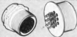
**GS (MS TYPE), KH, RKH, DAH, BFH, TBFH, DBH, KH30**... with steel shells and contacts to withstand high pressures from within or without. Insulation is a glass material, fused under high temperature to shell and contacts, thus forming a hermetic seal.
