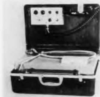
transmitter is from 25 to 30 w. The unit may be operated directly from a 6 or 12 v. battery. Current drain is kept low by employing quick heating tubes. The entire unit, including carrying case, weighs 52 lbs. less battery. A stripped chassis is provided on which users may add special equipment for time break circuits. Kaar Engineering Corp., P. O. Box 1320, Palo Alto, Calif.
