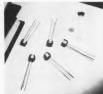
case. The case dimensions and lead configuration are suitable for insertion in printed boards by automatic equipment. General Electric Co., Syracuse, N. Y.
