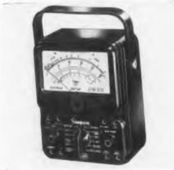
and a rugged printed circuit. DBM ranges run from -20 to +50 dbm, one millivolt in 600 ohms. The AC sensitivity has been increased to 5000 ohms/volt, and the frequency response now covers 5 to 500,000 cps. It also has a full-wave bridge rectifier system, and a rearranged interior for easier access to components. Simpson Electric Co., 5200 W. Kinzie St., Chicago 44, Ill.
