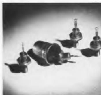
Maximum operating frequency for the new silicon rectifiers is specified as 100 kc. They will meet military mechanical specifications for rectifiers. General Electric Co., Syracuse, N. Y.
