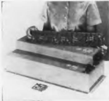
supplies a 16-bit, 24-hour binary code to hours, minutes and seconds. Signals generated by the equipment are suitable for recording timing marks or time codes on magnetic tape, oscillographs or to energize neon lights for indicating time code on the edge of motion picture film in optical instrumentation equipment. Electronic Eng. Co. of Calif., 1601 E. Chestnut Ave., Santa Ana, Calif.
