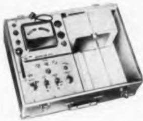
**WT-110A Automatic Electron-Tube Tester**—Automated punch-card tester, sets up all socket connections and all operating voltages at touch of lever. Scale indicates transconductance in terms of "Renew-? Good." Extremely versatile, simple to operate. Supplied with 263 cards. Accessory cards and punch available to keep card file up-to-date as new tube information is released. \$199.50\*
