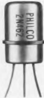
complementing circuits, bi-directional switches, bi-directional amplifiers, and phase detectors. It has good high voltage, current, and gain ratings. Maximum collector (or emitter) voltage is 40v; maximum collector current is 200 ma. DC current amplification factor ( $h_{FE}$ ) is typically 45, in either direction. Philco Corporation, Philadelphia, Pa.
