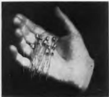
1/14 that of the JETEC-30 package. Four types, CK25, CK26, CK27 and CK28 duplicate the electrical characteristics of the Raytheon computer types. Four more types, CK13, CK14, CK16 and CK17 are for general purpose r-f use, four types, CK64, CK65, CK66 and CK67 are for general purpose audio use. Raytheon Mfg. Co., 55 Chapel St., Newton 58, Mass.
