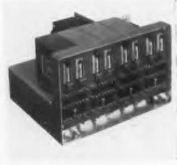
in the fidelity of pulse shape resulting from use indicates, among potentialities, an application in a demodulator for pulse code trains such as are used in air traffic control systems. Another application is the use of the delay line in computer operation where narrow pulses will permit an increase in the rapidity of calculation. Packard-Bell Electronics Corp., 12333 W. Olympic Blvd., Los Angeles 64, Calif.
