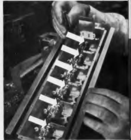
**ONLY ITS COUNTERPARTS CAN NOISE-TEST A 7077!** Evidence of Type 7077's low-noise, high-gain performance, is the use of five more of these General Electric triodes in a specially-developed multi-stage test amplifier that provides 90 db total gain. *Every 7077 built* receives this noise test!
