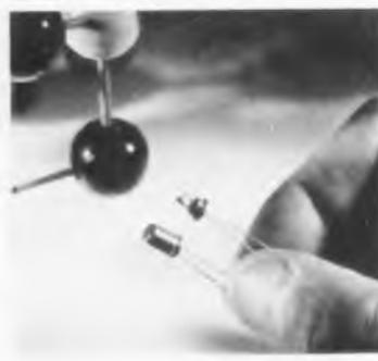
state (1 to 100 megohms) and a closed or low-impedance state (1 to 10 ohms). Characteristics of the diode suggest a versatile range of applications such as self-excited sawtooth oscillators, pulse generators, bi-stable memory circuits, and ring circuits. Shockley Semiconductor Lab., Beckman Instruments, Inc., Mountain View, Calif.
