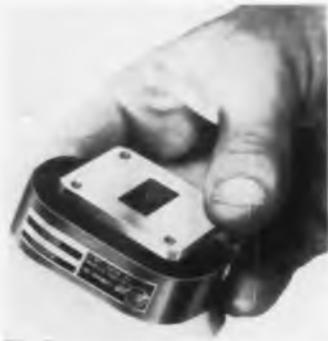
magnetic transverse field and ferrite sections built into the unit. Features area range of 8.5 to 9.6 KMC with isolation at 15 db min. and insertion loss of 1.0 db max. Other features include an input vswr of 1.10 to 1.5 max. Average power 200 w. and temperature-amb: 150°. Size is 1.000 deep x 2.100 high x 2.400 in. wide. Kearfott Co., 14844 Oxnard St., Van Nuys, Calif.
