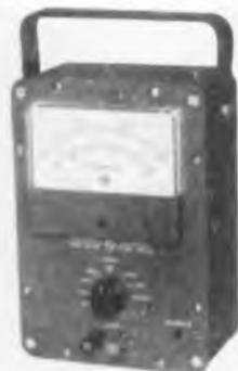
accuracy of 2 per cent regardless of wave shape down to 1 per cent duty cycle. To insure accurate, easy readability, seven full volt ranges of 100, 300, 1 kc, 3 kc, 10 kc, 30 kc and 100 kc are provided. Minimum input voltage is 0.1 v. rms and maximum 120 v. The instrument measures 8 $\frac{3}{4}$  x 5 $\frac{3}{4}$  x 4 in. Teletronics Laboratory, Inc., 54 Kinkel Street, Westbury, L. I., N. Y.
