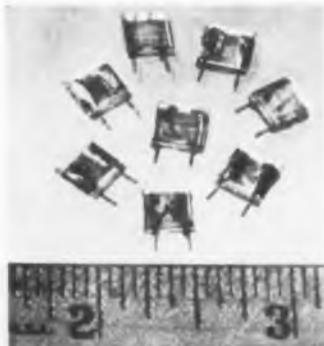
may be obtained in capacitances up to 1000  $\mu\text{f}$  at 300 v. rating. The WL-5 is larger and made in capacitances up to 2200  $\mu\text{f}$  at this rating. Corning Glass Works, Corning, N. Y.
