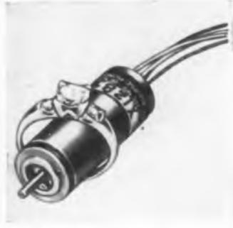
ings, a two-phase stator and a stainless steel housing. While the motor illustrated incorporates a tapered shaft, similar units can be supplied with shafts designed for specific applications. Some characteristics of the motor include: size, 5 frame; weight, 0.94 oz.; fixed phase and control phase voltage, 26 v.; frequency, 400 cps. Eclipse-Pioneer Div., Bendix Aviation Corp., Teterboro, N. J.
