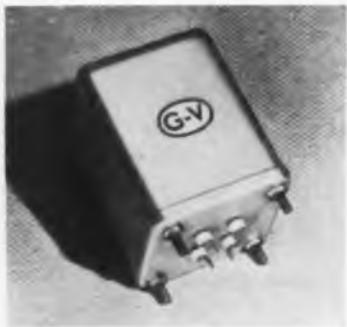
and magnetic elements mounted in a single case. Available for standard delay intervals of 2, 5, 15, 20, 30, 60, 120, 180, and 300 seconds. Other delay intervals on special order. Energizing voltage is 28 vdc. Output contacts are either normally open or normally closed, spst. Contacts are rated at 2 a. up to 230 vac. and 1 a. up to 32 v. dc. G-V Controls, Inc., Hollywood Plaza, East Orange, N. J.
