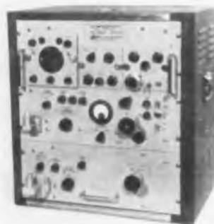
covers frequencies from 5200 to 5900 MC for C Band and 8500 to 10,000 MC for X Band. It contains a spectrum analyzer, power monitor, direct reading frequency meter and signal generator. The r-f section is constructed with umbilical cabling allowing for 8 in. clearance from main cabinet for maintenance or inspection. Kearfott Co., Inc., 253 N. Vinedo, Pasadena 8, Calif.
