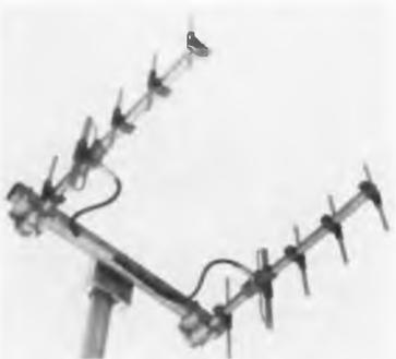
element is made of 3/4-in. tube. All elements are mounted by a heavy aluminum casting. The "T" match on the dipole is fed by a Teflon insulated balun inside the antenna boom. All internal wiring is potted under pressure. Antenna is shipped with N-type connector and 2 U-bolt clamps. Other type clamps and connectors are available. Scala Radio Co., 2814 19th St., San Francisco 10, Calif.
