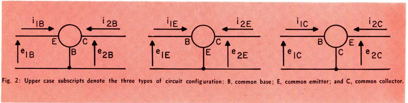
Fig. 2: Upper case subscripts denote the three types of circuit configuration: B, common base; E, common emitter; and C, common collector.
