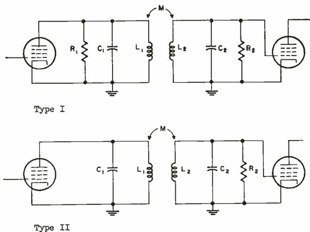
Fig. 1: Both of these interstages have equal resonant frequencies; Type I has equal damping, Type II unilateral.
