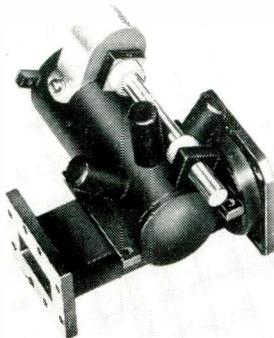
Compact, single-section, dual mode filter designed for lower power use in X-band systems, employs two orthogonal  $TE_{111}$  modes. Filter provides performance equaling that of a two-section filter. Insertion loss is less than 1.0 db and VSWR is less than 1.20. Airtron Inc.
