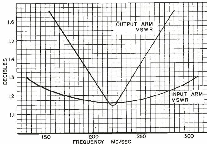
Fig. 8: VSWR of an input arm and the output of antenna arm
