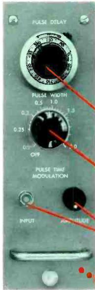
Five plug-in pulse generators provide any code—1 to 5 pulses — with completely independent adjustment of width and delay for each pulse.
