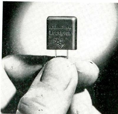
into printed circuit boards. Providing 600 mw dissipation, it is available in zener voltage ranges from 4.3 to 30 v. International Rectifier Corp., 1521 E. Grane Ave., El Segundo, Calif.
