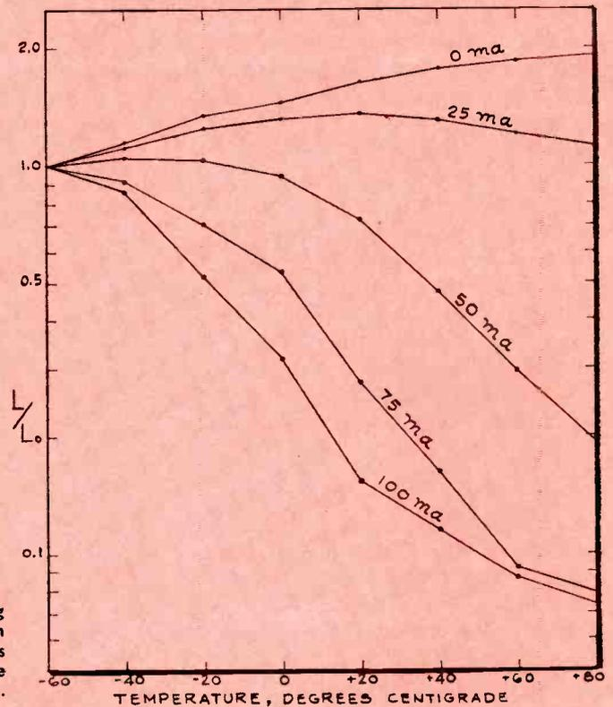
Fig. 4: For Ceramag 27 the effect on the inductance is much greater at the higher flux densities.
