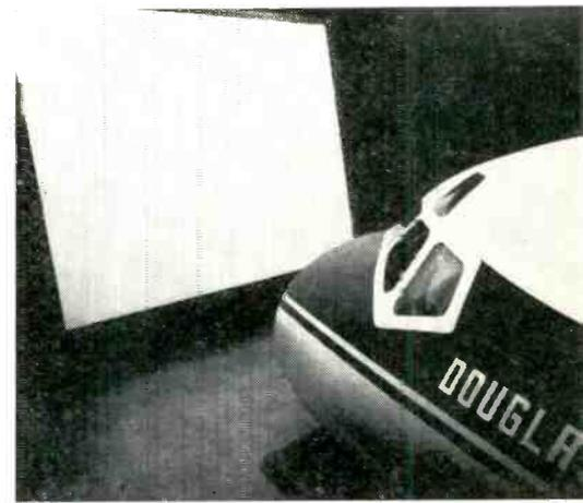
External view of the simulator cockpit and 12 x 15 ft. screen on which TV image is projected. Pilot can then see his position and altitude in relation to an airport.
