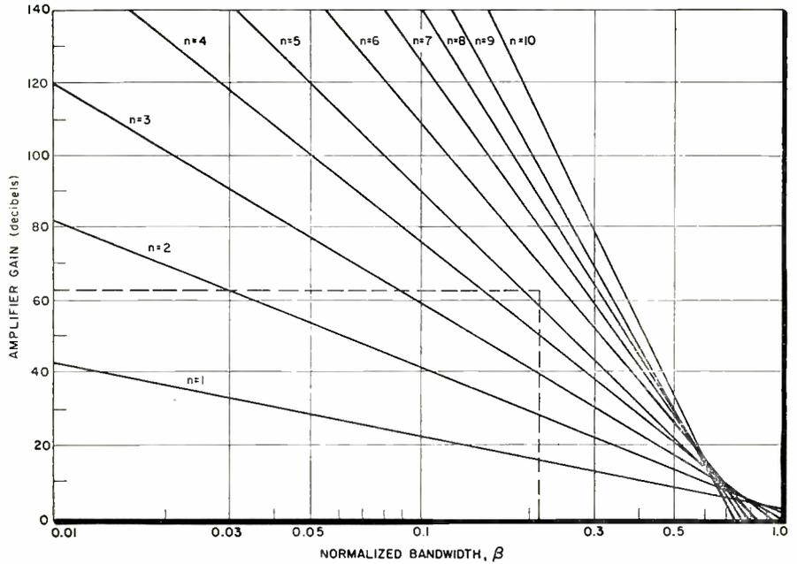
Fig. 2: Curves for  $n$  cascaded Type I, equal damping, maximally-flat interstages.
