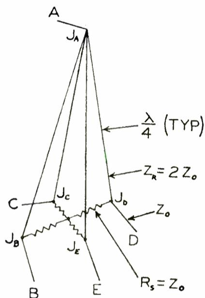
Fig. 6: Four-to-one coupler star connected
