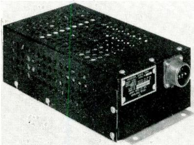
over the environmental range of  $-55^{\circ}\text{C}$  to  $+71^{\circ}\text{C}$ . Utilizing transistors in a bridge switching circuit for maximum reliability, 170-200 VA of single phase power and approximately 50 watts of three phase power are obtained from a unit weighing only 9½ lbs. Operates to  $71^{\circ}\text{C}$  without heat sinks or cooling air. Varo Manufacturing Co., Inc., 2201 Walnut St., Garland, Tex.
