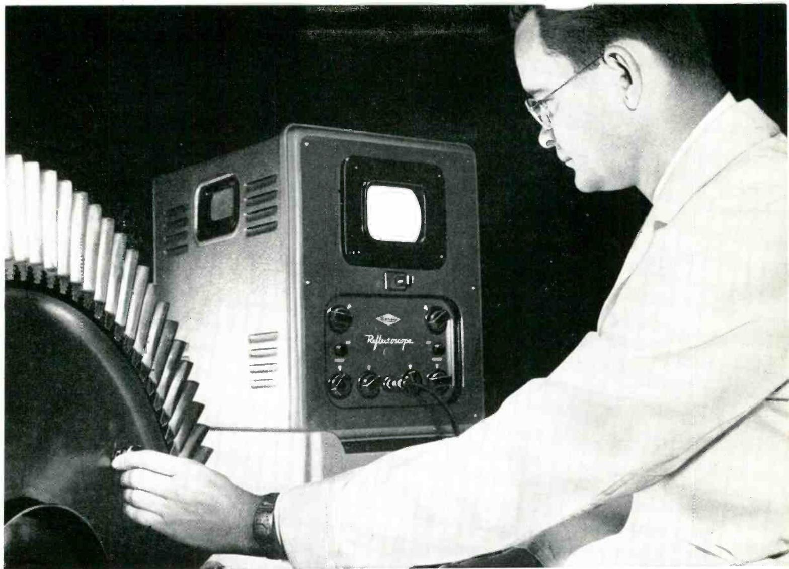
**TEST ENGINEER** touches Sperry Reflectoscope search unit to completed jet rotor forging in test for material flaws. A quartz crystal in the search unit converts high power pulse supplied by a Tung-Sol/Chatham 1258 hydrogen thyatron
