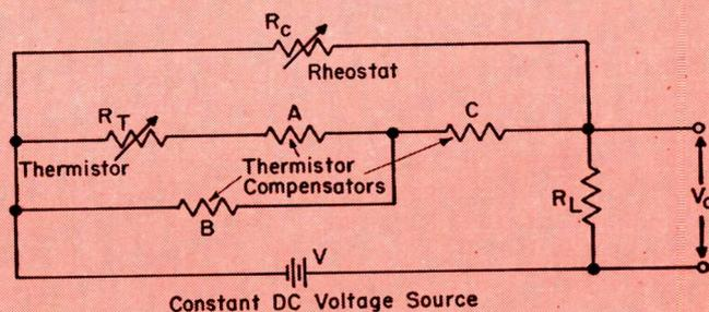
$$V / \left[ R_L + 1 / \left( \frac{1}{R_c} + \frac{1}{R_{TC}} \right) \right],$$
