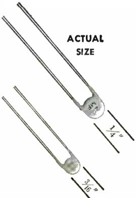
... with performance characteristics that equal or exceed much larger or more costly components. Excellent temperature stability: plus or minus 25% from 10° to 85° C. Extremely low power factor. Working voltage, 3 VDC. GMV tolerances. Maximum thickness, 0.156".
