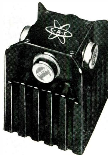
100 watts output at 40,000 ft. and operate at 71° C ambient temperature with no heat sink required. Converters are capable of output power up to 200 watts dc continuous. Operating range is from -55° to 71° C. Unit weighs only 2.7 lbs. Communication Accessories Co., Lee's Summit, Mo.
