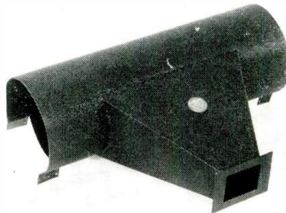
A ducted Netic traveling wave tube shield which directs the magnetic field developed by the enclosed solenoid structure, acts as a diversionary shield for fields originating in associated equipment, and provides more uniform cooling. Magnetic Shield Div. Perfection Mica Co.
