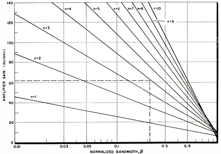
Fig. 3: Curves similar to Fig. 2 except for use with Type II amplifier interstages.
