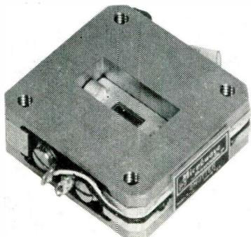
Rotary waveguide shutter for use in RG-52/U X-band, exhibits greater than 30 db attenuation over the band. In the closed position, shutter sharply attenuates radar leakage power from nearby radars thus preventing degradation or burnout of diodes in radar receiver. Microwave Associates, Inc.
