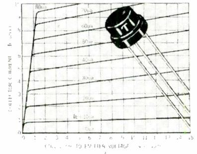
from -65° to 150° C. The 2N543, 2N542 and 2N541 operate at 45, 30 and 15 v. respectively and are good for multistage amplifier applications. Offering more gain per stage, these transistors reduce the number of amplification stages required. Transistron Electronic Corp., Wakefield, Mass.
