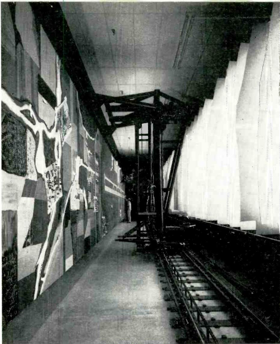
A miniature relief map, built to a 300:1 scale, is scanned by a TV camera on a travelling crane (center) in the "map room" of the Douglas DC-8 Simulator. Movement of the camera is governed by the electronic response of the simulated Jetliner to the pilot's controls, and an enlarged image is projected on a large screen in front of the simulator cockpit.
