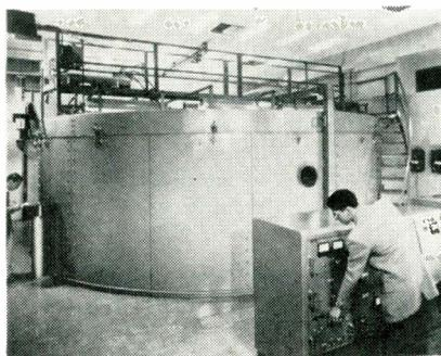
Delicate accelerometers for TITAN inertial guidance systems will be tested in new Genisco C-460 Ultra-Precision Centrifuge at American Bosch Arma Corp., Garden City, N. Y.
