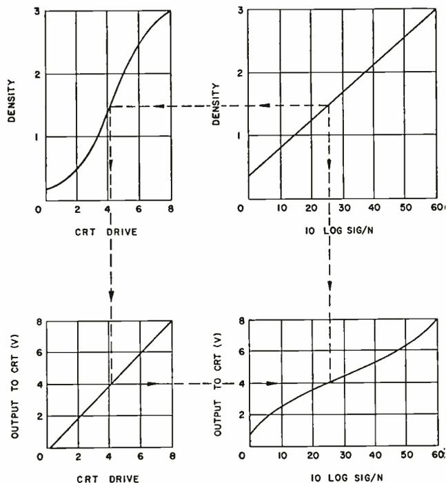
Fig. 10: Finding receiver compression for a linear density receiver.
