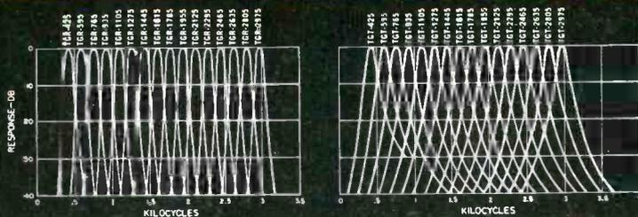
These band pass filters for multiplex transmitting and receiving provide maximum stability in miniature sizes. Both receiving and transmitting types are 600 ohms in and out, and employ 7 terminal header for sub-miniature 7 pin socket.
