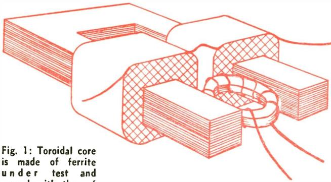
Fig. 1: Toroidal core is made of ferrite under test and wound with the r-f coil.
