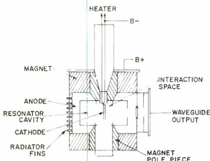
Fig. 3: The split-anode magnetron
