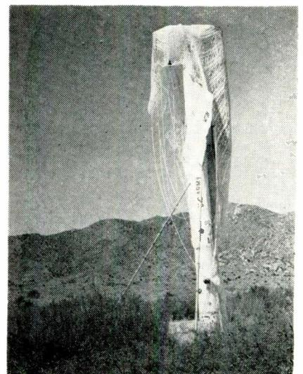
Intercepted and blasted out of the sky by Talos guided missile this Lockheed Kingfisher will be resurrected for still another target mission. Its recovery system consists of a parachute and a long nose spike.
