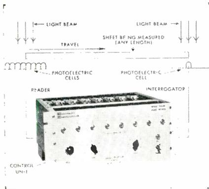
sired. Accuracy of the system is  $\pm 0.003$  in. which is completely independent of the speed of the conveyor line. Eldorado Electronics, Berkeley, Calif. Circle 271 on Inquiry Card. page 149
