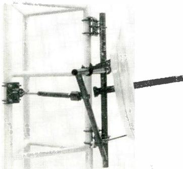
A 3-point suspension mounting frame for spun aluminum parabolic reflectors can be adjusted independently. The 3 load points absorb equal wind forces and offer maximum resistance to antenna twisting with minimum tower reaction stresses. Gabriel Electronics Div.
