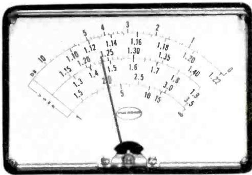
VSWR at any single frequency is indicated on the Ratio-Scope front panel meter.
