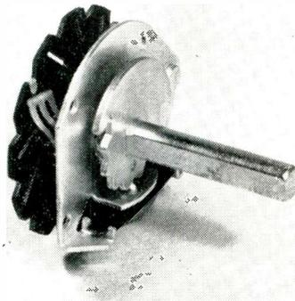
Indicated uses include switching of meter circuits, signal selection, tone selection, bias selection, circuit sampling and other applications in commercial and military equipment using printed circuitry. The switch is available in 2 to 12 position, excluding the 11-position arrangement. Current capacity is 10 a. P. R. Mallory & Co., Inc., Frankfort, Indiana.
