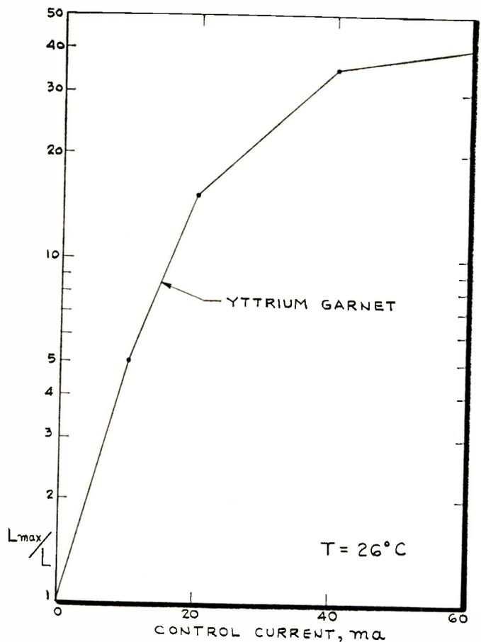
Fig. 6: Magnetic field effect on garnet's temperature coefficient of permeability.
