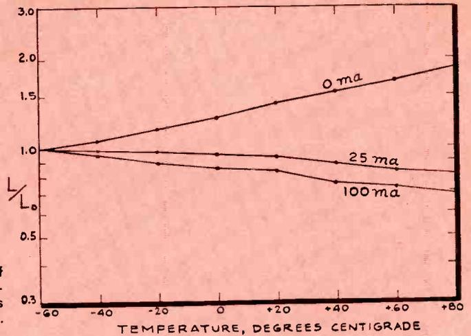
Fig. 3: Change of inductance for different flux densities when testing CR-20.
