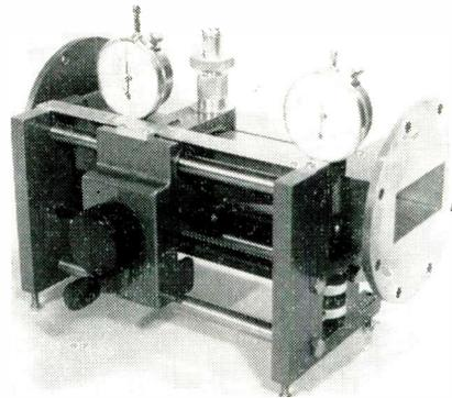
Designed primarily to cover 2600 to 40,000 MC using one carriage and appropriate slotted sections, the instrument features speed and ease of measurement at the testing bench. The carriage accommodates slotted sections ranging from Ka through S-Band. Sage Labs., Inc.
