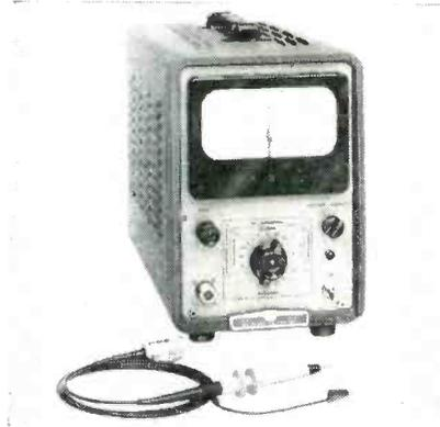
accuracy of  $\pm 3\%$  full scale. Use of a photoconductive chopper in place of the conventional mechanical vibrator helps achieve high sensitivity and reduces drift to less than 2  $\mu$ v. per hour after warm-up. Noise is less than 0.2  $\mu$ v. rms. It has a full-scale voltage sensitivity of  $\pm 10 \mu$ v. and a full-scale current sensitivity of  $\pm 10 \mu$ a. Hewlett-Packard Co., 275 Page Mill Rd., Palo Alto, Calif.
