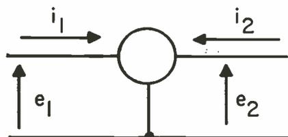
Fig. 1: Generalized circuit of transistor which is used in the theoretical considerations. All possible Jacobians are specified by six symbols.
