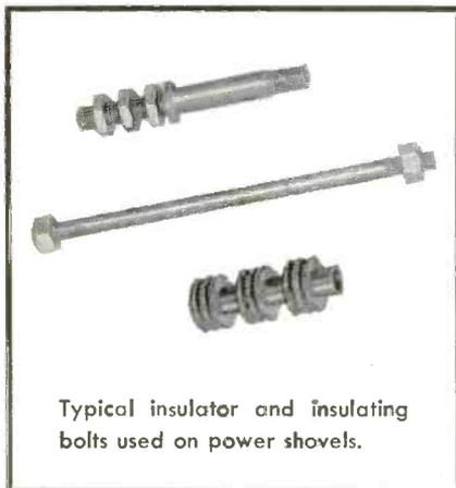
Typical insulator and insulating bolts used on power shovels.
