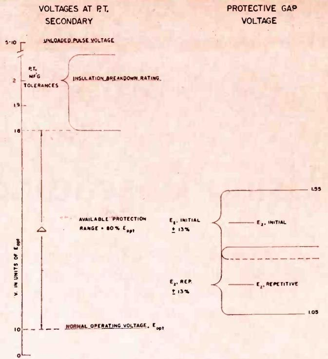
Fig. 1: The relative voltages at the pulse transformer secondary.
