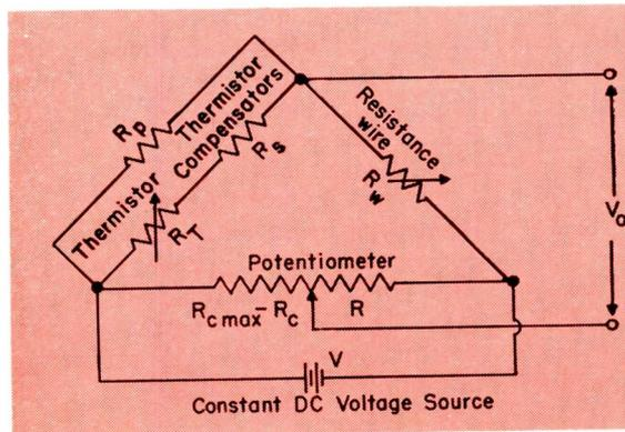
Fig. 1: (I) Temperature differential circuit
