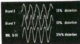
The highly efficient S-10 requires only 1/4 of the cone excursion of Brands X and Y to produce the same sound output. Result: greater inherent linearity and 75% less distortion.
