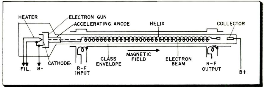
Fig. 4: Construction of the traveling wave tube
