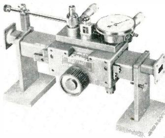
the Types 764 and 864 instruments operate over the frequencies 12.4 to 18.0 KMC/sec and 18.0 to 26.5 KMC/sec respectively. Separate tuning systems for probe and detector result in good sensitivity. Inclined dial presentations of probe position provide "Easy to Read" measurements to within 0.0005 in. Waveline Inc., Caldwell, N. J.
