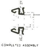
are snapped onto the panel. The male section of terminal connector is inserted into the rectangular panel hole, and as it passes through, spring legs of the clips compress and spring out again over the flanges projecting from either side of the connector. Flanges prevent the connector from passing completely through panel and clips prevent it from being pushed out when the other half of connector is applied. Tinnerman Products, Inc., Cleveland, Ohio.
