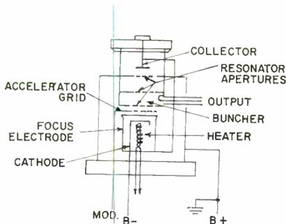
Fig. 2: Elements of the reflex Klystron
