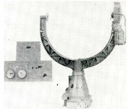
simultaneously tilt the antenna up to 180° and rotate 370° at variable speeds up to 30° per second. The rotator is remotely operated by means of a variac control and joy stick. Position indicators for both azimuth and tilt are in the control panel. It is built for service under severe weather conditions. Houston Fearless Corp., 11813 W. Olympic Blvd., Los Angeles, Calif.
