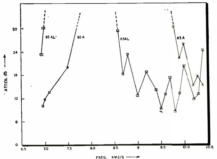
Fig. 5: Typical operation of beaded coaxial cables at discrete frequencies above 6,500 MC/S showing resonance effects.
