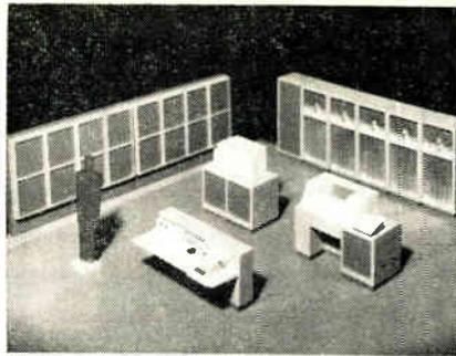
Honeywell 800 computer performs 30,000 three-address operations per second — handles 8 separate programs simultaneously
