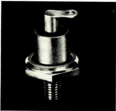
from -65°C to +200°C. It has a standard 14-28 threaded mounting stud and may be mounted in any position. The entire unit is hermetically sealed. Fansteel Metallurgical Corp., Dept. EIP, North Chicago, Illinois.
