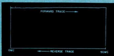
Fig. 3: With a generator sweeping from 0 to 50 MC, this is the pattern for an open circuit delay line  $\frac{1}{2}$  wavelength long.
