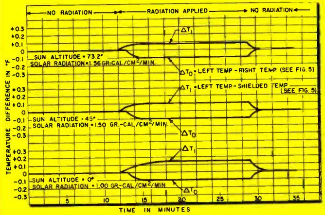
Fig. 6: Shielded thermometer performance characteristics are shown
