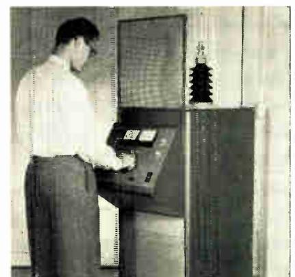
waist high panel sloped for easy reading. Two 4½ in. meters on the panel indicate output voltage and leakage current. Safety features are incorporated. The output test potential is continuously variable from zero to maximum and indicated by metering directly in the final output. Associated Research, Inc., 3777 W. Belmont Ave., Chicago 18, Ill.
