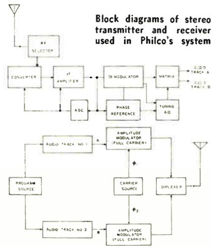
to the duplex radio transmission system Dr. Frank Conrad, Westinghouse radio pioneer, discovered in the twenties—has been shown by the Westinghouse Electric Corporation's television-radio division. The stereophonic signal is achieved by simultaneous amplitude and frequency modulation of the carrier.
