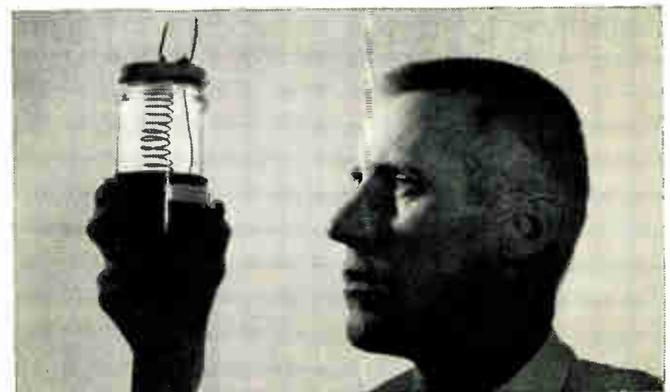
Seawater and sediment in bottle characterize ocean floor. Test sample of insulation on coiled wire is checked for bacterial attack by conductance and capacitance tests.
