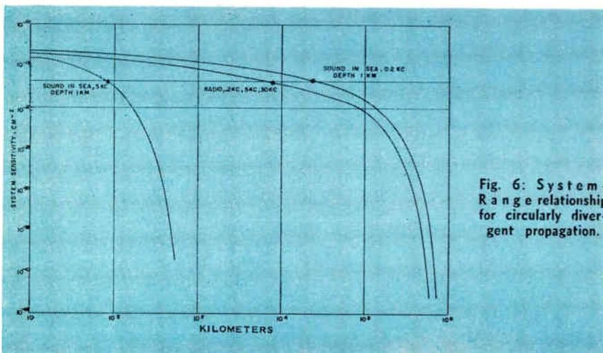
Fig. 6: System-Range relationship for circularly divergent propagation.
