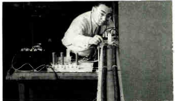
Highly precise instruments developed by Bell Laboratories engineers are used to detect infinitesimal changes in cable loss—to an accuracy of ten millionths of a decibel.
