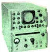
**Model SA-84 Multi-band Spectrum Analyzer** — 10 to 40,880 mc in a single unit. 25 kc resolution, 400 kc to 25 mc dispersion. Simple band switch, slide-rule dial. Military approved.
