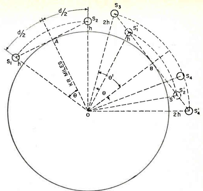
Fig. 6: Satellite communication geometry with the earth as a relay station.
