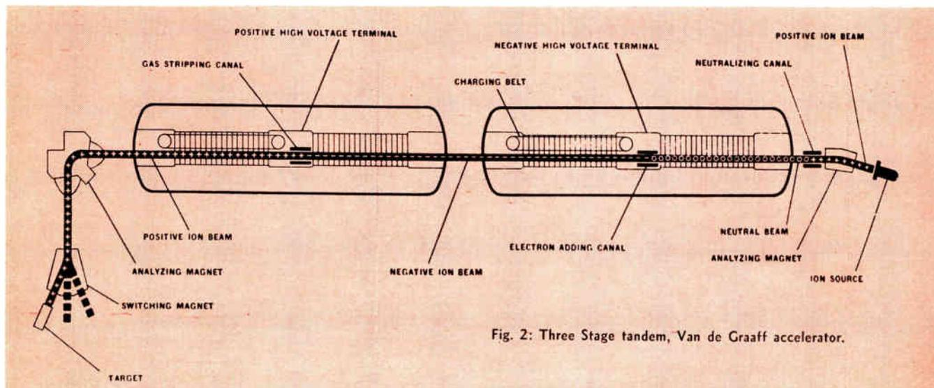
Fig. 2: Three Stage tandem, Van de Graaff accelerator.
