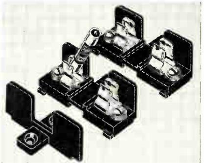
single pole blocks interlock and each unit is locked in place by a single screw. Additions may be made at either end. Poles may be added or removed without disconnecting terminal leads on other units. Each fuse permit raising one end of the fuse to a right angle position to the block. Bussmann Mfg. Div., McGraw-Edison Co., University at Jefferson, St. Louis 7, Mo.
