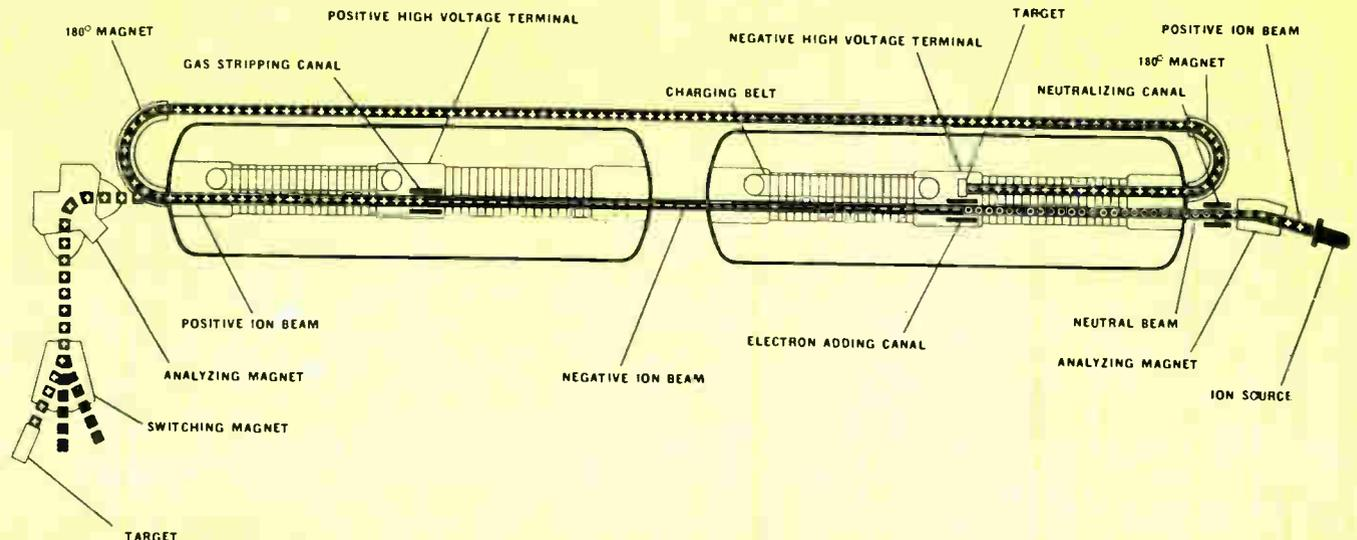
Fig. 3: Four stage tandem, Van de Graaff Accelerator.
