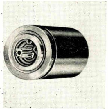
tapped winding for transistor use, and develops 0.33 oz. in stall torque in a standard size 8 BuOrd frame. The 2-phase winding is 26 v. on the fixed phase and the center-tapped control phase is 20/0/20 v. Power input is 2.7 w/phase at stall; operating temperature range -55°C to 150°C; speed at max. power output 3500 RPM; rotor moment of inertia 0.65 gm. cm<sup>2</sup>, and weight 1.6 oz. Meets Mil Specs. Induction Motors Corp., 570 Main St., Westbury, N. Y.
