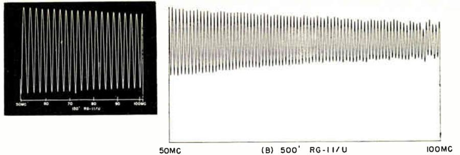
Fig. 7: (A) Ripple pattern from 150 ft. of RG11/U cable, shorted at the far end. Notice that the pattern is about the same as that for 66 ft. piece of RG59/U, in Fig. 6(B). The attenuation of RG11/U is about one-half that of RG59/U for a given length; so doubling the length just about cancels the attenuation improvement due to the larger cable. (B) shows the pattern from about 50 ft. of RG11/U showing the great reduction in ripple height at this length.
