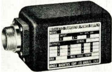
vdc; output voltage: 26 and 115 vac standard. Output frequency of 400 cps is standard, with 1200, 1500 and 2000 cps available. Output power: 40 va. Operating temperature range: -55°C to +71°C. Three standard terminations are available—A/N connector, wire-lead pigtail, and solder-lug terminals. Arnold Magnetics Corp., 4613 W. Jefferson Blvd., Los Angeles 16, Calif.
