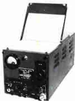
**HETERODYNE FREQUENCY METER** . . . accurate to .01% frequency measurement 100-10,000 mc (TFM-186).
