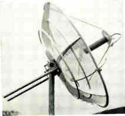
tion. Gain is 23 to 26 db over an isotropic source, nominal beam width is 8° to 14°. Frequency range is 940-980MC. VSWR of the complete antenna is less than 1.3. Azimuth adjustment is 360°; elevation adjustment 0-90°. Used for orbital and into-space telemetering or TV-Studio Transmitter Links (STLT) by feeding the dish with a 1990-2110 MC feed. Technical Appliance Corp., Box GC 38, Sherburne, N. Y.
