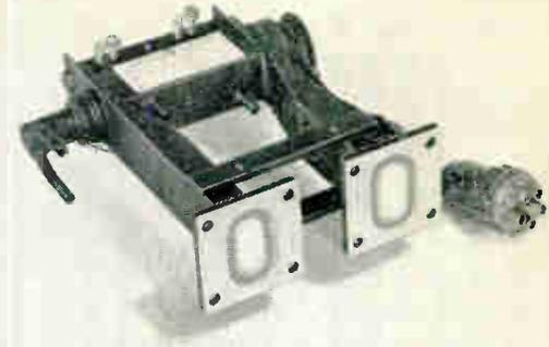
One of several unclassified designs in advanced development, this 100-watt CW tube features a multiple helix structure, involving four parallel beams for higher power output over a wider bandwidth. Frequency range is 7.5 to 11.3 kmc, with 25 db gain minimum.
