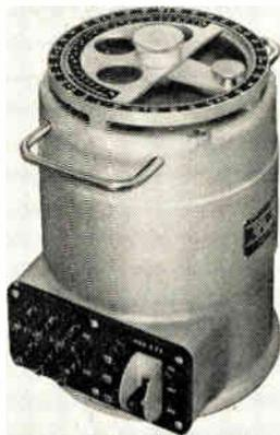
standards, wattmeters, power-factor indicators, induction relays, and instrument transformers. Direct-reading scales on the instrument, are calibrated in deg. for the electrical angle of displacement and in corresponding power-factor values. True-power-factor can be read directly. Ratings are: 1000 va continuous duty; input 120/240 v.; output, 120 or 240 v, 3 phase. Knopp Inc., 1307 66th St., Oakland 8, Calif.
