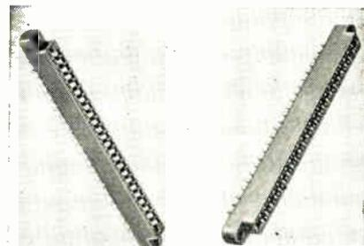
having 0.156 centers. They accommodate Class 1 (broad limits) tolerances on NEMA nominal 0.062 in. laminates. Maximum contact resistance is 4 mohm measured on a 0.054 in. card after insertion of a 0.074 in. card. The double side card receptacle maintains a minimum of 1 oz. per contact on a 0.054 in. thick card after 1000 insertions of a circuit board having a thickness of 0.074 in. Methode Mfg. Corp., 7447 W. Wilson Ave., Chicago 31, Ill.
