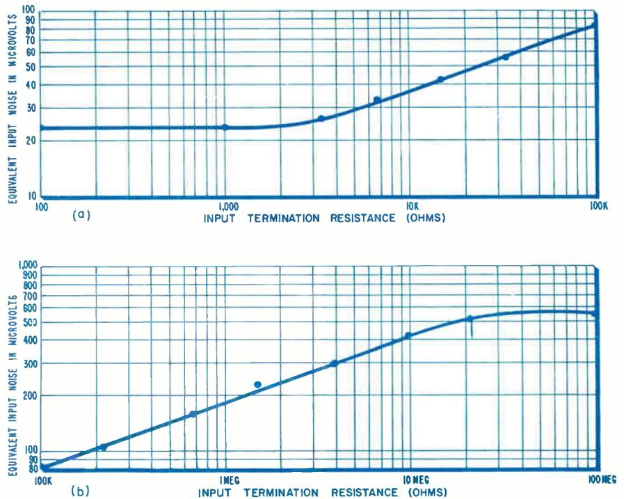
Fig. 5 (above): Noise level of the amplifier is a function of the input termination.
