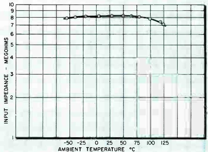
Fig. 3 (right): Relationship of input impedance, measured at 1 KC, to the ambient temperature.
