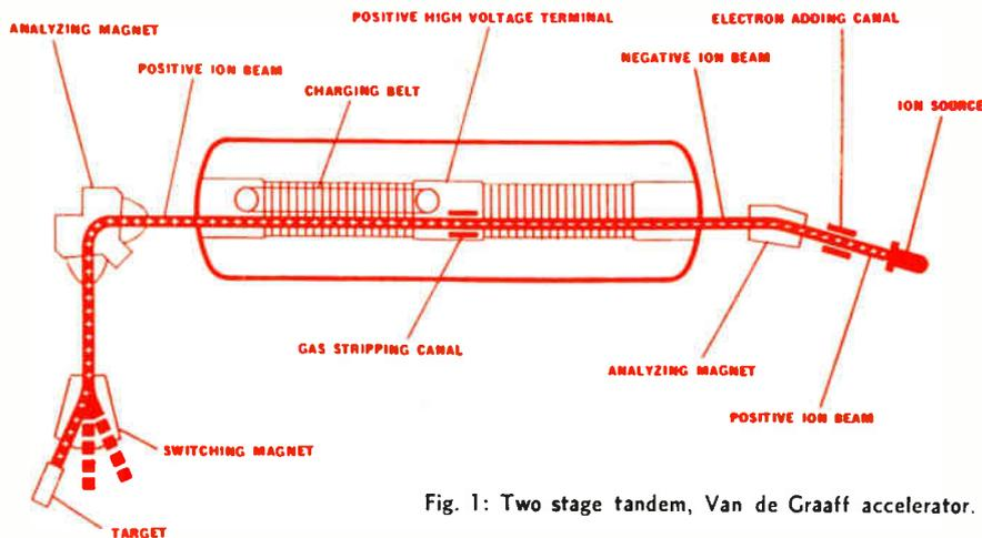
Fig. 1: Two stage tandem, Van de Graaff accelerator.
