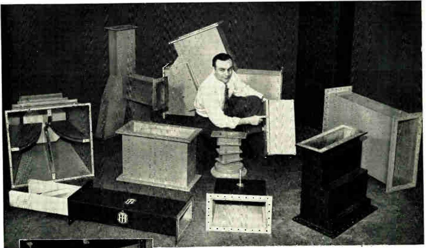
**A complete large waveguide service.** These units reflect I-T-E's design and production capabilities with large waveguide. Noncontacting short circuit section shown is available with servo-controlled motor drive. For proper electrical continuity, all waveguide flanges are held to 0.001 in. flatness (total indication) . . . are perpendicular within 0.030 (for two flanges, total indication). Available in sizes WR770 through WR2300.
