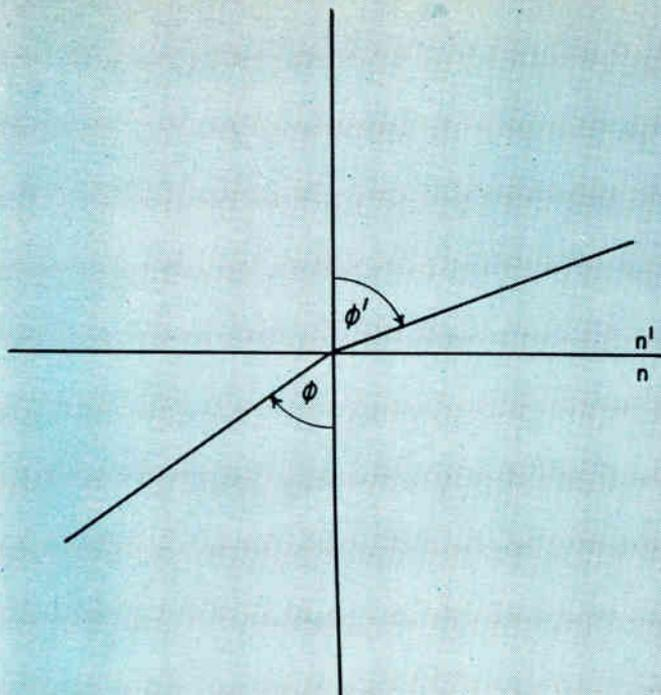
Fig. 4: Refraction from one medium to another.
