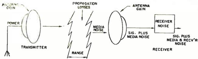
Fig. 4 (above): In the transmission medium, power is absorbed and spread so that only a fraction of it is delivered to the receiver.
