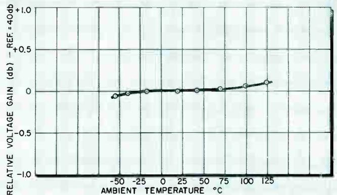
Fig. 4 (right): Voltage gain is almost independent of ambient temperature.
