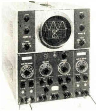
possible. Vertical resolution is 20  $\mu$ v on each of the 2 channels. Frequency response is from dc to beyond 100 kc. Featured is a full-scale amplitude measuring range of from one mv to 500 v. in 17 steps. Overall accuracy (amplitude) on the Y-axis of the identical channels is within 5% of full scale. Allen B. Du Mont Laboratories, Inc., 760 Bloomfield Ave., Clifton, N. J.
