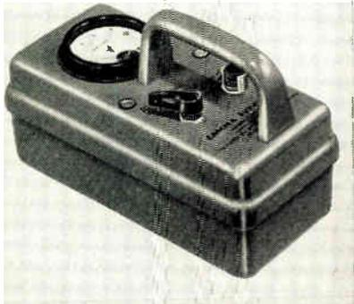
measurements by regulatory agencies. The unit has two controls: a range switch and a zeroing knob, and a 3-in. meter. The zero knob is protected against inadvertent movement. High impedance circuitry is hermetically sealed and range switching is performed in the low impedance portion of the circuit. The Victoreen Instrument Co., 5806 Hough Ave., Cleveland 3, Ohio.
