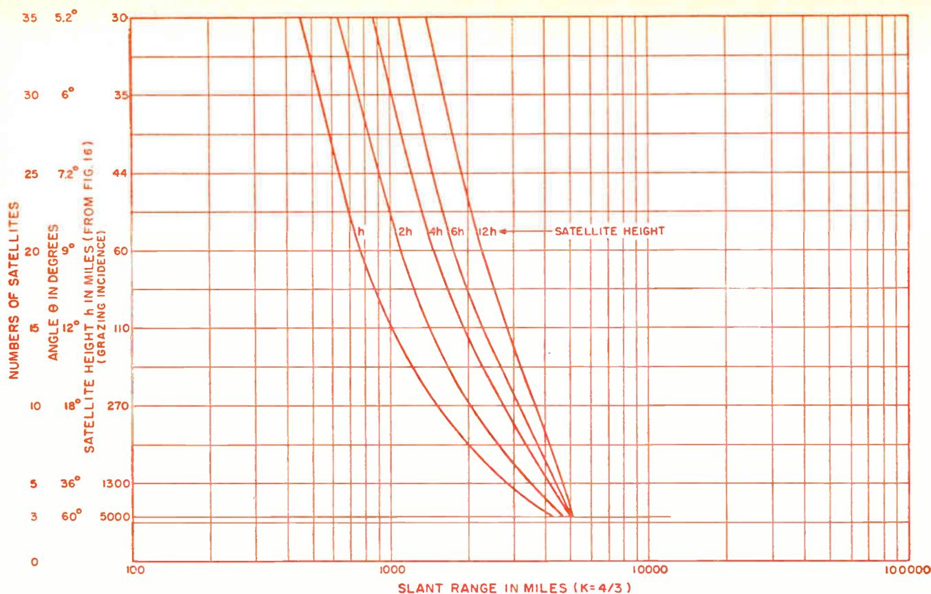
Fig. 9: The maximum slant range for various satellite heights.
