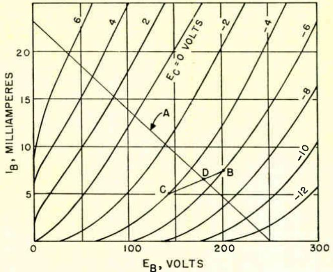
Fig. 2. Operating point is intersection D of load line A with line connecting two selected grid-cathode drops across  $R_k$  and the corresponding plate currents (points B and C).
