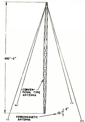
Fig. 7: A comparison of the ferromagnetic antenna with the conventional type.
