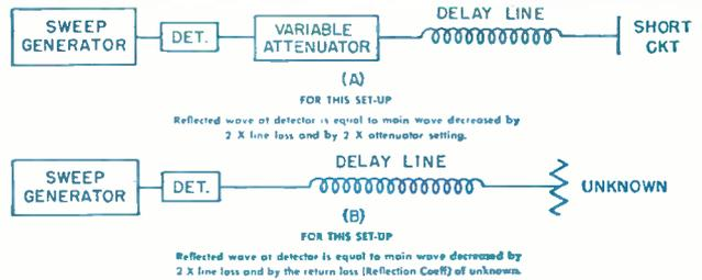
Fig. 14: If attenuator (A) is set for same ripple height as from unknown (B), return loss of the unknown equals twice the attenuator setting in db.
