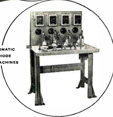
SEMI-AUTOMATIC GLASS DIODE SEALING MACHINES
