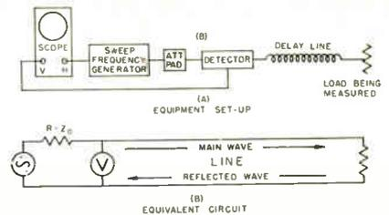
Fig. 1: This is the basic test set-up for making wide-band impedance measurements.
