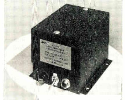
time duration of the pulse is proportional to the amplitude of the input signal. Gain is established at values between 80 and 1600, with external resistors. It may be modified for 400 CPS where max. power input is 16 w. Input impedance is 5 K-100 K ohms; signal frequency, 60 CPS; max. signal input, 30 v. RMS; voltage output, 40 v., 60 CPS. Kearfott Co., Inc., 1500 Main Ave., Clifton, N. J.
