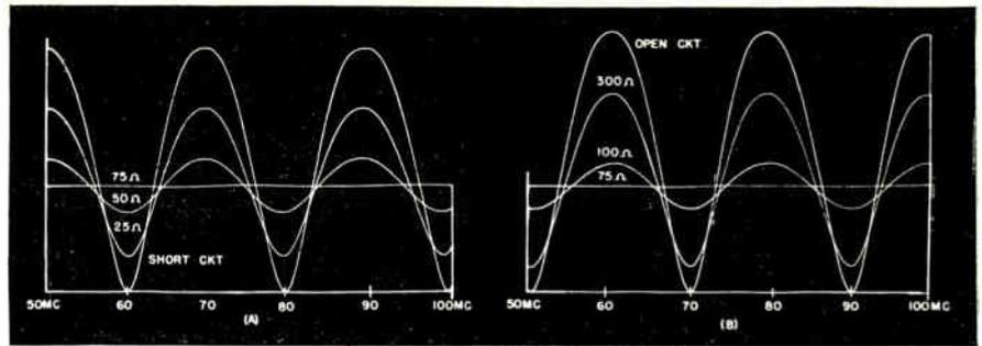
Fig. 8 (above): Patterns from several resistive terminations: when they are (A) lower than the characteristic impedance; (B) higher than characteristic impedance.
