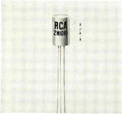
microphone preamplifiers, and hearing aids in which low noise factor is important. Designed to operate from extremely small input signals, it has a noise factor of 5 db with a generator resistance of 1000 ohms and an integrated noise bandwidth of 15 kc. Typical small-signal current gain is 35. Alpha-cutoff frequency is 2 mc. Semi-conductor and Materials Div., Radio Corp. of America, Somerville, N. J.
