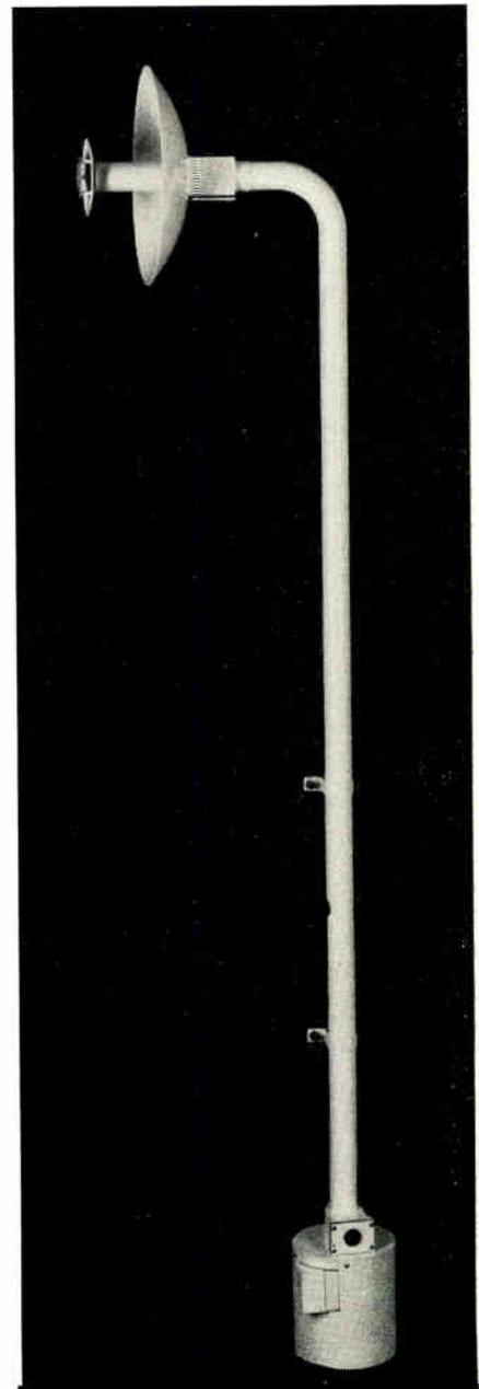
Fig. 2: Radiation shielded and aspirated thermometer unit.
