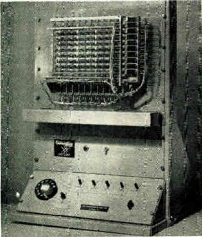
circuit with each of 100 sets of 6-wire terminals, at speeds up to 50 sets per second. It is designed for fast, quiet operation without adjustment over millions of operations, with low crosstalk between adjacent circuits at frequencies up to 10 megacycles. James Cunningham, Son & Co., Inc., P. O. Box 516, Rochester 2, N. Y.
