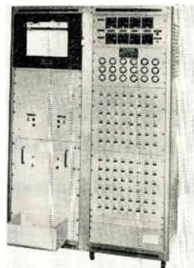
heavy-duty rotary type multideck switches. They can be modified for millivolt inputs such as thermocouples. Gilmore Industries, Inc., 13015 Woodland Ave., Cleveland.
