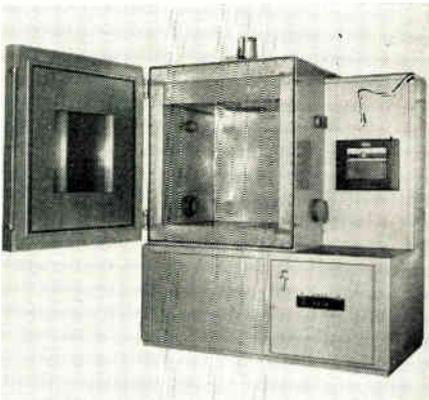
at -70°F. Temperature to -100°F can be attained in less than 1 hr. Chamber interior is stainless steel. Control within 2°F of set point is standard. Conrad, Inc., 141 Jefferson St., Holland, Mich.
