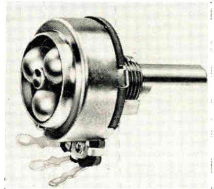
rotation approximately  $4000^{\circ}$ . Type VA-45 is  $15/16$  in. dia.,  $1/4$  to  $1/2$  w. Resistance range is 250 ohms through 10 megohms (linear taper). Voltage rating across end terminals is 500 vdc and voltage rating bushing to terminals 1000 volts ac for 1 min. hi-pot test with 750 vdc operating maximum. Chicago Telephone Supply Corp ration, Elkhart, Ind.
