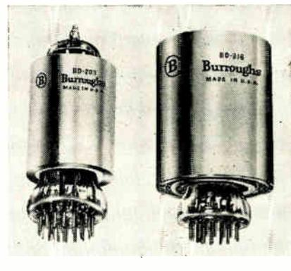
switching tubes. Dimensions are reduced by 35%. They may be used in direct contact with each other. They are 10 position tubes for distribution, counting, coding and decoding, sampling and conversion. Each tube may replace 20 or more transistors or other components. They can be arranged to switch in sequence or at random, can be preset to any position, and interconnected as distributors to any number of positions. Burroughs Corp., Electronic Tube Div., P. O. Box 1226, Plainfield, N. J.
