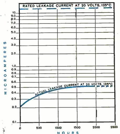
**LEAKAGE CURRENT vs. TIME AT 125°C**
