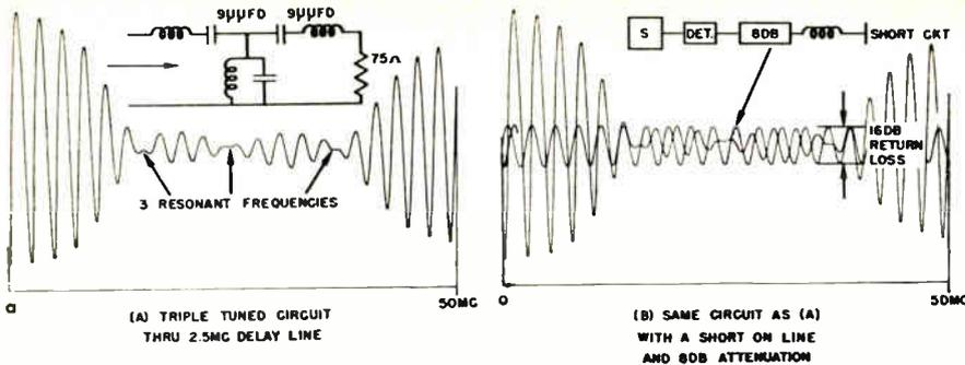
Fig 16: To determine the return loss: pattern for triple tuned bandpass filter connected to end of line (A) is superimposed on pattern of a shorted line with 8 db attenuation (B).
