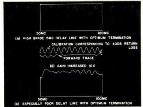
Fig. 17: These traces show the extremes that may be encountered in cable reflections.
