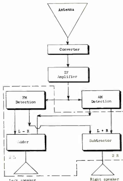
Block diagram of Westinghouse's AM compatible stereophonic receiver
