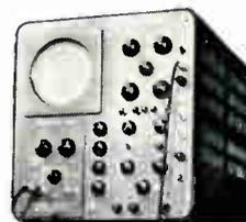
Trial and error methods necessary to capture elusive transients on conventional scopes waste time, film, and precious research dollars. Never again need this happen. With the Hughes MEMO-SCOPE® oscilloscope you may instantly "freeze" wave forms with brilliant clarity for careful study, comparison and analysis.
