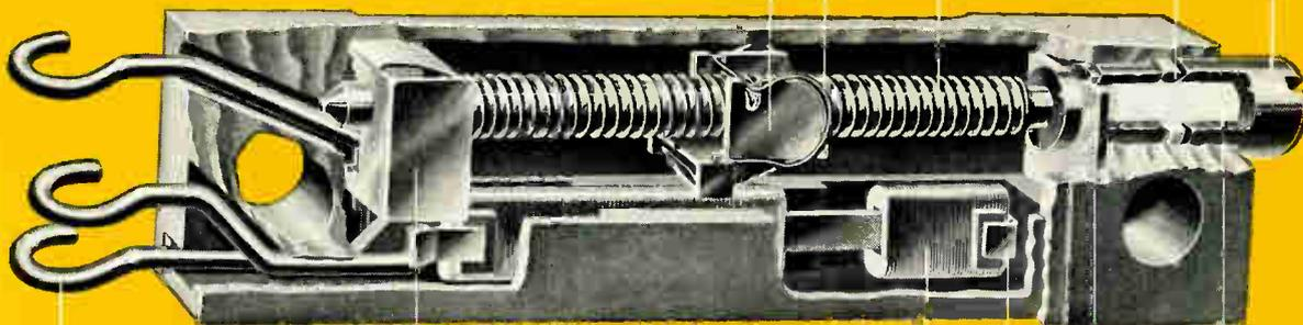
**SOLDER TERMINALS** — Tinned terminals are compact, yet large enough for easy soldering. Teflon-insulated leads and printed circuit pins are also available.
