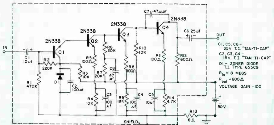
Fig. 2 (above): The complete amplifier circuit. Input impedance approximates product of amplifier current gain and feedback resistor,  $R_{13}$ .
