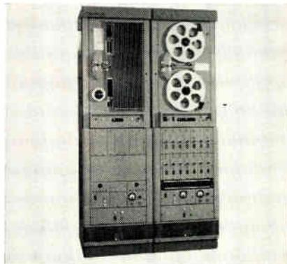
or simultaneous erase for 14 analog, FM, or PDM record/reproduce channels. It is compatible with the Type 5-752 reel recorder. Featured are: full-speed operation at 60 ips in less than 1 sec., full stop in less than 0.5 sec., simplified tape threading, automatic tape tensioning, and closed-loop tape drive, for precise control of tape movement over the magnetic read/write heads under the drive capstan. Consolidated Electroynamics Corp., 300 N. Sierra Madre Villa, Pasadena, Calif.
