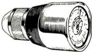
For quick, visible, precise measurements of extremely low starting and moving torques. Compact hand tool features Jacobs-style chuck for ease of use. Accuracy: ±5% of full scale standard. 48 models available, starting with low of .005 to .6, and a high of 2 to 40 oz. in. Most models available with CLOCKWISE, COUNTER-CLOCKWISE, or BI-DIRECTIONAL dials. Write for Folder 3001.
