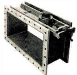
Type 223-LW Waveguide Rotary Standing Wave Indicator for standing wave and reflectivity measurements in WR-2100 waveguide systems over the frequency range from 350 to 530 mc/s. Residual VSWR less than 1.03.
