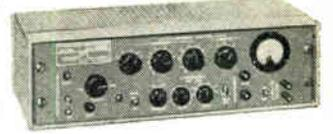
The G-6, Panoram's Broad Band Response Indicator, extends the range of Panoram's Curve Tracing Systems to 15 mcl In combination with the SPA-3, it shows response to fundamental frequency only, gives a single line presentation, discriminates against noise and hum and has virtually unlimited dynamic range. 0-15 mc range in 0-3 mc segments. 1 v. into 72 ohms output with up to 60 db attenuation.
