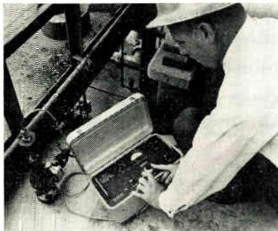
Differences of as little as 1-millionth of an inch in the internal corrosion in a pipe or tank are detected by this new measuring instrument by Crest Instr. Co. div. of Magna Products Co.
