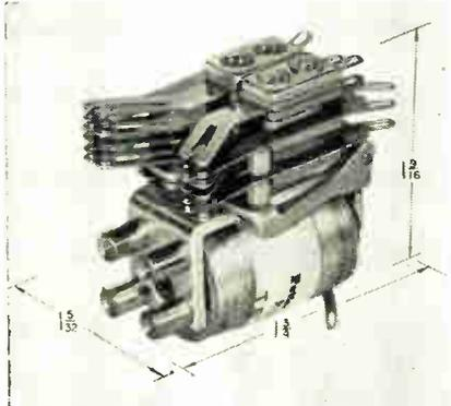
as 100 mw per movable arm and can be furnished to operate on voltages up to 110 vdc. It will switch up to 4 a. at 155 v. 60 cps, resistive loads. It is mounted with tapped #4-40 studs on 3/8 x 3/8 in. centers, and measures 1 5/32 in. long x 1 9/16 in. wide x 1 1/8 in. high. Weighs app. 3 oz. Relays are furnished with pierced solder lugs or taper tabs. Potter & Brumfield, Inc., Princeton, Ind.
