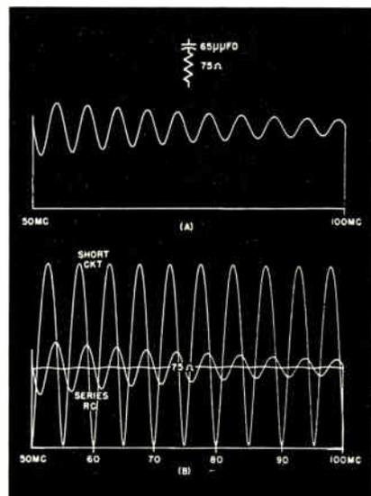
Fig. 11: A series resonant circuit termination pattern (A) is compared with matched and short circuit terminations (B).
