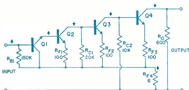
Fig. 1: Simplified circuit of the high input impedance amplifier has common-emitter collector stage followed by 3 common-emitter stages.
