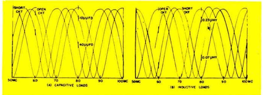
The impedance of a load giving a minimum at the same frequency as a short circuit is resistive and lower in resistance than  $Z_0$ .
