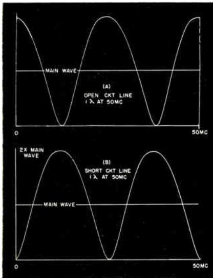
Fig. 5: Effect of doubling the line length is evident. Open circuit delay line pattern is shown in (A); short circuit in (B).
