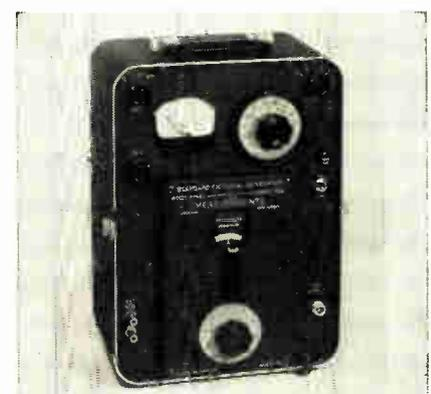
frequency ± 8 kc. Peak deviation to ± 16 kc is read directly on a meter. Output can be varied from 0.1 to 100,000 μv across a 50 ohm termination. Measurements Div., McGraw-Edison Co., Boonton, N. J.
