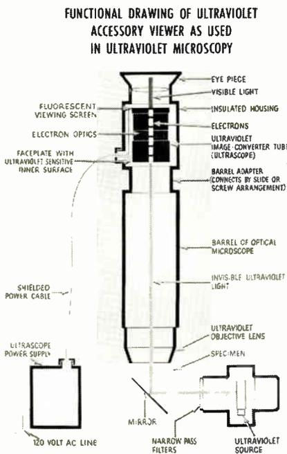
This simple drawing illustrates how specimens under ultraviolet light may be studied directly. The ultrascope unit, including power supply, is priced at \$1500; it replaces a TV system costing \$15,000.
