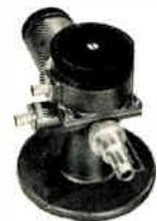
Type 219 Rotary Standing Wave Indicator for use in coaxial systems for standing wave and reflectivity measurements over the frequency range from 100 to 1,000 mc/s. Residual VSWR less than 1.03.
