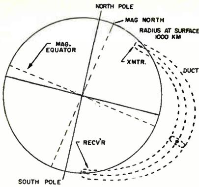
Fig. 3: Radio waves at 10 KC are conducted in this rare duct of about 2000 km dia.
