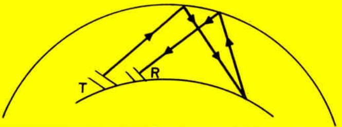
In the other case, transmitted power can be scattered back along the path transmitter—ionosphere—ground—ionosphere—receiver, as shown in Fig. 2.
