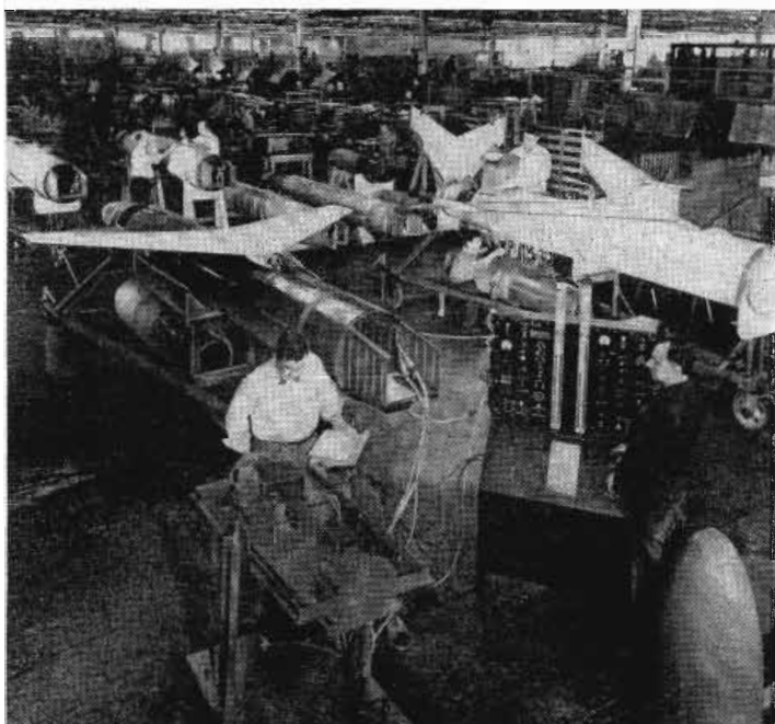
The Navy's new Martin KDM-1 pilotless target drones come off the sleepless Baltimore production lines. Powered by ram-jet engines, the target-drones are remote-controlled by radio and tracked by radar, to simulate the flight of an attacking airplane
