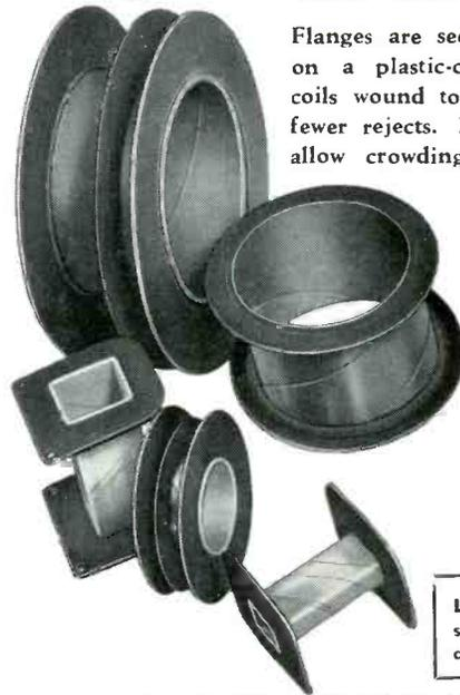
Flanges are securely locked in place on a plastic-coated core to assure coils wound to closer tolerances and fewer rejects. Flange cannot slide to allow crowding of turns, and wire cannot slip off coil form. Insulation is improved. Bobbins made any shape — round, square, rectangular — any size, of finest dielectric kraft, fish paper, cellulose acetate, or combinations. Low die costs cut unit prices surprisingly.
