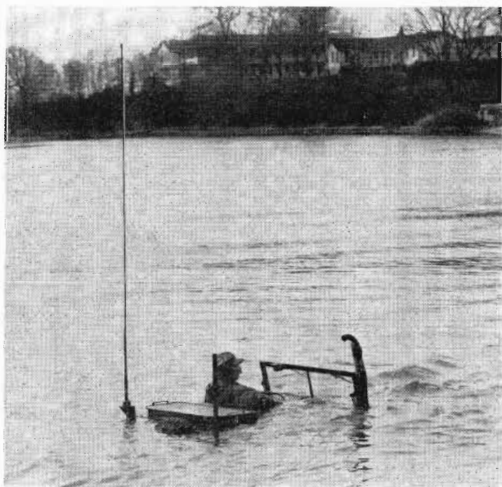
Both radio and jeep operate submerged as well as ever, even with water up to the driver's shoulders. This official U. S. Marine Corps photo shows one of the new units being developed for the Marine Corps Equipment Board
