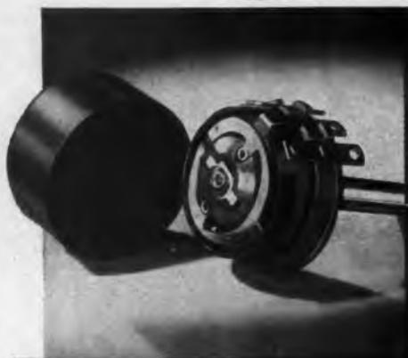
This precision potentiometer has a tapered winding held to plus/minus  $1\frac{1}{2}\%$  linearity as measured at 10 test points. Mechanical tolerances held to plus/minus 0.00025". Unit operates dependably over extreme ranges of temperature, humidity, altitude or barometric pressure, and severe vibration. Obviously built to a *quality* standard rather than to a price.
