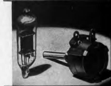
Shown alongside a miniature tube is this Clarostat Series 48 sub-miniature potentiometer. Only  $\frac{1}{4}$ " dia. — no bigger than a dime! Carbon element up to 3 megs. linear; slightly higher in taper. 0.4 watt rating. Single, dual, triple units. Essential in ultra-compact electronic assemblies. Here's *precision* in diminution.
