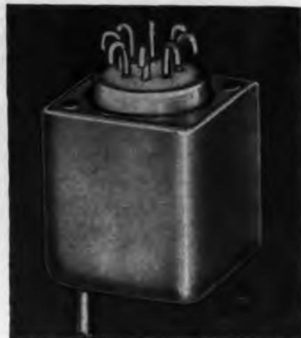
.600 O.D. and a new design balanced armature relay sealed in a ½ in. square drawn aluminum can. The entire unit is so constructed that it may be panel mounted from top or bottom. It is supplied with a dry air fill or vacuum pumped and pressure filled with dry nitrogen.—**Hermaseal Co., Inc., Elkhart, Indiana**—TELE-TECH.
