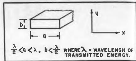
Fig. 3: Waveguide dimensions
