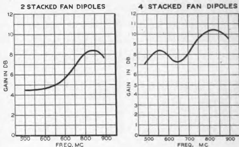
Figs. 7-10: (Left) Physical appearance of two-stacked (left) and four stacked fan dipoles. (Above) Gain vs frequency for the two types
