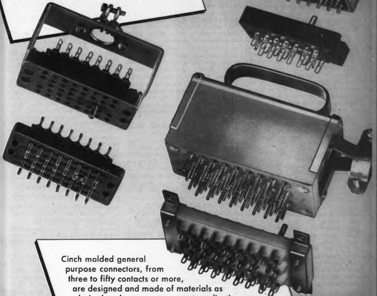
Cinch molded general purpose connectors, from three to fifty contacts or more, are designed and made of materials as desired and necessary to meet application requirements. They are available in low loss mica or melamine for chassis mounting or assembled with cap for cable applications. Terminals gold or silver plated. Consult Cinch!
