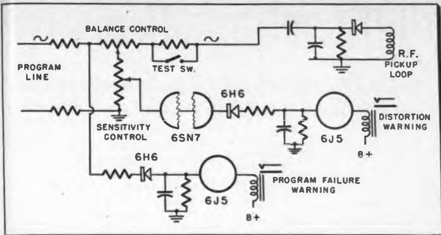
Transmitter quality monitor provides distortion indication through audio harmonics
