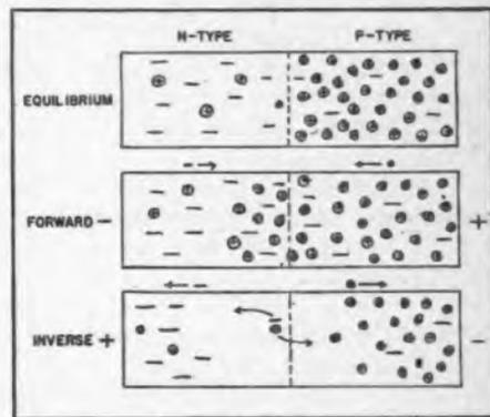
Fig. 4: Rectification by a P-N Junction
