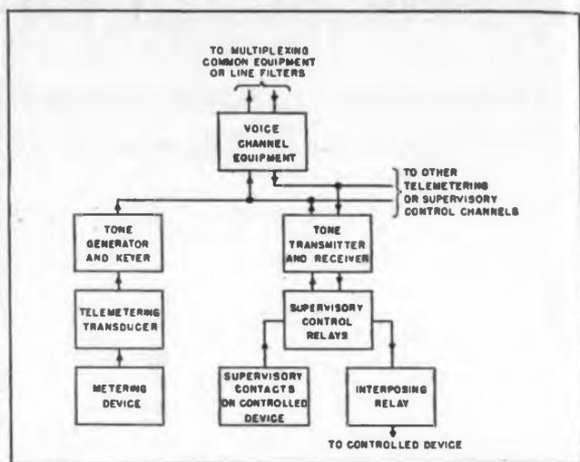
Fig. 5: Telemetering and supervisory control tone channels
