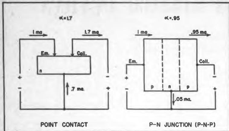
Fig. 7: Comparison of transistors
