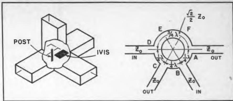
Fig. 7: (left) Interior view of hybrid junction. Fig. 8: (right) Sectional schematic of hybrid ring. Fig. 9: (below-left) Balanced mixer. Fig. 10: (below-right) Duplexer
