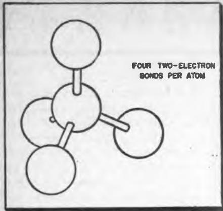
Fig. 1: In a perfect insulator electrons are tied up in interatomic bonds and cannot participate in conduction
