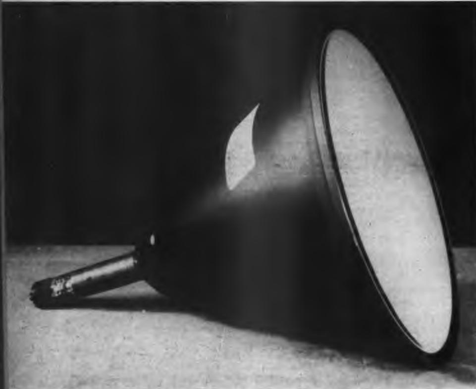
Photo of 16 in. flat-faced CR tube with an aluminized magnesium fluoride screen
