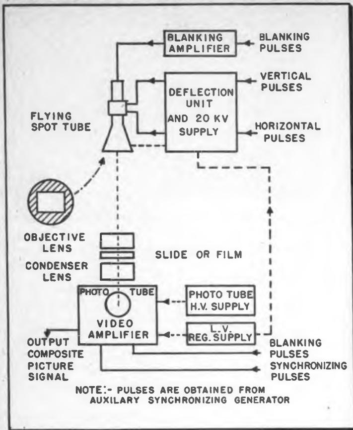
Fig. 1: Block diagram of flying spot scanner
