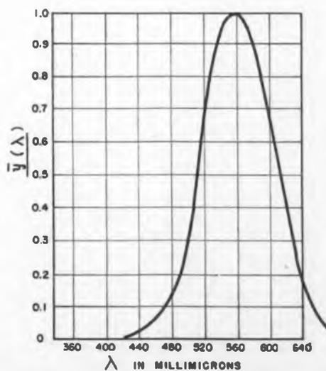
Fig. 6: Spectral response of an S4 surface
