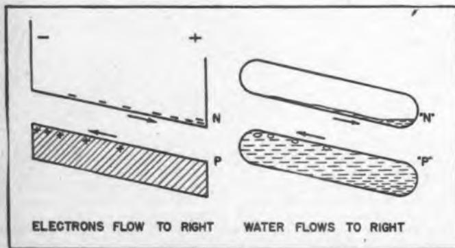
Fig. 2: Two conduction processes
