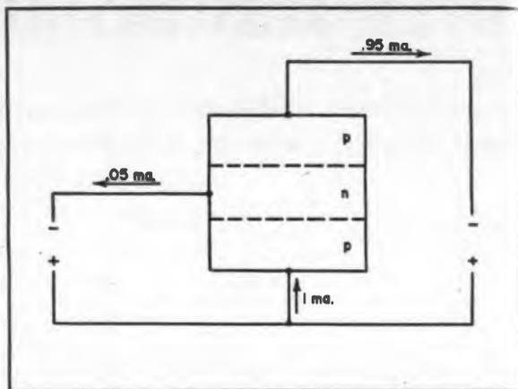
Fig. 8: Circuit current gain  $\alpha/(1-\alpha)$
