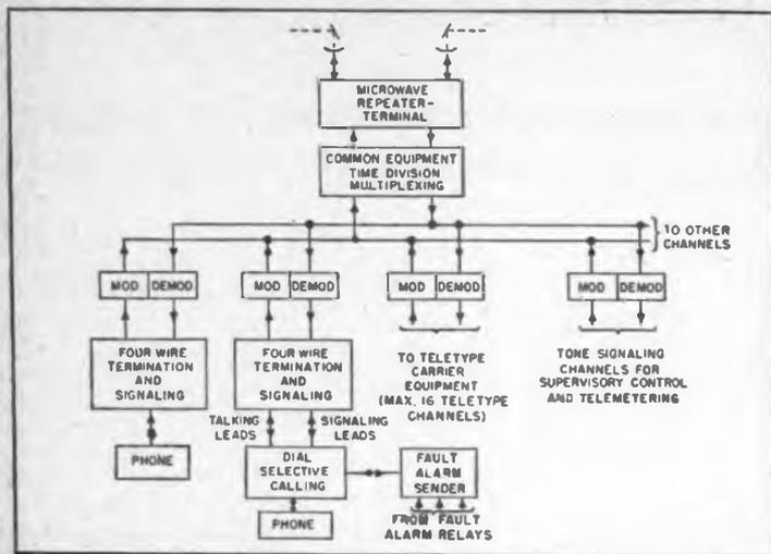
Fig. 4: Time division multiplexing at a microwave station
