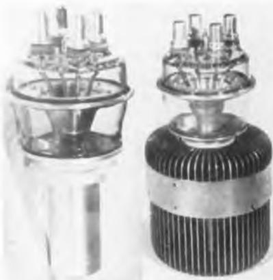
erate up to 220 MC. Tubes are compactly constructed with thoriated tungsten filament, disc type screen grid seal to minimize inductance, and two control grid pin connections with low capacitance and inductance. — Amperex Electronic Corp., 25 Washington St., Brooklyn 1, N. Y. — TELE-TECH.
