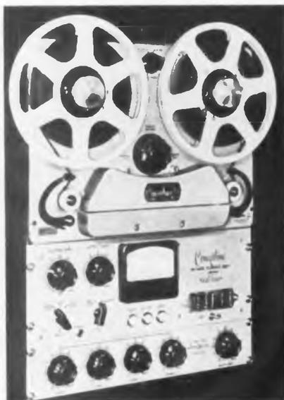
response is  $\pm 2$  db from 40 to 15,000 cps at 15 in./sec., and  $\pm 2$  db from 50 to 9,000 cps at 7.5 in./sec. Signal-to-noise ratio is 55 db and harmonic distortion is 2% at zero VU. Flutter and wow is 0.1% rms at 15 in./sec. and 0.2% at 7.5 in./sec., with playback timing accuracy  $\pm 0.2\%$ . —Berlant Associates, 4917 W. Jefferson Blvd., Los Angeles 16, Calif.—TELE-TECH.
