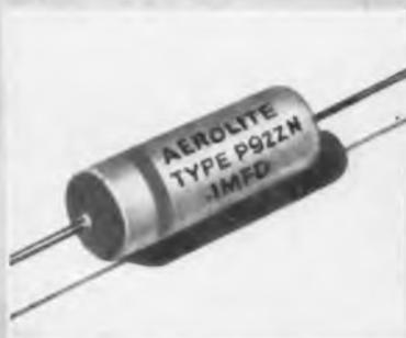
Series P92ZN Aerolene-impregnated metallized-paper capacitors are modified plastic-tubular duranite-end-sealed units in paper cases. Operating temperatures of  $-30^{\circ}\text{C}$ . to  $+100^{\circ}\text{C}$ . 200, 400 and 600 V. D.C. 0.01 to 2.0 mfd.
