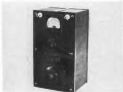
frequency range. With an impedance adjustable over a range of 40 steps from 2.5 ohms to 20,000 ohms, the instrument will measure 50 watts in steps of 0.1 mw., and db from -10 to plus 47 db. Over a range of 20 to 15,000 cps, the readings are accurate within 2%. The impedance changing network remains essentially resistive at audio frequencies, and the meter multiplier network has a constant impedance at all frequencies.—Daven Co., 191 Central Ave., Newark, N. J.—TELE-TECH.
