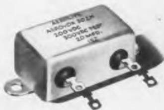
Series P30ZN Aerolene-impregnated metallized-paper capacitors housed in "bathtub" metal cases with vitrified or glass terminal seals. Operating temperature range of  $-55^{\circ}\text{C}$ . to  $+100^{\circ}\text{C}$ . at full rating; to  $+125^{\circ}\text{C}$ . at 75% of voltage rating. Capacitances available from 0.1 mfd. up to 15.0 mfd. at 150 V. D.C., and up to 3.0 mfd. at 600 V. D.C.
