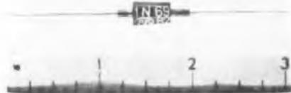
olic cartridge body indicates at a glance, by means of its taper, the direction of current flow. Nine different units, all vacuum filled with flexible wax, are available in following types: 1N48, 1N51, 1N52, 1N63, 1N65, 1N69, 1N70, 1N75, and 1N81. Range of characteristics for group is 2-5 ma at lv. forward, 50-1667 microamps at 50 v. reverse, 25-50 ma average, and 50-125 v. inverse peak.—Radio Receptor Co., 251 W. 19 St., New York 11, N. Y.—TELE-TECH.
