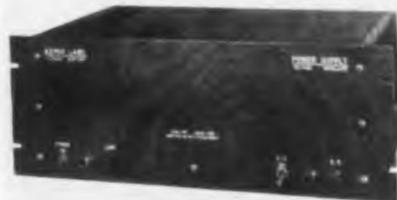
low output impedance. The dc output voltage is continuously variable from 0-3 v. and delivers from 0-100 ma. In the 0-3 v. range, the output voltage variation is less than 5 mv for both line fluctuations from 105-125 v. and load variation from 0-100 ma. Ripple is less than 1 mv. The unit is designed for relay rack mounting or bench use, width 19 in., height, 7 in., depth, 11 in.—Kepec Laboratories, Inc., 131-38 Sanford Ave., Flushing 55, N. Y.—TELE-TECH.
