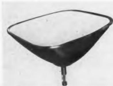
deflection. Screen provides picture area of approximately 390 sq. in. Face plate of tube is absorbent gray filter glass and is treated so that reflections from inner and outer surfaces are 97.5% eliminated. The 27QP4 can be used as a zero-voltage focus or can be focused to maximum sharpness with low-voltage supply. A single external magnetic field must be used in conjunction with the indicator ion trap to prevent ion spot blemish.—Rauland Corp., 4245 N. Knox Ave., Chicago 41, Ill.—TELE-TECH.
