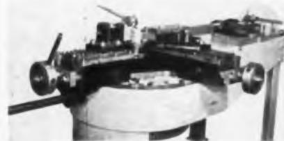
is 2 in. standard pipe 8 in. radius. The dies shown on the photograph are for bending 1/2 x 1 in. .065 wall copper tubing. Dies for larger size tubing can be furnished. The machine is arranged to travel 210° for bending parts requiring 203°, allowing for spring-back on large radius.—General Riveters, Inc., 785 Hertel Ave., Buffalo 7, N. Y.—TELE-TECH.
