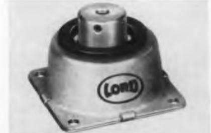
ature equipment function efficiently from  $-80^{\circ}\text{F.}$  to  $+250^{\circ}\text{F.}$  and can withstand a 30G drop test. Friction dampers prevent excessive equipment motion at resonant frequencies, and mounting drift is negligible even after long service.—Lord Manufacturing Co., Erie, Pa.—TELE-TECH.
