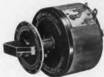
0-120/132 v., 1.25 amps, 150/165 va. This compact unit is intended for 50, 100 and 150 watt applications and operates cool. Type 10 is ruggedly designed for single hole mounting, has projection on its base for keying to panel, and may be installed under a 3 in. chassis.—Superior Electric Co., Bristol, Conn.—TELE-TECH.
