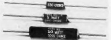
special silicone material seals the resistance element, making it impervious to moisture. Standard tolerance is 1%, but tolerances as high as 0.05% can be furnished if necessary. Temperature coefficient is practically flat. The resistance shift is less than 0.00002% C°. —Dale Products, Inc., Columbus, Nebraska.—TELE-TECH.
