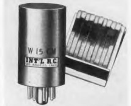
to fit standard sockets. All standard tube mountings are available. The unit illustrated (no. W15CM) is rated at 390 v. rms input; 550 v. peak inverse; 120 ma., 160 v. dc output at 35° C. ambient. Half wave and bridge circuits are also available—International Rectifier Corp., 1521 E. Grand Ave., El Segundo, Calif.—TELE-TECH.
