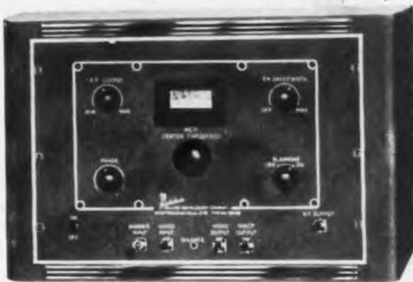
The Type 907 is a fundamental oscillator which can be swept in frequency over a band of not less than 10 mc/s for a center frequency of 35 mc/s. The sweep width is greater than 20 mc. for carrier frequencies above 60 mc/s. Output is continuously variable over a voltage range of 10 microvolts to 1 volt. Internal blanking circuits provide a "true zero" base line for an oscilloscope display.
