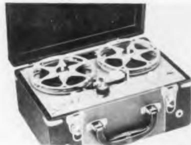
at 17½ in./sec. Monitored with earphones, the unit will pick up voices up to 100 ft. away. Frequency response is 100 to 3000 cps, signal-to-noise ratio is 45 db, speed variation is -0.2%, and battery life is 100 operating hours. Several optional accessories are available. Price is \$177.00 — Amplifier Corp. of America, 398 Broadway, New York 13, N. Y. — TELE-TECH.
