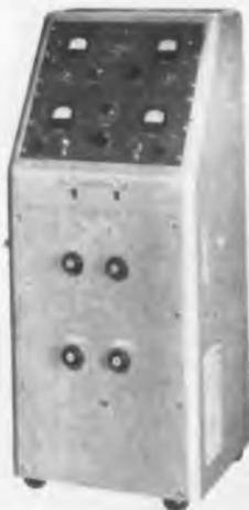
to one part of helium in 200,000 parts of air, or a leakage flow of less than 0.00001 standard cc/hr, presence of a leak is indicated by meter deflection or increase in pitch of an audio note. The unit is 22 in. wide, 21 in. deep, 52 in. high and weighs 350 lbs. Power consumption is about 800 watts at 115 v., 60 CPS. No cooling water is required. — Vacuum-Electronic Engineering Co., 756 Third Ave., Brooklyn 32, N. Y. — TELE-TECH.
