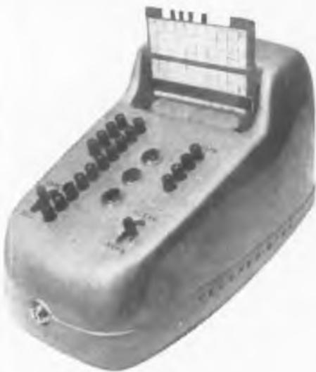
Fig. 1: Agent set with coded information plate queries storage drum to find seat availability
