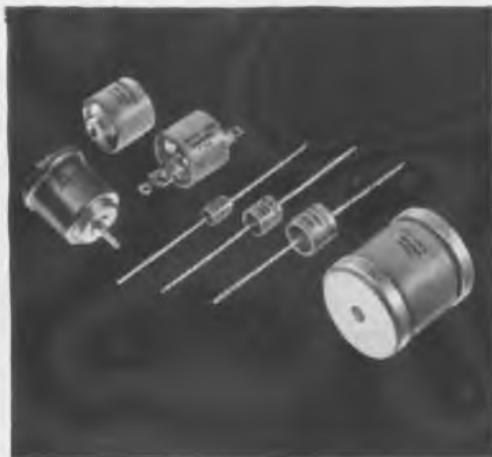
**HIGH VOLTAGE CERAMIC CAPACITORS.** Capacitance: 5 to 500 mmf, 5KV to 40 KV D.C. working. Ideal for portable or mobile equipment and high-voltage, high-frequency gear. Bulletin 42-102.
