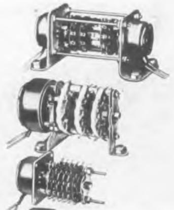
solenoids, have positive detent action and are self-stepping or external pulsing. Choice of wire sizes permits wide range of operating voltages. Solenoids are available in diameters from  $1\frac{1}{8}$  to  $3\frac{3}{8}$  in. with predetermined rotation up to  $95^\circ$ . Starting torque for  $45^\circ$  stroke range from 0.25 to 50 lb.-in. DC solenoids weigh from  $\frac{1}{8}$  to 4.25 lbs.—G. H. Leland, Inc., 123 Webster St., Dayton 2, Ohio.—TELE-TECH
