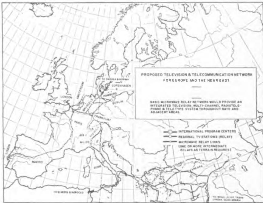
Map showing how principal cities of Europe can be linked in a microwave relay system that could provide an international television service along with both civilian and military communications facilities. Stations would be placed on mountain peaks and designed to operate unattended. Helicopters to be used to provide any necessary services. This system can also be integrated with a Trans-Atlantic TV System (see Aug. issue editorial and page 66, this issue). Full details in Tele-Tech next month.
