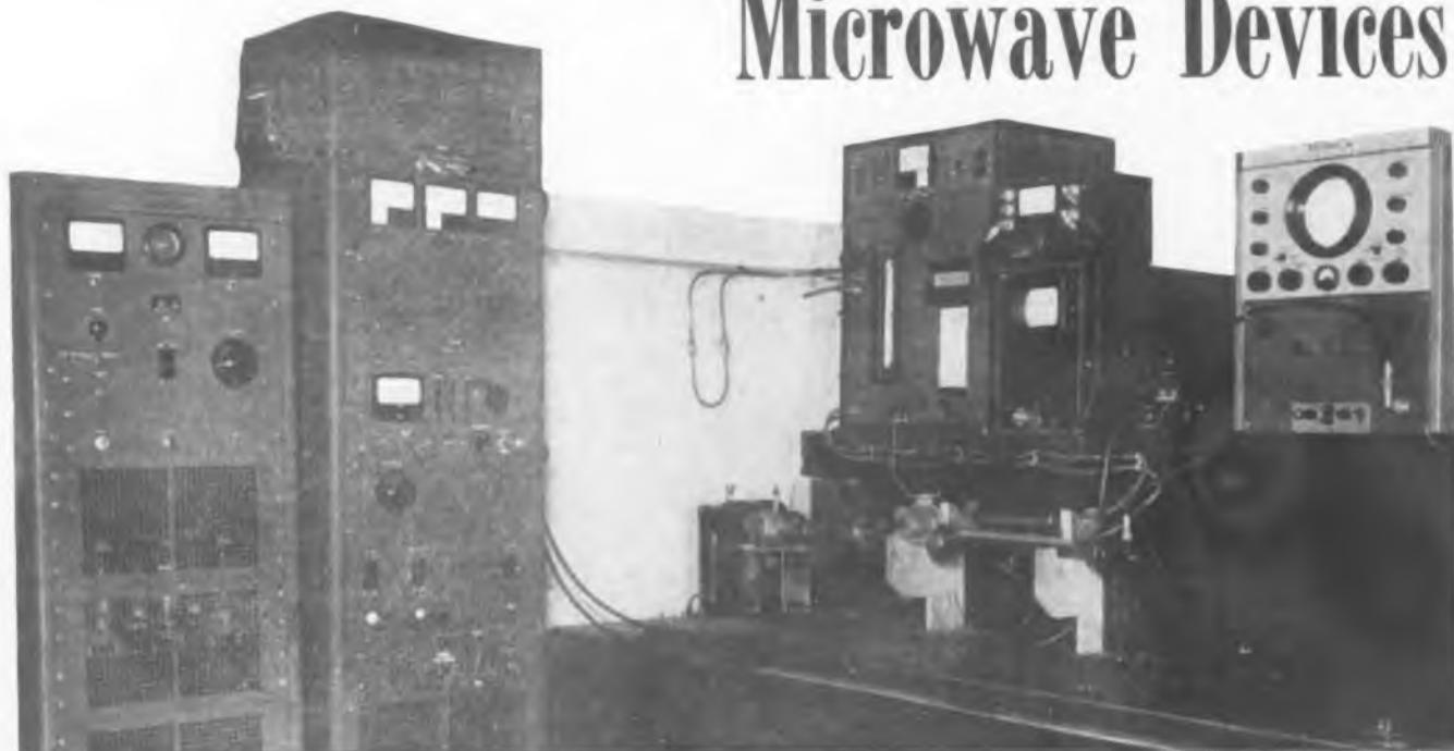
Fig. 1: Standard Amperex magnetron test station. Power supply, control and metering racks are at left. On shelf are power metering unit, synchroscope, r-f monitor and spectrum analyzer. Mounted above bench are magnetron under test, waveguide components, slotted section, wavemeter, and water load
