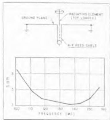
necessary because of the large aerodynamic drag figure of its predecessors resulting in decreased speed and maneuverability of the aircraft. The operating frequency of this built-in antenna is from approximately 100 to 156 MC,
