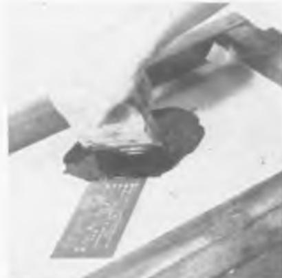
Fig. 7: Printing medium is poured at end of masked stencil and spread with rubber squeegee
