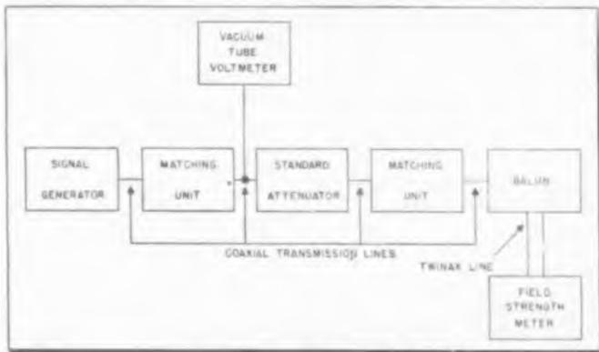
Fig. 3: (l) Arrangement used to determine overall linearity and attenuator ratios in VHF range uses balun and voltmeter monitor
