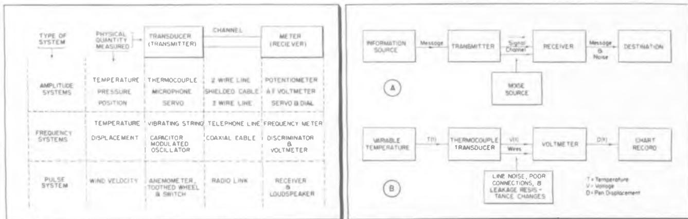
Table 1: (1) Examples of instrument systems for remote measurements. Fig. 1: (a) Elements of electrical and (b) instrument communication systems
