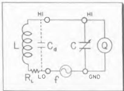
Fig. 1: (above) Basic circuit of Q-meter
