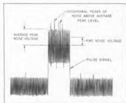
Fig. 2: Oscilloscope presentation of noise and signal. Average peak and rms noise are shown
