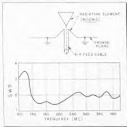
Command Equipment. The antenna was designed to operate satisfactorily inside the normal contours of jet aircraft with 50 ohm coaxial cable. It is described in USAF Specifications No. X-7074 and No. X-7172. The 55 oz. unit has the following dimensions: overall length, 15 in.; overall width, 2.5 in.; overall depth, 21.5 in. (forward-aft); length of element, 15 in.; and width of element, 2.5 in.
