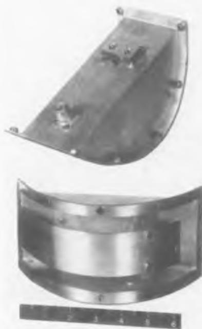
USAF Specification No. X-7196, and is particularly suitable for F-80 type airplanes. This antenna weighs 12 oz. and has the following dimensions: overall length, 7.75 in.; overall width, 4 in.; overall depth, 4 in.; length of element, 8.24 in.; and width of element, 1.75 in.
