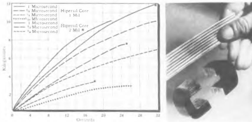
Fig. 5: (l) Comparison of effective permeability of 2- and 1-mil Hipersil cores. Fig. 6: (r) Extremely stable type-C core and a strip of the ribbed Hipersil steel from which it was wound
