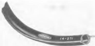
ticularly suitable for UHF-TV. Nominal impedance is 300 ohms and velocity of propagation is 84%. Attenuation in db/100 ft. is as follows: 30 MC, 0.63; 60 MC, 0.93; 100 MC, 1.25; 200 MC, 1.82; 400 MC, 2.7; 500 MC, 3.0; 700 MC, 3.6; and 900 MC, 4.2. List price is \$0.08 ft., and in lengths of 100, 500 and 1000 ft. The price is \$7.93, \$35.38, and \$68, respectively.—American Phenolic Corp., 1830 S. 54th Ave., Chicago 50, Ill.—TELE-TECH
