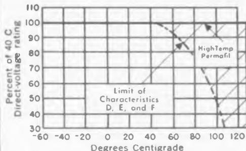
Comparison of operating voltages for JAN-C-25 characteristics D (vegetable oil), E (mineral oil), and F (synthetic insulating liquids) with Permafil impregnated capacitors—crosshatched area reveals advantages of Permafil over other impregnants in the high-temperature range above 40 C.
