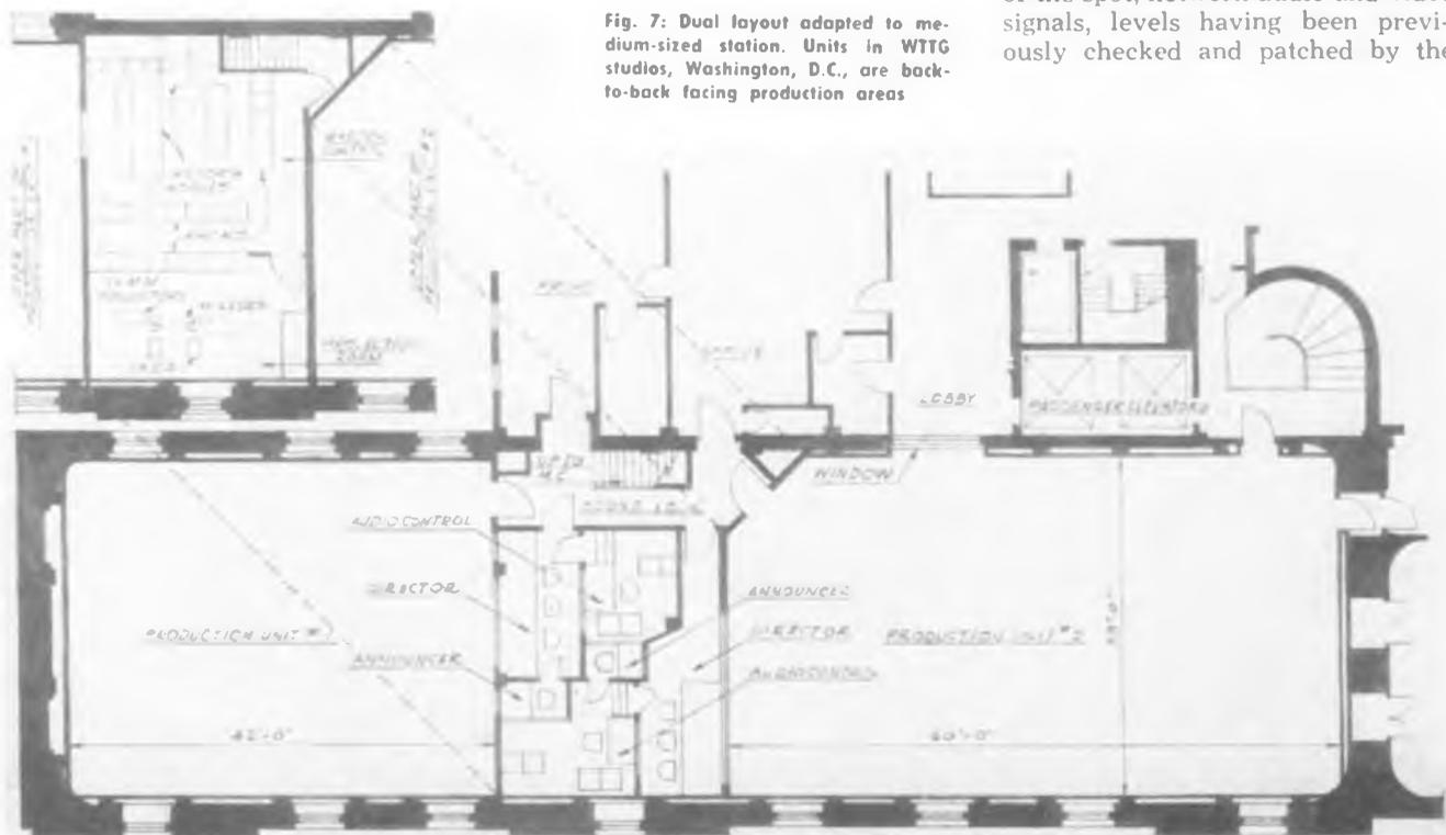
Fig. 7: Dual layout adapted to medium-sized station. Units in WTTG studios, Washington, D.C., are back-to-back facing production areas
