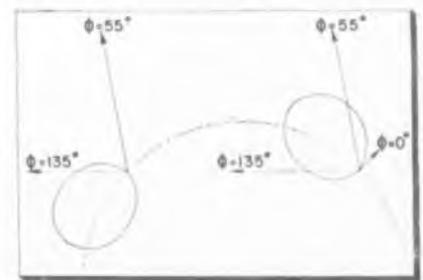
Fig. 4: Skewing element patterns around the supporting structure prevents deep nulls
