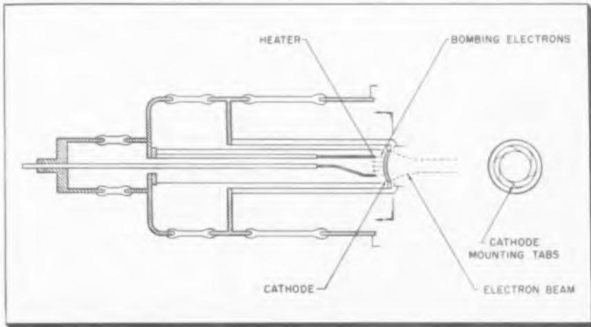
Fig. 2: Cross-section shows demountable cathode structure. Hatched areas are Kovar, clear areas glass
