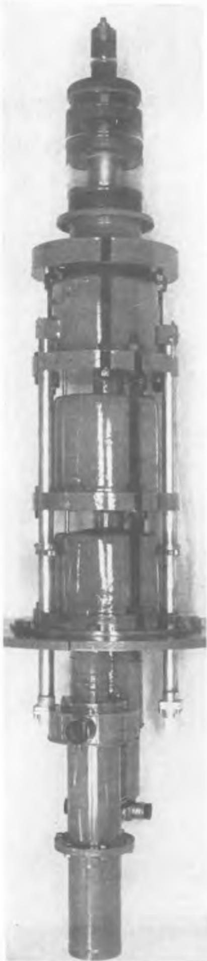
SEVERAL high-power klystrons have been produced and are seeing service in the 1000 mc region. These include the V-25 operated at 1036 mc by the National Bureau of Standards on Cheyenne Mountain, Colo., and delivering 5 kw, and the X-16 which forms a part of the General Electric TV transmitter announced last year.
