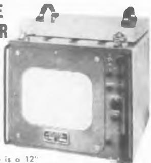
Model M-105 is a 12" picture monitor of size sufficient for ease of observation under studio conditions. It is a high impedance device and may be connected across a video transmission line without affecting the terminal impedance of the line. All adjustments are accessible from front panel.
