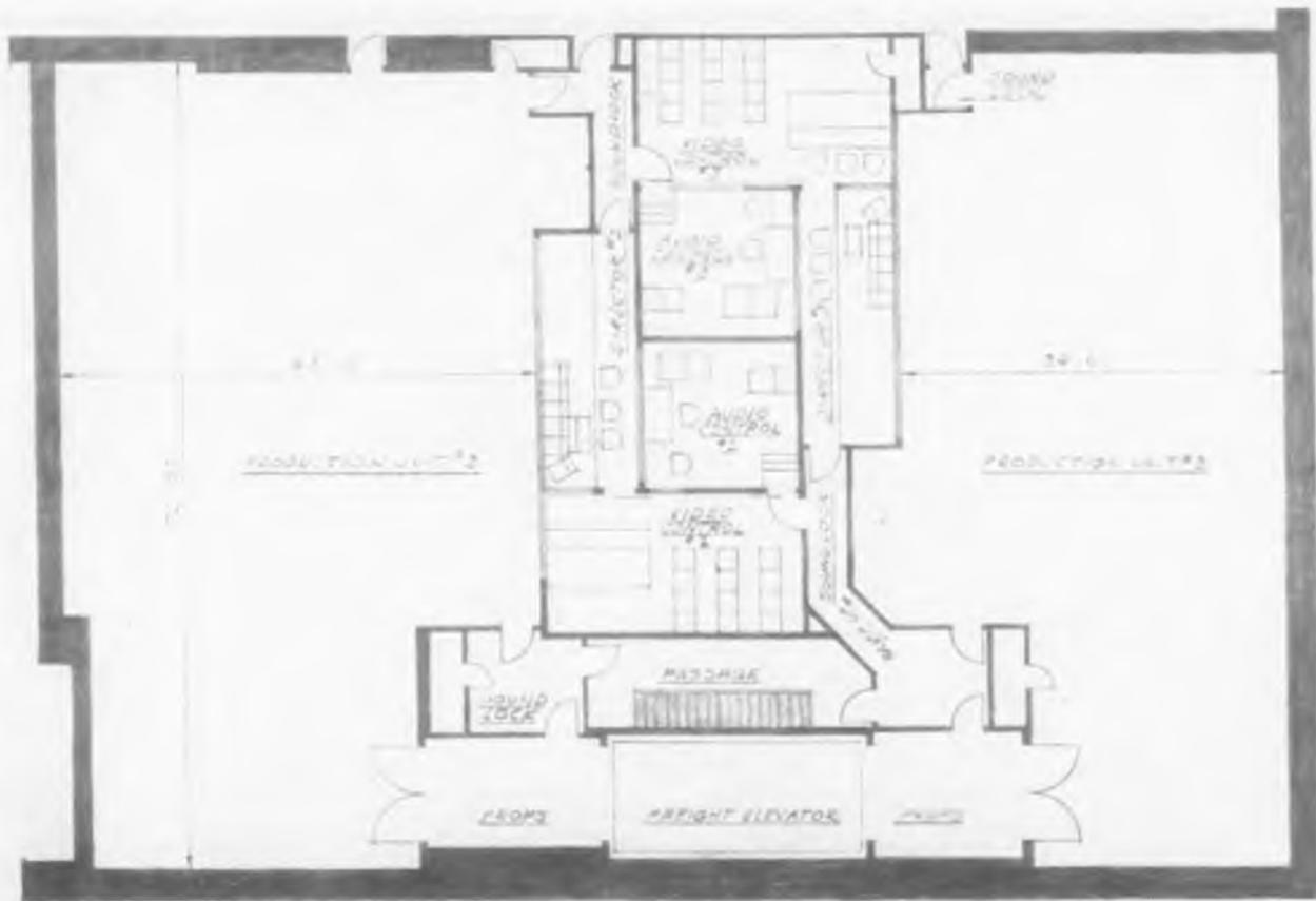
Fig. 6: Standard layout adapted to dual studio set-up. This type of control room is primarily for a station that is network origination center
