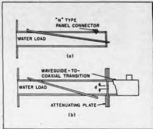
Fig. 5: (1) Two methods of sampling r-f in water load systems. Fig. 6: (r) R-F power monitor
