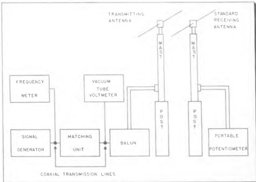
Fig. 5: Measuring antenna coefficient in the VHF range using the standard-antenna method
