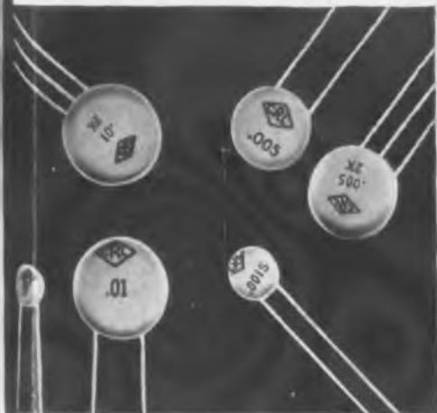
**CERAMIC DISC HI-KAP CAPACITORS** hold thickness to a minimum. Make possible very high capacity in extremely small size. Used in IIF by-pass and coupling. For details, write for Bulletin 42-4R.
