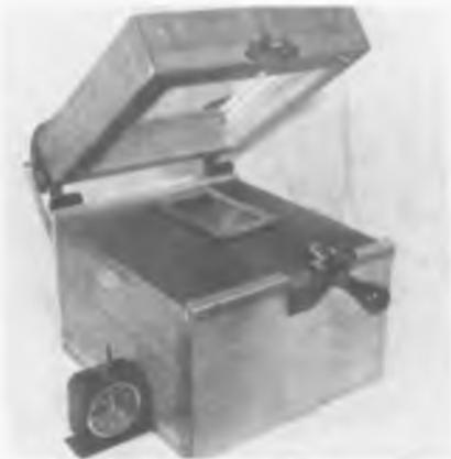
Fig. 4: Contact printer used to expose sensitized stencil film to pattern on transparency
