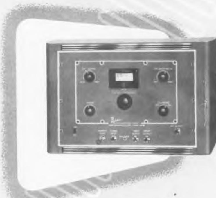
The Type 907 is a fundamental oscillator which can be swept in frequency over a band of not less than 10 mc/s for a center frequency of 35 mc/s. The sweep width is greater than 20 mc. for carrier frequencies above 60 mc/s. Output is continuously variable over a voltage range of 10 microvolts to 1 volt. Other features include a video blanking circuit for providing a true horizontal zero base line and a terminal for inserting external frequency markers.
