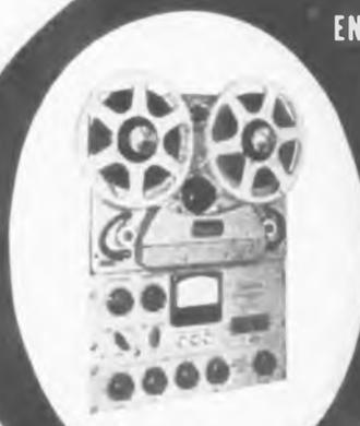
Direct drive eliminates idlers and clutches. Self-adjusting, positive disc brakes minimize maintenance. Simple threading plus push-button control affords foolproof operation.
