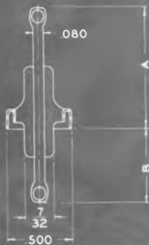
HERMETIC's new high voltage terminal is a glass-metal header that can take up to 10,000 volts and yet occupies only  $\frac{1}{2}$ " diameter on the mounting surface. It is amazingly rugged and will insure foolproof operation because of the diaphragm construction of the mounting. It is available with solid or tubular center conductors. Applications are many, among which are its use in transformers, choke coils, capacitors and pulsed circuits.
