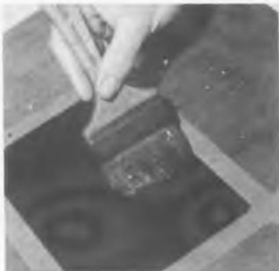
Fig. 3: Sensitizer is applied to film with a very soft camel hair brush, and then dried
