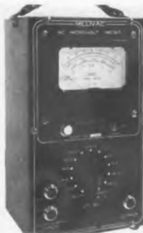
KC. The new meter has been extended to 6 MC. The instrument has a six-state amplifier with a novel ac regulated power supply. It measures voltages between 70 and 1000 v.—Millivac Instrument Corp., 444 Second St., Schenectady 6, N. Y.—TELE-TECH
