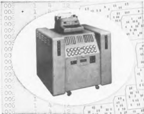
← **The Telecordex records** the Telereader measurements in decimal form electronically on its own electric typewriter, transmits the data to an IBM Summary Punch for card punching.
