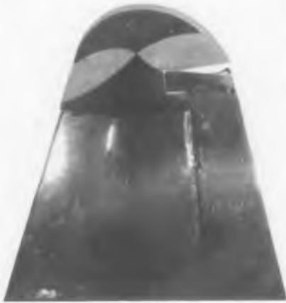
early part of 1946 to satisfy the requirements of a broadband antenna covering the frequency range of 100 to 400 MC and could be used with the following current equipments: VHF Command Equipment, IFF Equipment, and UHF
