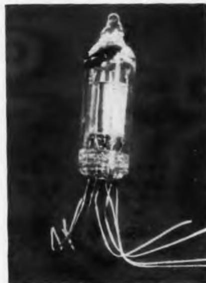
Fig. 8: High temperature subminiature tube
