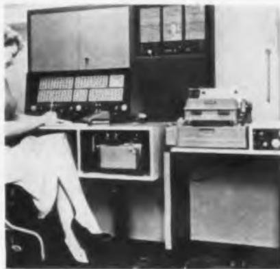
upon in parallel, while each successive decimal digit is handled serially. By this series—parallel operation, computational speed is materially increased over ordinary series operation, and the necessity for conversion from and to the decimal system for input and output is eliminated. **Consolidated Engineering Corp., Computer Div., 300 N. Sierra Madre Villa, Pasadena 15, Calif.**—TELE-TECH & ELECTRONIC INDUSTRIES
