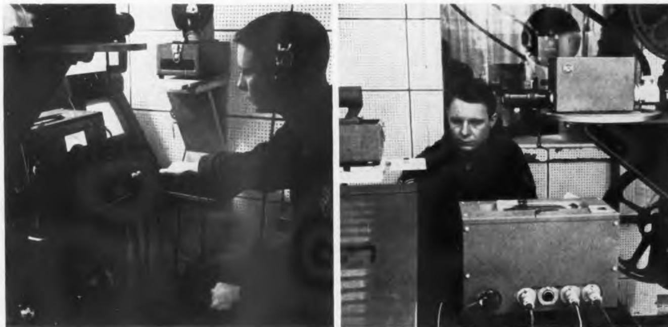
Control console program monitor (1) of the Air Force TV station at Limestone, Maine, which broadcasts programs of information and entertainment furnished without charge by major networks. Station is operated 5½ hours daily by base personnel under FCC approval. Power is 8 watts on channel 8. Vidicon camera chain (r) in 20 x 20 ft. studio is directed at slide projector. Camera may be swung by hand to face motion picture projector (reel visible at right)
