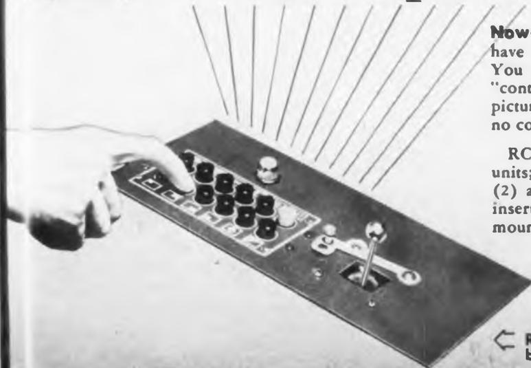
← RCA Special Effects Control Panel—with 12 push-button selection and 360° rotatable stick control.
