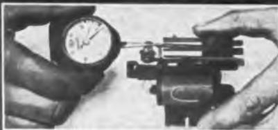
For determining the force required to actuate delicate mechanisms.
