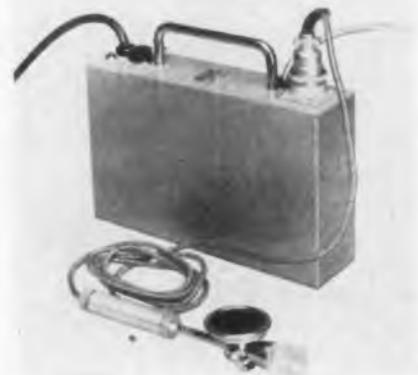
Heart microphone system developed by Altec Lansing includes small mike attached to stethoscope and power supply. Special cardiac conditions may be tape recorded for medical study. Amplifier is also used
