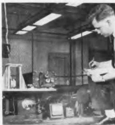
**6** Amplifier being vibrated. All units undergo sustained four-hour vibration test. Prototypes of this equipment have operated for two years without servicing.
