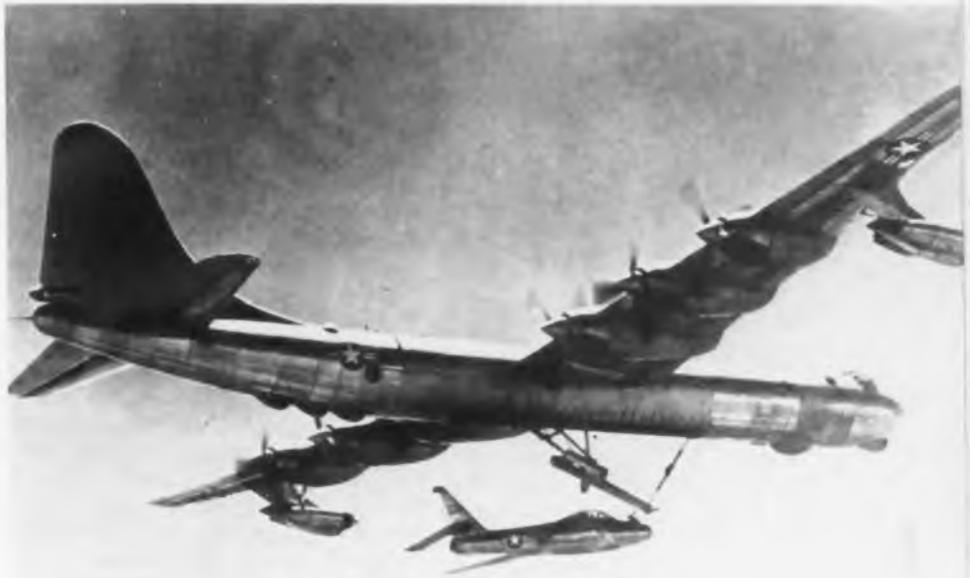
Parasite F-84F about to make contact with retrieving mechanism of RB-36F carrier plane
