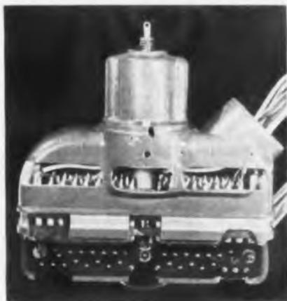
Fig. 8: Cut away view of early GMC type multi-contact connector designed for missile use. A number of contacts have been wired.
