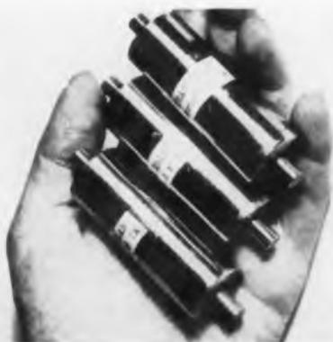
Unusual atomic battery developed by Alexander Thomas of Tracerlab uses radioactive tritium, can produce up to 400 volts at 0.01 to 1.0  $\mu$ w, and has a useful life of 10 to 30 years.
