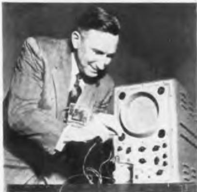
E. Finley Carter, Sylvania vice president and technical director, demonstrates by means of electronic testing equipment that an uncased transistor, stabilized by new scientific methods developed by Sylvania Electric Products Inc. was not affected by immersion in water. Demonstration took place recently in Washington before a group of high-ranking military officials.
