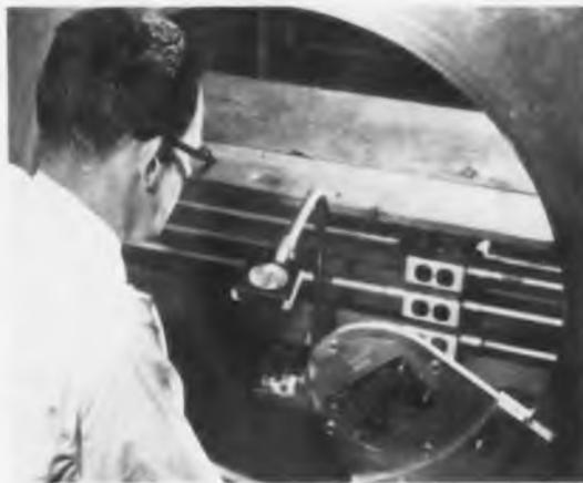
**7** Units mounted on the instrument panel must be checked for magnetic properties. Compass needle indicates effect of computer control being rotated in magnetic field
