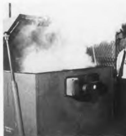
**5** Hot salt spray rises from tank subjecting units to 50 hours of corrosive atmosphere. Hermetic sealing and durability of plating and paint are rigidly controlled
