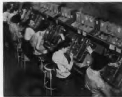
Color TV Chassis being assembled at GE plant in Syracuse, N.Y. Shipments of these sets are being made to areas covered by color TV broadcasts
