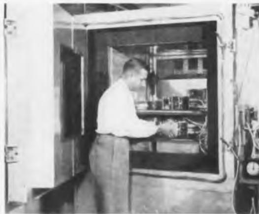
**4** Checking of units in high altitude chamber ensures efficient operation over wide temperature range—from -65° F to +160° F—and at altitudes up to 50,000 feet
