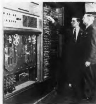
Fig. 10: Oarac digital computer developed by GE for ARDC contains 1400 tubes, 7000 diodes
