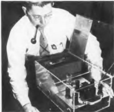
Transistorized 20 watt linear audio amplifier, developed by GE, uses two 6-watt, three 2-watt, and four 1/10-watt experimental transistors. The power transistors will be commercially available within two years
