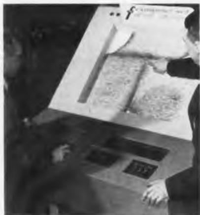
**2** Moving aircraft being tracked on display model of Ground Position Indicator. Accuracy depends largely on wind information and original settings
