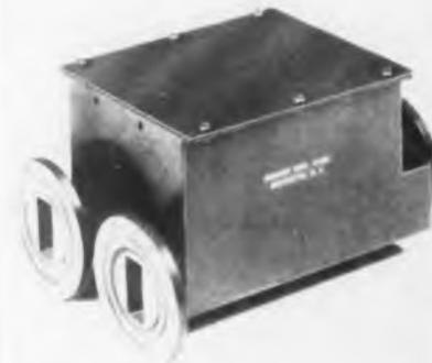
the disconnected member automatically, which provides a termination for the switched member and increases the isolation between arms to better than 60 db. VSWR is less than 1.10 over a 17% bandwidth, and the entire unit is operated by a momentary pulse at 115 v., 60 cps. power. Insertion loss through the connected member is less than 0.1 db. **Bogart Manufacturing Corp., 315 Seigel St., Brooklyn, N. Y.—TELE-TECH & ELECTRONIC INDUSTRIES**
