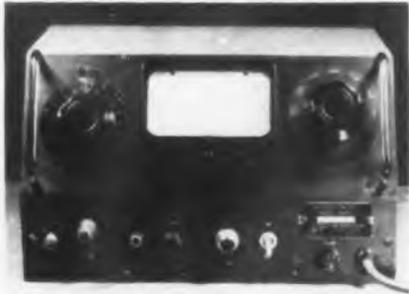
Fig. 1: FM demodulator and deviation meter
