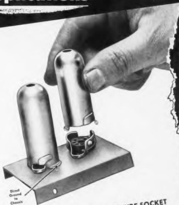
Recent addition to METHODE line of TUBE SOCKET ACCESSORIES is this new "Twist-On" type of tube shield and base, mounted in combination with molded sockets, as illustrated. Projecting lugs on shields provide direct ground to chassis under screw pressure and a reliable shock and vibration proof mount.
