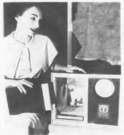
The Bigelow-Sanford Carpet Co. recently displayed its "impactometer," a device to measure sounds in the home. The hammer dropping on sample floor material inserted at left creates sound waves which are picked up by microphone. These sound amplitudes are then visible in CRO at right.
