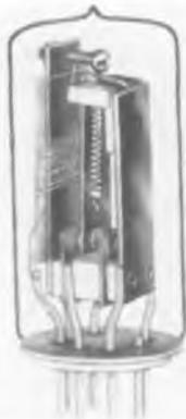
signed for ambient temperature operation ranges from 60° to 80° C., the relay operates on 6.3, 26.5, 115 v ac or dc, or as required. Time delay is from 2 seconds up. Withstands vibration of 30 G at frequencies from 5 to 55 cps. **Elly Electronics Corp., P.O. Box 395, Fair Lawn, N. J.—TELE-TECH & ELECTRONIC INDUSTRIES.**
