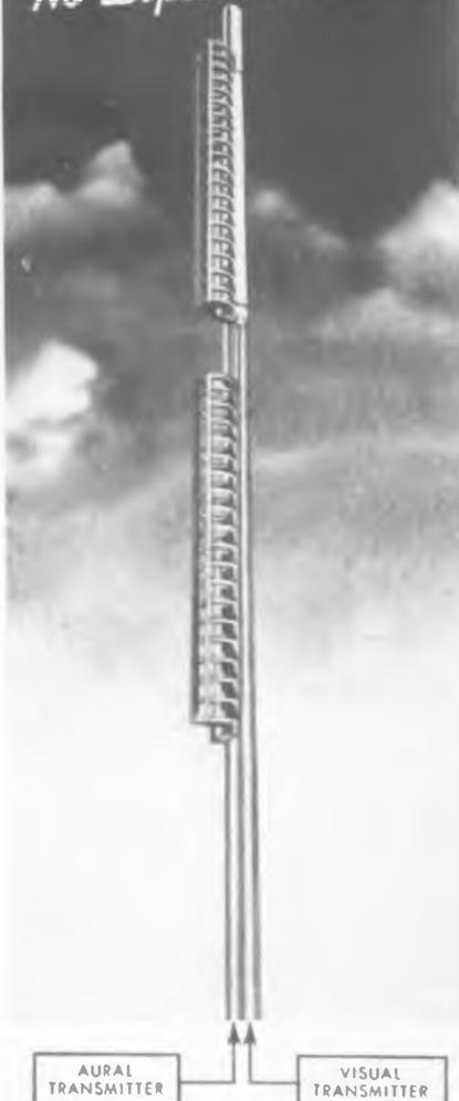
A simple, versatile and economical system consisting of two separate bays of type 1020 slotted-ring antenna can be used with a 50 kw transmitter. No diplexer of any kind is needed. The aural and visual transmission lines need not be of equal lengths. Write for Bulletin T-854.
