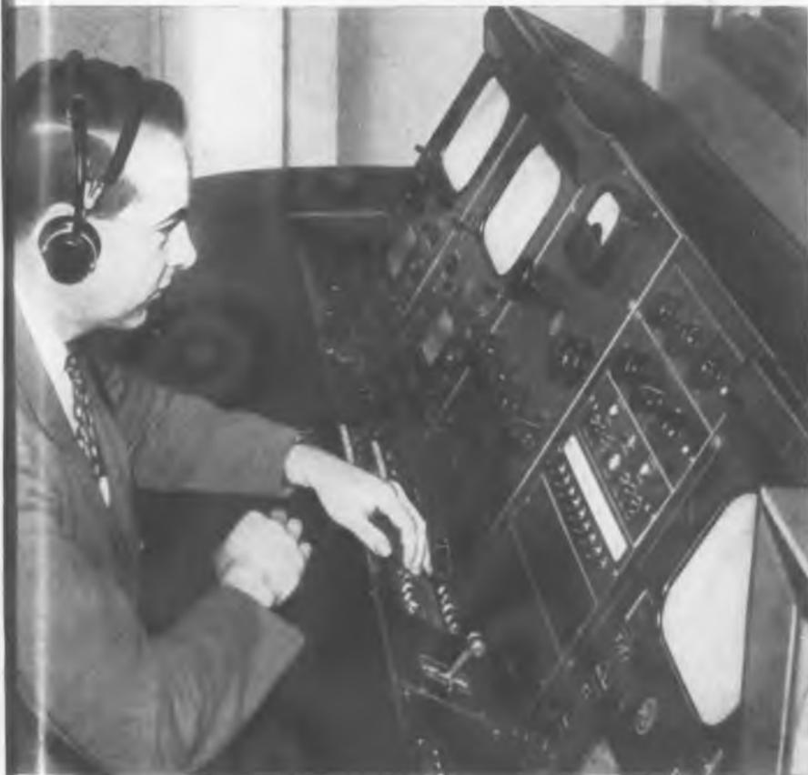
The RCA TS-5A Video Switcher is a flexible two-unit equipment designed to mount in a single standard console housing. The push-button and fader panel may be located as illustrated or in the upper face of the console. The TS-5A is designed for color use as well as for monochrome.
