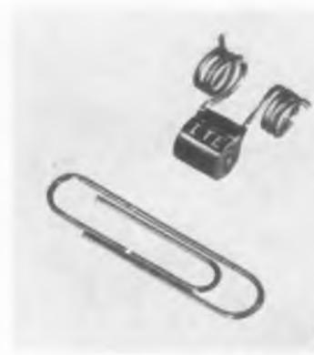
sealed unit is available in standard sizes down to  $\frac{1}{4}$  by  $\frac{1}{4}$  in. Designed to operate precisely in ambient temperatures ranging from -55 to 125° C. The unit features a low temperature coefficient of 20 ppm/degree C. and high stability. Resistance change with time is less than one-third the tolerance. **I-T-E Circuit Breaker Co., 19th and Hamilton Sts., Philadelphia 30, Pa.—TELE-TECH & ELECTRONIC INDUSTRIES.**
