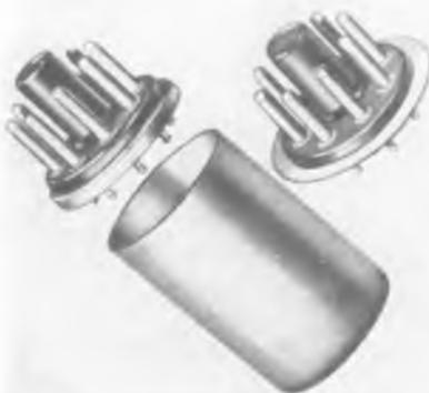
octal socket. Constructed as present Triad terminals, these plug-in terminals meet MIL-T-27 requirements and feature gold alloy plated solid brass pins to promote easier soldering and prevent corrosion. Available with either rolled or flat flanges. The rolled flange will fit either 1 in. or 1½ in. O.D. round can available at **Triad Transformer Corp., 4055 Redwood Ave., Venice, Calif.**—TELE-TECH & ELECTRONIC INDUSTRIES.
