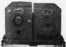
R-138 Receiver with D-10A Dynamotor
