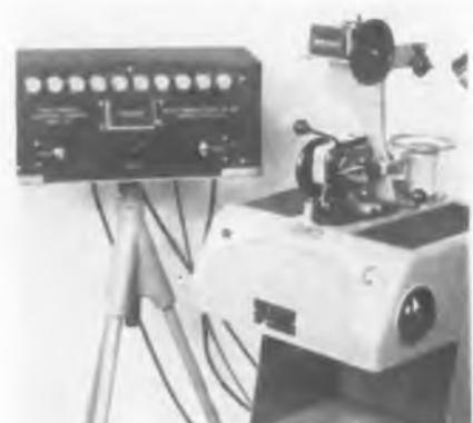
capable of winding down to ⅛ ID is now under test. Wire size range is #36 AWG through #46 AWG. With care, #48 can be used. Winding speed is adjustable from 0 to 600 turns/min. thereby enabling selection of the optimum speed for any winding problem. Controlled starting acceleration virtually eliminates wire breakage. **Boesch Mfg. Co., 45 River St., Danbury, Conn.**—TELE-TECH & ELECTRONIC INDUSTRIES.
