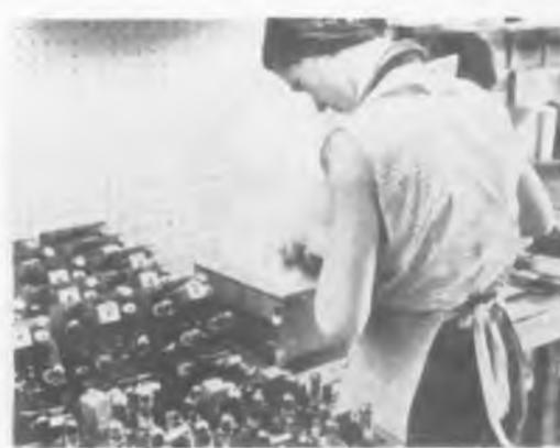
Dip soldering completes assembly. Robot I success has caused company to build two other larger machines scheduled for early 1955
