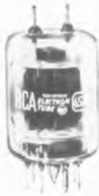
RCA-6524 is a new twin-beam power tube well-suited for fixed and mobile UHF design—as a balanced push-pull rf power amplifier or frequency tripler. The tube can deliver 20 watts (approx.) in class C cw and fm services—at 462 Mc! Max. plate dissipation is 25 watts (ICAS). A common cathode for the two units reduces cathode inductance to a negligible value.
