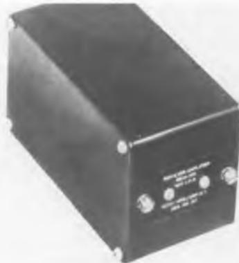
high frequency. Phase margin, 35 degrees—low and high frequency. Typical operating characteristics for frequencies between 380 and 420 cps are input 14 v, phase shift + 0.3 minutes, magnitude variation + 0.0004. Input 0.25 v, phase shift + 2.0 minutes, magnitude variation - 0.003. Ambient temperature range -55°C. to +75°C, phase shift ±1.0, magnitude variation, ±0.001. **Ketay Mfg. Corp., 555 Broadway, New York 12, N. Y.**—TELE-TECH & ELECTRONIC INDUSTRIES.
