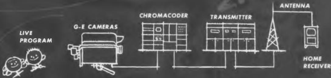
Excellent colorcasting results from either system, but Chromacoder, in fixed location, handles registration for all cameras in its system, and such adjustments are stable. See 3,5+7 for other advantages of fixed equipment.
