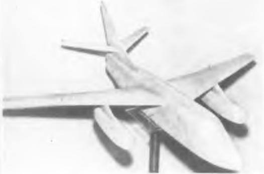
Fig. 6: 7-ft. long 1/12 scale model of Douglas RB66 has flame sprayed copper surface and weighs 33.5 lbs. Fabrication time 6 weeks
