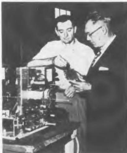
Walter L. Schott and Fred Miller (left) check printed circuit strip from new TV chassis PC-9. Design employs 25 tubes. Use of printed circuits reduces solder connections from 2900 to 56
