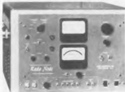
tubes of 1,200 to 26,500 mc in eight bands depending on wave-guide size. Noise figure is range 0 to 21 db. Its accuracy is to  $\pm 0.25$  db. IF amplifier frequency is (1) 30 mc (2) 60 mc. Amplifier gain is 75 db. Amplifier bandwidth is 14 mc. Input impedance is 50 ohms. **Kay Electric Co., Pine Brook, N. J.—TELE-TECH & ELECTRONIC INDUSTRIES.**
