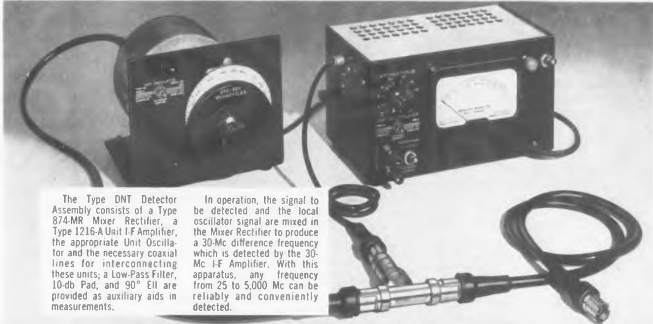
The Type DNT Detector Assembly consists of a Type 874-MR Mixer Rectifier, a Type 1216-A Unit I-F Amplifier, the appropriate Unit Oscillator and the necessary coaxial lines for interconnecting these units; a Low-Pass Filter, 10-db Pad, and  $90^\circ$  Ell are provided as auxiliary aids in measurements.
