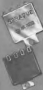
Mounted flat against a chassis with a screw or rivet, these miniature capacitors provide a highly secure mounting. 1 to 4 sections in the shallow pan are insulated and moisture-protected by a phenolic resin. Ideal for military electronics. These units have an unusually high self resonant frequency, and eliminate lead dress problems when mounted adjacent to a miniature tube socket. Available in ratings from 100 to 500 volts d-c. Write for Engineering Bulletin 611.
