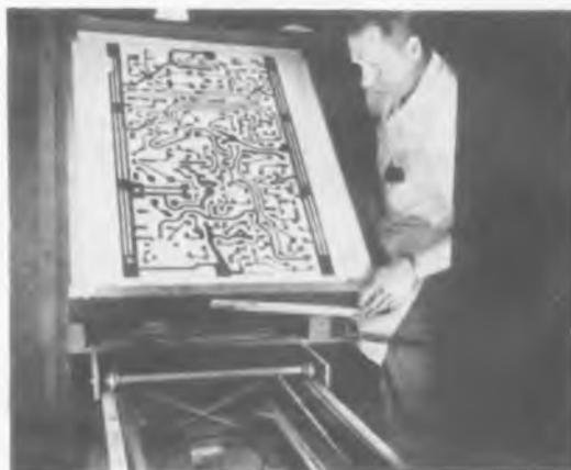
Large drawing of circuit layout is photographed and reduced to sharp actual sized negative. "Picture" is printed on aluminated plastic sheet one side of which is covered with copper foil
