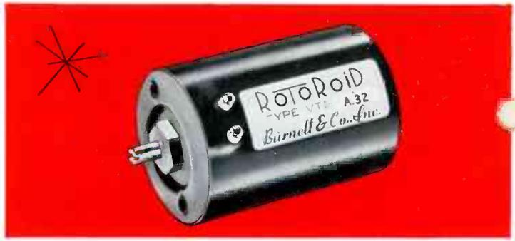
**ROTOROIDS®** A continuously variable, stepless toroidal inductor which can provide a 3:1 range of maximum to minimum inductance in 180° rotation of a shaft. Write for new brochure which gives complete technical data.
