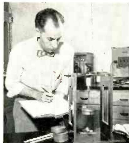
Fig. 4: Testing bond tightness. Done on a 1 x 4 in. strip with a 1 in. peel
