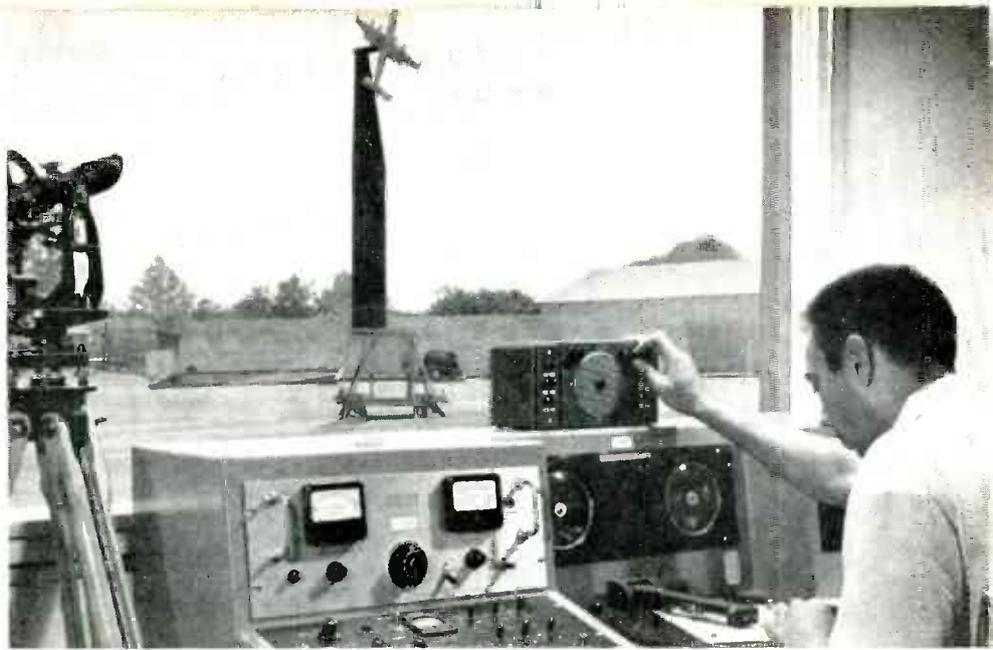
**Electronics Research Engineer Irving Alne** records radiation antenna patterns. Twenty-two foot plastic tower in background minimizes ground reflections. Approximates free space. Pattern integrator, high gain amplifier, square root amplifier and logarithmic amplifier shown in picture are of Lockheed design.
