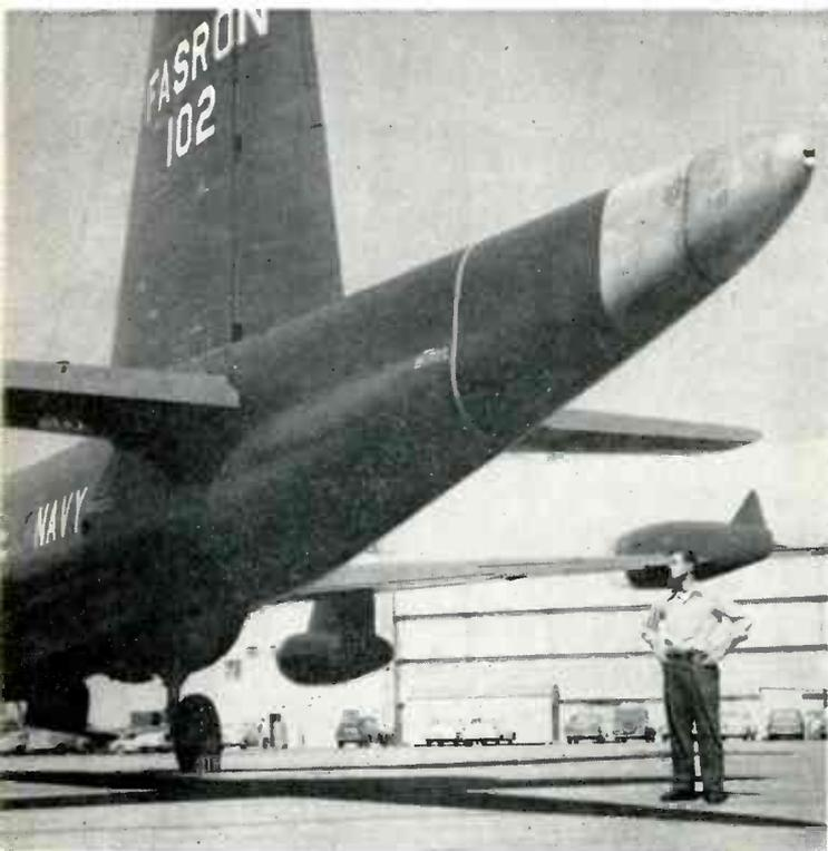
Stinger tail on U.S. Navy Neptune P2V-7 contains new electronic device capable of locating submarines hiding submerged beneath the sea. The Lockheed aircraft, called the "MAD-bird"—MAD standing for magnetic airborne detector—spots the subs by registering disturbances in the earth's magnetic field, and then lets loose with depth charges or torpedoes.
