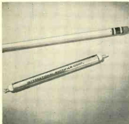
load. At 71°C ambient temperature—typical airborne ambient—the unit delivers 1.2 ma. dc current at 1,360 v. dc from 2,130 v. RMS ac. input. Lightweight tin-plated brass construction. Measures 5 1/8 in. overall with a 5/16 in. O.D. Also available is a complete range of selenium rectifiers with input voltages from 33 v. to 660 v. International Rectifier Corp., 1521 E. Grand Ave., El Segundo, Calif., TELE-TECH & ELECTRONIC INDUSTRIES. (Ask for 5-65)
