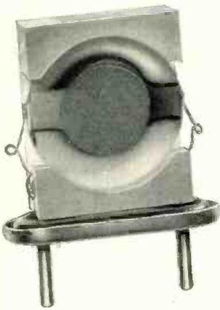
USE THE RH-7N, 1 mc CRYSTAL UNIT for exceptional frequency control. The Reeves-Hoffman RH-7N is securely shock mounted in a nylon nest, which all but eliminates frequency deviation. The RH-7N, a 1 mc crystal in an HC-6 holder, is built to meet requirements for MIL types: CR-18, 19, 27, 28, 35, 36 and 48/u.
