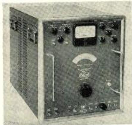
control with a direct reading dial and double-tuned r-f pre-selection. The unit receives AM, FM, and pulse, reads directly in db, and provides separate audio and video outputs. It provides for external metering and recording, and connectors for external i-f attenuators. Klystron voltages are automatically regulated and tracked with the oscillator. Polarad Electronics Corp., 43-20 34th., Long Island City 1, N. Y. TELE-TECH & ELECTRONIC INDUSTRIES. (Ask for 5-1)
