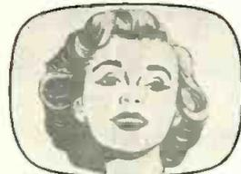
**RESULT**—A light background within the tube which reduces picture contrast.
