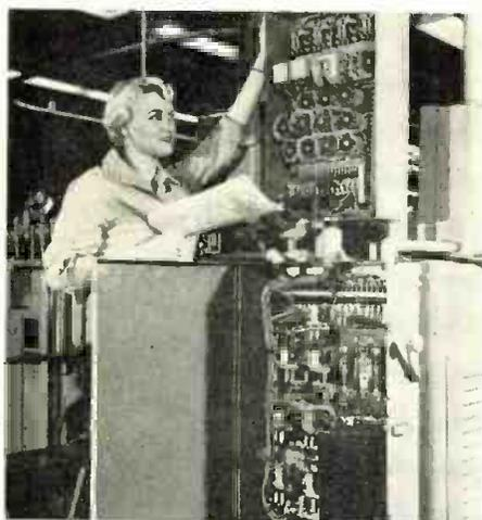
Cypak system panel (top) and relay control panel (below) for automatic bus duct welder
