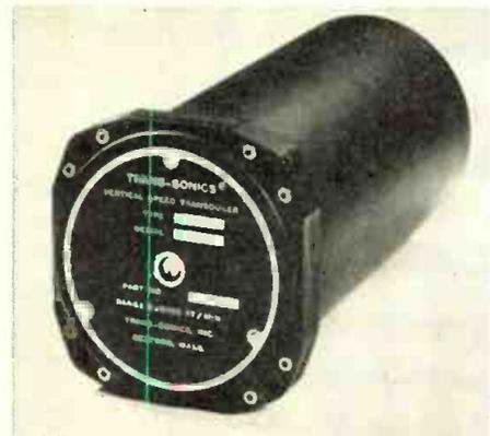
amic functions. The potentiometer wiper moves linearly with pressure over the range 3.42 to 30.36 in. of mercury. Accuracy,  $\pm 1\%$  of full scale voltage ratio. Trans-Sonics, Inc., Bedford Airport, Bedford, Mass. (Inquiry Card No. 6-38)
