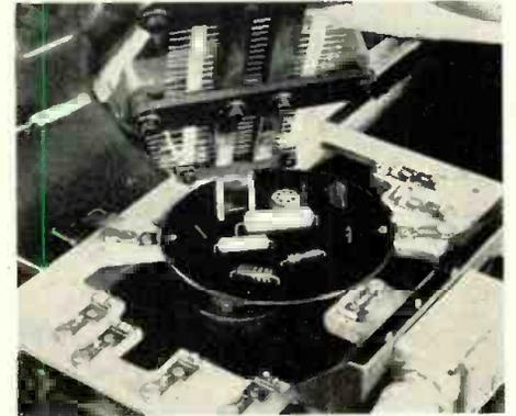
disc type capacitors; jumper wires; tube sockets; and i-f transformers. Included in this system is an advanced method of automatic dip soldering.
