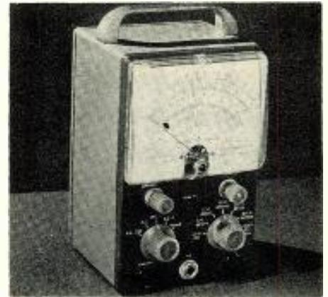
seven ac. (RMS) and dc. voltage ranges of 1.5, 5, 15, 50, 500, and 1,500; seven peak-to-peak ac voltage ranges of 4, 14, 40, 140, 400, 1,400, and 4,000; and ohm-meter ranges of X1, X10, X100, X1,000, X10k, X100k, and X1 megohm. A db scale is provided and a zero-center operation is within the range of front panel controls. Employs 4½ in. meter—1% precision resistors—ac. power supply. Heath Co., 305 Territorial Rd., Benton Harbor, Mich. (Inquiry card No. 6-22)
