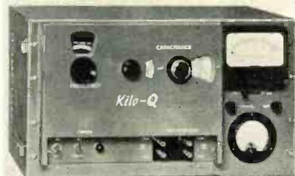
60-1,200  $\mu\text{f}$ . A vernier capacitor control in shunt facilitates tuning sharp "Qs." Oscillator frequency accuracy, 2 to 5%. Calibration capacitance accuracy, 1%. Kay Electric Co., 14 Maple Ave., Pine Brook, N. J. (Inquiry Card No. 6-54)
