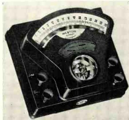
the moving coil; the instrument's first basic change. The outer frame serves as the yoke and provides excellent shielding and allows a minimum loss of flux. Relatively immune to the effects of external field influence, the movement has a high degree of magnetic stability. Used 15 inches from a conductor carrying 1,000 amps (a 5 oersteds field), effect is less than 0.10%. Weston Electrical Instrument Corp., 614 Frelinghuysen Ave., Newark 5, N. J. (Inquiry Card No. 6-16)
