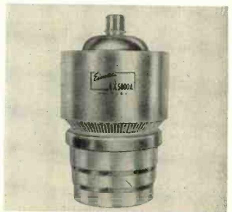
30 mc. The new tetrode delivers 10 kw. output in Class AB1 service and handles high inputs without going into the positive grid region. The simple coaxial structure allows low lead inductance, and a finned anode improves cooling with low air pressure. Offers greater electron tube reliability and increased immunity to thermal and physical shock damage. Eitel-McCullough, Inc., Technical Service Department, San Bruno, Calif., TELE-TECH & ELECTRONIC INDUSTRIES. (Ask for 6-9)
