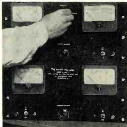
operation: series aiding, 400 to 1,000 v., 0-300 ma, grounded either polarity or anywhere between the two ends; parallel, 200-500 v., 0-600 ma, grounded either polarity with accurate load division up to full rating. Series bucking, 0-300 v. at 0-300 ma, grounded either polarity. Isolated, two identical, independent 200-500 v. supplies that can be operated in any polarity up to 1,500 v. apart. New Jersey Electronics Corp., 345 Carnegie Ave., Kenilworth, N.J. (Inquiry Card No. 6-77)
