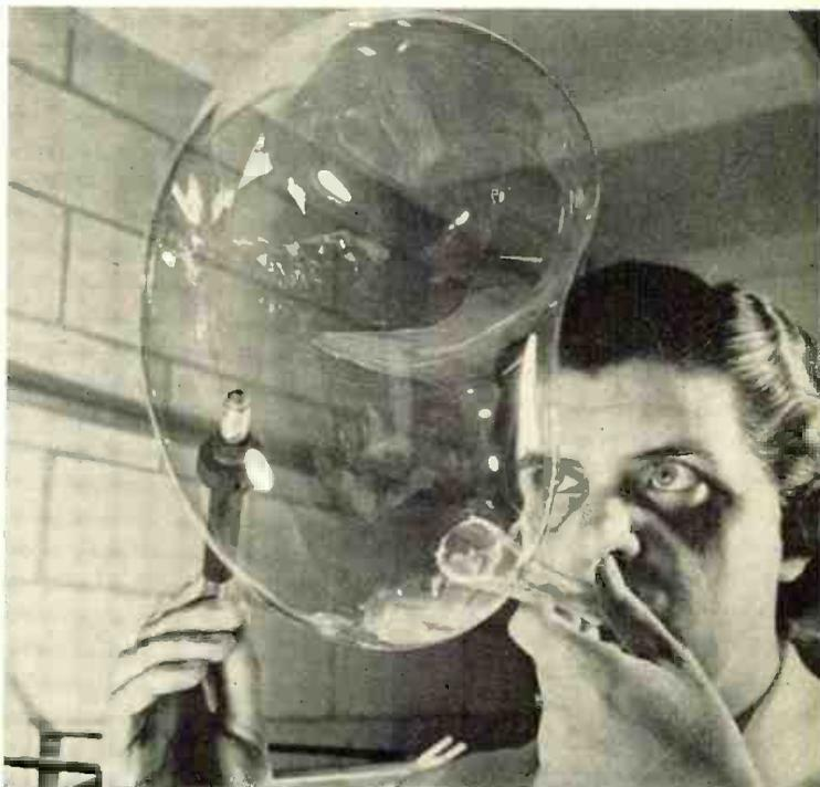
An employee at the RCA tube plant in Lancaster, Pa., blows a bubble from high quality optical glass and with a hydrogen flame cuts out a section having the exact curvature required for the “target” of an image orthicon camera tube. Only one “target” can be obtained from each bubble.
