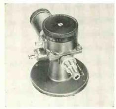
and easily in this region. VSWR may be read directly on the indicator meter by connecting the output to a VSWR indicator. The reflection coefficient angle is determined by rotating the top drum dial to a minimum indication on the meter and reading it directly in electrical degrees. Polytechnic Research & Development Co., Inc., 202 Tillary St., Brooklyn 1, N.Y.—TELE-TECH & ELECTRONIC INDUSTRIES (Ask for 9-57)
