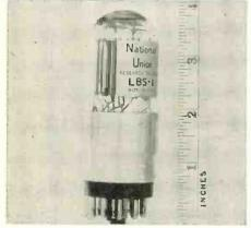
separate output anodes are provided. Outputs of 35 v. peak from each anode are obtainable across 100 K load resistors. By placing the unused anodes at B plus, less than 10 anodes can be used. Under normal 300 v. operation with 6ma. of cathode current, the 10 output anodes can be swept with a deflection voltage of 60 v. National Union Electric Corp., 405 Lexington Ave., New York, N. Y. TELE-TECH & ELEC-TRONIC INDUSTRIES. (Ask for 9-62)
