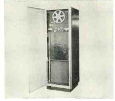
dated. With a Bk-1322 head and a 2-in. tape, 22 channels can be obtained; 44 by interlacing. Reel powered by a 1/2000 hp torque motor. Brush Electronics Co., 3405 Perkins Ave., Cleveland 14, O, TELE-TECH & ELECTRONICS IN-DUSTRIES (Ask for 9-55)
