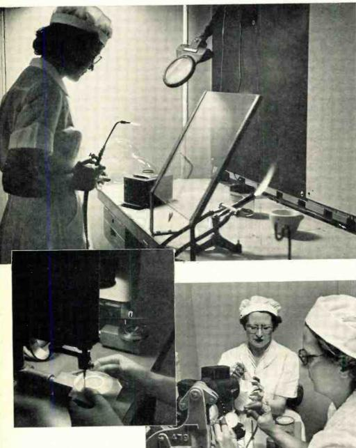
Extreme delicacy in processing parts for G-E camera tubes is shown as this glass technician fabricates an image-orthicon target. The glass bubble she holds is only 1/10,000 inch thick. After cutting out a small section, she seals this carefully to a metal ring. Any slip or other false movement would completely ruin the fragile target.
