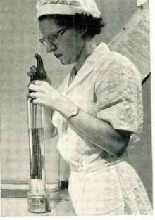
18-inch offset screwdrivers are used to tighten the set-screws holding target and mesh assembly in place in the camera tube. Skill, care, and time are needed to complete the delicate operation. Again, dust and lint are barred. An important step toward cleanliness, is the lint-free Nylon garments worn by all persons in the G-E camera-tube area.
