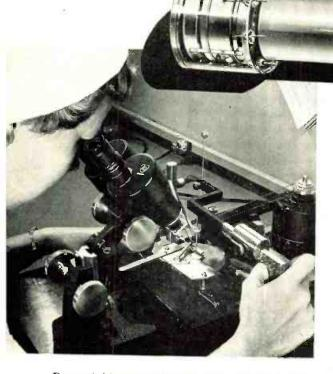
Powerful lenses aid trained hands. In building G-E camera tubes, numerous precision operations call for the aid of microscopes. Here a micro-drill operator drills a 1/500inch hole—less than the diameter of a hair —for the beam-limiting aperture in the first dynode of a G-E image orthicon tube.
