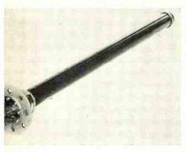
Reliability of a properly designed capacitance fuel guage has been demonstrated over the past ten years. This reliability is materially increased through transistors to obtain necessary amplification between the sensing tank units and fuel indicator. The new combination system is described herewith.
