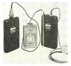
operates in the FM band of 26.110 to 26.470 MC with a 15 kc nominal deviation. A compact battery pack provides a minimum of 5 hours continuous operation. Power output is 75 mw and when used with type 128B receiver, broadcasting transmission (50-12,000 cps,  $\pm$  2 db) is achieved over distances of several hundred feet. Budelman Radio Corp., 375 Fairfield A.ve., Stamford, Conn. TELE-TECH & ELECTRONIC INDUSTRIES (Ask for 9-22)
