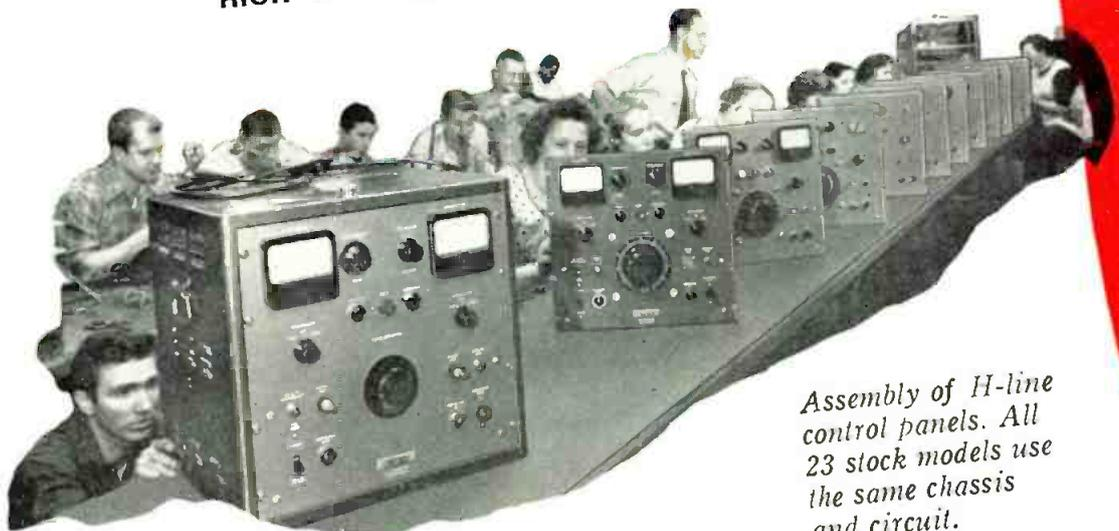
Assembly of H-line control panels. All 23 stock models use the same chassis and circuit.
