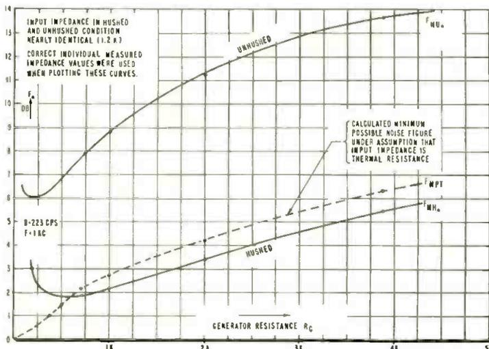
Fig. 10: Noise figure of same transistor in hushed and unshushed condition, measured at 1 kc.
