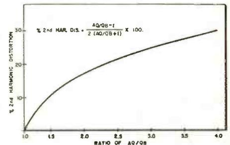
Fig. 1: Second harmonic distortion as a function of plate current swing
