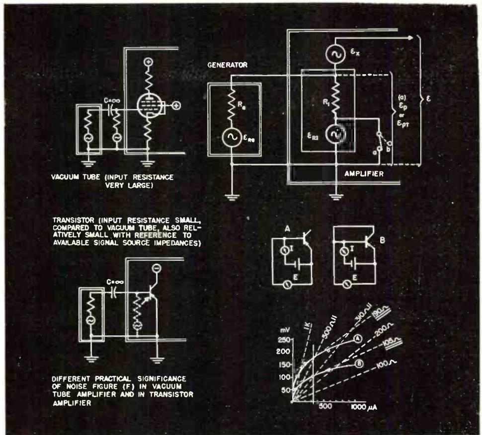
Fig. 11: (Left) Input circuits: of vacuum tube, and transistor, amplifiers. (Top right) Possible interpretations of  $F$ , by definition, or according to actual thermal noise conditions in input circuit
