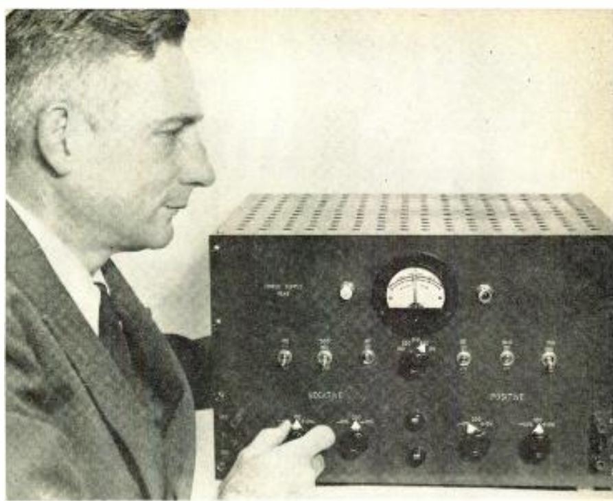
Stabilized voltage regulator in operation at NBS Labs
