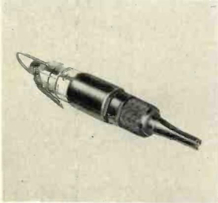
be used. Terminals may be made from commonly used metals and may be sq. or rectangular. Max. terminal dimensions are: .132 x .132 in. with a min. .375 in. spacing between terminals. Connection is 11/32 in. long. Tool weighs 2 lbs. An automatic device stops the bit in the correct starting position. Keller Tool Div., Gardner-Denver Co., Grand Haven, Mich. TELE-TECH & ELECTRONIC INDUSTRIES (Ask for 1-38)
