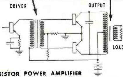
CLASS B TRANSISTOR POWER AMPLIFIER
