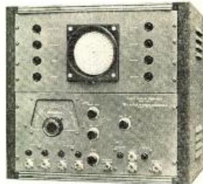
An important application of the PDE-1 is the study of phase response about the subcarrier frequency in color television receiver design. Shown below are typical displays of non-linear and linear phase systems.
