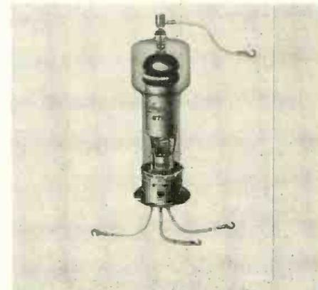
the 6786 is also grid-controlled. The tube has a "plate" type mounting support base and insulated flexible leads which make installation in equipment rapid and simple. Amperex Electronic Corp., 230 Duffy Ave., Hicksville, N. Y. TELE-TECH & ELECTRONIC INDUSTRIES (Ask for 1-30)
