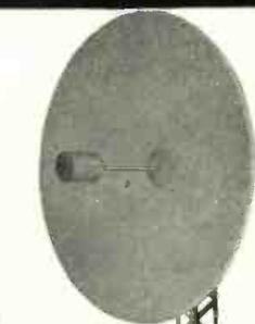
2000 mc antenna with dipole feed.
