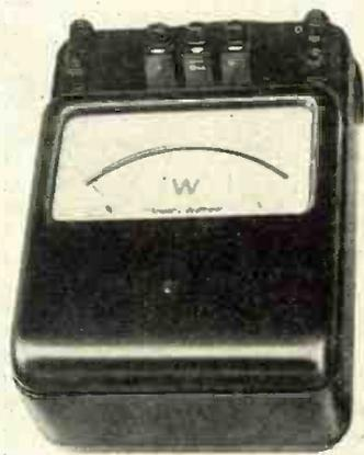
well adapted to the measurement of power consumption in relay coils, voltage coils, etc. Physics Research Laboratories, Inc., 507 Hempstead Turnpike, West Hempstead, N. Y. TELE-TECH & ELECTRONIC INDUSTRIES (Ask for 1-20)
