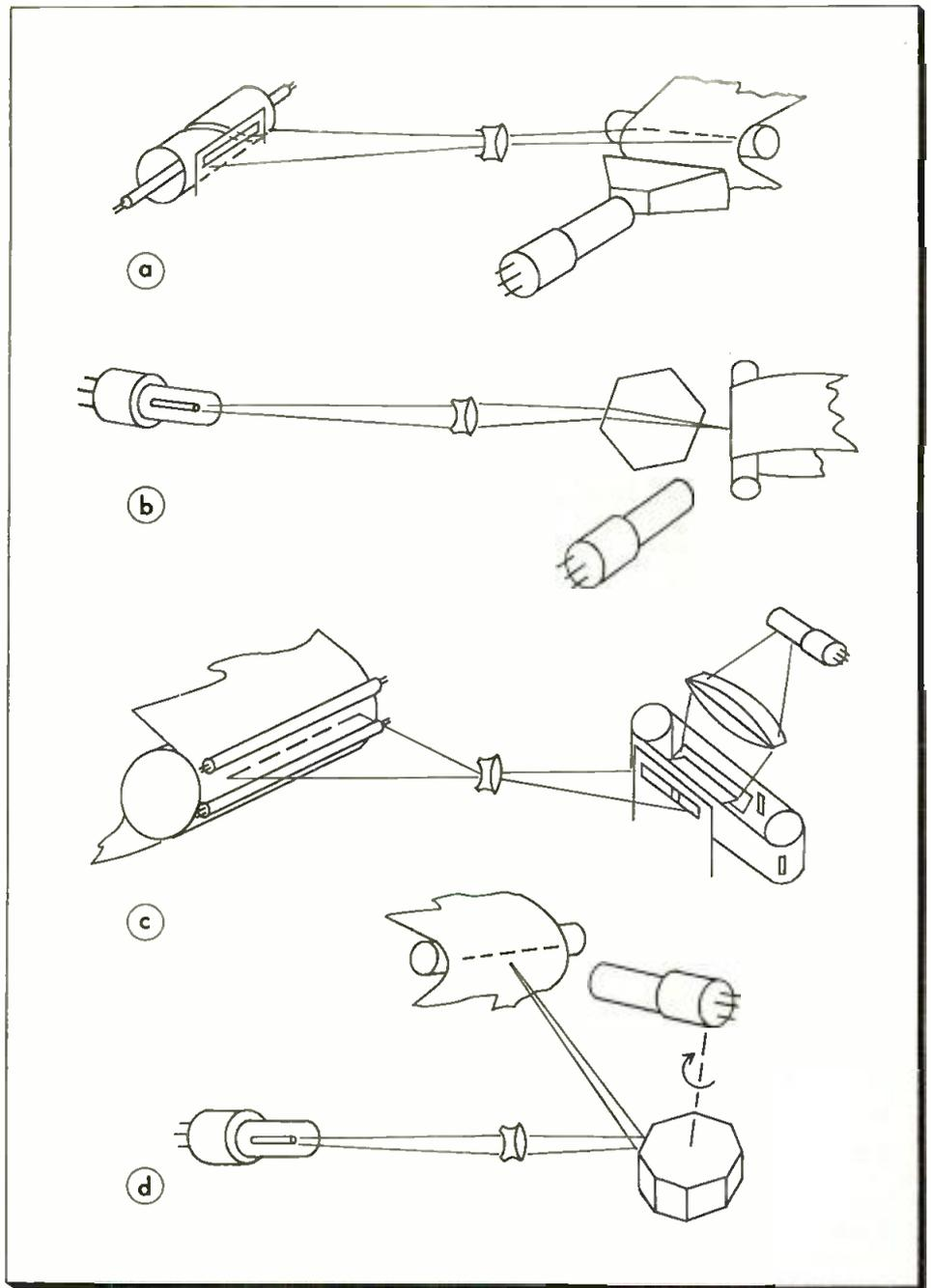
Fig. 3: Scanning methods: a. Helix and slit; b. Refraction through polygon; c. Slits on endless belt; d. Reflection from mirror.
