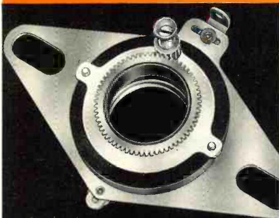
A Stackpole Ceramagnet ring  $3\frac{1}{8}$ " in diameter by  $\frac{1}{2}$ " thick forms the "heart" of this efficient, magnetic focusing unit produced by Glaser-Steers Corporation, Belleville, N. J. The entire unit weighs less than 13 ounces.
