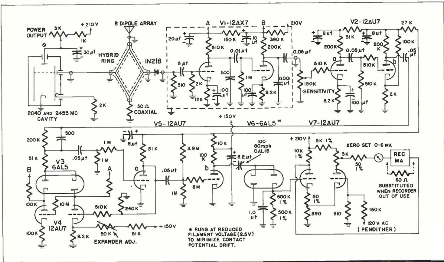
Fig. 1: Schematic diagram of typical radar speed meter. Power supply is omitted
