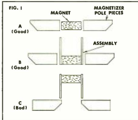
Magnetizing permanent magnets after assembly into the product offers several advantages. Higher field strengths are obtainable. The magnetic field produced in a loudspeaker, for example, using an Alnico V permanent magnet that has been magnetized after assembly, is about three times as great as the field obtained when the same magnet is magnetized before assembly.
