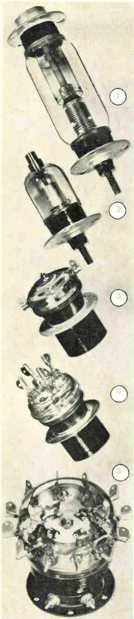
Fig. 1: (top) Metallic bellows type sealing
