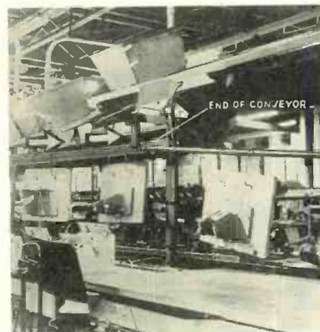
Rotating cable conveyor delivering empty pallets to slide rail storage
