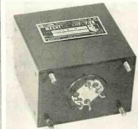
gain: 60; low drift: 1μa. Gives 5 mw output with a 300 mv input. Temp. range: -55°C. to +85°C. Units can be cascaded. Polytechnic Research & Development Co., Inc., 202 Tillary St., Brooklyn, N. Y. TELE-TECH & ELECTRONIC INDUSTRIES (Ask for 1-27)
