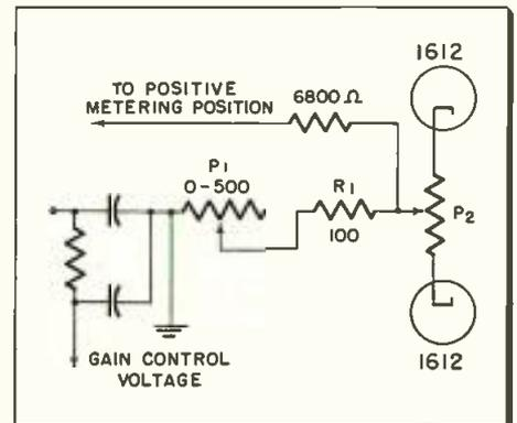
Tap off limiter provides remote metering
