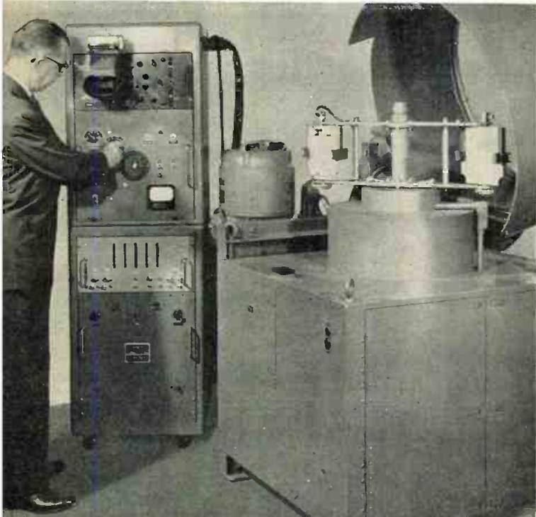
Unique new "Vari-G" Centrifuge, designed and built for the Navy by Hycon Mfg. Co. of Pasadena, Calif., will test two 1-lb. specimens simultaneously up to 300 G's, and two 10-lb. units up to 100 G's. The unit reaches peak velocity in less than 1/7th of a second, and virtually any acceleration can be simulated. Designed specifically for testing rocket fuses, the machine has reduced costs from \$120 to 20¢ per test.
