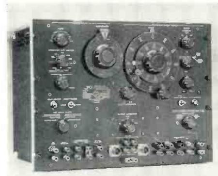
times of pulses, which are continuously adjustable in duration from 0.05 microsecond to 0.1 sec., can be precisely set at any point by amplitude comparators. General Radio Co., Cambridge, Mass. (Ref. No. 11-32).
