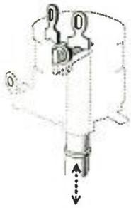
*Push the shaft and the set turns off. Pull, and it turns on at the same volume setting. New "floating ring" contacts give exceptionally long, trouble-free life.*
