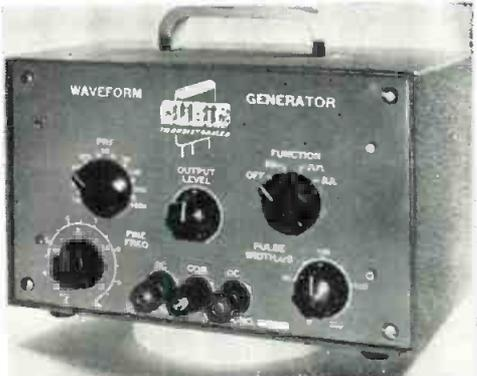
voltage an output of 7 volts at 2000 ohms impedance is available. The rectangular wave shape is continuously variable in pulse width from 5 to in excess of 200  $\mu$ sec. Cubic Corp., San Diego. (Ref. No. 11-23).
