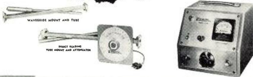
The WAVELINE Model 2200 microwave noise source—gas noise tube in combination with its Waveguide mount and power unit—provides a random noise source of known output level in the frequency range from 2,600 to 26,000 MCS. Throughout this range it also functions as an untuned termination.
