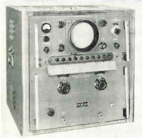
crowave test equipment development. The broadband r-f heads of FXR's Spectrum Analyzer permit operation with 1 head in the range from 950 to 16,000 MC. This improved microwave receiver affords greater sweep width and range, display is better and all controls are more convenient. Electronics & X-Ray Div., F-R Machine Works, Inc., Woodside, N. Y. (Ref. No. 11-15).
