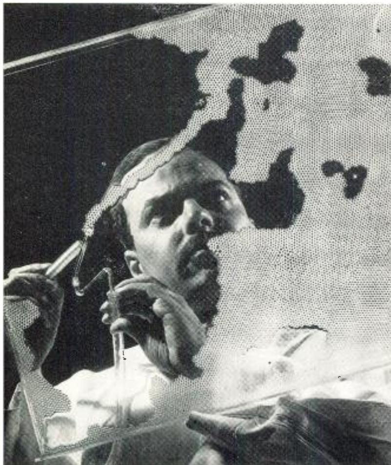
Dr. Wm. Mullins of Westinghouse Research Labs illustrates with soap bubbles how atoms group themselves into orderly "crystal structures." "Bubble" technique permits scientists to investigate on a vastly larger scale the patterns and defect structures formed by atoms in nature.
