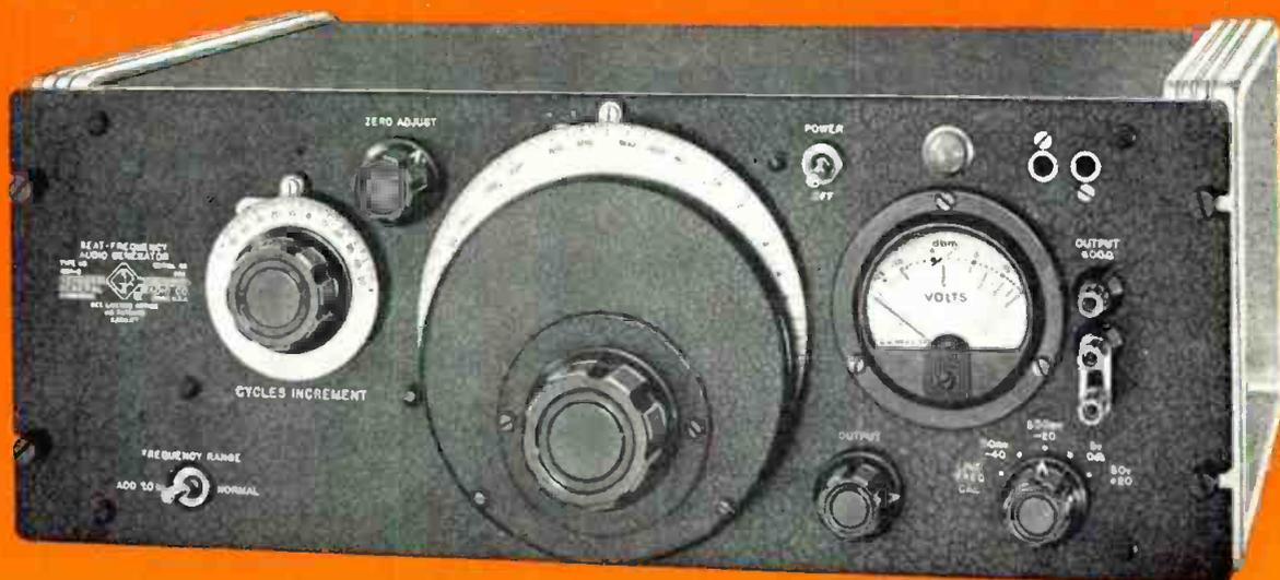
The versatile G-R Type 1304-B Beat-Frequency Audio Generator is the best test-signal generator for use at both audio and ultrasonic frequencies.
