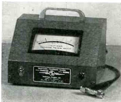
scale range is 0 to 0.01 in. H<sub>2</sub>O. Detects differences as small as 0.0001 in. H<sub>2</sub>O. Hastings-Raydist, Inc. Booth 3807.
