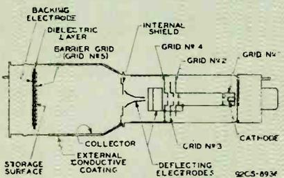
Fig. 6: Arrangement of elements in a barrier grid storage tube.
