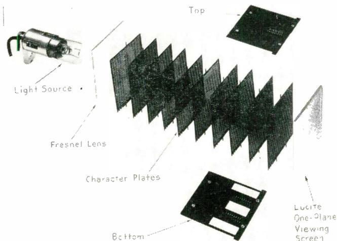
(Left) The various components of the readout display are shown in this exploded view.
