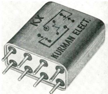
250 mw. Armature offers 20 g 2,000 cycle vibration and 50 g shock immunity. Kurman Electric Corp. Booth 2134.
