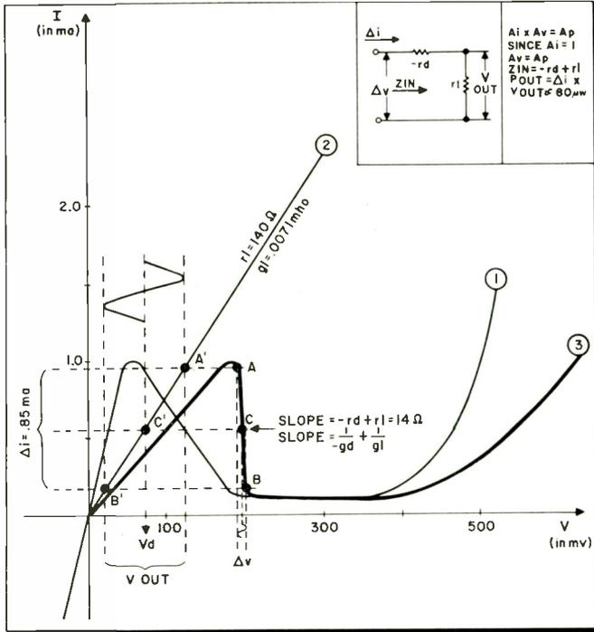
Fig. 7: This convenient graph should be used in studying the performance of series connection (open circuit stable) amplifier circuits.
