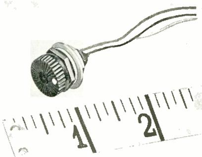
depth is 5/16 in. Power rating 0.5 w at 40°C, derated linearly to 0 at 105°C. Linear functions only. Dielectric strength is 900 VRMS at sea level for 1 min. Type A to 5000 ohms max.—tolerance  $\pm 5\%$  (25,000 cycles min. at 10 cycles/min. at rated power.) Type B (Trimmer) to 10,000 ohms max.—tolerance  $\pm 10\%$  (500 cycles min. at 2 cycles/min. at rated power.) Clarostat Mfg. Co., Inc., Dover, N. H.
