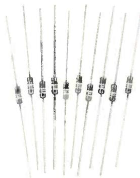
feature high forward-conduction and good recovery-time in units that are relatively low in cost. Available in all-glass "min" package with power dissipation capabilities averaging 80mW.
