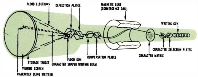
Fig. 16: Arrangement of elements in the Typotron, a display storage tube manufactured by Vacuum Tube Prods. Div., Hughes Aircraft Co.
