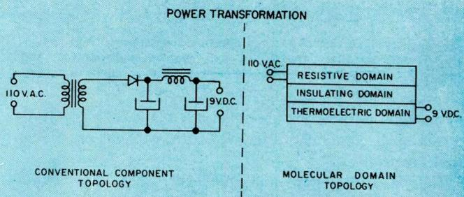
Fig. 7: AC to dc power supplies show (1) molecular element with its various domains, and (2) method using the conventional components.
