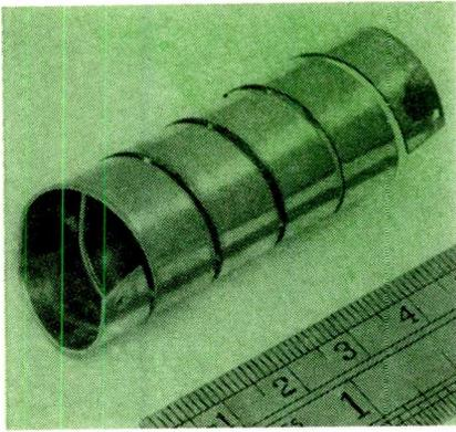
Fig. 29: Deflection plate used in the DuMont travelling wave deflection cathode ray tube.
