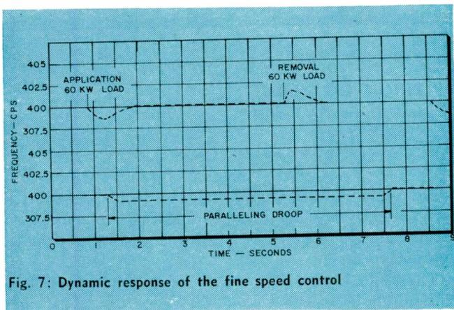
Fig. 7: Dynamic response of the fine speed control
