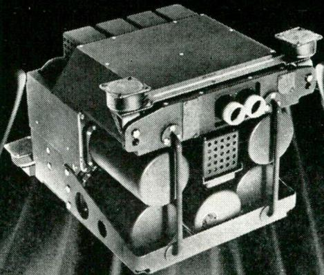
• *AiResearch Central Air Data Computer for North American's A3J, Navy's first weapon system, provides information dealing with bombing, navigation, engine inlet control, radar, automatic flight control and cockpit instrumentation.*
