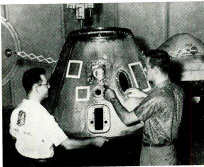
General Electric missile re-entry vehicle is equipped with instruments for measuring meteor sizes and electrical energy in space. J. Frissora of Geo-Sciences, Inc., Alamogordo, N.M., points to his self-designed membrane detector. It measures size of meteors by escaping gas. Extended ears are for measuring ion densities and potential of vehicle.
