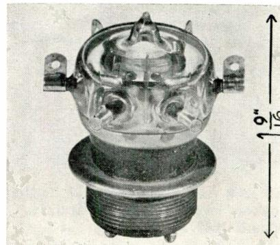
it measures 1-9/16 in. overall but has a rated operating voltage of 4 kv at 60 CPS and 2.5 kv at 16 MC. Continuous current rating is 6 a. at 60 CPS and 3 a. at 16 MC. It has a vacuum dielectric, sapphire actuating rod, and sealed rocker contacts for heavy contact pressure and resistance to vibration and shock. Contact resistance is low. Removable actuating coils are available for 26.5 vdc or 115 vdc operation. Jennings Radio Mfg. Corp., P. O. Box 1278, San Jose, Calif.
