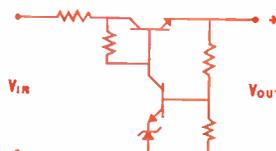
High voltage ratings and high temperature operation, plus internal power dissipation of 150 watts made possible by low thermal resistance of .7°C/watt make the 2N1015 and 2N1016 an ideal choice for constant voltage and constant current regulators.
