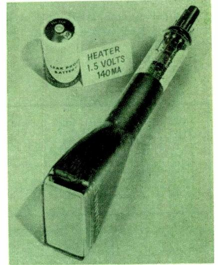
Fig. 30: First of a series of new developments will be lowering of the heater power.
