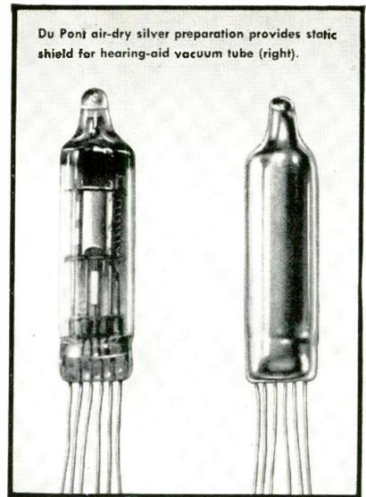
Du Pont air-dry silver preparation provides static shield for hearing-aid vacuum tube (right).
