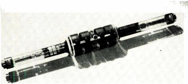
Fig. 8: The Raytheon dual-gun scan converter recording storage tube.
