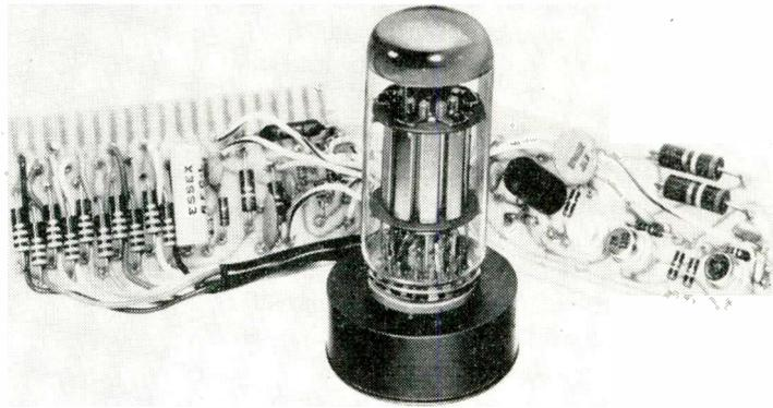
This Beam-X counting module uses only 56 components. All transistor module would require 146. Unit handles 110 KC counting frequency.
