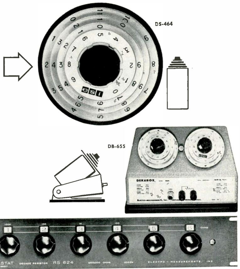
**MODEL DS SERIES DEKASTAT®**— Precision decade resistors for panel mounting, featuring the exclusive ESI DEKADIAL® concentric dial assembly for convenient straight line readings. Total resistance values available from 1,200 to 120,000 ohms with accuracy of  $\pm 0.05\%$ . Power rating,  $\frac{1}{2}$  watt per step. 3 or 4 decades of resolution. *Standard units available from stock. Prices: \$63.00 to \$110.00.*
