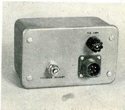
change; residual noise 1 mv typical; output impedance 0.10 ohm max., dc-5 KC; size 3 x 3 x 5 in.; weight 16 oz. Valor Instruments, Inc., 13214 Crenshaw Blvd., Gardena, Calif.
