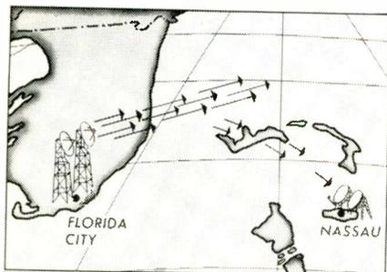
Dish-like antennas at "over-the-horizon" site at Florida City, Fla., are aimed at Nassau in the Bahamas. New system will carry 24 simultaneous telephone conversations. New link is joint undertaking of Long Lines Dept. of American Telephone and Telegraph Co., and the Telecommunications Dept. of the Bahamas Government.
