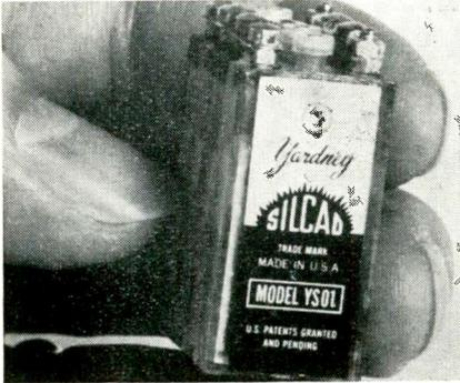
ampere-hr nominal capacity. It operates for 12 to 15 hrs before recharging. Yardney Electric Corp. Booth 2127.
