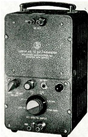
shunted by 15  $\mu$ f to 25  $\mu$ f depending on range. Output is a linear function of input voltage within its range. Ballantine Laboratories, Inc., Boonton, N. J.
