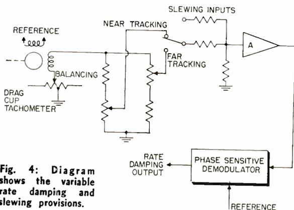
Fig. 4: Diagram shows the variable rate damping and slewing provisions.
