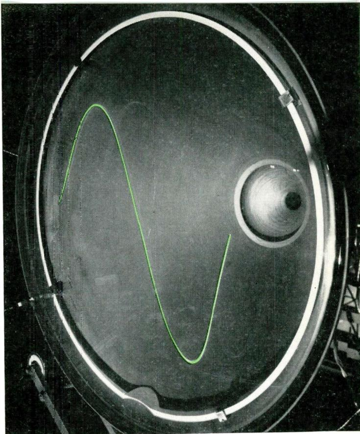
Fig. 2: Trace apparently suspended in mid-air on a DuMont 21 in. tube using a transparent phosphor. Used when ambient light is high.
