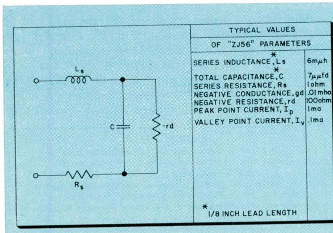
Fig. 2: Simplified equivalent circuit and parameters of a tunnel diode.
