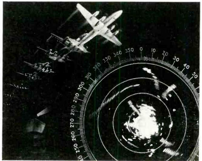
Aircraft at upper left, symbolizing the memory function, appears as target trail on Raytheon's Flight Tracker. System uses a Recording Storage Tube; presentation is on a high resolution picture tube.
