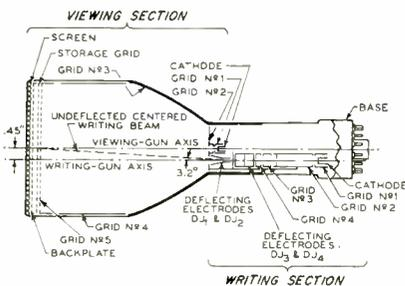
Fig. 14: Arrangement of elements in a display storage tube.
