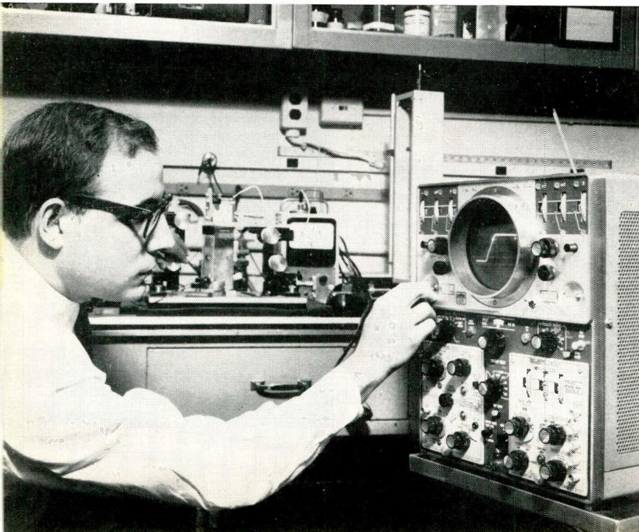
Du Mont engineers designed the 425 to include five separate modules. As a result, the distributed amplifier, one of the plug-in modules, was designed with a canted tube alignment to minimize coupling. Equipment does not require selected tubes for replacements.
