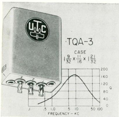
to 1% accuracy. Max. Q is approx. 160 at 7.5 KC down to 20 at 400 CPS and to approx. 30 at 75 KC for low inductance values. Hum pickup is low due to uniform toroid winding plus a high permeability outer case, providing 80 db at coupling attenuation. Units meet MIL-T-27A and carry MIL identification TF4RX20YY. United Transformer Corp., 150 Varick St., New York 13, N. Y.
