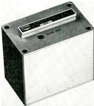
meets MIL-E-5272B Procedure III. It handles signals as low as 0 to 10 mv and as high as 250 mv. Under max. gain, an input signal of  $\pm 10$  mv will produce output signals of  $\pm 5$  v. Carrier rejection is 60 db or greater below max. output. Operating power is +20v. at 25 ma  $\pm 5\%$ . United Electro-Dynamics, 200 Allendale Rd., Pasadena, Calif.
