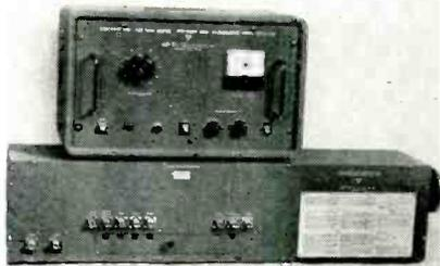
$\pm 1\%$  or  $\pm 0.05^\circ$  from 200 MC to over 1000 MC. Operating principle based on comparison method. Ad-Yu Electronics Lab. Booth 3705.
