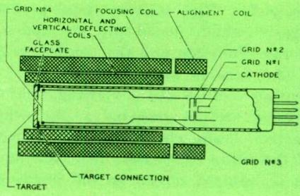
Fig. 19 (right): Arrangement of elements for operating a typical vidicon.
