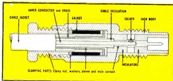
The inside story of ConheX superiority. Positive clamping action distributes holding action on jacket, shield and conductor of coaxial cable—different, and far better.
