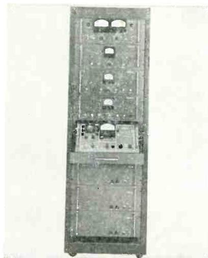
AM Stereo Adapter system develops two independent sidebands which are individually modulated by the two stereo inputs. Each sideband of the envelope wave can be demodulated by a standard AM receiver.
