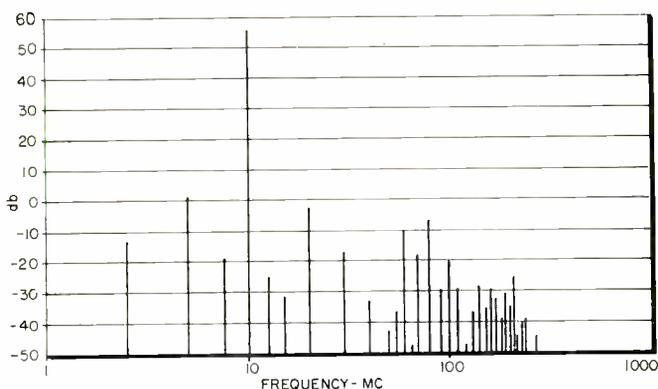
Fig. 5: Measured spurious and harmonic output for a transmitter which uses two frequency doublers is plotted
