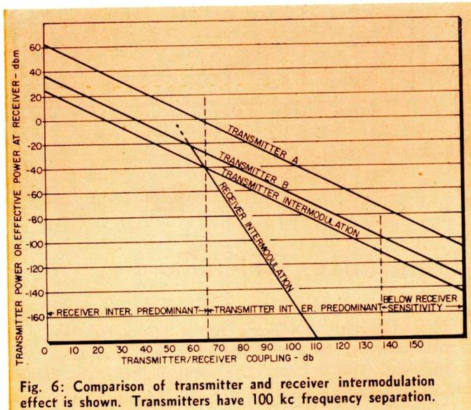
Fig. 6: Comparison of transmitter and receiver intermodulation effect is shown. Transmitters have 100 kc frequency separation.
