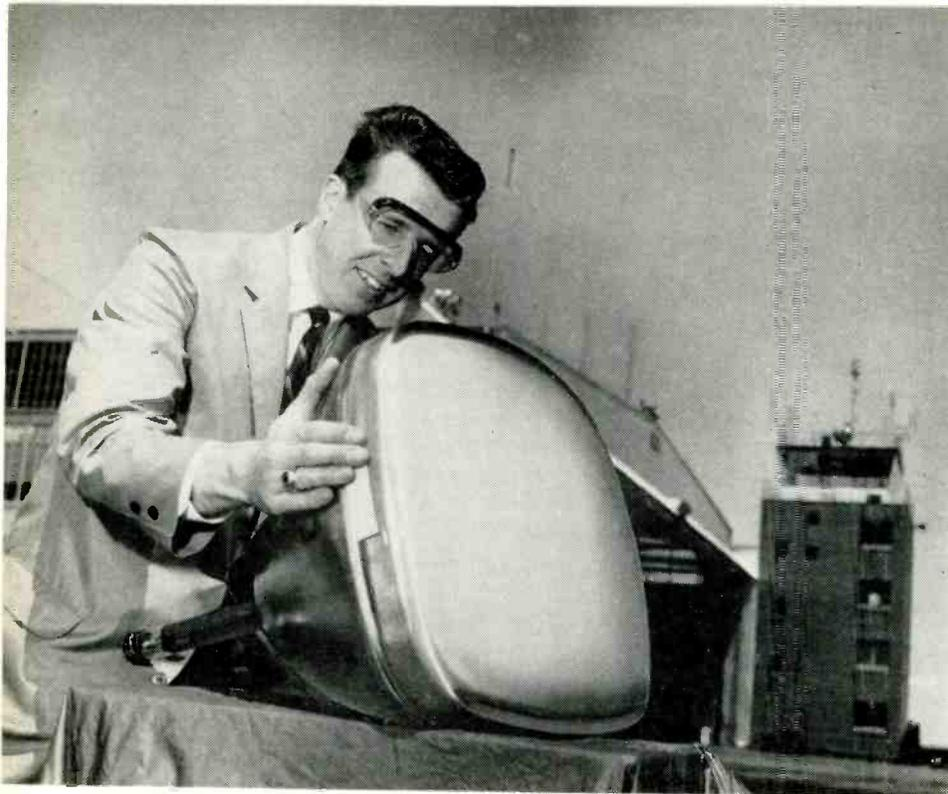
Fig. 27: A high resolution, high brightness monitor tube, made by GE, can be used with scan converters in aircraft control systems.
