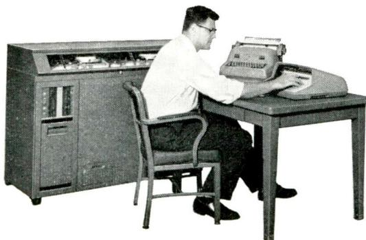
Spectrol uses an IBM 610 computer to turn out complex non-linear precision pots in record time, both single-turn and multi-turn. This in itself saves weeks of time, assures more accurate performance. Spectrol alone maintains a computer on the premises for this purpose.
