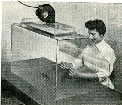
area filter. The filter removes airborne dust particles down to 0.5 micron in dia. and provides an internal "positive" pressure which prevents unfiltered room air from entering the open front. Working area measures 34 x 24 x 19 1/4 in. It is constructed of optically-clear, 1/4 in. "Plexiglas." Air-Shields Inc., Industrial Division, Hatboro, Penna.
