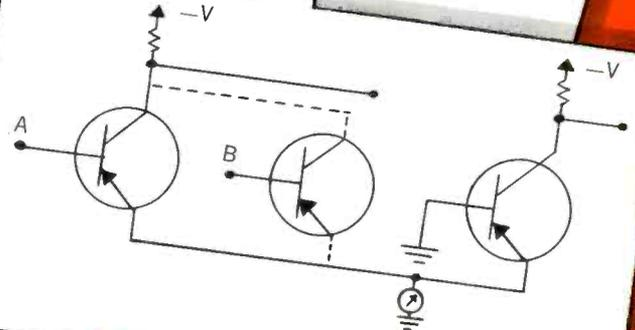
"NOR" diode-transistor gates
