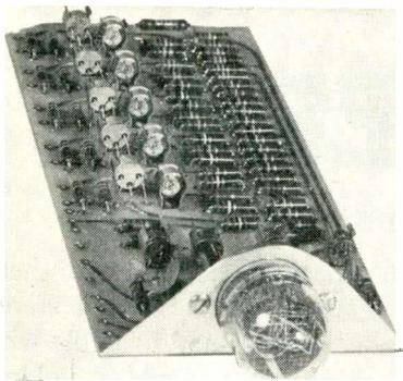
puts. Relays and tubes are eliminated. No preventive maintenance required. It activates a cold-cathode decimal display equivalent to a "Nixie" tube. Filamentary projected readout equivalent to IEE Alpha-Numeric unit available. A variety of 4 bit codes can be converted. Hermes Electronics Co., 75 Cambridge Pkwy., Cambridge 42, Mass.
