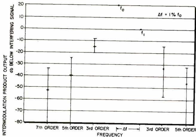
Fig. 7: Plot of normalized transmitter intermodulation
