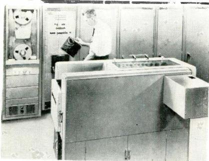
The high-speed printer-plotter system was designed by Briggs Associates, Inc. The system will be turned over to G.E.'s MSVD for use on the Atlas Missile program
