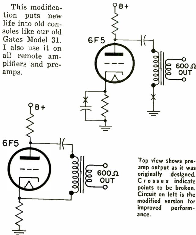
Top view shows pre-amp output as it was originally designed. Crosses indicate points to be broken. Circuit on left is the modified version for improved performance.
