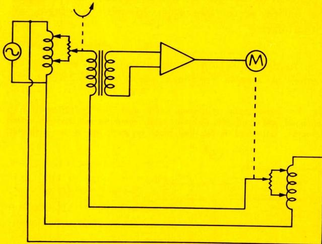
Fig. 8: Circuit performs same function as fig. 7. Two AC Potentiometers are connected in a bridge circuit. Voltage step-up may be achieved in the null transformer. This and elimination of the summing resistors reduces gain which must be provided by the amplifier.
