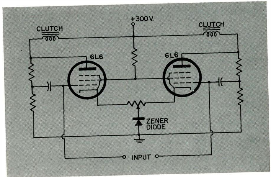
Fig. 2: Schematic shows the hysteresis clutch field coil amplifier.
