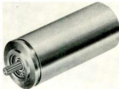
stall. Tachometer generator has 26 v RMS, 400 CPS rated input voltage and 0.26 v RMS output voltage at 1,000 RPM. John Oster Mfg. Co., Avionic Div., 1 Main St., Racine, Wis.
