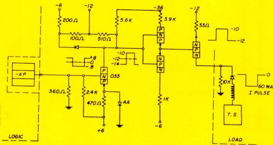
Fig. 5: Schematic diagram shows the write driver circuit with transistors
