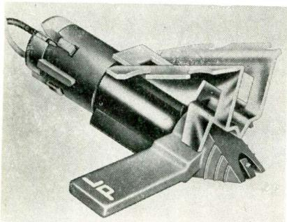
basic stereo features which assure safe mono reproduction of stereo records. Equal compliance in all directions eliminates the problem of groove breakdown. The other stereo feature is a 0.7-mil jewel tip instead of the usual 1-mil tip used in mono cartridges. Smooth from 20 to 20,000 cycles, the frequency response is flat out to 15,000 cycles with a gradual rolloff beyond. Sonotone Corp., Elmsford, N. Y.
