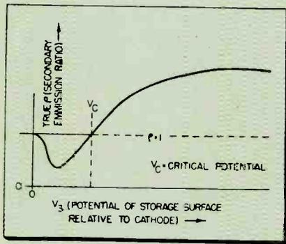
Fig. 4: Operation of storage tubes is based on the secondary-emission curve.
