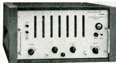
0.00003%  $\pm$  0.1 CPS. Input impedance is 1 M ohms to 10 MC, 100 ohms above 10 MC. Berkeley Div., Beckman Instruments, Inc. Booth 3416.
