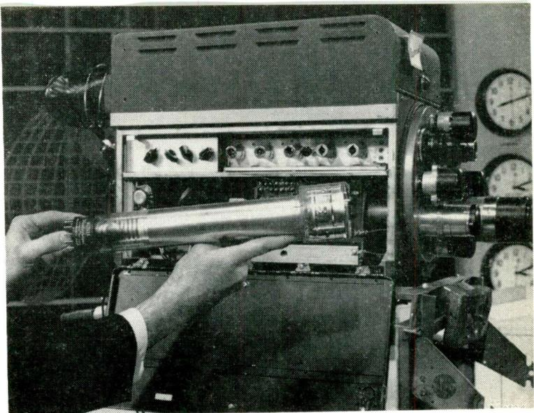
Fig. 22: A new extended-life, 1000-hour warranty, image orthicon which uses a new target material is interchangeable with the 5820.
