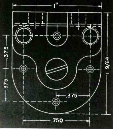
Stromberg-Carlson's type "E" relay combines the time-proven characteristics of the type "A" relay with a mounting arrangement common to many other makes.
