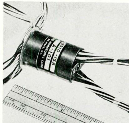
of the drive flange which is 0.750 in. in dia. Leakage resistance is more than 20,000 megohms at 500 vdc. between all circuits and between each circuit and ground. Current ratings are 0.5 a on 12 circuits and 0.25 a on the remaining 44 circuits. Torque required is 65 gram-centimeters for reliability at 25 g between 0 and 2,000 CPS. Electro-Miniatures Corp., 600 Huyler St., So. Hackensack, N. J.
