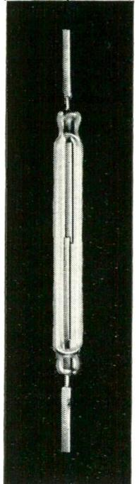
Switch capsule consists of a pair of magnetically operated contacts, hermetically sealed in an atmosphere of inert gas.
