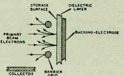
Fig. 7b: Storage surface instantaneously negative with respect to barrier grid.
