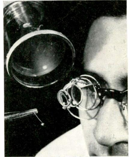
"Solid State Ionization Chamber" is smaller than the head of a pin. Developed by Hughes Aircraft Co. Labs at Los Angeles and Newport Beach, Calif., it measures the number and energy of atomic particles. It uses "doped" silicon which emits a measurable pulse when struck with a charged nuclear particle.
