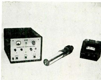
indicating range of 50 sec.  $\pm 25$  sec., and working distance to 30 ft. between sensing unit and reflecting surface. Other features: Response—20 msec; drift less than 1% in 24 hrs. Output voltage  $\pm 15$  v. (full scale range). Sensitivity selection has a 3-position switch with ranges of  $\pm 1$ , 10 and 25 sec. Electronic damping with 2-sec. time constant provided. Keuffel & Esser Co., 3rd and Adams Sts., Hoboken, N. J.
