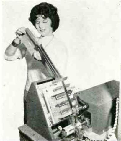
$\pm 0.1\%$ ; 2 megohms to 10 megohms,  $\pm 0.2\%$ ; 10 megohms to 100 megohms,  $\pm 0.3\%$ . A built-in 7-dial resistance decade is provided for setting to nominal values of resistance. Tolerance limits are set by plug-in units. Resettable electro mechanical counters tally the pieces in each bin. Industrial Instruments Automation Corp., 89 Commerce Rd., Cedar Grove, N. J.
