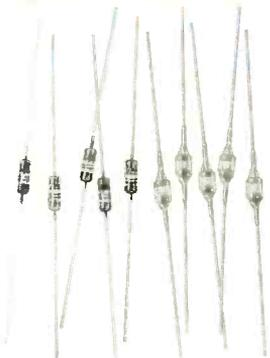
feature low cost, low capacitance, and exceptionally fast recovery time. Available in all-glass "min" package with power dissipation capabilities to 80mW. Available in solder-seal package for wire-in or clip-in use with power dissipation capabilities to 225mW.
