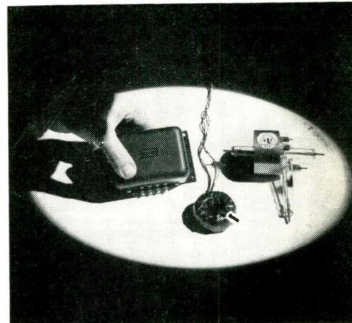
This illustration shows packaged solid-state current sensor, toroidal transformer which monitors input current and high vacuum relay for rapid disconnect.
