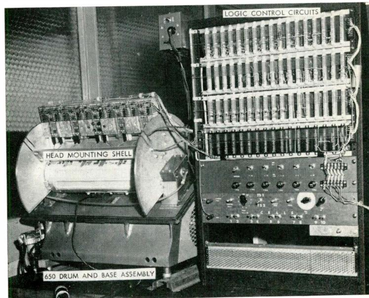
Fig. 4: Photograph of one megabit drum memory prototype
