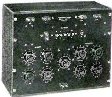
Accurate inductance measurement with or without superimposed D.C., for all types of iron core components
