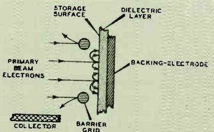
Fig. 7a: Storage surface instantaneously positive with respect to barrier grid.
