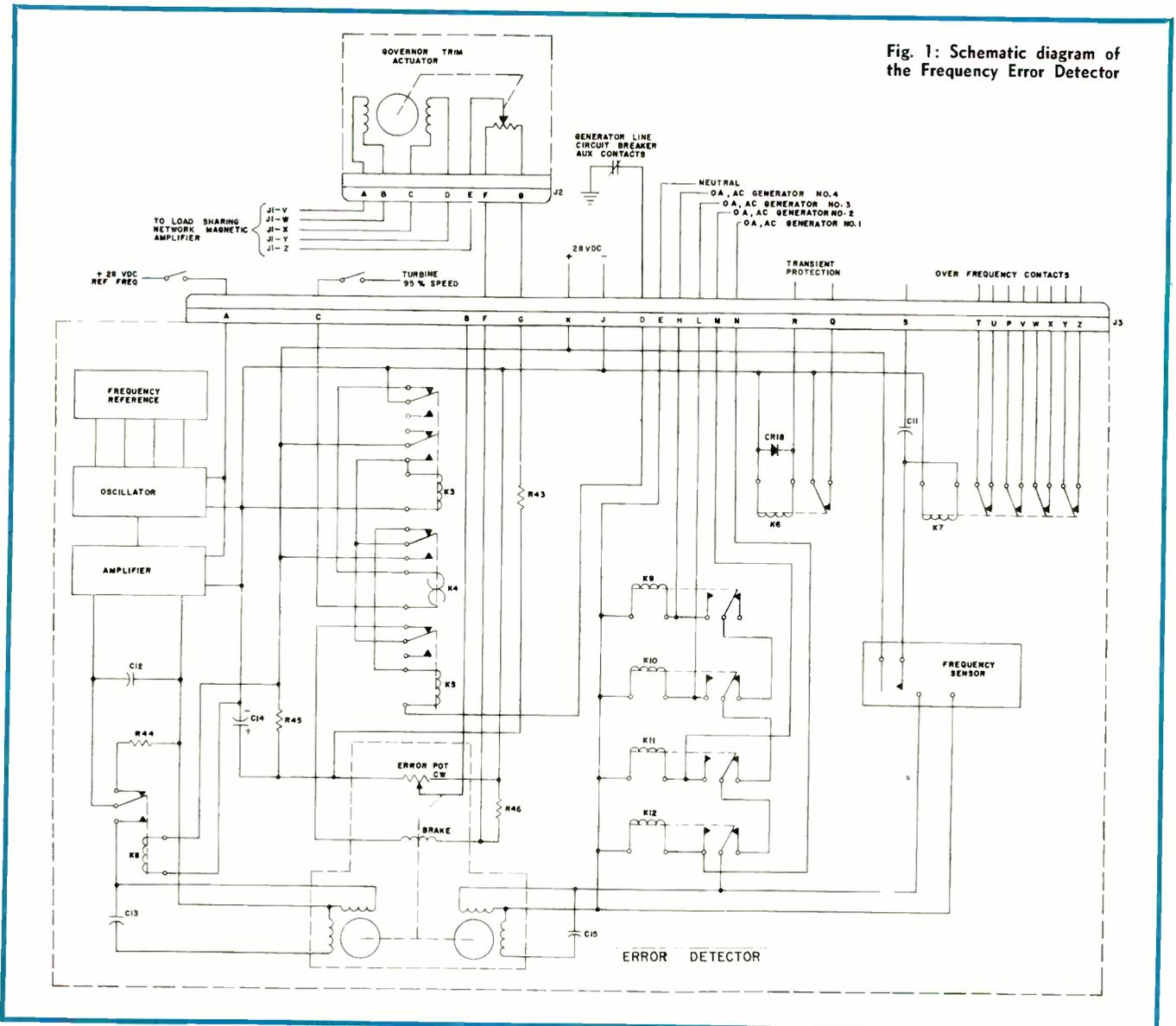
Fig. 1: Schematic diagram of the Frequency Error Detector
