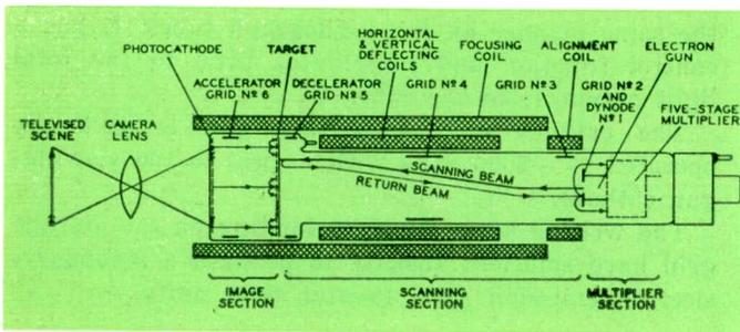
Fig. 18 (left): Arrangement of elements in a typical image orthicon.
