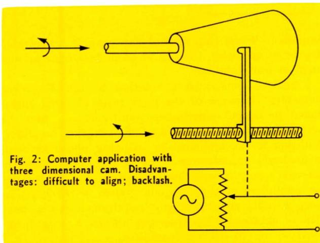
Fig. 2: Computer application with three dimensional cam. Disadvantages: difficult to align; backlash.
