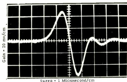
Fig. 3: Oscillogram of readback single bit
