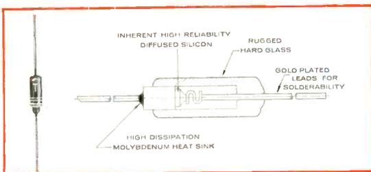
Design NOW with industry's *fastest* high-voltage computer diodes and benefit from the speed of 4-millimicrosecond switching\* and the design safety provided by 75-v PIV.
