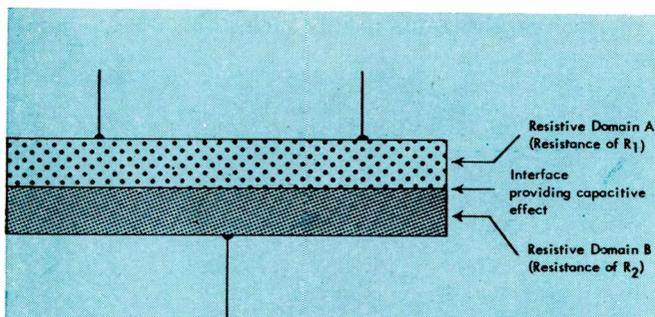
Fig. 6: Function block of two resistive domains and one capacitive interface, whose total effect is that of an RC or time-delay circuit.
