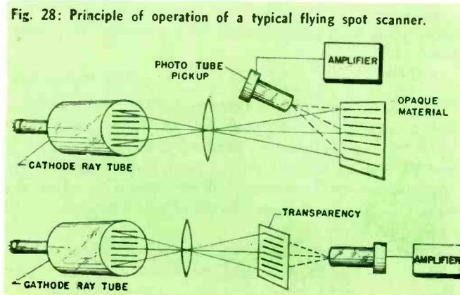
Fig. 28: Principle of operation of a typical flying spot scanner.
