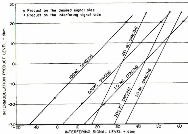
Fig. 8: Typical h-f transmitter intermodulation curves—third order product on the interfering signal side.
