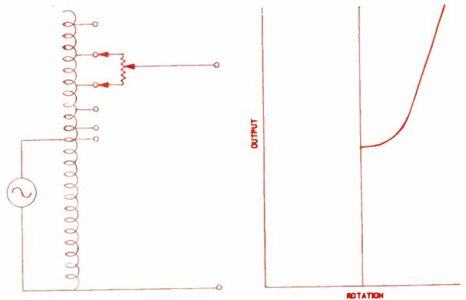
Fig. 6: The voltage step-up feature is used to generate the secant function. The taps are located in the unexcited portion of the transformer so the output voltage ratio will always be greater than one.
