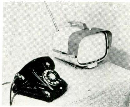
The Sony Corp. of Japan has completed a production model of a TV set which is all transistorized. Set has 8-inch crt and operates on batteries or ac power
