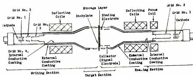
Fig. 9: Arrangement of elements in the RCA scan converter tube.
