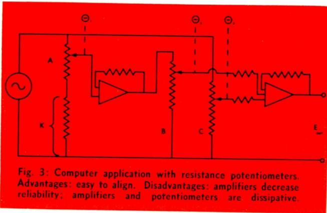
Fig. 3: Computer application with resistance potentiometers. Advantages: easy to align. Disadvantages: amplifiers decrease reliability; amplifiers and potentiometers are dissipative.
