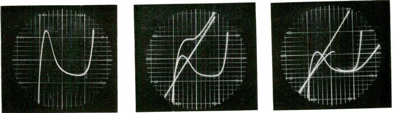
Tracings of the tunnel diode characteristic curve and also its dynamic characteristics. Views are similar to Figs. 1, 6, & 7.
