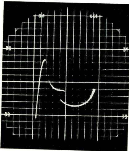
Fig. 4: Self oscillation with 10 uuf across the diode.
