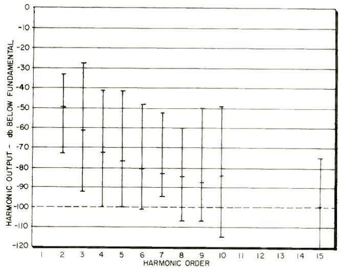
Fig. 4: Normalized harmonic emissions. Line length represents range of values and mark near line center is the mean value.
