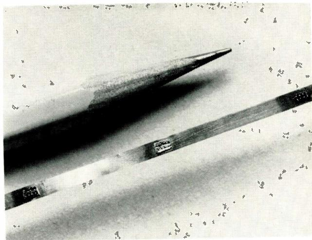
Fig. 8: Ribbon bearing multiple junction systems on germanium crystal produced by dendrite process. Three systems are shown on ribbon.
