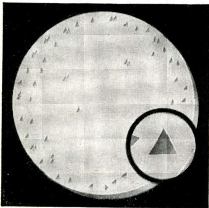
Dislocation density, Knapic silicon monocrystals: Crystal diameters to 3/8"—None; 3/8" to 3/4"—less than 10 per sq. cm.; 3/4" to 1 1/4"—less than 100 per sq. cm.; 1 1/2" to 2"—less than 1000 per sq. cm.
