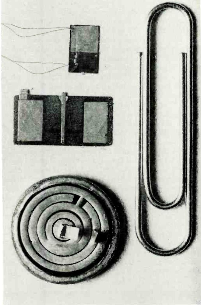
Fig. 2: Three function blocks representing subsystems: (top) a two-stage video amplifier; (center) a free running multivibrator; and, (bottom) the device with the concentric arcs, an audio amplifier.
