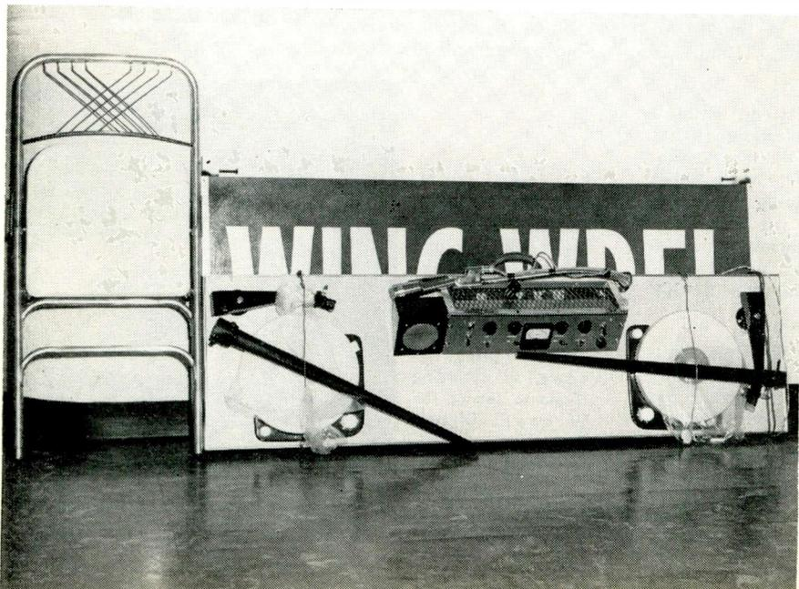
Simple high impedance mixing is used in the consolette, with a flat preamplifier being used for the microphone input, and equalized preamps being used for the GE variable reluctance pickup inputs. The circuit used in the latter is similar to the one recommended by the manufacturer.
