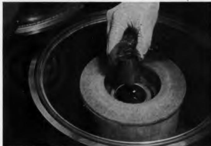
*Pre-packaged* single piece crucible charges . . . in sizes and weights to meet the exact requirements of your Czochralski crystal growing equipment . . . are now available from Dow Corning.
