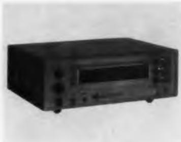
The Model 728B measures and displays freqs. directly without heterodyning techniques from dc to 100 MC, measures time intervals and periods to  $10^{-4}$  sec. and counts at rates to 100 MC with self-contained time base. The universal counter-timer consists of 3 input channels, a special decade count-down time base which eliminates the need for divider adjustment, and a series of plug-in transistorized decade counting units. Computer Measurements Co., 12970 Bradley Ave., Sylmar, Calif.
