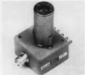
These packaged units, called the SO series produce a signal whose freq. is controlled by applying either a current or voltage, eliminating manual tuning requirements. In a typical vacuum-tube, single-band unit, a change in freq. of 5 to 1 is produced by applying a control current between 0 and 70 ma over the 10 KC to 200 MC range. Units require an extended power source of 150 v. at 30 ma and 6.3 vac at 0.4 a. Increductor Magnetics Dept., Trak Electronics Co., Inc., Wilton, Conn.
