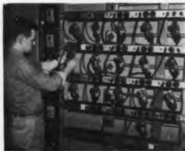
Technician at Automatic Electric Company's plant in Northlake, Ill. sets up rotary stepping switch for "wear-in" period before final adjustment. Each switch is run for at least 100,000 steps.
