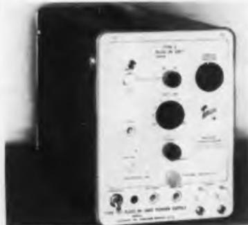
Electronically-regulated power supply provides an easily-portable housing for any Tektronix A-to-Z plug-in unit, enabling the plug-ins to be used with or without an oscilloscope. Internal amplifier of the Type 132 has a freq. response of dc to 22 MC, rise-time of 15 nsec., noise level less than 0.5 mv, peak-to-peak (referred to internal amplifier input). Front-panel terminals permit push-pull or single-ended + or - input. Tektronix, Inc., P. O. Box 500, Beaverton, Ore.
