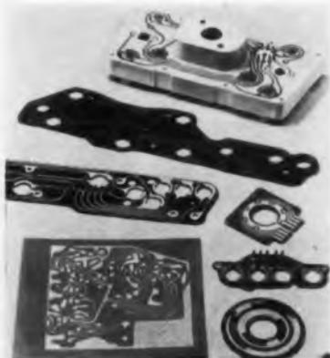
Various sizes and shapes of die stamped circuits are illustrated. Produced by a dry process, there is no excess metal to remove by chemical etching.
