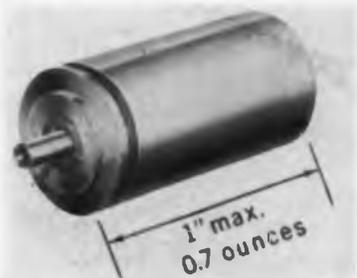
Type 5351-01 is only 1 in. long, weighs 0.7 oz., has 0.12 oz. in. torque at stall and 47,000 rad./sec. torque to inertia ratio. The unit can operate continuously at  $-55^{\circ}\text{C}$  to  $+125^{\circ}\text{C}$  temp. range. No load speed is 9,500 RPM min. Rated voltage at 400 cps is 26 v. (can be available in 18 v. or 33 v.). Effective resistance at stall 400 $\Omega$ . Corrosion resistant materials are used throughout. John Oster Mfg. Co., Avionic Div., Racine, Wis.
