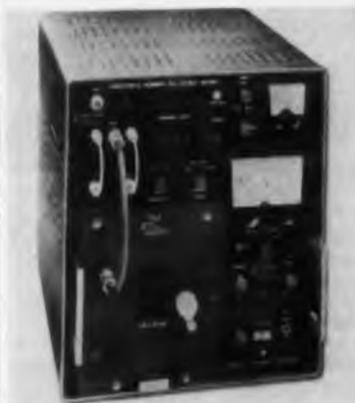
Entire complement of equipment consists of a basic unit, 4 interchangeable r-f tuning units, an impulse calibrator, 5 antennas, and a tripod. Model CFI is designed to perform the tests prescribed by the latest mil. specs covering r-f leakage and interference in electronic and associated equipment. The instrument has single-knob Unidal® tuning; 3 impulse bandwidths; 1 mc, 5 mc, and 8 mc; and an accurate, direct-reading freq. dial. Polarad Electronics Corp., 43-20 34th St., Long Island City, N. Y.
