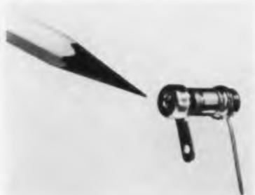
Mini-Trimmer® model, equipped with 1 wire lead and 1 tab lead, made in 4 models with capacitance ranges as broad as 1 to 18 pf. Featuring fixed cavity tuning and a linear tuning curve, the new type makes possible sturdy, 2 terminal mounting for printed circuit boards or for custom applications. Combination of glass and hardware provides low inductance at high freqs., thermal stability and ruggedness. Electronic Components Div., Corning Glass Works, Corning, N. Y.
