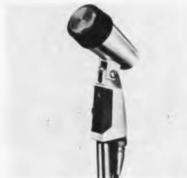
This allows the user to tailor the microphone to the application. Model 540S, has a high output dynamic element, a freq. response of 60-10,000 CPS dual impedance and an on-off switch. Unit suitable for "difficult" public address installations and home recording activities. Unit is said to be the only microphone of its kind with the capability for adjustment of both high and low end freq. response independently or together. Shure Bros., Inc., 222 Hartrey Ave. Evanston, Ill.
