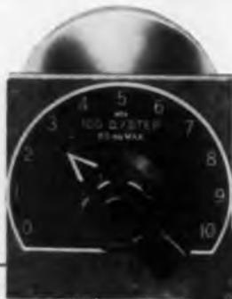
Accuracy of  $\pm 0.05\%$  for most units, except 10 $\Omega$  (total) decade which is  $\pm 0.15\%$ ; 1 $\Omega$  decade  $\pm 0.5\%$ ; and 0.1 $\Omega$  decade  $\pm 2\%$ . Supplied with aluminum shield can, knob, dial plate.
