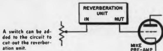
A switch can be added to the circuit to cut-out the reverberation unit.
