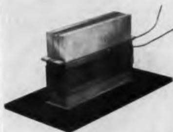
Omnimite®, a magnetostrictive transducer, metallically bonded to a ¼ in. thick 316-L stainless steel diaphragm is used in this new series of sonic cleaners. Every Bendix Omnimite transducer diaphragm assembly is guaranteed unconditionally not to break, crack, depolarize, deteriorate, become detached or in any way cease to function for the lifetime of the cleaning unit. The Bendix Corp., Pioneer-Central Div., Sonic Energy Products, Davenport, Iowa.
