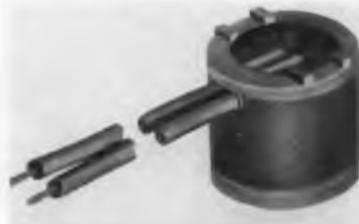
Known as Type GP Stevens Commercial Thermostats, they are enclosed in a polypropylene boot filled with epoxy resin. The bimetal disc thermal element in close proximity to aluminum or tin-plated brass sensor cap providing rapid response to temp. changes. Rated for 100 KC up to a max. operating temp. of 176°F. Uses include pilot duty and temp. protection in refrigerators, freezers, liquid coolers and industrial apparatus. Stevens Mfg. Co., Inc., P. O. Box 1007, Mansfield, Ohio.
