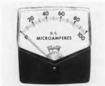
Four sizes offered in transparent and black molded plastic: 220-M, scale length 2.5 in.; 320-M, scale length 3.34 in.; 420-M, scale length 4.5 in.; and 820-M, scale length 7 in. "M" Series have 3-way terminals permitting use of time-saving push-on solderless connectors; or conventional solder terminals; or conventional wrap-around (binding head screws). Have Triplett-Bar-Ring® self-shielded movements with Alnico magnets. Triplett Electrical Instrument Co., Bluffton, Ohio.
