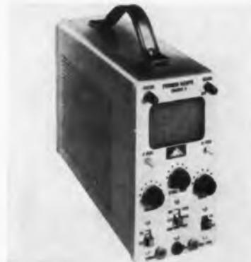
The Primer-Scope®, Mark I, is small and versatile, in the low price range. Weighing under 6 lbs., favors its inclusion in heavy service kits. Its size is 7¼ x 3½ x 11¼ in. The main scope component is a special 3 in. Rayonic® CRT, incorporating an integral magnetic shield to prevent stray or spurious pickups. Accelerating potential is approx. 840 v. Trace is bright and sharp. An instruction manual is included. Waterman Products Co., 2445 Emerald St., Phila., 25, Pa.
