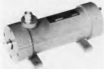
Another standard model CW oscillator utilizing the GL-7391 tube covers from 5400 to 5900 MC. Standard oscillators feature a single freq. tuning control and power output adjustment normally preset to provide the min. power over entire freq. range. Operate from a 200 v. plate power supply and can draw up to the max. current specified by the electron tube manufacturer. Designed to provide max. performance under extreme environmental conditions. Waveline Inc., Caldwell, N. J.
