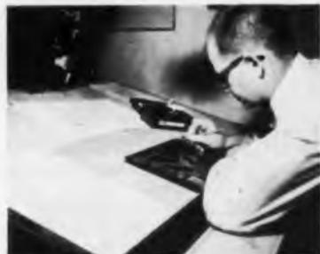
Fig. 3. Master is corrected using specially prepared touch-up fluid.
