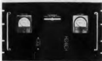
LA Series models have line regulation better than 0.05% or 8 mv, whichever is greater, for input variations from 100-130 vac. Load regulation is better than 0.10% or 15 mv, whichever is greater, for load variations from zero to full load. Swing-open backs permit easy servicing in rack, all major component terminals are accessible from the rear. Rated for continuous operation at 50°C ambient, Lambda Electronics Corp., 515 Broad Hollow Rd., Huntington, L. I., N. Y.
