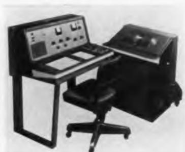
The Analytical NMR Spectrometer System is sensitive to the hydrogen nucleus at an operating freq. of 60 MC and a magnetic field strength of 14,092 gauss. Typical volume of a liquid sample is 0.2 to 0.4 cc. (cylindrical). Instrument can resolve 2 lines separated by 1 part in  $10^4$  and has sensitivity sufficient for a wide range of analytical problems. Power is 208-230 v., 1 $\phi$ , at 50 or 60 cps (as specified). Instrument Div., Varian Associates, 611 Hansen Way, Palo Alto, Calif.
