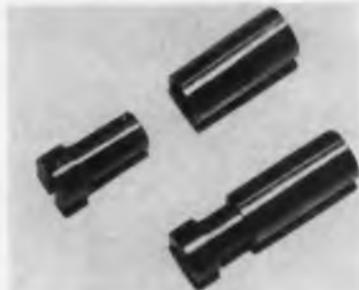
Machined from #303 stainless steel, with clear passivate finish, the 2-piece adapters provide a 0.2497 (+0.000 -0.002) standard shaft on tapered shaft motors, such as Diehl FPE-25 and FPE-49, and Bureau of Ordnance type rotating components, such as synchros, resolvers and tachometer generators. PIC Design Corp., 477 Atlantic Ave., E. Rockaway, L. I., N. Y. Circle 235 on Inquiry Card
