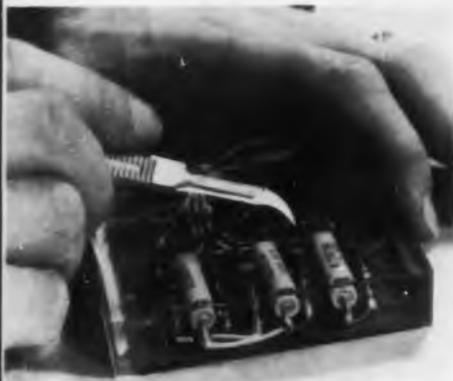
Fig. 3a: All components in circuits encapsulated with the resin illustrated in Fig. 2 are clearly visible. The resin can be cut away from around the defective part with a knife.
