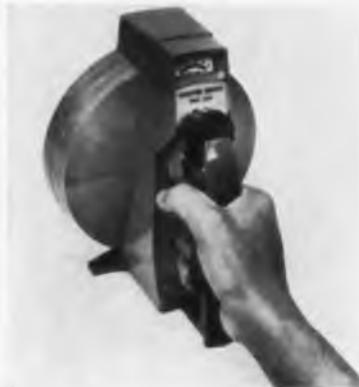
Designed for hand-carrying or to stand and operate unsupported, it has a strong plastic housing, one knob operation without freq. range switching. Model B86B1 operates over a freq. range from 400 MC to 10 GC has a single integral antenna and utilizes standard, large-capacity mercury batteries. Providing a rapid and simplified means for monitoring power density over its wide band, the instrument responds to all planes of polarization. Sperry Microwave Electronics Co., Clearwater, Fla.
