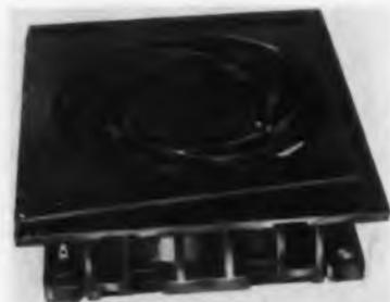
It measures the same as the former Muffin basic configuration providing interchangeable mounting. Output capacity is 100 cfm at free delivery. It operates on 115 v., 60 CPS, 1  $\phi$ . Available as a skeleton, venturi, or grided fan. Incorporated new rigid leads between motor and redesigned terminals, both fabricated as integral parts of the housing eliminate internal electrical breakdown. New bearing design results in smooth, quiet, long life. Rotron Mfg. Co., Inc., Woodstock, N. Y.
