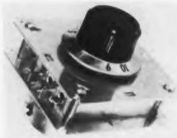
Designed for industrial applications, Series 41500 adjustable interval timer has a precision snap-action SPDT switch. Designed to operate either as a time delay mechanism or as a straight interval timer. Models are available with 1 to 4 switches in the same package size, rated life in the standard version is 40,000 CPS at 15 a., 115 v. 60 CPS. It measures 3 in. sq. x 1 57/64 in. deep; timer has shaft extension of 1/4 in. dia x 3/8 in. long. The A. W. Haydon Co., Waterbury, Conn.
