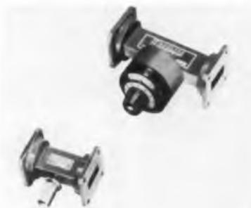
Shielding is provided for interference free operation at low r-f levels even in areas of exterior high level fields. The standard calibrated units provide an attenuation range of 30 db. with calibrations provided at 5 db. points at a single freq. (Model 611 covers 8.20 to 12.4 GC; Model 711 covers 12.4 to 18.0 GC). The standard variable pad attenuator provides an attenuation range of 20 db. (Model 613 covers 8.20 to 12.4 GC). Waveline Inc., Caldwell, N. J.
