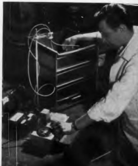
Working in a typical laboratory set-up designed for the preparation of thin magnetic films by electro-deposition, this technician is attaching a lead to the cathode in the plating solution. (Experimental rig at Remington Rand Laboratories.)
