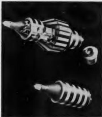
Artist's drawing shows expandable structures in space proposed by Aeronutronic Div. of Ford Motor Co., Newport Beach, Calif. Structure in orbit at top has been expanded to provide laboratory area for space experimentation. Boost configuration at right prepares to rendezvous. Configuration at bottom is going into orbit.
