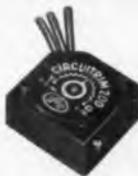
Set it and forget it is the paramount feature of IRC's new square trimmer, made possible by an exclusive self-locking, antibacklash spiroid drive gear. Square Circuitrim has superior moisture, shock and vibration characteristics, and is interchangeable with earlier designs. Teflon leads and seals standard. Printed circuit terminals available. 10 ohms to 50K ohms, 1 watt. Write for technical bulletins. International Resistance Company, 401 N. Broad St., Philadelphia 8, Pa.
