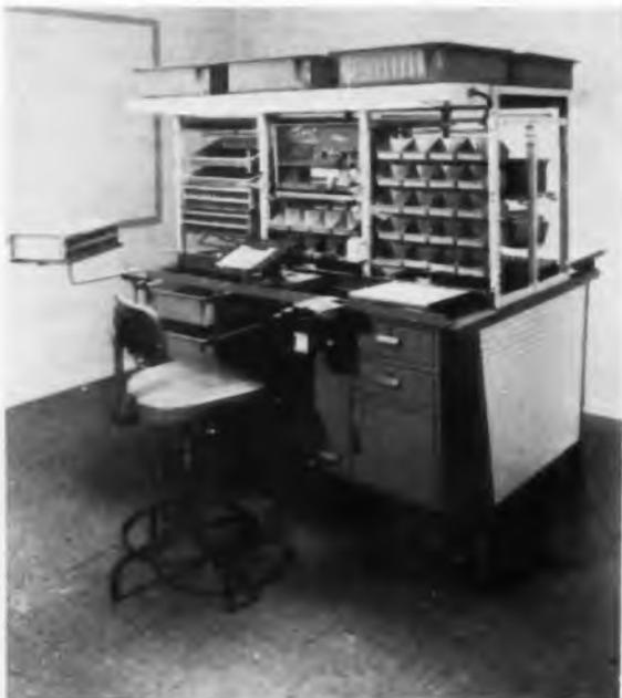
Fig. 1: Dual back to back Hughes Production Station. Also available as a single side station, separate super structure or separate work bench. A wide choice of module boxes, trays, racks, etc., is offered.
