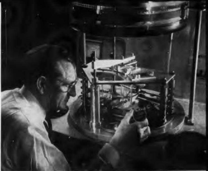
ing a device that is only a few ten-thousandths of an inch thick. In the evaporation process, the cadmium sulfide crystals and the metal are heated in successive steps in a vacuum. The vapor is collected by condensation on the glass plate in the same manner as steam condenses in a film on a cooler surface.
