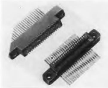
40 contacts with a 0.050 in. center-to-center spacing are mounted in a 1 11/16 in. long molding. Contacts are reliable, patented "bellowform" type, providing coil spring action grip. Recommended test voltage at sea level is 900 RMS. current rating 1 a. Illustrated are wire terminals in 2 positions: straight; and with right angle bend. Body material is glass reinforced Diallyl Phthalate per Mil-M-19833, Type GDI-30 specs. Continental Connector Corp., Woodside 77, N. Y.
