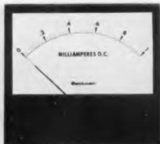
They are gasket sealed to keep out dirt and moisture, and steel enclosures protect the movements from effects of magnetic fields and stray r-f. These front mounting panel meters, (approx. 4.1 x 4.7 in.) use glass windows to eliminate errors due to static charges. Scale length is 3.97 in., standard accuracies are 2%. Among 95 standard models available are ammeters, milliammeters and microammeters. Helipot Div., Beckman Instruments, Inc., 2500 Fullerton Rd., Fullerton, Calif.
