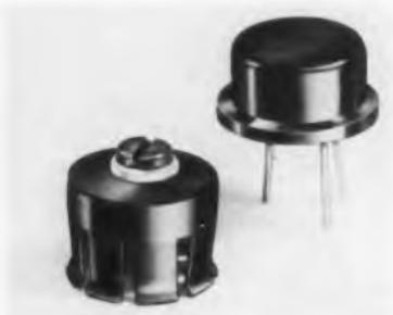
TXBP-018-028 is made entirely of beryllium copper with spring finger construction. Will fit case dia. from 0.175 to 0.190 in. Mount by pushing onto transistor and will not damage case. Suitable for printed circuit boards, chassis and heat sinks. Available in insulube or black cadmium finish. TO-18 Transistor Heat-Dissipating Retainers mount to chassis by screw-attachment. IERC Div., International Electronic Research Corp., 135 W. Magnolia Blvd., Burbank, Calif.
