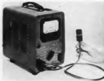
Each unit is individually calibrated in a known field, RMS voltage output is noted as a function of gauss level and is legibly printed on connector shield. Probe consists of an air core inductor, epoxy cast, within an electrostatic shield enclosure. Terminals from inductor are brought out in a pair of electrostatically shielded cables, the other end terminated with standard  $\frac{3}{4}$  in. center banana plugs. Magnetic Shield Div., Perfection Mica Co., 1322 No. Elston Ave., Chicago, Ill.
