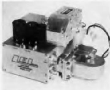
Model RA-1b has a single Klystron serving the dual function of up-converter pump and down-converter local oscillator, thus cancelling freq. drift. The standard model is designed for 225-260 MC operation, but may be modified for operation up to 1 GC. Its small size and light weight make airborne and missile applications practical. Specs: Gain, 25 db.; Passband, 225-260 MC; Noise figure, 1.0 to 2.0 db.; Weight, 6 lbs. LEL, Inc., 75 Akron St., Copiague, N. Y.
