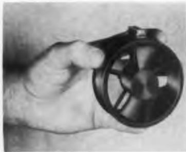
The new 60 CPS Propimax 2 measures slightly over 3 in. in dia., 1 1/2 in. deep and weighs 6 1/2 oz. It moves 17.5 CFM under free delivery conditions. Materials and finishes meet most applicable military specs. Power required is 0.05 a. at 115 v., under free delivery conditions. Mounting is by means of servo-ring. Impeller runs on 2 precision, double-shielded, stainless steel ball bearings. RPM at free delivery is 3250. Rotron Mfg. Co., Inc., Woodstock, N. Y.
