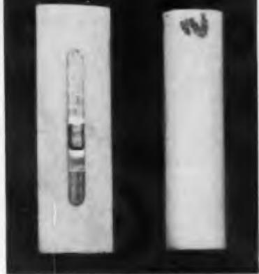
Fig. 1: Brass-plated rod successfully encapsulated in Teflon without void or air space between pin and the TFE resin.
