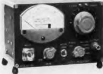
Tuned amplifier and null detector, Type 1232-A, measures 8 x 6 x 7 1/4 in. In addition to its main use as a bridge detector, it has applications as a preamplifier and an audio spectrum analyzer. Completely transistorized and battery-operated, the unit is housed in a G-R rack bench cabinet. Filter freq. range from flat to 100 KC. Controls include linear/log meter switch. General Radio Co., West Concord, Mass.
