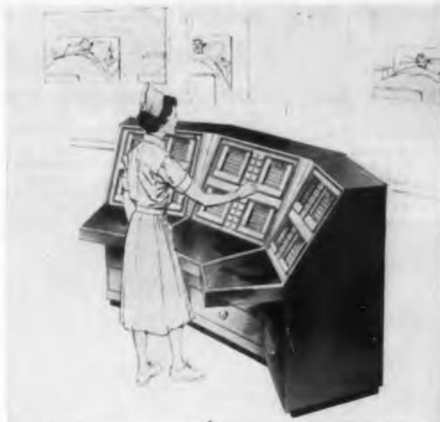
Fig. 1: A single nurse can monitor the condition of a dozen intensive-care hospital patients with this Minneapolis-Honeywell electronic medical system. Mounted on the nurse's central station console is a recorder-alarm unit for each of the 12 patients.
