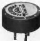
The new IRC  $\frac{1}{2}$ " round Circuitrim trimmer with its unique mechanical design (depicted above) simplifies the complex mechanical linkage used for adjustment in most trimmers making it more reliable and less costly. This round trimmer design employs the same fine electrical assembly found in IRC's popular square trimmer. Available in twelve standard ranges from 10 ohms to 50K ohms, 1 watt. Higher power rating available.
