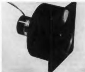
Power requirements: 1  $\phi$ , 117 v., 60 cps source. Blower is enclosed in a precision cast aluminum housing for max ruggedness. Continuous operation life is rated in excess of 2500 hrs.; unit is designed to meet appropriate MIL specs. Mounting flange dimensions are 3.44 in. sq.; bolt holes spaced 2.75 in. apart. Overall length is 3.25 in. Weight: 12 oz. Globe Industries, Inc., 1784 Stanley Ave., Dayton 4, Ohio.
