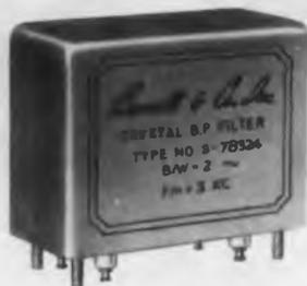
Specs include: Insertion loss, 3.5 db; Attenuation, 3 db bandwidth, 2 cps; Shape factor, 30/3, 5:1; Temp. coefficient, 0.021 cps/°C; Input impedance, 500 KΩ; Output impedance, 500 KΩ. The low freq. crystal filter meets Mil-C-3908B for vibration standards as well as applicable portions of Mil-T-27A. Other crystal filters available from 1 kc to 30 mc in a wide range of impedances. Burnell & Co., 10 Pelham Pkwy., Pelham, N. Y.
