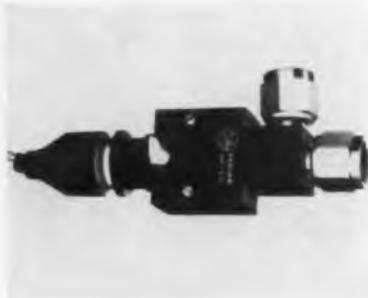
The VA-511 produces 50 w. min. power at 10.0 GC and operates at 10 kv, 60 ma. This fixed-freq., 2-cavity oscillator has an FM noise figure less than 1 CPS, and is electrostatically-focused. Weighs less than 24 oz., measures 6¼ x 2¼ x 1¼ in. Varian Assoc., Tube Div., 611 Hansen Way, Palo Alto, Calif.
