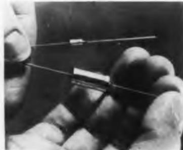
Ratings range from 0.033 to 330 $\mu$ f and from 6 to 35 wdc. They are polar capacitors for use with a dc bias exceeding the peak value of the ac component. Operating temp. from -55°C to +125°C. Leakage currents are below Mil spec. limits. For use in airborne computer, guidance-control, and data-processing systems. Standardized into 4 miniaturized case sizes from 0.250 to 0.750 in. and in dia. from 0.125 to 0.341. Fansteel Metallurgical Corp., Rectifier-Capacitor Div., N. Chicago, Ill.
