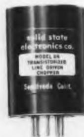
Model 64 Plug-in Line Driven Chopper (or modulator), has a transformer-coupled isolating drive network and clipping diodes so that it can be driven from a 400 CPS sine wave power line or from a drive source common to the dc voltage being chopped. Sinusoidal or square wave drive may be used over a freq. range 70 CPS to 10 KC sine wave, or 40 CPS to 12 KC square wave. Operating temp. -55°C to +90°C. Solid State Electronics Co., 15321 Rayen St., Sealpueda, Calif.
