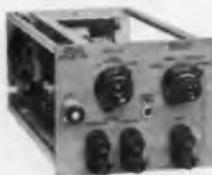
⊕ **166C Display Scanner (Time-Axis plug-in)** provides output to duplicate, on an X-Y recorder, any repetitive waveform appearing on CRT trace. Resolution with permanent, large-scale records is higher than either scope CRT or photograph, and you can observe the scope trace while records are made. Unit converts high speed signals to slower signals having the same waveshape; scanning speed is arranged to keep Y output within the bandwidth of conventional recorders. ⊕ 166C, \$300.00.
