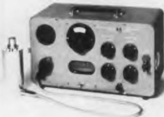
Model 393 is a transfer device by means of which an unknown ac voltage may be measured with high accuracy in terms of a dc voltage. Its primary uses will be in standards laboratories for calibration of r-f signal sources, r-f voltmeters, and the freq. response of amplifiers or other devices. Accuracy of transfer 0.1% 25 CPS to 10 MC, and 0.5% 10 MC to 30 MC. Ballantine Laboratories, Inc., Boonton, N. J.
