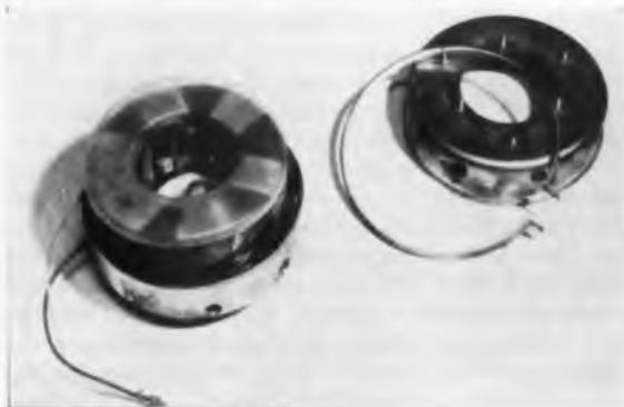
The purpose, of this endcap, is to provide insulation between the random wound coil and the coil housing, which serves as a magnetic circuit for the magnetron. To obtain the best size and cost for the electromagnet assembly, Class "B" insulation is required.
