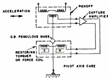
**Inertial Accelerometers.** A typical force balance pendulous accelerometer utilizing a differential transformer pickoff, a high gain capture amplifier, and a DC permanent magnet force coil is illustrated. This type of accelerometer, together with its amplifier, is a high-gain null-seeking servo in which the current flowing through the force balance coil, measured as voltage across a resistor in series with the coil, is directly proportional to the acceleration applied.
