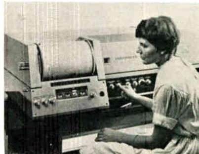
Infrared grating spectrophotometer scans complete wavelength range from 1 to 25 microns and permits continuous recording of spectra without change of components. Model 125 instrument was developed by Perkin-Elmer Corporation's West German affiliate, Bodenseewerk Perkin-Elmer & Co. G.m.b.H.
