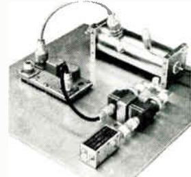
**TYPE 2971 RF ASSEMBLY** — Transmitter receiver system, nominal operation frequency 1.6 KMc. Solid-state duplexer, balanced mixer, in strip-line design insures maximum reliability and small size. Typical system characteristics: 5 KW min. peak transmitter output at a duty cycle of .0033 max., receiver tangential sensitivity of -96 DBM min. (assuming 290°K antenna temp. and a 1.5 DB IF NF); system wgt. 3 lbs. max.; component vol. 100 cubic in. max.
