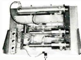
**TYPE 2974 HARMONIC GENERATOR** — Greater than 30 watts CW output at 942 Mc. 1 watt CW input at 137 Mc. Consists of 2974X3 tripler, 2974X2 doubler and two 2974A amplifiers. Component vol. less than 900 cubic in.
