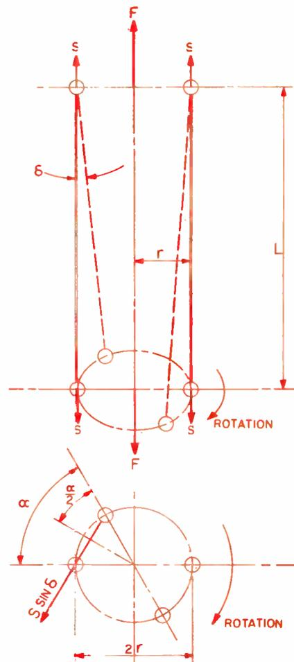
Fig. 2: The arrangement of the 2 suspension wires on one end of coil and their tensioning forces are shown.
