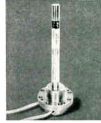
**Vertical Sensing Element.** A frictionless, wire-suspended pendulum acts as the moving portion of two orthogonally mounted differential transformers to provide phase-sensitive ac output signals proportional to the tilt angle. A typical application is initial alignment of a gyro platform. The unit has exceptional repeatability to vertical, high sensitivity, and low null voltage.
