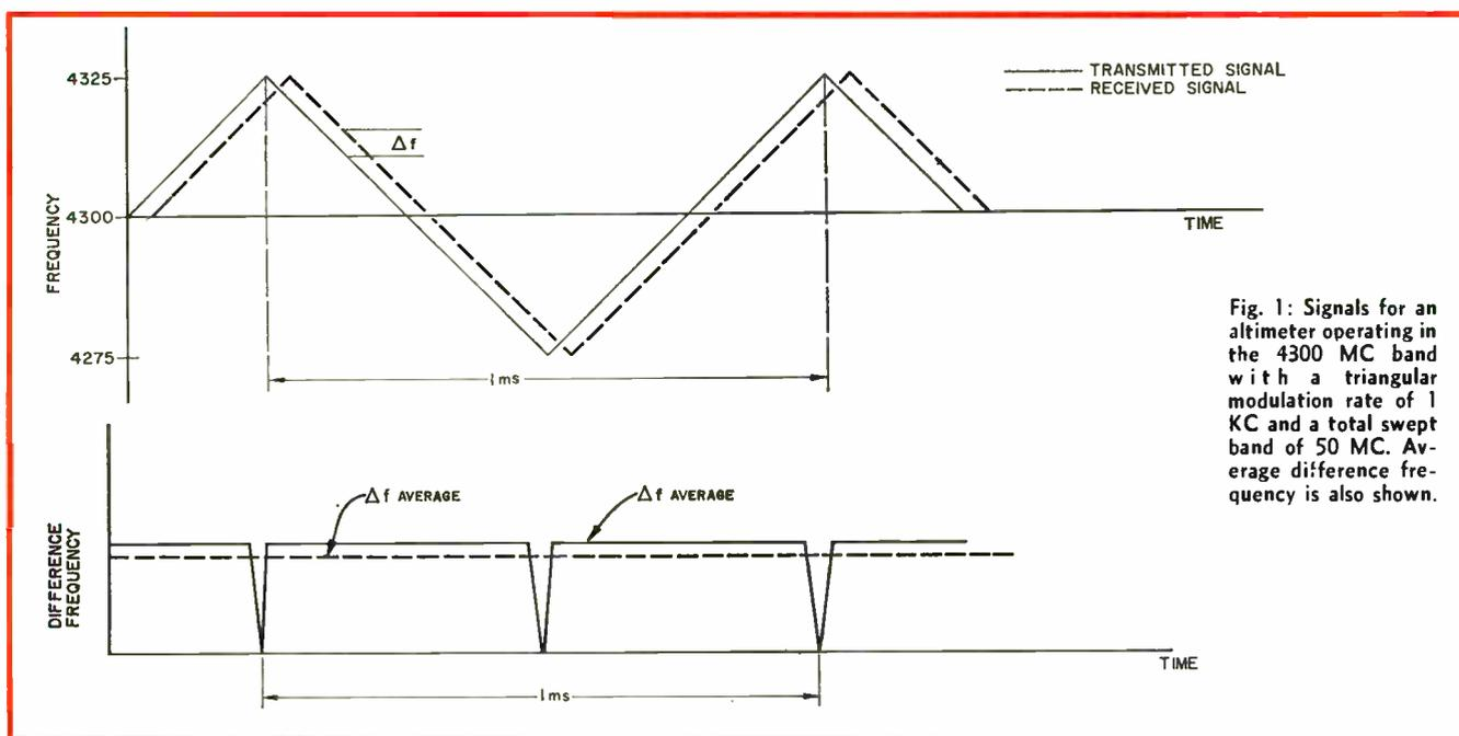
Fig. 1: Signals for an altimeter operating in the 4300 MC band with a triangular modulation rate of 1 KC and a total swept band of 50 MC. Average difference frequency is also shown.
