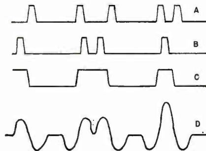
Fig. 21: The non-return-to-zero (NRZ) modes of operation. (C) is input to the line.
