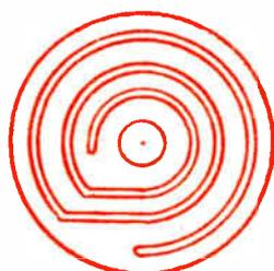
Fig. 3: Disc springs supply constant tension force.
