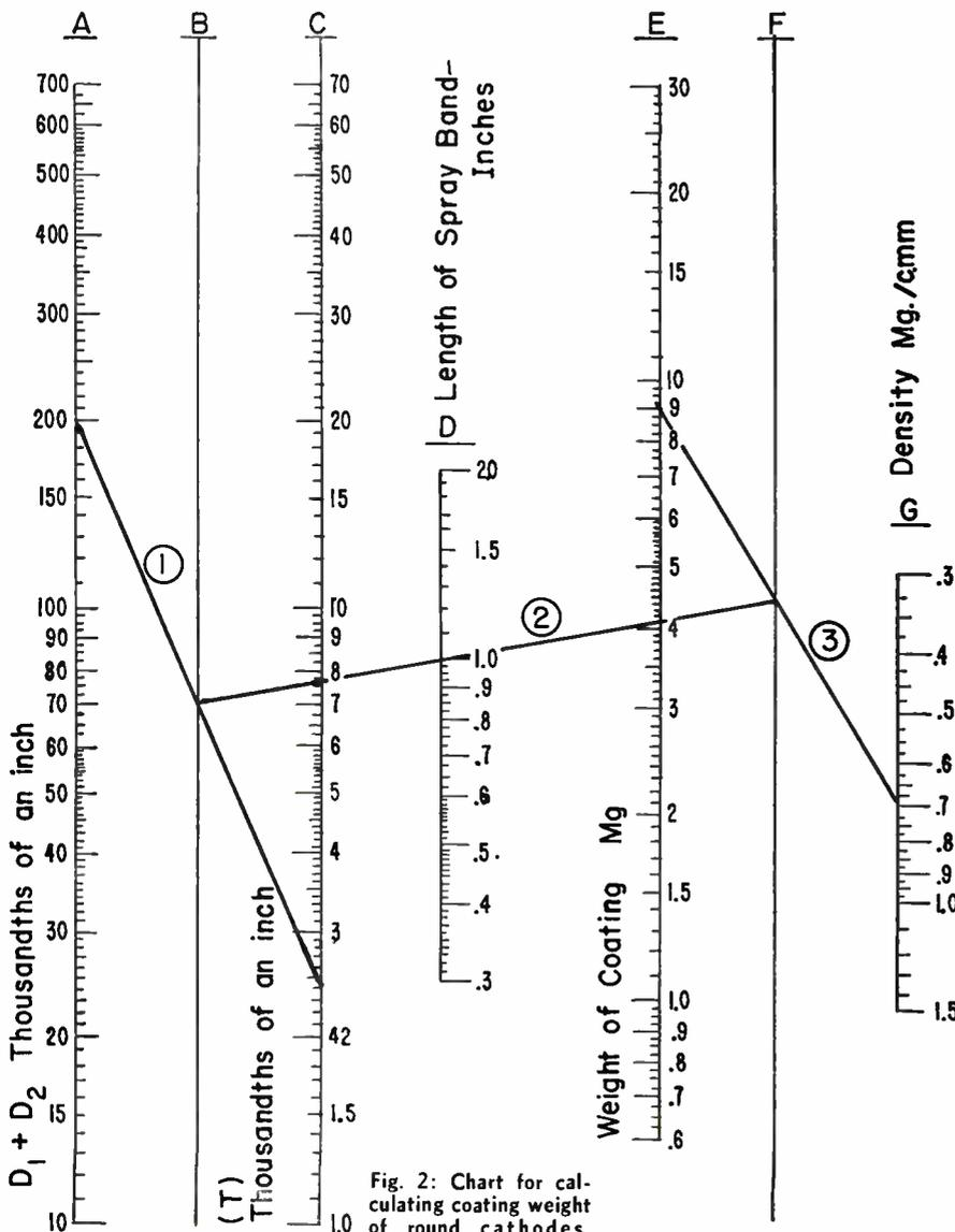
eral solution we have used a unit length of 1 inch and a density in terms of lb./in.<sup>3</sup> Diameter and thickness are in terms of inches.
