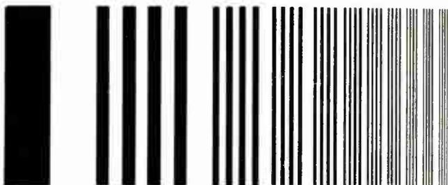
Fig. 1 (left): On the new resolution chart this pattern is displayed 9 times—3 rows vertically, 3 horizontally. In this way, the standard aspect ratio may be retained.
