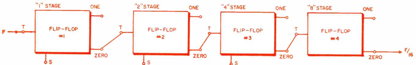
Fig. 2: Block diagram shows a straight through four-stage binary counter made possible by cascading circuit in Fig. 1.
