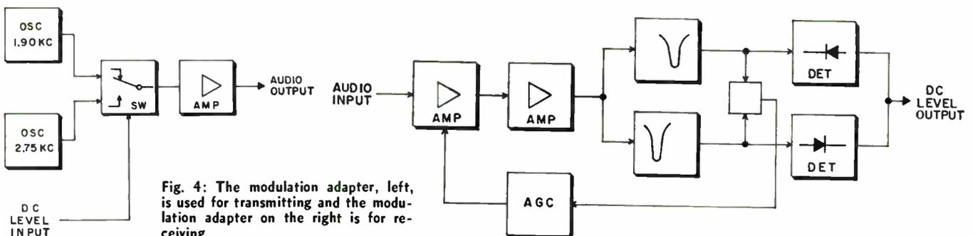
Fig. 4: The modulation adapter, left, is used for transmitting and the modulation adapter on the right is for receiving.
