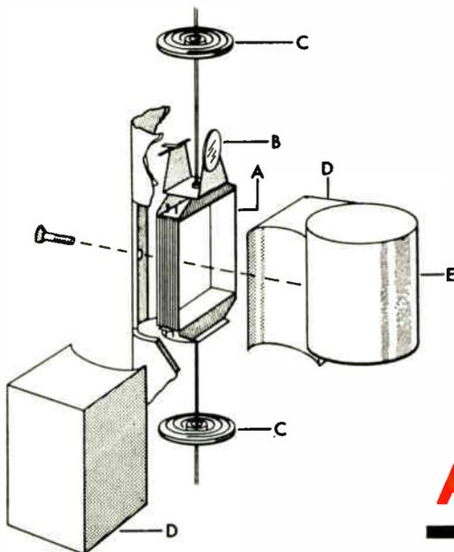
Fig. 1: Cut-away view of a bifilar meter movement showing the basic parts used. (A. Moving coil; B. Mirror; C. Disc spring; D. Pole piece; E. Core.)
