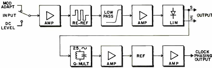
Fig. 5: The preamble is recognized by storing energy in a 25 cycle resonant circuit.
