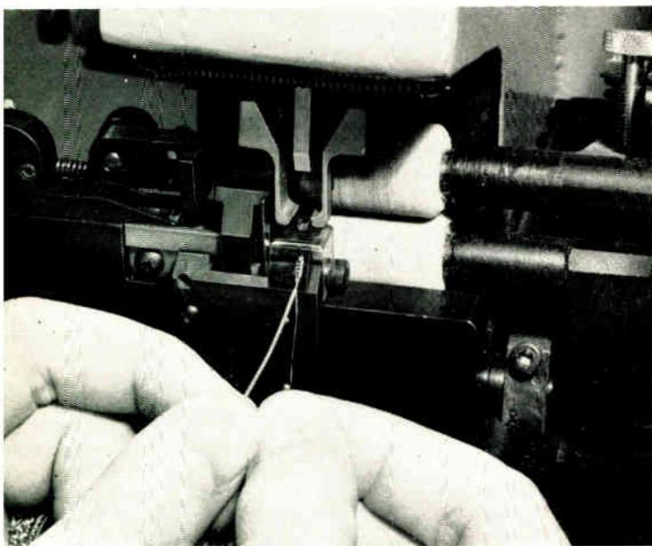
One hand positions the stripped fine wire into splice, the other hand positions pre-stripped lead wire into splice.
