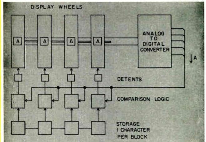
Fig. 11: The display wheels are turned in synchronism with the shaft position indicator.
