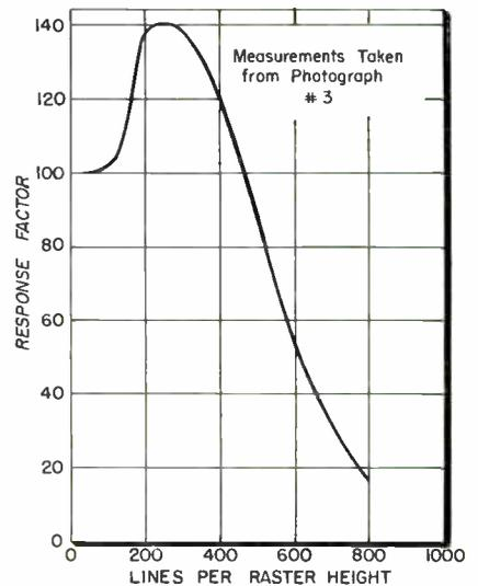
Fig. 5 (right): This is the curve for a signal from a system with "aperture boost."
