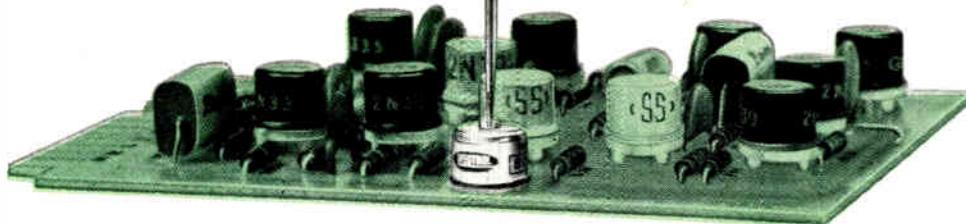
New Spectrol Model 80 single-turn trimming potentiometers in TO-9 size case...*the smallest MIL qualified trimming potentiometers available today...* give your circuits precision adjustment in  $\frac{1}{4}$  of the space required for most other trimmers.
