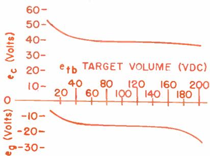
Fig. 3: The target-grid characteristics have a safety factor of 20 volts added to the data supplied by the manufacturers.
