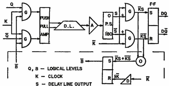
Fig. 28: Logical information delayed and clocked by phase reversal.
