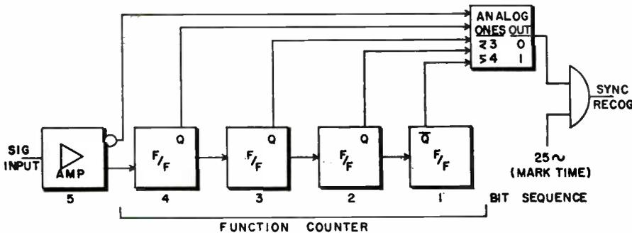
Fig. 7: The block diagram illustrates the sync recognition/function counter circuits.
