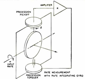
**Floated Rate Integrating Gyros.** Floated Rate Integrating Gyros are used where exceptionally high-level performance is required. Should the rotor mass of a gyro wheel having an angular momentum of  $1.0 \times 10^6$  gm. cm.<sup>2</sup>/sec. shift by as little as one micro-inch, a drift of 0.1°/hr. could result. The difficulty in achieving ultra-high precision and accuracy is apparent, and the necessity for obtaining low drift gyros is of paramount importance.
