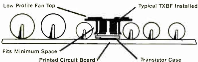
Unique Fan Top design places the heat-dissipating mass above and away from the transistor for greater cooling effectiveness in natural or forced air. Angled fan segments induce turbulence and faster convection. Spring fingers friction-fit to TO-5 transistor case variations from .305" to .335" and withstand maximum shock and vibration. Substantial junction temperature reductions improve switching speeds and other transistor characteristics!
