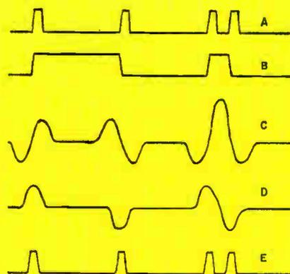
rate advantages. Figs. 21 (A) and (B) represent "one"s of the two methods. The amplified output, Fig. 21 (D), a combination of full and half-height positive and negative pulses can be detected by several different methods. Here are 3 such methods.
