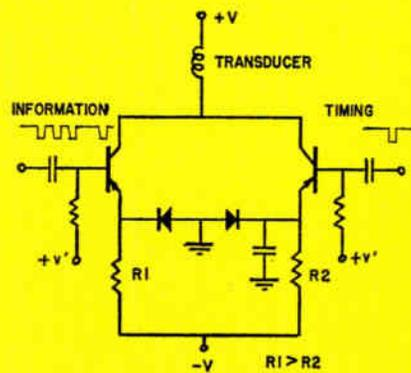
Fig. 26 (right): Input amplifier for two level recording.
