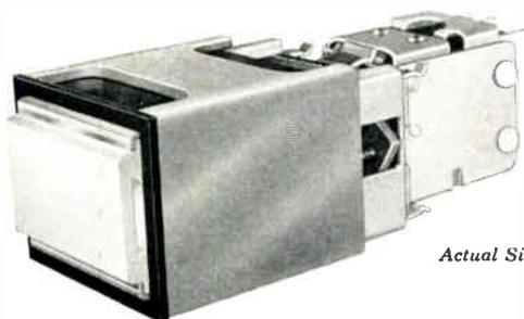
New **M**-SERIES Switchlite features: four independent MS 25237 lamps with silicon rubber color filters. Four types of ground circuits. Relamps from front of panel without tools.
