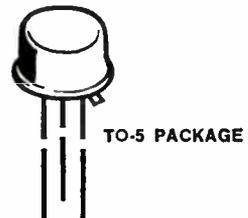
The PNP 2N1765 is a 3-junction, 3-terminal diffused silicon transistor in a vacuum-tight enclosure suitable for fast, high-current, pulse switching. This device's rise time to 30 amperes is less than 100 nanoseconds. Turn off time is approximately 1 microsecond. It is operational at emitter currents to 50a with gate drives from 5ma to 2a.
