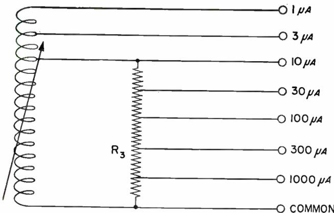
Fig. 6: Conventional meters use a large shunt across the coil.
