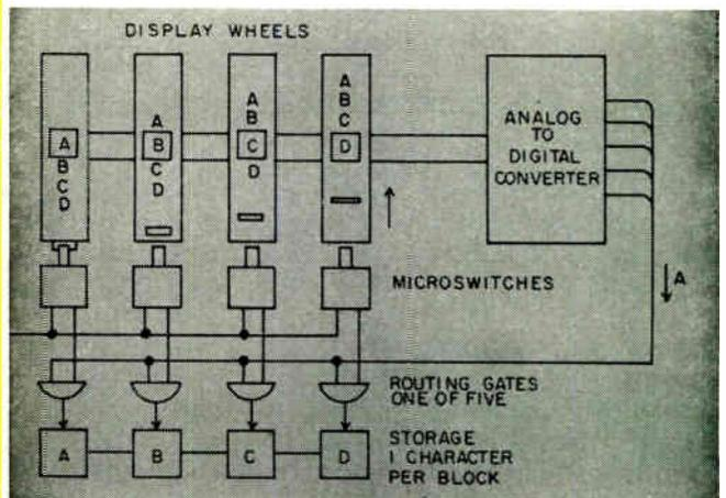
Fig. 12: Pushing transmit button transfers displayed mode and signature to storage.
