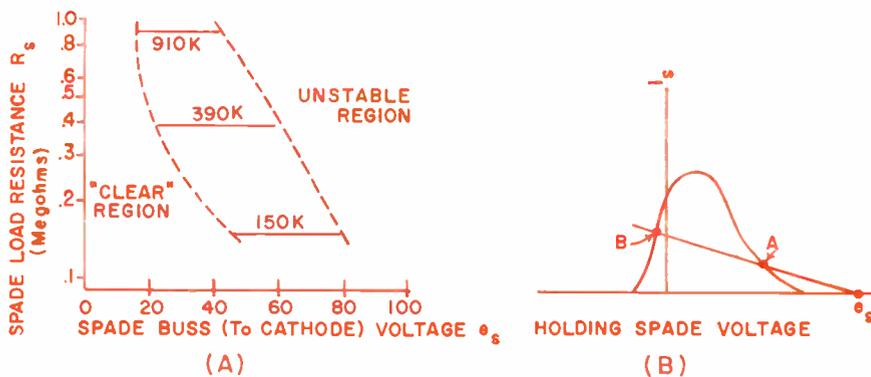
Fig. 2: The spade characteristics are used in the first step for designing circuitry.
