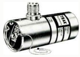
**TYPE 2970 (CW) LOCAL OSCILLATORS** — Power output greater than 5 mw. over entire C-Band. Temp. stability less than  $\pm$  2 Mc from -20°C to +105°C. Diameter 7/8", length 2". Weight 3 oz.
