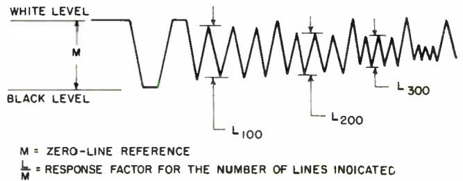
Fig. 4 (above): This is the method that is used to take data from scope trace photo.
