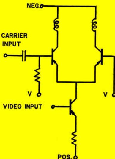
Fig. 29: Example of a video input transducer drive.
