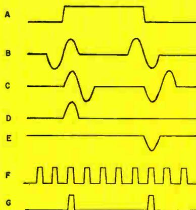
Fig. 24: Integrating method NRZ waveforms.
