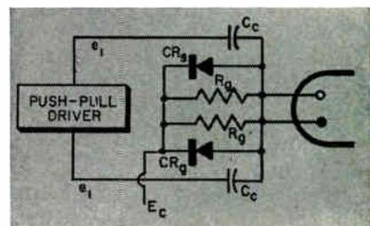
Fig. 7: This circuit provides dc restoration when the drive frequencies are too high to permit the grid network time constant to differentiate the input square waves.
