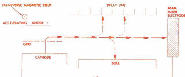
Fig. 1: Schematic of the beam miser indicates function in a standard beam-type tube.
