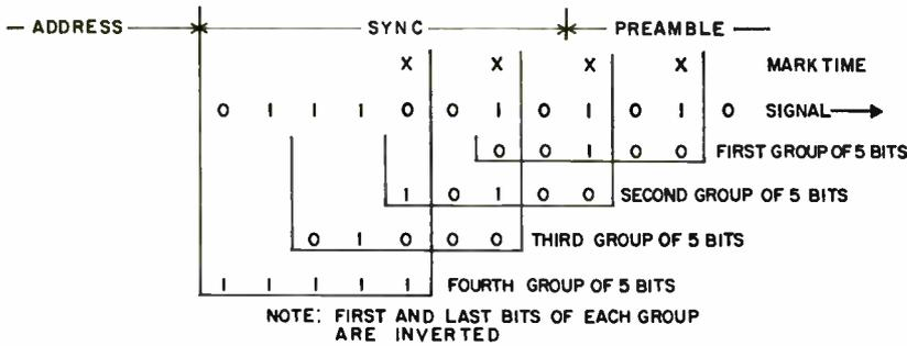
Fig. 6: Drawing shows that the first recognition of sync will be the proper one.
