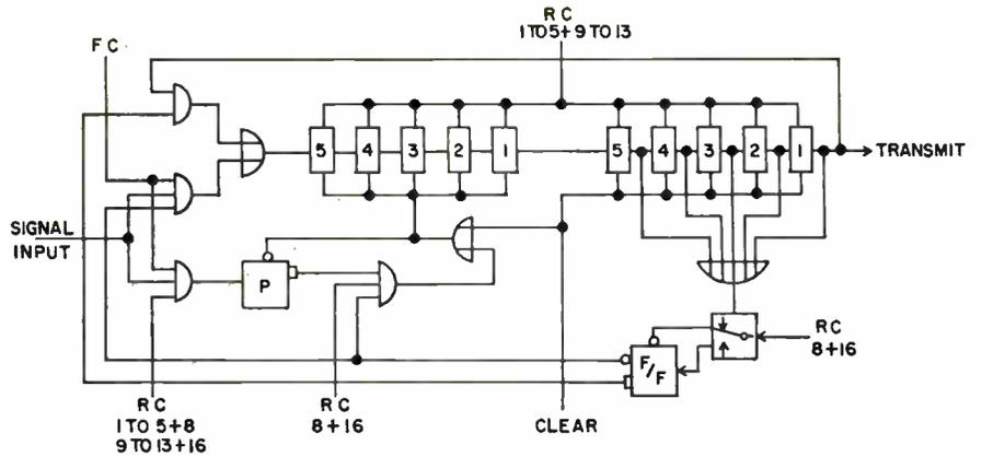
Fig. 9 (above): If the address is recognized, the signal is gated to mode storage as shown.
