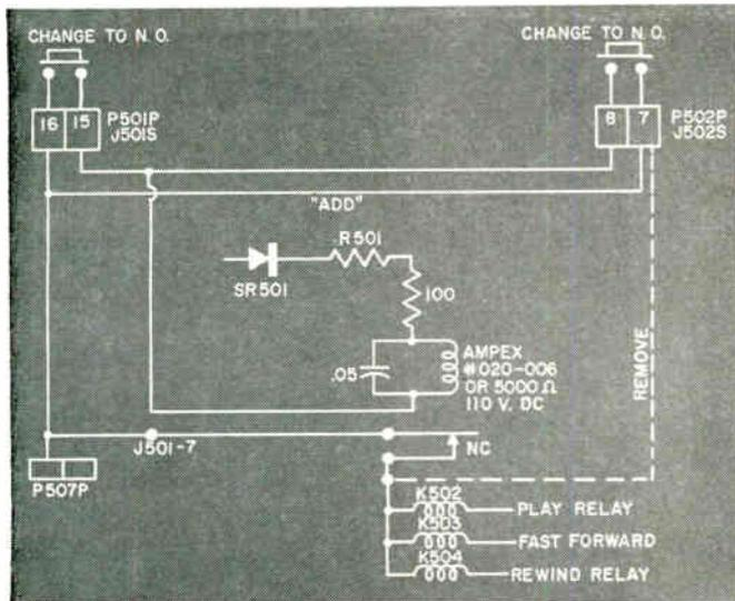
Relays added to "stop" circuit increases flexibility.
