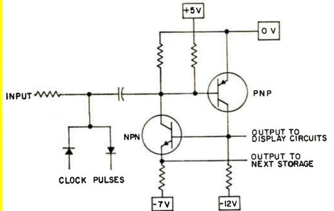
Fig. 10: Transistors are used in the storage circuit.
