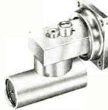
**TYPE 2969X3 X-BAND HARMONIC GENERATOR** — Requires 150 to 175 VDC at less than 12 ma and 6.3 V at 240 ma. One adjustment covers 8800 to 9000 Mc range with minimum of 5 mw output power.
