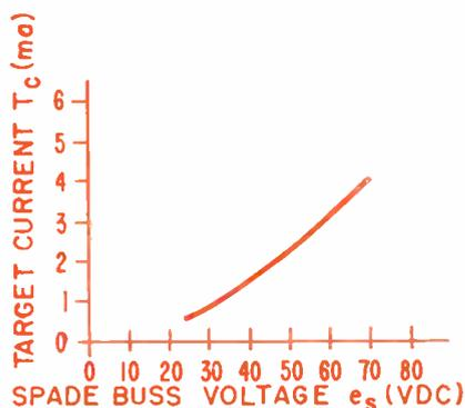
Fig. 4: The target-spade characteristics may also be used in the selection of the minimum spade-buss-to-cathode voltage.
