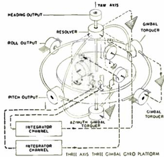
**Stable Platforms.** Essentially a cluster of gyros mounted within gimbals and utilizing acceleration sensing components, stable platforms perform the important function of having the gyro out-puts control the gimbals by means of a servo loop. By manipulating various arrangements of gimbals and gyros, a variety of platform types can be produced. They are used as reference elements and to stabilize accelerometers, star trackers, and similar devices in space.
