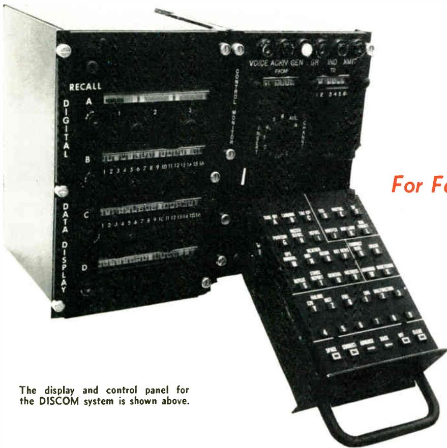
The display and control panel for the DISCOM system is shown above.
