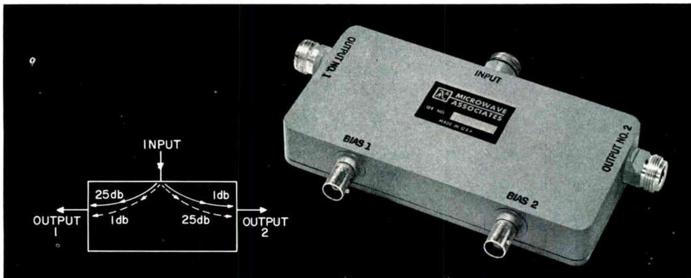
Microwave Associates has expanded its line of all-solid-state microwave devices with this new family of high power switches.
