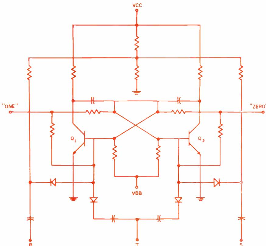
COUNTING circuits employing bistable flip-flop stages are widely used in electronic equipment design. This article describes a method for designing flip-flop counters without resort to logical equations or switching algebra. The procedure, which is based on a standard circuit configuration, is simplified by capitalizing on the cyclic properties of a binary chain. A decade counter is analyzed to illustrate the design technique.
