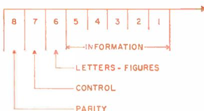
Fig. 1 (l): Field data code structure is illustrated.
