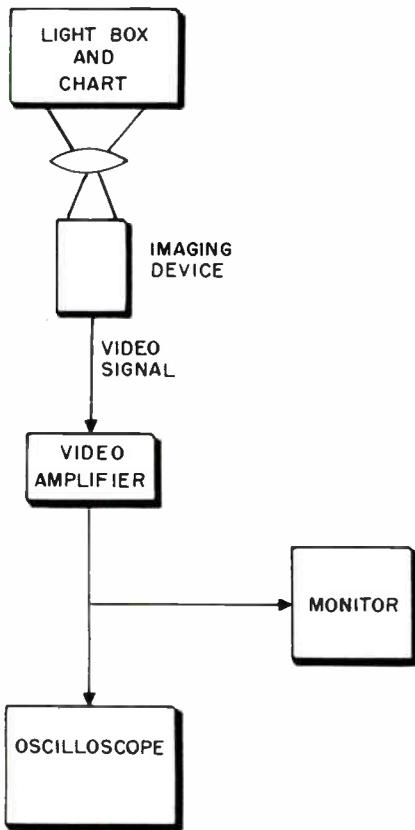
Fig. 3 (left): This basic measuring scheme is used to evaluate image tubes. The scope presentation is photographed, then curves similar to those shown in Fig. 2 are drawn.
