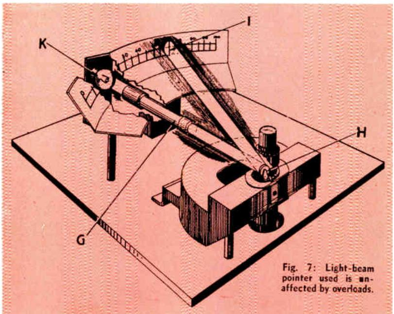
Fig. 7: Light-beam pointer used is unaffected by overloads.
