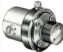
**TYPE 2975 CW OSCILLATOR** — Frequency 2 KMc, tuneable  $\pm$  20 Mc; power output 15 watts CW. Size 3 1/2" by 2 1/2" diameter. Weight 1 lb. Type 2975A CW amplifier with same specifications and power gain of 10 DB.
