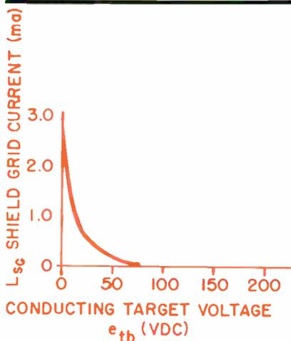
Fig. 5: The shield grid current can be found by using this target-shield curve.
