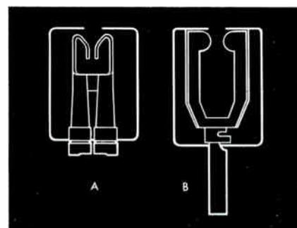
Wedging action of Amphenol ribbon-type (A) and long spring base of Amphenol Prin-Cir connectors (B) assure firm printed circuit board retention, whether board happens to fall at low (.055") or high (.073") end of thickness tolerance.
