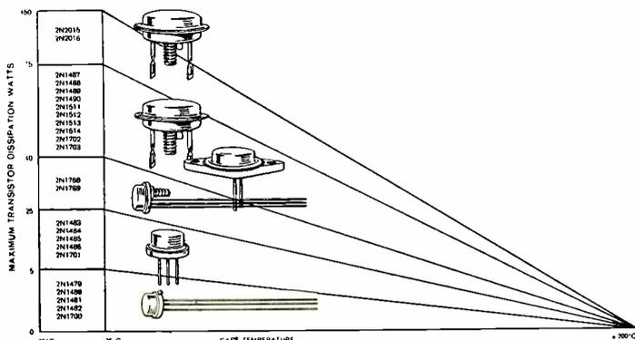
New Low Prices On RCA 2N2015 and 2N2016—10 Amp Silicon Power Units... Mass production economies make 200°C Silicon Power Transistors available at lower prices than ever before. These popular types incorporate the following outstanding features: 0.25-ohm max saturation resistance at  $I_C = 5$  amp... Beta of 15 to 50 at  $I_C = 5$  amp... Min. beta of 7.5 at  $I_C = 10$  amp.
