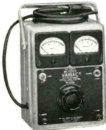
**W5MT3A** VOLTMETER/AMMETER COMBINATION
