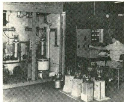
A linear amplifier test set for testing low mu factor, high perveance, high-power audio, and ultrasonic power tubes is shown in operation at the Westinghouse electronic tube division, Elmira, N. Y. Operator at the equipment console is matching two water-cooled tubes.
