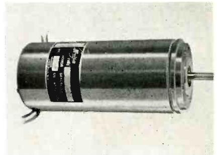
The V896-26B high performance servo motor generator is temperature stabilized by magnetic amplifier control to assure consistent accuracy despite temperature variations. Typical mechanical data includes: 4500RPM minimum no load speed; 2.35 in. oz. minimum stall torque; 35gm cm<sup>2</sup> rotor moment of inertia; and 4730 radians/sec. theoretical acceleration. The V896-26B weighs 27 ounces. Kearfott Div. General Precision, 1150 McBride Ave., Little Falls, N. J.
