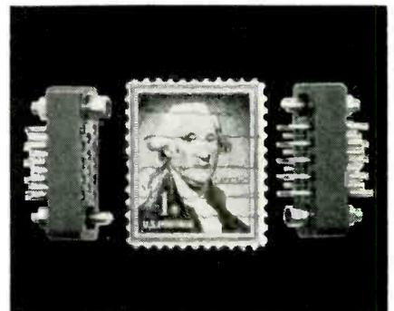
This connector line features: Dialyl Phthalate molding; 1-piece 3-48 thread screwlock; bow washers to eliminate axial float; square shoulder in molding for fixed screwlock; strengthened "C" clip groove; and controlled float in socket contact. The mounting pad surrounds the entire guide hole. Both male and female contacts are of phosphor bronze. The MM22 Series meets applicable Mil specs. Lionel Electronic Laboratories, Inc., 1226 Flushing Ave., Brooklyn 37, N. Y.
