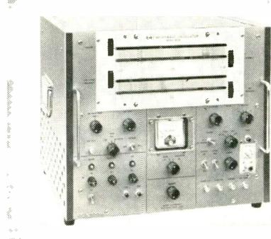
They have built-in Levelers which hold power output to approx. ±0.75 db over the entire freq. range and nominally to ±0.1 over any 100mc interval. All Series 620B oscillators also feature symmetrical freq. deviation about any center freq. These oscillators have very low residual FM and drift stability. Min. power output is 10mw. Freq. range adjustable freq. markers and sweep time can be seen at a glance. Alfred Electronics, 3176 Porter Dr., Stanford Industrial Pk., Palo Alto, Calif.
