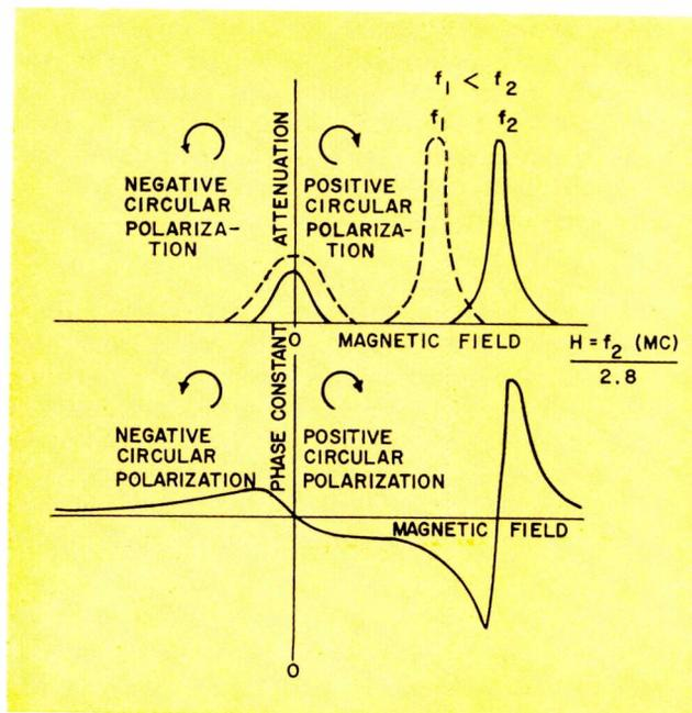
Fig. 3: Some typical phase and attenuation characteristics plotted as a function of the direct current field strength which is applied.
