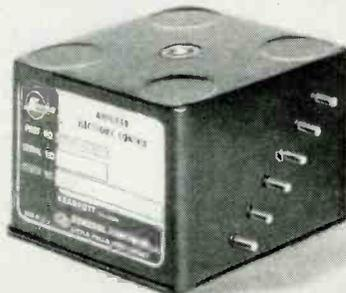
This encapsulated 5-watt amplifier, approximates one cubic inch in volume. Component elements are mounted in a high-density three-dimensional mass, and leads are interconnected by resistance spot welding. This process assures extremely high reliability.
