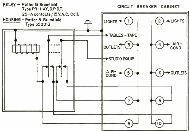
Throw On breakers 7, 8, 9 & 10. The relay should energize. To check out the system, throw breaker #9 to Off. Only a momentary interruption of power will take place as the relay is de-energized and the controlled loads move over to the other "live leg."
