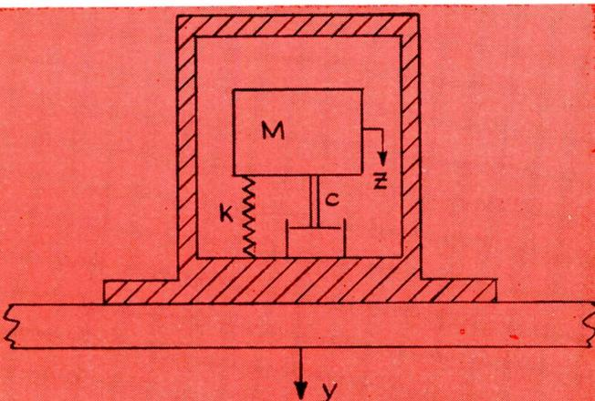
Equation of motion  $-m\ddot{z} + c(\dot{z} - \dot{y}) + k(z - y) = 0$
