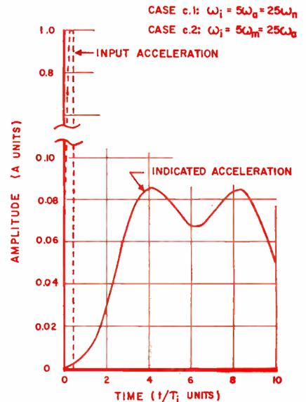
Fig. 7: Cases c.1 & c. 2 do not follow the input acceleration.
