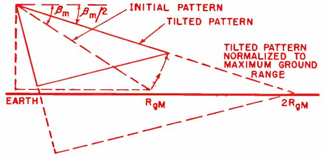
Fig. 2: Positive tilt is equal to half of  $\beta_m$ .
