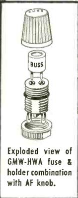
Exploded view of GMW-HWA fuse & holder combination with AF knob.
