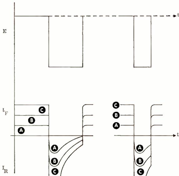
Fig. 7: The recovery characteristics of a junction diode to a long pulse and a short pulse for various values of forward current. With the large forward currents, the recovery time becomes greater.
