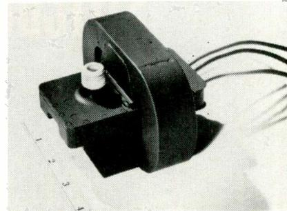
Designated the ZM-6050, it covers the 2.2 to 3.85gc freq. range and has a CW power output of 2w. Used as a local oscillator or a signal generator for rapid sweep applications such as radar and electronic countermeasures. The tube's low noise figure is the integrated noise in a band from 100kc to 100mc on both sides of the carrier freq. It weighs 3.5 lbs. and can be installed in any position. General Electric Co., Power Tube Dept., Schenectady, N. Y.
