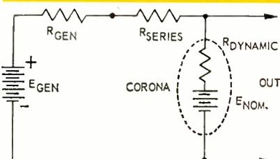
Fig. 7: A simple circuit used to analyze the tube in Fig. 6.
