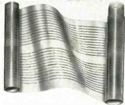
The conductors are encapsulated in Mylar. The material, a new variation of Methode's Plyo-Duct, is available in continuous lengths and contains up to 24 pairs or 48 conductors of 0.002 in. round copper wire. This wire, in a film 0.004 in. thick, has spacing tolerances of 0.002 in. Plyo-Duct has high dielectric strength under severe environmental conditions, with very good flex-life and min. weight characteristics. Methode Electronics, Inc., 7447 W. Wilson Ave., Chicago 31, Ill.
