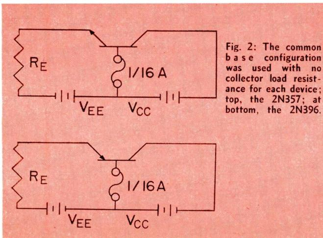
Fig. 2: The common base configuration was used with no collector load resistance for each device; top, the 2N357; at bottom, the 2N396.
