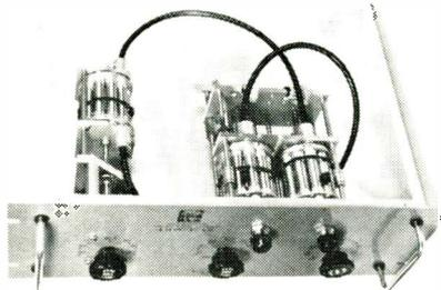
Stoddart R-F Step Attenuators use the "Pull-Turn-Push" turrent control. They are for use with standard 50Ω coaxial cable circuits, and are available in either 2 or 3 turrent models. These attenuators have high accuracy from dc to 30C with a very low phase shift characteristic at i-f freqs. up to 160Mc. VSWR is less than 1.5 overall. Stoddart Aircraft Radio Co., Inc., 6644 Santa Monica Blvd., Hollywood 38, Calif.
