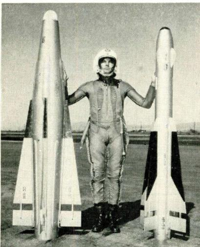
Test pilot Bart Warren holds air-to-air guided missiles, the HM-55 (l) and the HM-58 Falcons, which are being developed for the Swedish Air Force by Hughes Aircraft Co. of Culver City, Cal. Missiles will be manufactured in Sweden to Hughes' design. The HM-55 is radar guided and the HM-58 is infrared guided.
