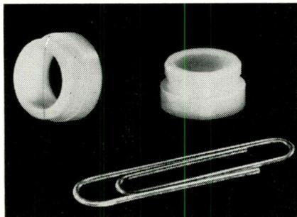
It provides mechanical mounting of the transistor without the need of a socket on metal chassis. The Sealectro B-1470 (Teflon) Transistor Bushing is pressed into a prepared hole 0.4 in. in dia. The Bushing is hollow, with a lead hole of 0.330 in. in dia. for connection of transistor leads. The receptacle for the transistor body is 0.300 in. in dia., and is chamfered for easy inserting. Height above chassis is 0.120 in. Sealectro Corp., 139 Hoyt St., Mamaroneck, N. Y.
