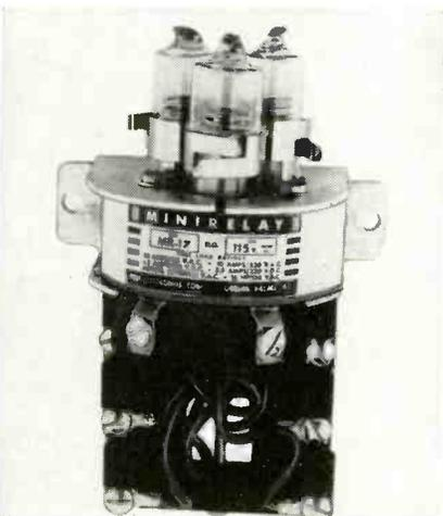
The MR-17, 3PST Minirelay, has mercury-to-mercury contacts for silent, maintenance-free operation. Hermetically sealed in an inert gas atmosphere, there are no contacts to pit, stick or corrode, even after millions of operations. Each tube of the MR-17 is rated 20a at 115vac, 10a at 230vac and 5a at 440vac. The 3 $\phi$  motor rating is 2 HP at 115 or 230vac. It measures 5 x 2 1/2 x 3 1/4 in. Ebert Electronics Corp., 212-26 Jamaica Ave., Queens Village 28, N. Y.
