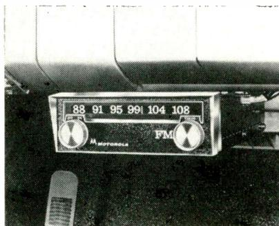
Motorola's new model operates through car's existing AM radio system. Chassis features seven tubes, two limiters with its own r-f stage, automatic gain and frequency controls. Suggested retail price is \$69.95.
