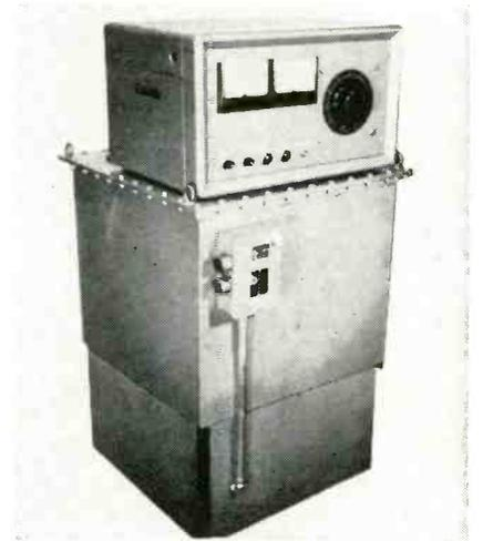
Input requires 105 to 125vac, 60CPS. The instrument and control center, mounted on the high voltage assembly tank, may be used at a remote point. The instrument and control center contains complete metering, overload protection, switches and indicators, as well as the output control. The high voltage assembly tank with casters measures 24 x 24 x 40 in. The control center measures 21 9/16 x 14 7/8 x 13 in. Plastic Capacitors, Inc., 2630 N. Clybourn Ave., Chicago, Ill.
