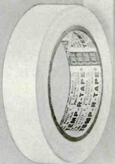
Pressure Sensitive Temp-R-Tape® is produced by CHR in a good variety of thicknesses and widths. If you require reliability Temp-R-Tape has it . . . ■ High dielectric. ■ Resistant to environmental aging. ■ Withstands temperatures from -100 to +500°F. ■ Extremely thin and lightweight. ■ High elongation — tight wrap over sharp bends. ■ Non corrosive — non contaminating. ■ Non moisture absorbing. ■ Temp-R-Tape is stocked by distributors
