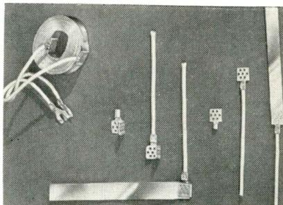
The TERMI-FOIL terminal is designed to reduce costs and improve performance of electrical equipment using aluminum foil and strips. It eliminates surface preparation. When the terminal is pressed into the foil by flat surface dies, tab projections pierce the foil, then fold over, securely riveting the foil to the surface of the terminal. The terminal will cover aluminum sheeting from 0.002 to 0.035 in. and can be spliced to 12-10 size wire. AMP INC., Harburg, Pa.
