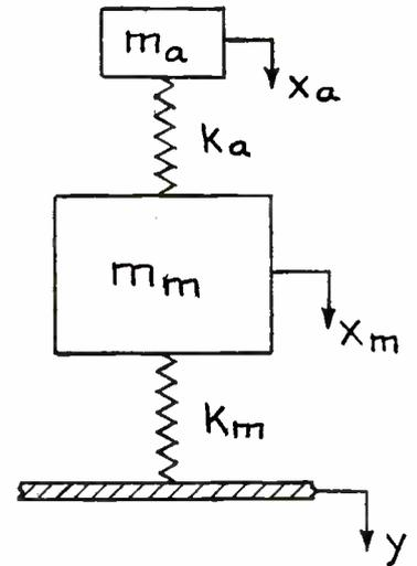
Fig. 3 (r.): The equivalent mechanical system of the encircled portion of Fig. 2.
