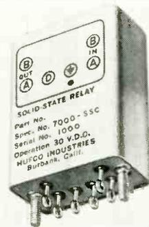
A SPST relay, with a contact rating of 1a, it operates on an input voltage of 10 to 30vdc. Contact voltage freq. range: from 300CPS to 30KC. Pickup time is 1msec. for relay latching, and dropout time is 2msec. after removal of contact voltage. Unit withstands temperature from -55°C to +100°C, with special models to +125°C. Weight is less than 2 oz. Multipole ac or dc types are also available. Hufeco Industries, 2815 W. Olive Ave., Burbank, Calif.
