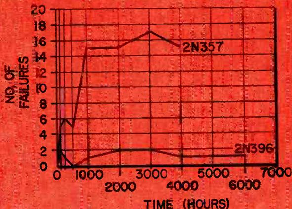
Fig. 6: The failure rates for the two types of transistors tested.
