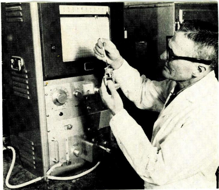
Gas chromatography is used in detecting major and trace constituents in the manufacture of chemicals for the electronic industry.
