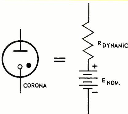
Fig. 6: The equivalent circuit for a gas discharge tube in the corona mode.
