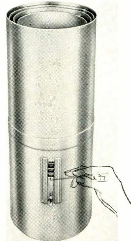
This line of diversionary Netic and Co-Netic magnetic shields use 2, 3 or 4 concentric cylindrical shields, one inside the other. The shield illustrated is 36 in. high and 15 in. O.D. It consists of 3 inner shields of high permeability Co-Netic alloy and 1 outer shield of heavy gauge Netic alloy. For viewing the sample under cryogenic test, a multi-section viewing port is provided. Magnetic Shield Div., Perfection Mica Co., 1322 No. Elston Ave., Chicago 22, Ill.
