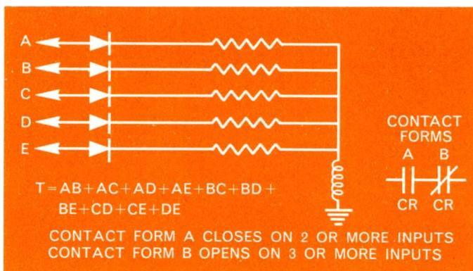
To perform 2 out of 5 logic, five inputs, five resistors and a simple Clareed Control Module with normally open and normally closed contacts are used. This
