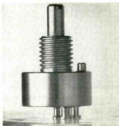
The JP/2 is a panel mount potentiometer, smaller in overall volume than standard ½ in. miniature pots and considerably lower in cost. It is designed to meet standard military environmental specs. The JP/2 can be interchanged with most ½ in. pots. It is available in a resistance range from 10Ω to 20kΩ. Waters Manufacturing, Inc., Wayland, Mass.
