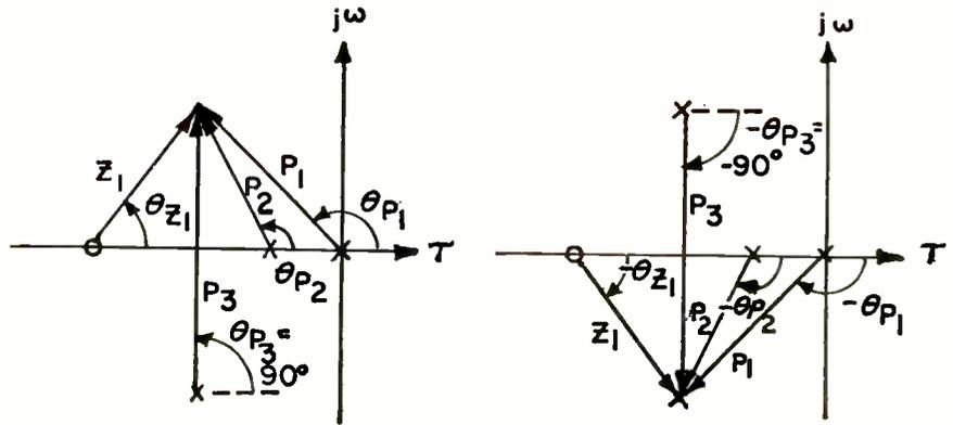
Fig. 4: Coefficients corresponding to complex conjugate poles are also complex conjugates.
