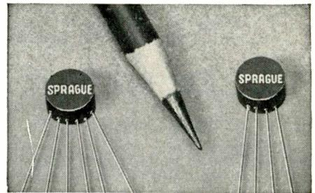
Digital circuit designers will find the new Sprague Type 43Z Nanosecond Pulse Transformers of considerable interest. These tiny transformers have been carefully designed for the all-important parameter of minimum rise time at high repetition rates up to 10 mc.
