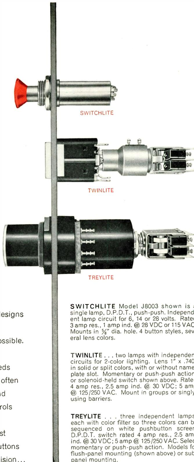
**SWITCHLITE** Model J8003 shown is a single lamp, D.P.D.T., push-push. Independent lamp circuit for 6, 14 or 28 volts. Rated 3 amp res., 1 amp ind. @ 28 VDC or 115 VAC. Mounts in 5/8" dia. hole. 4 button styles, several lens colors.
