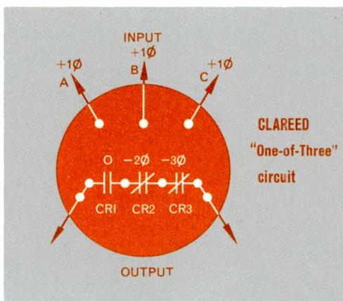
and opens. No output is obtained. A "one of three" check has been established.
