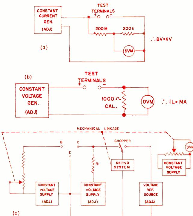
The automatic test set, Fig. 4, has circuits for measuring voltage breakdown, leakage current, and current gain, Fig. 5. The current gain module affords a direct digital readout of current gain.
