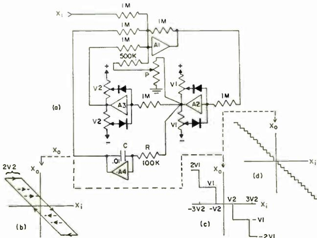
Fig. 3a: Addition of integral feedback. b: Backlash simulation. c: Quantizing simulation. d: Granularity simulation (small quantizing steps).
