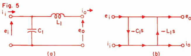
The remainder of the flowgraph is drawn with the rest of the elements in order, one at a time. The transmittances of parallel components are drawn as subtractive admittances, directed toward the current flow. The transmittances of series components are represented by impedances subtracting from the voltage signal flow path. The flowgraph will now be as in Fig. 6a.
