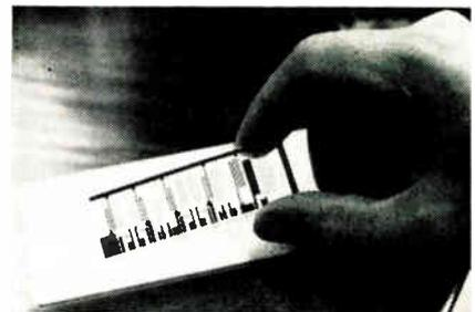
Heretofore, tantalum devices have been sputtered in an atmosphere of inert gas such as argon. Traces of certain impurities, like oxygen and water vapor, usually appear in these tantalum films, resulting in resistors with relatively wide variances in resistivity and temperature coefficient.
