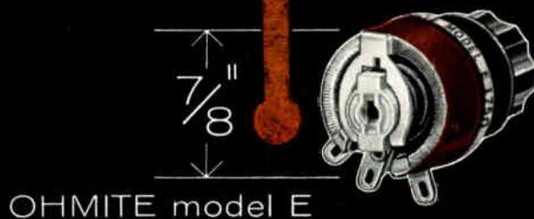
■ Here's real power in a small package for operation at elevated temperatures where units with organic materials fail. All ceramic and metal in construction, the Model E rheostat is designed to operate at a maximum hot spot temperature of  $340^{\circ}\text{C}$  without charring, shrinkage, or deterioration. Full rating is  $12\frac{1}{2}$  watts at  $40^{\circ}\text{C}$ , but even at  $125^{\circ}\text{C}$ , there is still a sizeable 8-watt rating for units through 5000 ohms.
