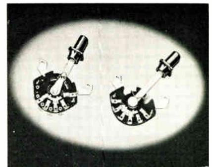
The PA-700 series is available as single units or ganged assemblies with end brackets for mounting. Rated at 1.5a at 28vdc, 230ma at 115-vac, with a current carrying capacity of 9a. Clips and rotor contacts are silver plated brass and clips will accommodate up to No. 18 wire. Silver alloy clips are available. Insulation is laminated phenolic with voltage breakdown between critical parts of 1000v RMS. Centralab. The Electronics Div. of Globe-Union Inc., 900 E. Keefe Ave., Milwaukee 1, Wisc.
