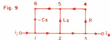
The graph of Fig. 9 has a single path (1,2,3), +1. Its loops are the same as for the flowgraph of input impedance, Fig. 7d. Current gain,
