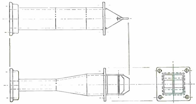
Fig. 4: Drawing of X-band vertical polarized antenna.
