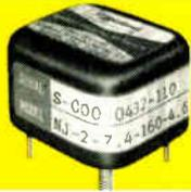
Hermetically sealed, four-crystal, wide-band filters. Dimensions are 1-1/8L x 1-1/8W x 3/4H. Designed to withstand 100 g shock and 15 g to 2 KC vibration. Operating temperature range —55°C to +90°C. 40db/3db Band Width Ratio is 1.8.
