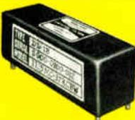
Hermetically sealed, four-crystal, narrow-band filter. Dimensions are 2-3/16L x 3/4W x 3/4H. Designed to withstand 200 g shock and 15 g to 2 KC vibration. 60db/3db Band Width Ratio is 6.3.
