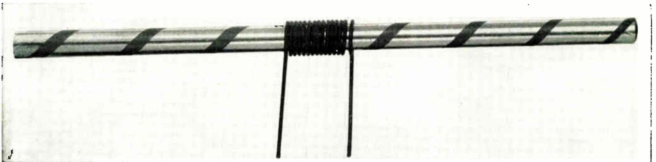
Fig. 9. Demonstration element of helically wrapped metallic-tape twistor storage method, enlarged. Incomplete systems, multiple drive
