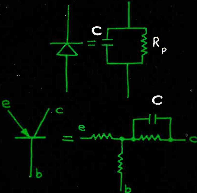
If you must measure C between 20  $\mu$ pf and 11,000 pf or  $R_p$  between 1000 ohms and 1000 megohms, we know you will be interested in our Capacitance Bridges.
