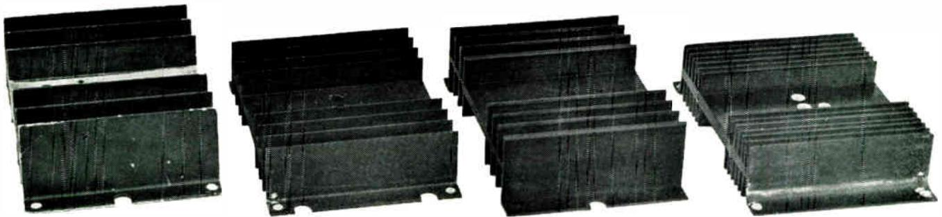
Fig. 1: Shown are some of the heat sinks used to determine the optimum configuration for the best heat dissipation.
