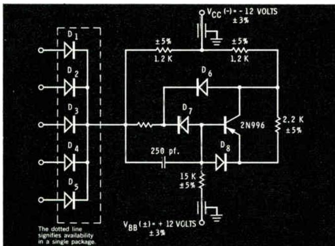
FAN OUT MAXIMUM = 5; TYPICAL PROPAGATION DELAY = 15 nSec.
