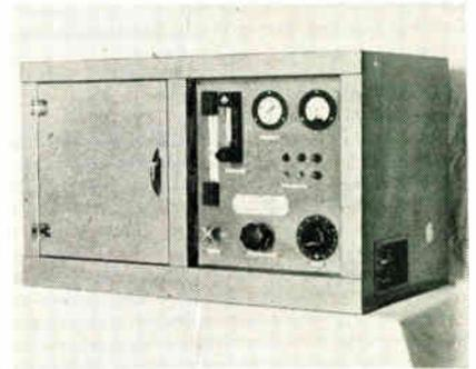
OREC O3C Series Ozonators produce ozone up to 36 grams/hr. and may be used for both laboratory and production process applications. Ozone output is panel regulated and units incorporate integral ozone monitoring equipment. Ozone concentrations as high as 70mv/liter can be delivered using oxygen as parent gas. Power requirements: Model O3C6, 650w; Model O3C12, 1300w. Ozone Research and Equipment Corp., 3840 N. 40th Ave., Phoenix, Ariz.
