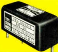
Hermetically sealed, eight-crystal, narrow-band filters. Dimensions are 2-3/8L x 1W x 1-1/32H. Designed to withstand 200 g shock and 15 g to 2 KC vibration. Operating temperature range —55°C to +90°C. 60db/6db Band Width Ratio is 2.3.
