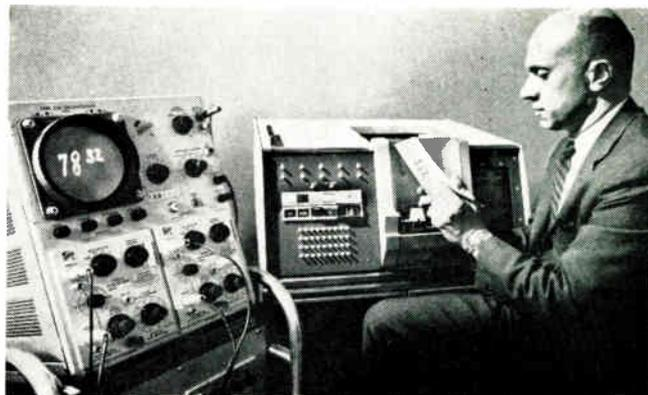
IBM's experimental numeral reader recognizes numbers that are handwritten in a variety of styles, sizes and positions.
