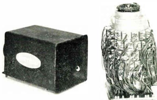
Fig. 5. Magnetic drum, developed by Ex-Cell-O Corp. (Bryant Computer Div.), stores over 12,000 words, rotates at 12,000 rpm. It is used in a high-density military airborne computer.
