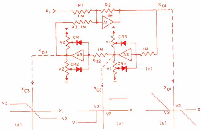
A BASIC circuit using the high gain negative feedback method for nonlinear simulation is shown in Fig. 1a. Operational amplifier  $A_1$  has unity gain from  $X_i$  to  $X_{O1}$  (since  $R_1 = R_2$ ); the feedback path is from  $X_{O1}$  through  $A_2$  and  $A_3$  in series back through  $R_3$  to  $A_1$ . The circuit has two distinct modes of operation: (1) when the input signal at  $X_i$  is less than the bias voltage  $V_2$ , and (2) when  $X_i$  is greater than  $V_2$ .
