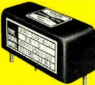
Hermetically sealed, eight-crystal, narrow-band filters. Dimensions are 2-3/8L x 1W x 1-1/32H. Designed to withstand 200 g shock and 15 g to 2 KC vibration. Operating temperature range —55°C to +90°C. 60db/6db Band Width Ratio is 1.8.
