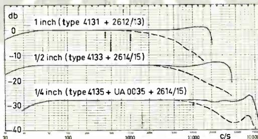
Typical frequency response of the B & K free-field calibrated Microphones. The curves in full are the free-field response for normal (0°) incidence with protecting grid in the case of 1-inch and 1/2-inch Microphones and without protecting grid for 1/4-inch Microphones. The dotted line in each case represents the over-damped pressure response. NOTE: The sensitivity of the Microphones is referred to 5 mV/μbar = -46 db, re. 1 V/μbar.
