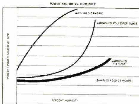
**MOISTURE ABSORPTION — COATED INSULATIONS —** In moist or humid environments "Fibremat" outperforms varnished cambric or polyester-glass materials. Continuous filaments in woven fabrics wick up moisture and offer a direct path for moisture to follow. The non-woven construction of "Fibremat" prevents wicking and moisture absorption. The power factor of varnished "Fibremat" remains relatively stable while the power factor of the other insulations zoom upward under increased humidity conditions.
