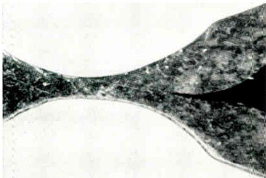
Cold-Welded germanium power transistors originated with Tung-Sol. The Cold-Weld process provides Tung-Sol transistors (in all case styles) with several significant advantages over transistors sealed by other techniques:
