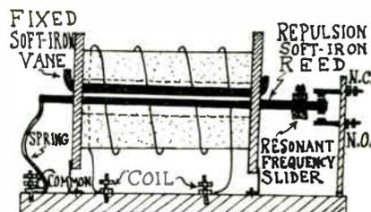
Adjustable slider is shifted in a slotted hole to vary frequency of relay.
