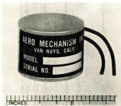
The Model 9026 actuates on an increase in altitude from 15,000 to 18,000 ft. and deactivates on decreasing altitude from 15,000 to 12,000 ft. It is a SPDT switch, rated at 2a resistive with contacts in either NO or NC position. Temp. range under continuous operation is from -54° to 125°C, per Mil-Std. 202B, Method 102A. Meets or exceeds Mil-Std. 202B for resistance to humidity, salt spray, sand and dust. Aero Mechanism, Inc., 7750 Burnet Ave., Van Nuys, Calif.
