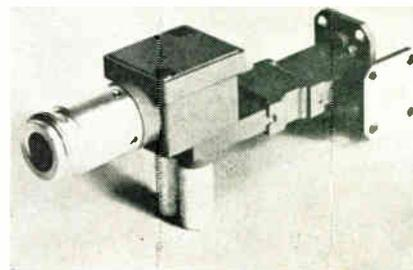
The Sidewall Balanced Mixer has an i-f output of 2.9Gc with input frequencies of 34.0—36.0Gc. The i-f output uses a type "N" connector and has a vswr of 1.20. This compact unit measures less than 4.00 in length and uses 1N53 crystals. Electrical specifications include: vswr=1.30 max. and isolation=12 db min. Microwave Development Laboratories, Inc., 15 Strathmore Rd., Natick Industrial Centre, Natick, Mass.
