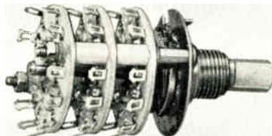
The 1 in. "Acorn" Rotary Switch has a dia. of just 1 in. (13/32 in. over 45° bend terminals). It can provide 12 positions, with each position being mechanically indexed by OAK precision dual-ball spring operated mechanism. Available in a variety of configurations. Stops can be fixed at any specified total number of positions. Performance tolerances include a temp. range of standard commercial -25° to +85°C. and military -65° to +125°C. Oak Manufacturing Co., Crystal Lake, Ill.
