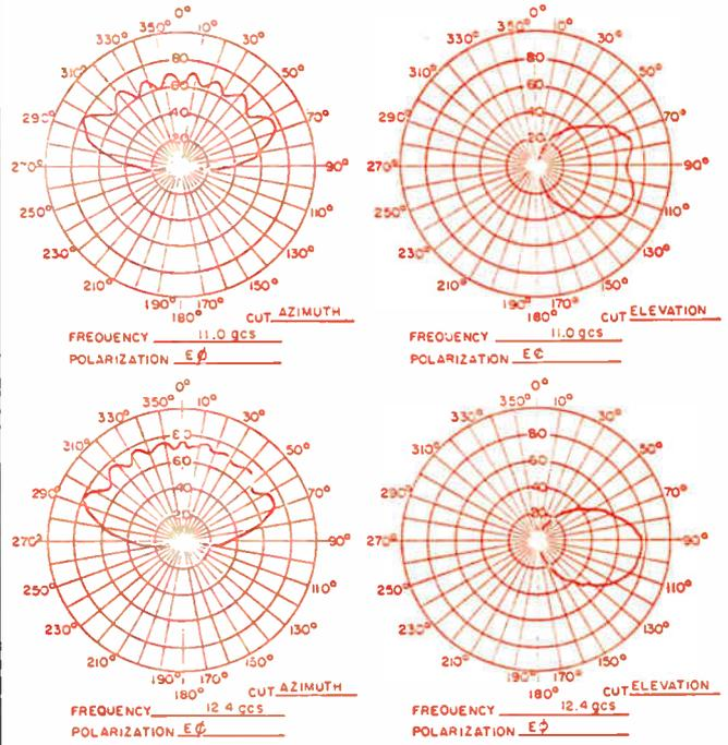
Fig. 11: Radiation pattern data for linear horizontal antenna.
