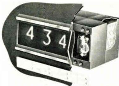
TNR Series transistor-driven readout, measures 1 x 1 1/4 in. x 3 in. External drive circuits or relays are eliminated by the self-contained NIXIE® driver. Internal circuits controlled by input signals of 4v to select numeral. High voltage, 180vdc at 2 to 3ma to fire numeral elements, is confined to unit and console. Only low level control signals required from logic circuits. TEC-LITE Div., Transistor Electronics Corp., 3357 Republic Ave., Minneapolis 26, Minn.
