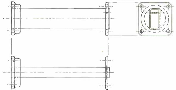
Fig. 5: Drawing of X-band horizontal polarized antenna.
