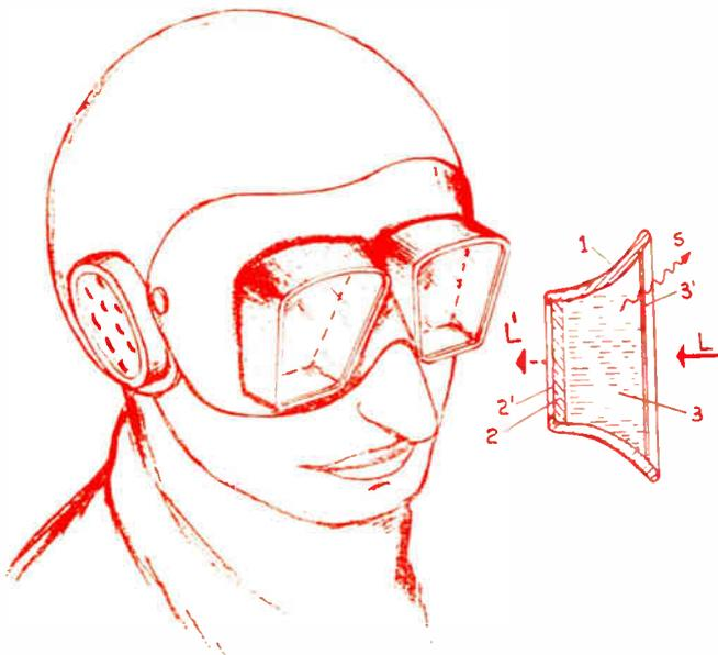
Fig. 7: Shown is eye armor design. The lens passes only enough light for working vision by means of a filter.
