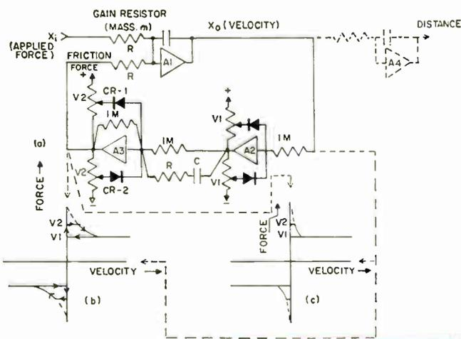
dead space voltage  $V_2$ , a step of magnitude  $V_1$  appears at the output  $A_2$  as explained before. A fast acting integrator,  $A_4$ , integrates this voltage and applies additional negative feedback to the input of  $A_1$ . The action continues until the output of  $A_2$  is forced back to zero, at which time the circuit returns to the dead space condition.
