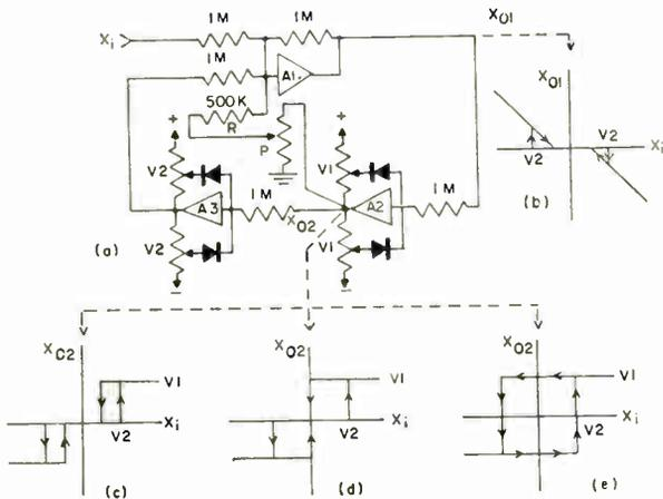
Fig. 2a: Addition of positive feedback to basic circuit. b: Output of  $A_1$  ( $\beta V_1 = 0.5V_2$ ). c:  $\beta V_1 = 0.5V_2$ . d:  $\beta V_1 = V_2$ . e:  $\beta V_1 = 2V_2$ .  $\beta$  is the positive feedback factor and is determined by the setting of potentiometer P and resistor R.
