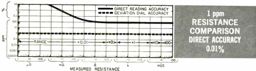
Two like resistances can be compared to an accuracy which is limited only by the resolution, sensitivity, and short term stability of the resistance measuring system. Outstanding stability results from the use of specially designed ESI resistors, assuring comparison accuracy of 1 ppm and direct accuracy to 0.01%.
