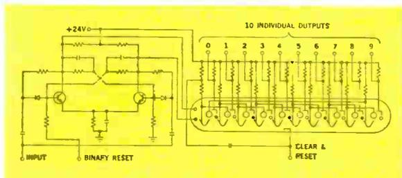
Fig. 1 BEAM-X Switch Decade Counter
