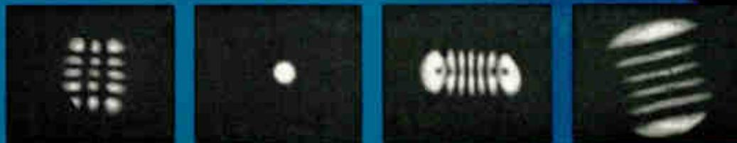
Photographs of simple standing wave modes set up on the GL-6211. Patterns are stable and reproduceable.
