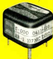
Solder-sealed 1-1/8L x 1-1/8W x 3/4H case. Center frequency adjustment screw, bottom-center. Voltage output essentially linear from  $f_0$  to  $\pm 15$  KC. Recommended circuit for use with Midland Type AB-1 Discriminator is shown below.
