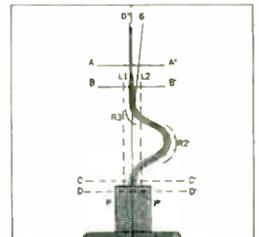
Shadowgraph inspection of whisker shape is typical of careful controls and checks in Sylvania diode manufacture.
