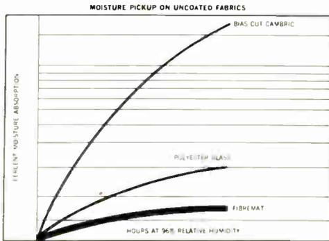
**MOISTURE ABSORPTION — UNCOATED FABRICS —** There's no pre-baking to drive out moisture when you use "Fibremat." The non-hygroscopic base fabric resists moisture. When exposed to 96 percent relative-humidity for 45 hours bias-cut cambric showed a moisture absorption of 25 percent, polyester-glass showed a moisture absorption of 2 percent, while "Fibremat" showed a moisture absorption of less than .7 of one percent. Proof of the superior moisture-resistance of "Fibremat" Insulation.
