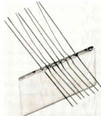
Copper ribbon wires (0.002" x 0.01") welded to edge of nickel-plated ceramic substrate. Shows wide range of thicknesses and materials which can be joined on the same machine.
