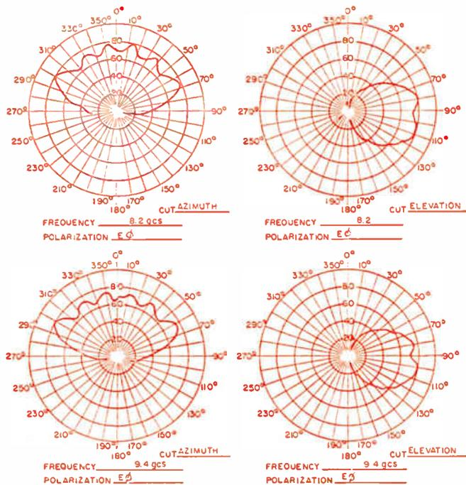
Fig. 10: Radiation pattern data for linear horizontal antenna.
