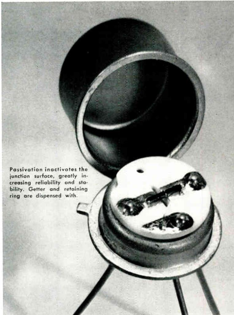
Passivation inactivates the junction surface, greatly increasing reliability and stability. Getter and retaining ring are dispensed with.
