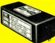
Hermetically sealed, eight-crystal, narrow-band filter. Dimensions are 2-3/16L x 1W x 3/4H. Designed to withstand 200 g shock and 15 g to 2 KC vibration. Operating temperature range —55°C to +90°C. 60db/3db Band Width Ratio is 2.8.
