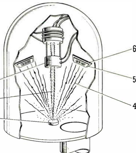
A 20,000 volt electron beam gun (1) directs electrons (2) at a material (3) causing it to evaporate. The resultant vapor (4) passes through a mask to form a film on ceramic (6).
