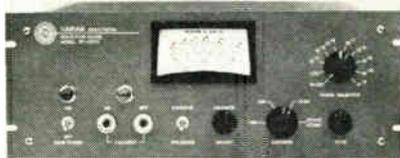
Pressures between 10<sup>-4</sup> and 2 x 10<sup>-11</sup>mm Hg can be read from linear scales. The grid supply produces a stabilized current output which can be varied between 50 $\mu$ a and 10ma for use with most ionization gauges. Recorder output terminals, electron bombardment degassing of both grid and collector, filament protection circuit and external relay circuit are some of the additional features. Vacuum Products Div., Varian Associates, 611 Hansen Way, Palo Alto, Calif.
