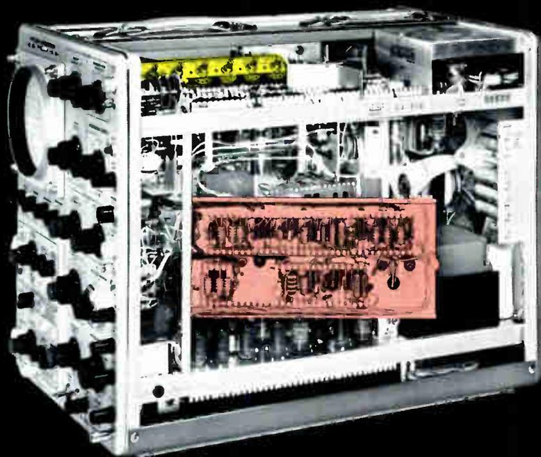
This shows the use of A-B fixed and variable resistors in the Tektronix Type 545A high-speed DC to 30 mc laboratory oscilloscope.
