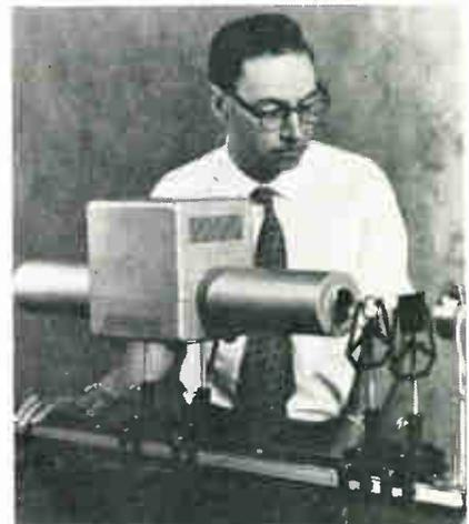
Continuous wave helium-neon gas phase laser being checked above is first such device commercially available. It produces highly directional, coherent beam of near-infrared light. Plasma tube is fused silica construction, and the radio frequency excitation unit is integrally mounted in tube center. New laser, developed by Perkin-Elmer Corp. and Spectra-Physics, Inc., will be marketed by latter.
