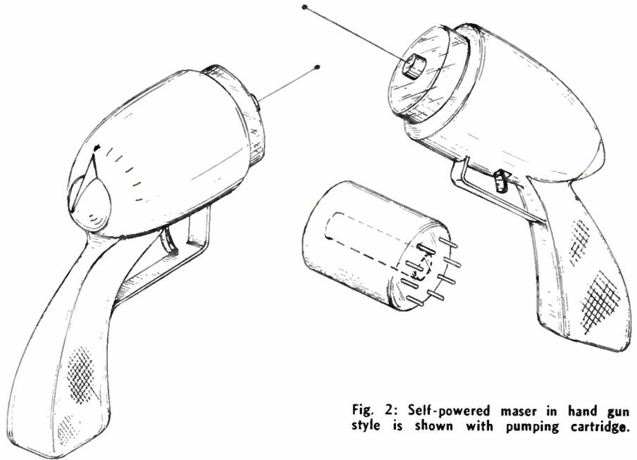
Fig. 2: Self-powered maser in hand gun style is shown with pumping cartridge.
