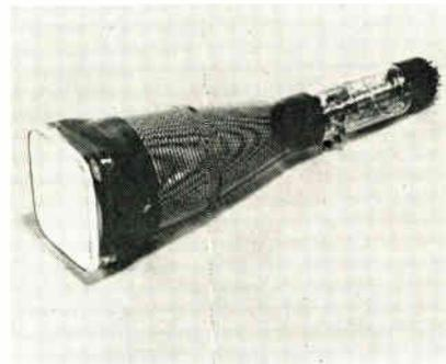
These 2 high sensitivity CRT's, are designated SC-3377 and SC-3511, and feature high deflection sensitivity and a 3 1/2 inch square face for optimum use of display space. Overall tube length is only 13 3/4 in. Typical operating conditions are: A3 voltage—3kc; A2 voltage—1kv; A1 voltage for focus—0-300v; Eco is —30 to —50v; Line width @ Ib3=10µa—0.45mm max; and deflection factors—ID2 is 27 to 33v/in. and 3D4 is 23 to 29v/in. Sylvania Electric Products Inc., 1100 Main St., Buffalo 9, N. Y.
