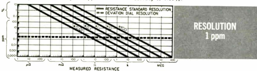
Deviation dial has a resolution of 1 ppm (part per million) for all resistance values. Resistance standard slide wire has 100 microhm per division resolution but can be set to a small fraction of a division. Deviation or resistance dials can be used to calibrate meter sensitivity for even higher resolution.
