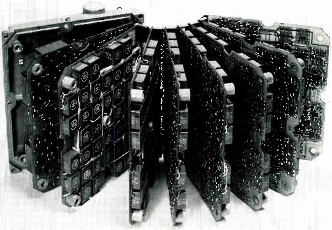
Fig. 2. Control system is packaged for extreme environmental conditions (230°F temperature variation, 6000 Gs shock, free-fall water
