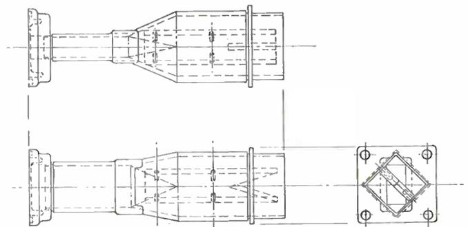
Fig. 6: Drawing of X-band circular polarized antenna.
