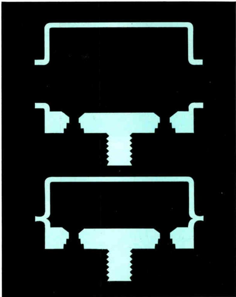
To be Cold-Welded, the flanges of the transistor can must be free of contaminants. The two surfaces are united under evenly distributed high pressure, causing copper molecules to flow together, producing an unbreakable, hermetic seal. Photomicrograph (45X) reveals absence of seam or interface. In addition to photomicrographs, Tung-Sol non-destructively tests weld quality with 100-psi water bomb immersion, mass spectrometer and radioactive tracer tests.
