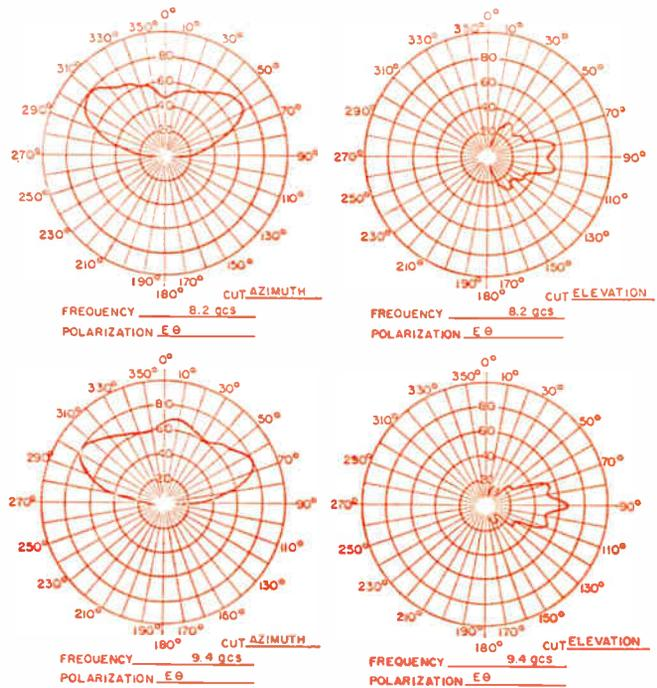
Fig. 8: Radiation pattern data for linear vertical antenna.
