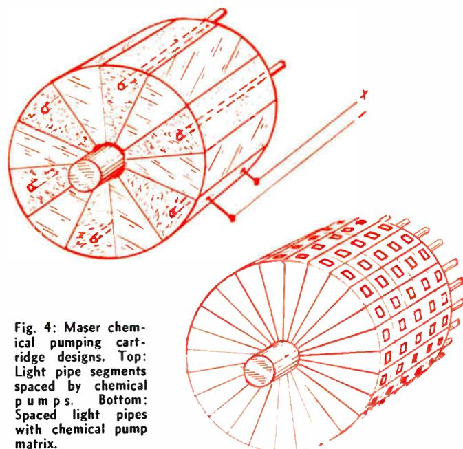
Fig. 4: Maser chemical pumping cartridge designs. Top: Light pipe segments spaced by chemical pumps. Bottom: Spaced light pipes with chemical pump matrix.
