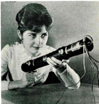
Maureen O'Donnell of RCA's Electron Tube Div., examines a traveling-wave tube that will amplify signals for NASA's relay communications satellite. The 150-lb satellite will be used to investigate global TV.
