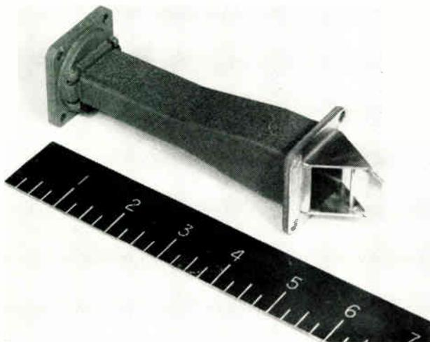
Fig. 2: Photograph of X-band horizontal polarized antenna.
