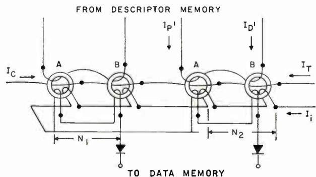
Fig. 6: Detector Coupling Circuit further provides isolation of Descriptor memory storage from Detector circuit interrogation.
