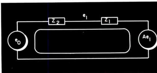
Fig. 3: Equivalent circuit used in the Loop analysis
