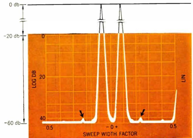
CRT detail of SSB-3b Analyzer shows two-tone test signals deflected 20 db above full scale. Third order IM products at arrows are seen to be 60 db from sideband level.
