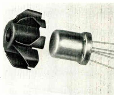
Model 9036 Radiator Holders for R.C.A. Nuistor satisfies need for high efficiency heat dissipator (36°C/watt). In applications where nuistors are mounted on printed circuit boards, the use of a heat dissipator is essential for maximum efficiency and longer life. They are available from stock. Augat Inc., 33 Perry Ave., Attleboro, Mass.
