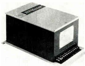
The transducers are designed to convert temp. freq., ac watts, power factor, and ac voltage and current. The temp. transducer is basically a Wheatstone-bridge circuit with a 10 copper resistance-temp. detector as a variable resistance in one of the bridge arms. It is rated for 120v, 60cps operation, with continuous 20% overload capacity. A watt to dc transducer is for applications requiring dc millivolts. General Electric Co., Instrument Dept., West Lynn, Mass.
