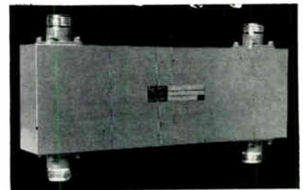
NOW... FOR THE FIRST TIME... a single AEL model HCN, 100 Series, 3db HYBRID COUPLER can be used to cover an extremely wide band, and completely eliminates the need for additional intermediate couplers.
