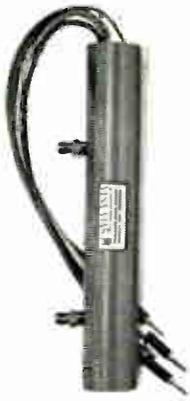
Greater range for ECM and space communications systems is what this new Sylvania traveling-wave tube offers. It is the only PPM-focused tube available with 100 watts minimum CW power, and 30 db gain from 7 to 11 Gc. Key to this performance is a new approach to helix structure which results in effective cooling at high power levels.
