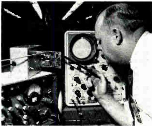
Radio Frequency Fault Detection testing of an F-104 sub-assembly card. Engineer Frank Hagert taps card making fault more apparent. O-scope shows intermittent r-f noise from a faulty diode on card.
