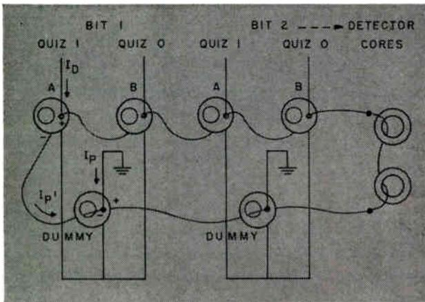
Fig. 3: Descriptor memory has separate drive windings for the transfluxors, but a single output winding in the word direction.
