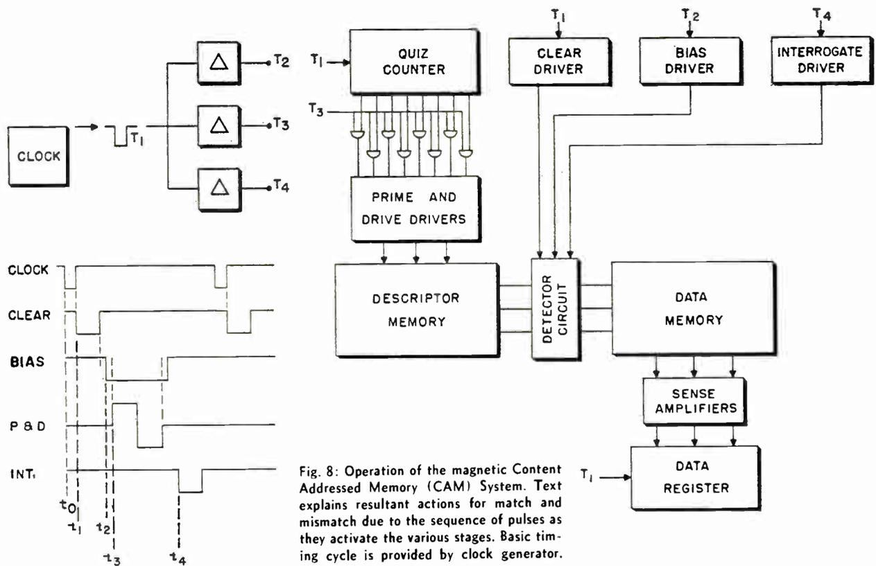
Fig. 8: Operation of the magnetic Content Addressed Memory (CAM) System. Text explains resultant actions for match and mismatch due to the sequence of pulses as they activate the various stages. Basic timing cycle is provided by clock generator.
