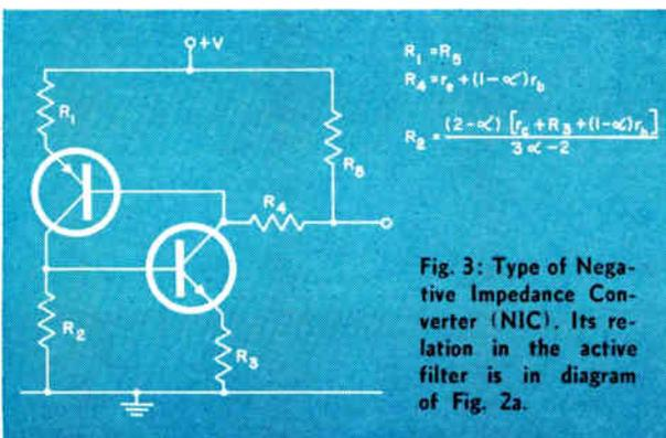
Fig. 3: Type of Negative Impedance Converter (NIC). Its relation in the active filter is in diagram of Fig. 2a.
