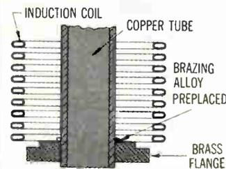
Induction brazing has proved to be an excellent method for production assembly of wave guides. In the diagram, a rectangular copper tube is joined to a brass flange using a pre-placed ring of brazing alloy. Uniform localized heating minimizes distortion. Induction brazing produces consistently sound joints with smooth fillets.
