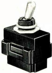
For use in electronic apparatus, test instruments, and communication. The Bulletin 7516 and 7517 feature plug-in terminals, for rapid connection by merely inserting the wire into switch body. Other standard features include: 1 hole insulated mounting with nylon threaded bushing; bussing connection; and semi-dusttight construction. Rated 3 and 5a at 250v, and 6 and 10a at 125v. Cutler-Hammer, 315 N. 12th St., Milwaukee 1, Wis.
