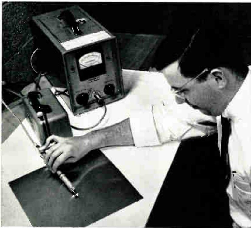
One of the many instruments used by Taylor to check product quality is the Profilometer. Here a quality-control specialist is inspecting surface finish on a composite sheet.
