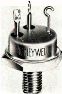
Packaged in a 11/16 inch hex double-ended, gold-plated case, the 10 amp series is offered in two voltage and two gain ranges.  $BV_{CEO}$  is 100 or 80 min.  $BV_{CBO}$  is 80 or 60 min., gain is 20 - 60 or 40 - 120.  $BV_{EBO}$  is 8 min.,  $V_{CE}$  (sat) is 0.5v max. and  $V_{BE}$  (sat) is 1.2v max. @  $I_C=5A$  for all four types. Minneapolis-Honeywell Regulator Co., Semiconductor Products, 2747 Fourth Ave. So., Minneapolis 8, Minn.
