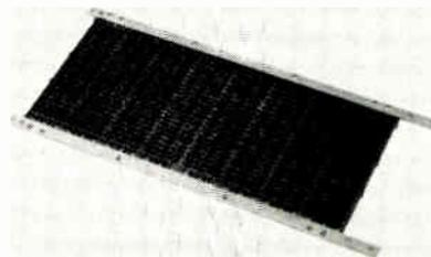
This buss-line wiring technique offers contacts on strips which act as wires, furnished in endless reels, eliminating high cost and unreliability of soldering contacts to wires individually. Buss-lines also speed mass assembly wiring of complex circuitry. Another new product to be shown will be the company's Vari-panels and Series 7028-7029 connectors, applicable to buss-line wiring. Elco Corp., Willow Grove, Pa.
