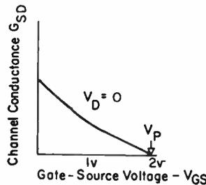
Fig. 3: Channel conductance varies with gate-to-source voltage.
