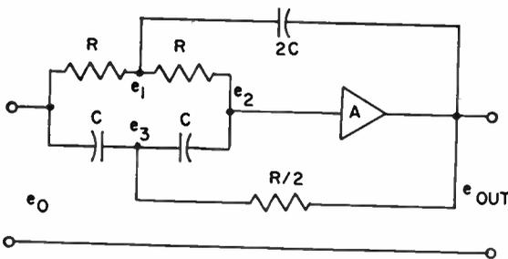
Fig. 7: Active RC notch filter
