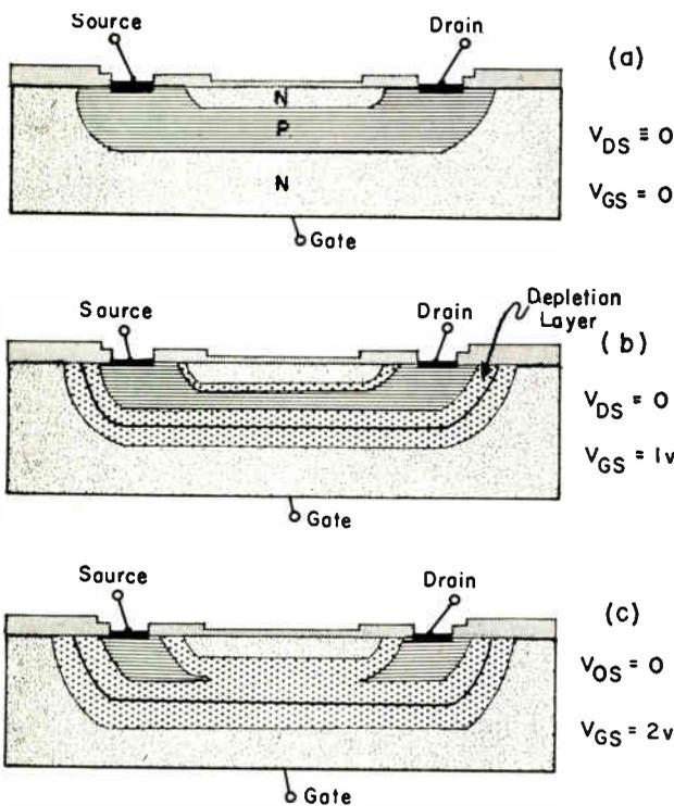
Fig. 2: Increasing the depletion layer width decreases the effective channel thickness  $T$ , and reduces channel conductance  $G$ .
