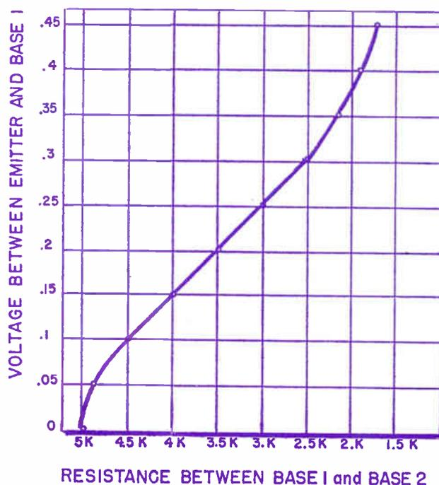
product is zero. If the No. 2 input voltage is made positive, the resistance of the unijunction transistors decreases, thereby unbalancing the bridge in one direction. If the No. 2 input voltage is made negative, the resistance of the bridge is unbalanced in the opposite direction.
