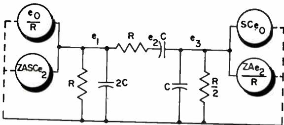
Fig. 8: Node equivalent circuit of the circuit above
