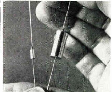
Solid tantalum with ratings from 6 to 35v. They are polar types for use with a dc bias exceeding peak value of the ac component. Rated from 0.033 to 330 $\mu$ f; will withstand operating temps. from  $-55^{\circ}$  to  $+125^{\circ}$ C. Standardized into 4 case sizes ranging from 0.250 to 0.750 in. long and 0.125 to 0.341 in. dia. Standard units hermetically sealed in a plated metal case with a glass-to-metal seal. Rectifier-Capacitor Div., Fansteel Metallurgical Corp., No. Chicago, Ill.
