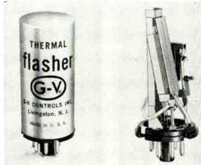
Type DF 9000 Series Flasher combines the principles of differential expansion and snap-action for rapid stabilization. Standard flashing rates of 1 to 60 cycles-per-minute and heater voltages of 6.3, 12, 28, 48, and 115vac or dc available. The on-off flashing ratio can be factory-set for ratios of 50:50 to 80:20. Contact rating is 3a to 250vac, 1a resistive to 32vdc. Life 1,000,000 cycles minimum. Measures 2 3/4 in. high and 1 1/4 in. in dia. G-V Controls Inc., 101 Okner Pkwy., Livingston, N. J.
