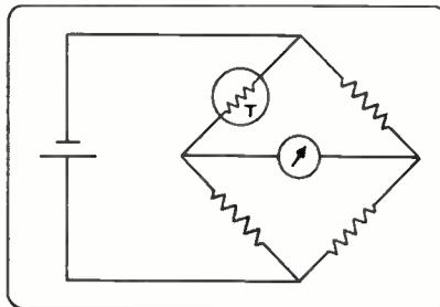
Typical thermistor temperature indicator circuit (simplified). Such units can indicate to a precision of .001° F. operating mode is useful in such devices as voltage regulators, microwave power meters, gas analyzers, vacuum gauges, flow meters and automatic volume and power level controls. By using appropriate circuitry almost any desired time lag may be introduced in the response of self-heated thermistors, which makes them useful in time delay and surge suppression applications.
