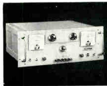
Outputs are wide range, 0-32, or 0-60v, at 0-5, 0-10, 0-15, or 0-30a. Features include auto-crossover from constant-voltage to constant-current or vice versa, with adjustable limiting in either mode inherent in operation. Other features include programmability in c-v or c-c output modes; Mhogrammability, the conductance-programming technique; master-slave series or parallel operation; 0.01% or 2mv line or load regulation in constant-voltage. Electronic Measurements Co., Eatontown, N. J.
