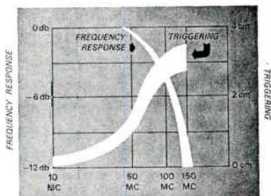
Typical frequency response and triggering characteristics of 580/82 combination—showing minimum number of centimeters necessary for triggering.
