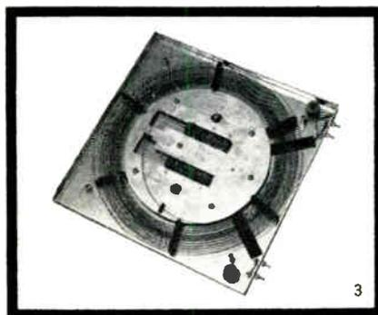
**3 WIRE SONIC DELAY LINES** provide low insert losses, higher storage rates, and reliable operation—even in severe vibration environments. Sonic delay lines are available in special designs to meet a wide range of requirements. Applications include computer serial memories, buffer data storage, and signal processing. Input/output circuitry is furnished where desired.
