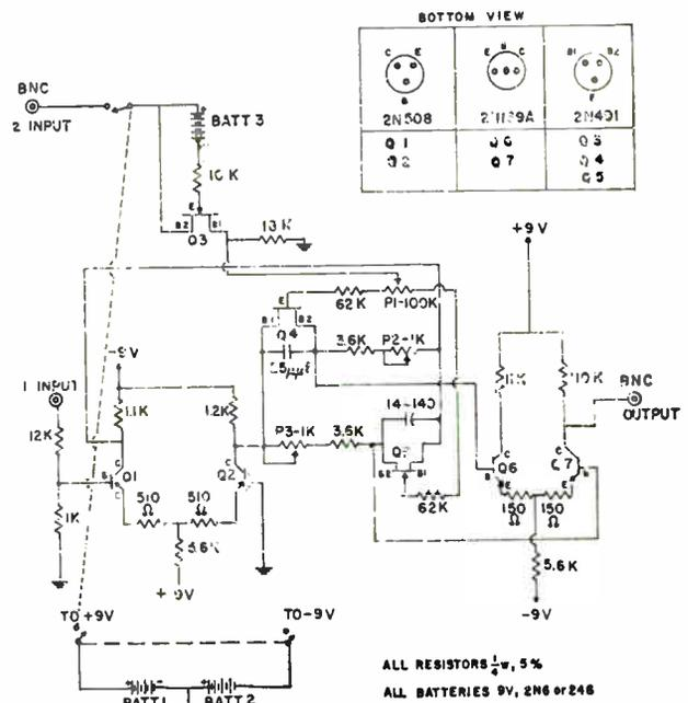
Fig. 3: Schematic diagram of the transistor multiplier. This device offers four quadrant electronic multiplication.
