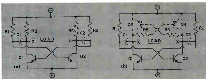
Fig. 1: The component parts common to both the (a) conventional astable and (b) complementary-symmetrical astable multivibrators: R1, R2, C1, C2, Q1 & Q2.
