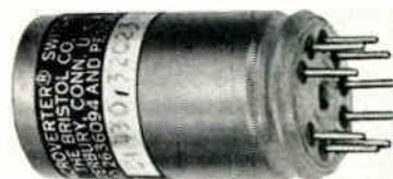
For example, the Miniature DPDT Chopper operates at 400cps. Action is "make before—break after." Tracking is very good; the maximum difference in phase lag is 3°. Vibration limit is 3g's, 0-2000cps. The Bristol Co., Waterbury 20, Conn.
