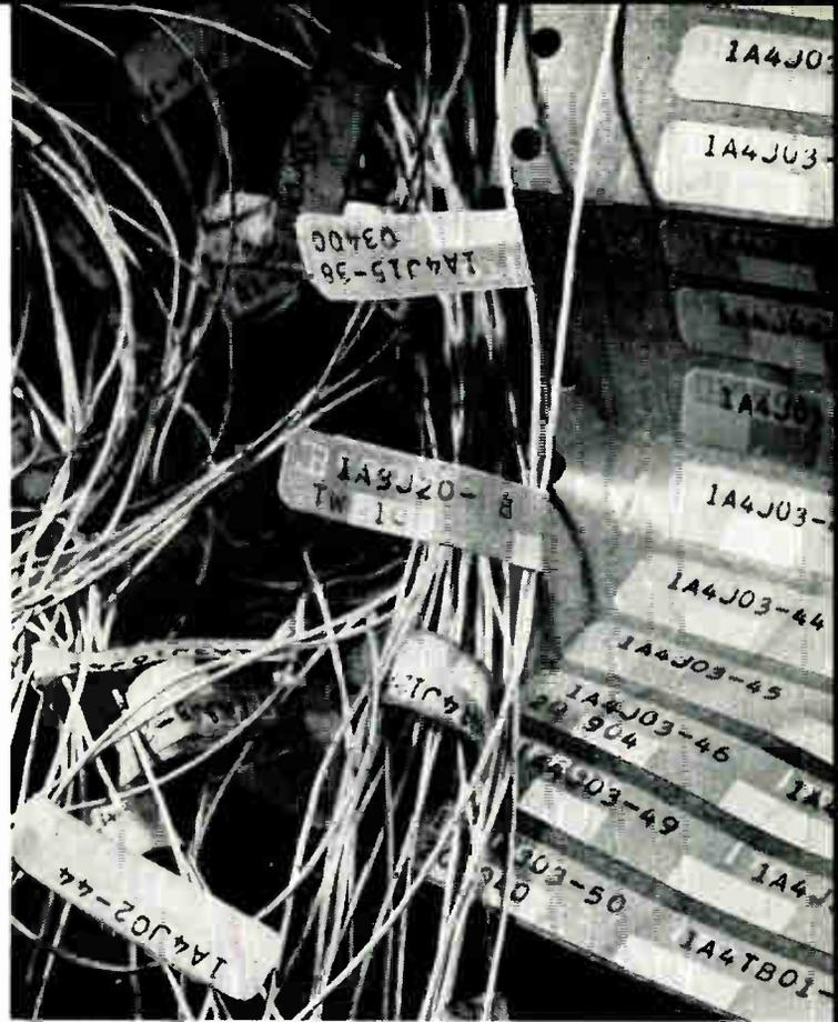
Wires are labeled by signal function. The labels are attached by hand pressure.
