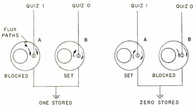
Fig. 2: Basic memory storage device for the non-destructive interrogation of a stored One or Zero. The transfluxor can be interrogated in one of two stable states, blocked or set.
