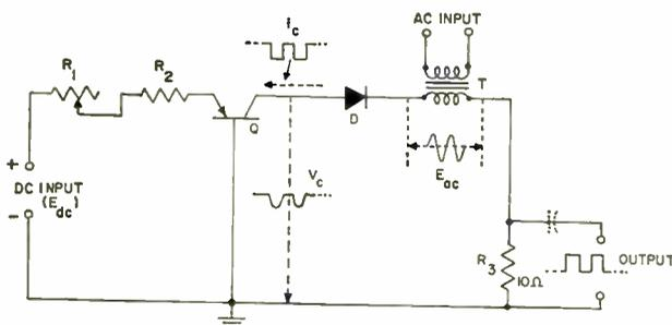
governed by the applied emitter-base dc voltage,  $E_{dc}$ , and thus to flow as square waves ( $i_c$ ). These current pulses develop a square-wave output voltage across the low resistance  $R_3$ .
