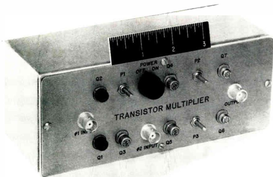
Photograph shows the electronic multiplier. Compact unit has all switches, inputs and transistors mounted on the front.
