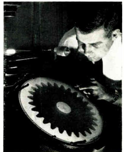
Nylon gear of planetary gear system magnified 20 times. System used in motor-driven type Volt-Pac variable transformers.
