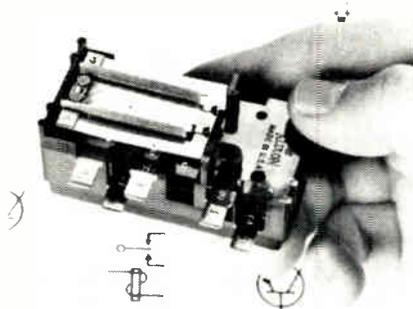
Now being used in time delay systems for electronic tube protection and alarm systems. The KLIXON® 59000 Series is available with SPDT or SPST switching and has an average inherent response time of 26 sec. (ON) and 50 sec. (OFF). It handles 25a, 240v; 120v resistive load, and costs less than magnetic relays. It is sensitive to low-power output of transistors, rectifiers, thermistors and other sensors. Metals & Controls Inc., Div. of Texas Instruments Incorporated, Attleboro, Mass.
