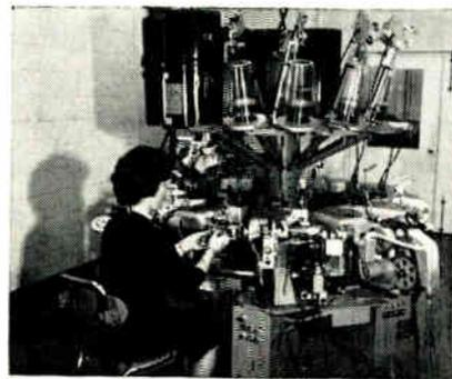
No. 116 features labor-saving devices to reduce handling costs from 66 to 75%. Such operations as taping the start lead, taping or waxing the finished coil, cutting the wire, ejecting the coil and sorting 2 different coils are all automatic on the No. 116. All the operator has to do is load the coil and attach the wire. The Automatic Bachi Bobbin Winder is manufactured with 6, 8, 10, or 12 individually operated winding heads. Leesona Corp., 333 Strawberry Field Rd., Warwick, R. I.
