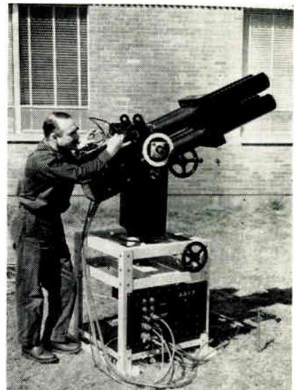
Optical photometer to detect presence of nuclear debris from high-altitude explosions is checked by Dr. E. Manning, of Geophysics Corp. of America, Bedford, Mass., developer of equipment. Rapid-response photometer observes and records fast intensity changes in four spectral regions simultaneously.
