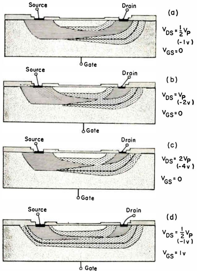
Fig. 4: Effects of varying gate-to-source and gate-drain-to-source  $V$ .
