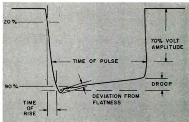
Fig. 3: Typical modulator pulse shape characteristics.
