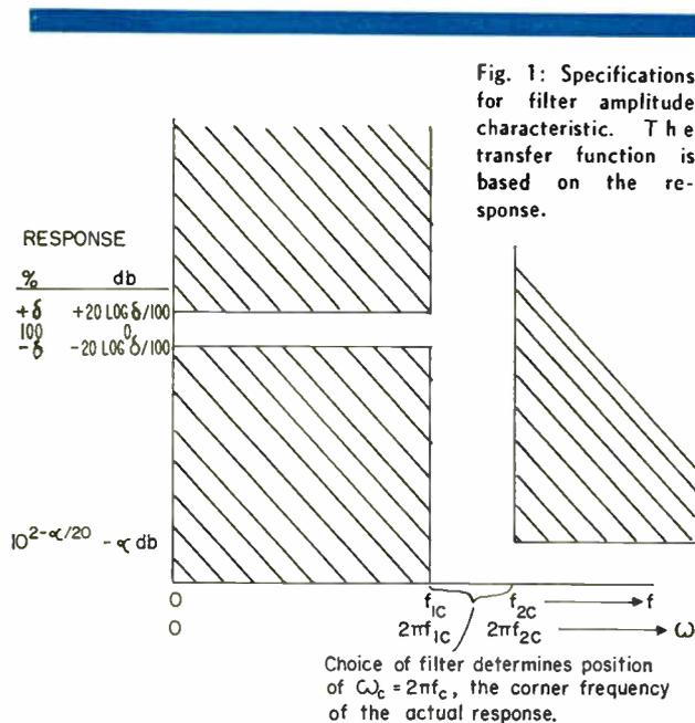
1.  $\delta\%$  transmission inaccuracy from dc (0 cps) to  $f_{1c}$  cps.
