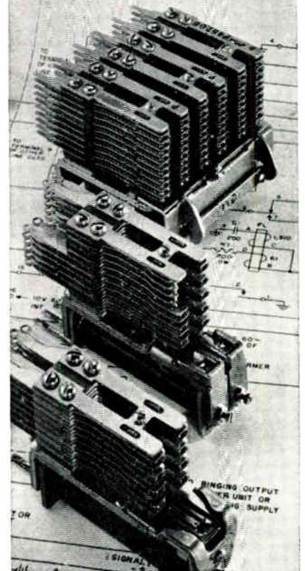
The sound design and long, reliable life of these Stromberg-Carlson relays have been proved by many years of successful use in the exacting field of telecommunication:
