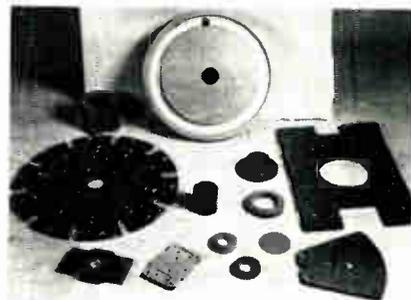
Micaceram retains its properties in applications where temperatures go as high as 1800°F. One of its outstanding features is the ease of machining this material. It is either purchased in a slab and machined by the customer, or M.D.I. will machine it. The material is then purchased in its final form and no firing is necessary after machining. It has a low loss factor and is non-out gassing. Molecular Dielectrics, Inc., 101 Clifton Blvd., Clifton, N. J.
