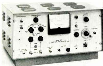
Useful in the microwave area for measuring the gain of pulsed tubes and the power levels in pulsed r-f systems. Model 405 is also useful in metering pulse droop in microwave systems or absolute pulse levels in digital systems. Instrument is furnished with a flat crystal detector which monitors the r-f power by means of its detected output. The sampling time is set by means of a variable sampling delay circuit. Wiltron Co., 717 Loma Verde Ave., Palo Alto, Calif.
