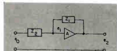
Fig. 2: Node equivalent circuit
