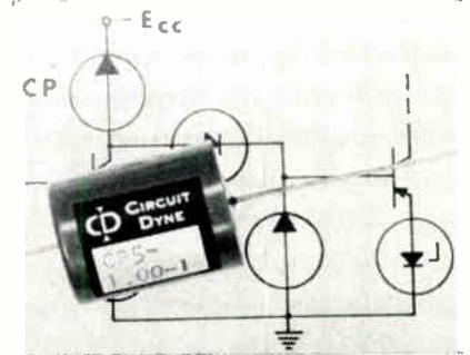
The CP-5 "Corrector" current regulator is a 2-terminal, solid state component, capable of maintaining a current value within ±2% of its rated value up to 25v. The CP-5 is a polar type; a non-polar version, the CN-5 is also available. It is available with current ratings from 1.0 to 20.5ma in 5% increments. Measures 0.8 in. dia. x 1.05 in. long and is packaged in a rugged epoxy-filled dp case. Leads may be specified axial or single-ended. CircuitDyne Corp., 480 Mermaid St., Laguna Beach, Calif.
