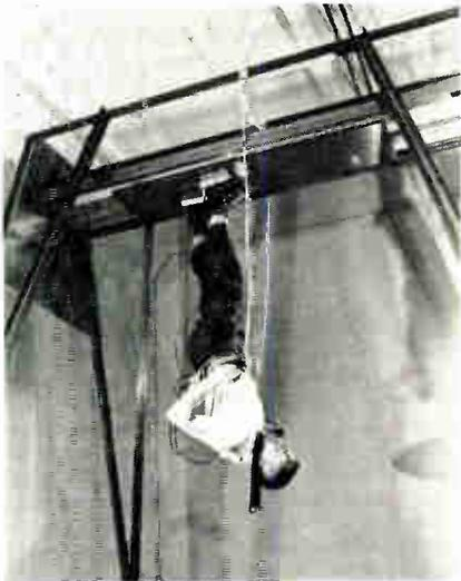
Ceiling walker shows how new Westinghouse magnet combining advantages of permanent and electromagnet works. It can be turned on and off, allowing steps to be taken. Magnet has a "memory," exerting pull in same direction until reversed. Ceramic magnet is between 2 soft steel layers. Electrical connection at one pole causes flux transfer, reversing polarity. Shoe's pull is 30-50 lbs.
