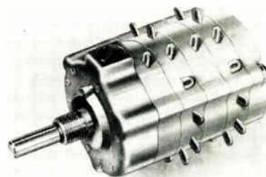
The Series 700 rotary switch also features: fully enclosed 1½ in. diameter; a variable detent action; positive positioning; 12 contacts in either nickel silver or coin silver rated 5a @ 115vac res.; 3a @ 28vdc res., and 2a @ 28vdc ind. It also included 3 solder lugs on common ring wafer instead of the usual 1 lug construction. Vemaline Products Co., Switch Div., Box 1, Franklin Lakes, N. J.
