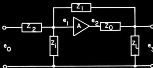
Fig. 4: Amplifier with feedback, considering impedances.
