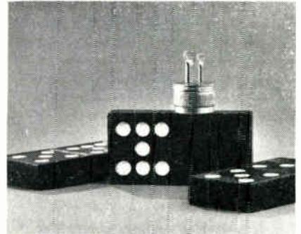
The ZJ265 is for use where the max. device temp. can be kept below 100°C. Applications include: relay replacement; motor speed controls for hand tools; and appliance controls. For automatic assembly in large volume, the silicon controlled rectifier is in the popular cup-type package which can either be pressed, soldered or clipped onto a suitable heatsink. A stud mounted version will also be available (ZJ226). General Electric Co., Rectifier Components Div., W. Genesee St., Auburn, N. Y.
