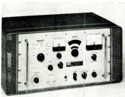
Measures bandwidth, sensitivity, and distortion of FM telemetry receivers in the 225 to 800mc range. AMI Model 303 FM, features a carrier freq. tunable from 225 to 800mc in 2 bands with freq. stability of  $\pm 0.005\%$  and calibration accuracy of  $\pm 0.5\%$  receivers. Three FM deviation ranges are: 0-30, 0-100, and 0-300kc, with  $\pm 5\%$  FSD on all ranges from 225 to 400mc, and  $\pm 10\%$  FSD from 400 to 800mc. Advanced Measurement Instruments, Inc., 109 Dover St., Somerville 44, Mass.
