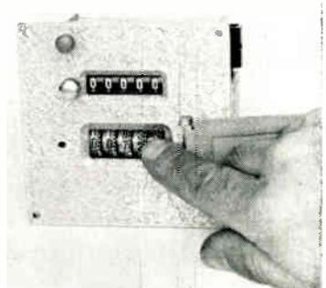
This is a differential impulse counter capable of counting up or down and accepting simultaneous adding or subtracting pulses at a rate up to 15/sec. with push button reset. It has 2 sets of contacts, one of which is closed when the counter passes through 0 and one at a variable pre-set point. Pre-setting may be any number within the total 5 digit capacity of the unit. Front panel dimensions are 3¼ x 3¼ x 3½ in. deep. Presin Co., Inc., 226 Cherry St., Bridgeport 5, Conn.
