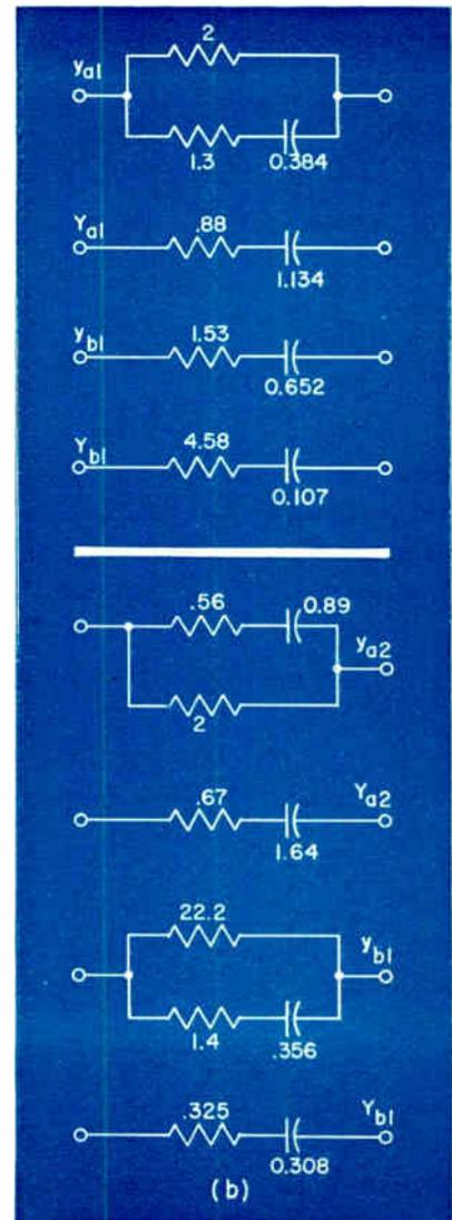
Fig. 2b (right): Scheme of resultant values of components required in corresponding admittances shown in (a).
