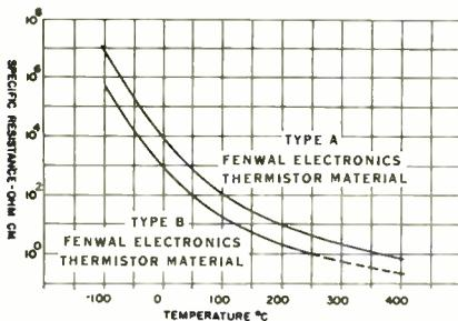
Change in resistance with temperature of two typical Fenwal Electronics thermistor materials.
