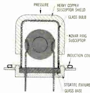
Holders for quartz crystals are sealed by induction heating in an evacuated bell-jar. A glass-coated kovar metal ring is used as a susceptor between bulb and base. Steatite nest, held in plate-type induction coil positions glass base, while spring-loaded copper block locates glass bulb and also provides pressure to cause plastic flow of glass after localized heating. In production, several crystals are sealed at one time.
