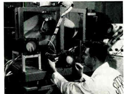
Sperry Gyroscope Co. technician Conrad Hansen performs tests on one of a number of radar sets being made for Air Force. Called the APN-59, the radars can handle search surveillance, storm detection and other all-weather navigation work.
