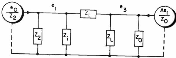
Fig. 5: Node equivalent circuit
