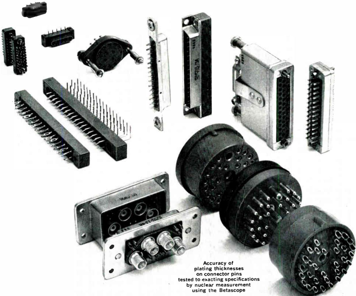
Accuracy of plating thicknesses on connector pins tested to exacting specifications by nuclear measurement using the Betascope
