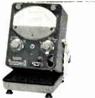
Type 1806-A Electronic Voltmeter also has ac and dc voltage ranges to 1500v. As an ohmmeter it measures resistances from 0.2Ω to 1000megs. Input impedance for dc measurements is 100megs; for ac, 25megs in parallel with 2pi, except 25megs in parallel with 15pi on highest 1500v range. Open-grid dc measurements possible up to 150v. Includes a new, small-sized probe for use in limited space. For quickest readout, only 2 voltage scales appear on large panel meter. General Radio Co., W. Concord, Mass.
