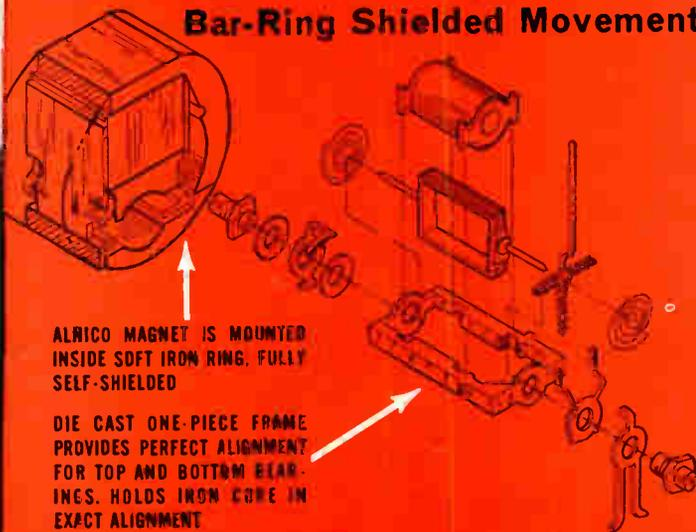
ALRICO MAGNET IS MOUNTED INSIDE SOFT IRON RING, FULLY SELF-SHIELDED
