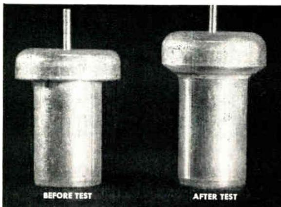
**Crimp-sealed Fansteel tantalum capacitors stay leak-proof\* even in outer space**
