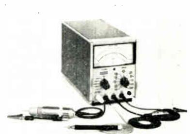
Model 410C will measure dc voltage ( $\pm 2\%$ ) from 1.5mv to 1500v; dc current ( $\pm 3\%$ ) from 0.15ma to 150ma and resistance from  $0.2\Omega$  to 500megs. With an optional plug-in probe, ac voltages (20cps to 700mc) from 50mv to 300v may be measured. Floating dc voltages to 400v above instrument ground measured with complete safety. High sensitivity and low noise permit use as a preamplifier for analog recorders. Hewlett-Packard Co., 1501 Page Mill Rd., Palo Alto, Calif.
