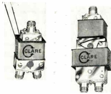
Display very low crosstalk, vswr, and insertion loss for a variety of switching operations, at freqs. up to 700mc, applications include: i-f switching in microwave networks; transmit-receive antenna switching in the uhf range of 100-500mc; and switching PCM data in telemetering systems without deterioration of square wave form. Two types are available—the HGS2C (left) coaxial relay displaying crosstalk isolation of 80db min. C. P. Clare & Co., 3101 Pratt Blvd., Chicago 45, Ill.
