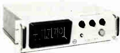
The RV2 also offers high speed, automatic range and polarity changing, and the reliability of hermetically-sealed reed relays. Speed is 4 readings/sec., average. Ranges of the DVM are  $\pm 9,999, 99,99, 999,9v$ . Accuracy is  $\pm (0.01\%$  of full scale  $+1$  digit), and resolution is  $\pm 1$  digit. Input resistance is 10megs. Input circuits are completely isolated from the chassis. An LC filter attenuates input signal noise. Non-Linear Systems, Inc., Del Mar, Calif.
