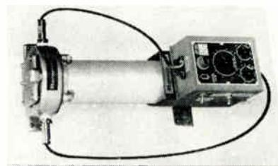
Model PL- $\frac{1}{2}$  Repurification Loop is a compact model designed for smaller cooling systems that hold up to 150 gal. of coolant. The Barnstead PL- $\frac{1}{2}$  loop continuously repurifies the coolant while the tube is in operation and prevents build-up of scale, copper oxide, carbon dioxide, oxygen, organics and other impurities which cause corrosion or impair heat transfer and needlessly curtail tube service life. Barnstead Still and Sterilizer Co., Boston 31, Mass.
