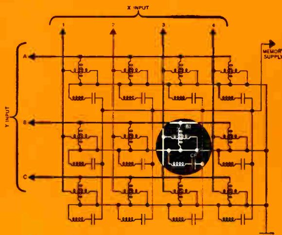
**NOTE:** Each crosspoint of a Clareed Single-Mode Memory Matrix consists of one or several Clareed switches enclosed in each of the multiwound coils shown.
