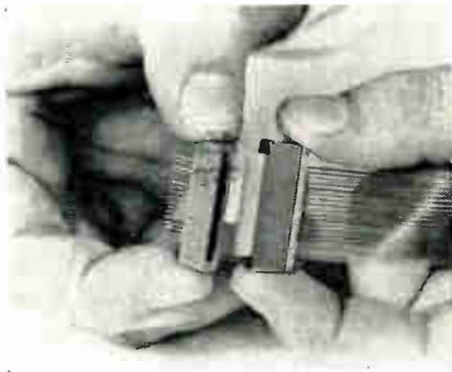
Developed for sizes of cable in accordance with the IPC standard, this connector allows 19 connections to be made in 19 sec. This connector has been designed specifically for use with flat flexible cable. The TAPECON connector has designs for use in applications for tape-to-wire, tape-to-tape, tape-to-miniature round (Mil-C-26482) connector, and tape-to-printed circuit board. Contact in the connector is accomplished through insulation "milling." Burnly Corp., Norwalk, Conn.
