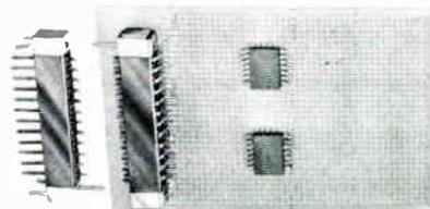
These plug-in boards, for integrated-circuit fabricating, are 1/32 in. thick pre-punched epoxy glass with 0.025 in. dia. holes on 0.05 in. C-to-C spacing, or 0.042 in. dia. holes on 0.1 in. spacing. Plugboards have micro-miniature connector with 9, 12, or 15 contacts. Matching receptacles for mother board mounting are also offered. Vector Electronic Co., Inc., 1100 Flower St., Glendale, Calif.
