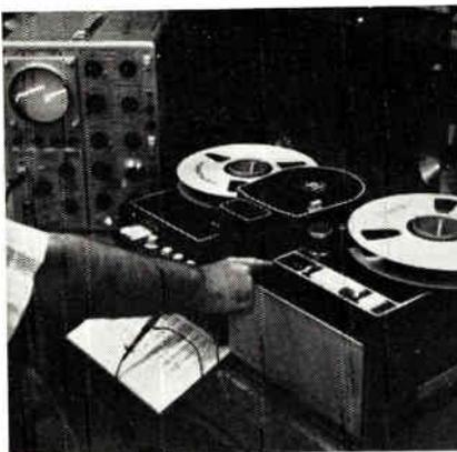
By recording hf signals, then reproducing them in its stop-motion mode, a 75-lb. TV tape recorder makes it practical to study a wide variety of transients without need for loop recorders and readout devices, or related equipment. Technician (above) stops tape on Precision Instrument Co.'s PI-3V recorder to show recorded transient signal.
