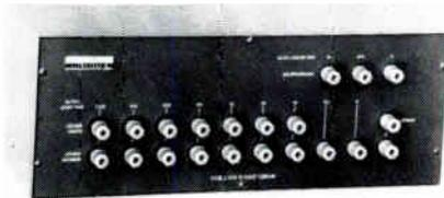
Model 2851 is a 17 lb. instrument for rack mounting or bench use. It has separate working and guard circuits. Input working taps are 3, 7.5, 15, 30, 75, 150, 300, 750 and 1500v.; input guard taps are 15v. and above. Guaranteed error limit for the volt box is  $\pm 0.005\%$ . Calibrated accuracy is  $\pm 0.002\%$ . The instrument is thermally and electrostatically shielded. Honeywell, Denver Div., 4800 E. Dry Creek Rd., Denver, Colo.
