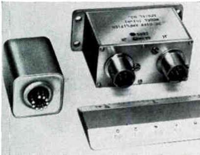
The FA1-A1 provides a  $\pm 5$ vdc (or 10v.) full-scale output from the low mv signals originating from strain-gage type transducers. Continuously adjustable zero balance and gain from 20 to 1000 is available. It contains a highly regulated transducer power supply, reverse polarity protection, input-output isolation and RFI filter. Fairchild Controls, Div. of Fairchild Camera and Instrument Corp., 225 Park Ave., Hicksville, N. Y.
