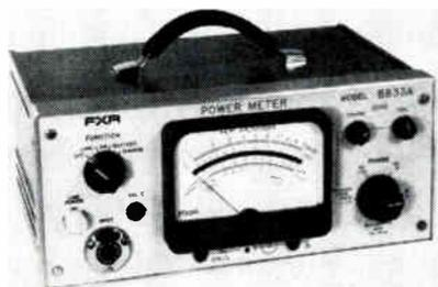
Model B833A uses a dc self-balancing r-f bridge for accuracies of 0.15% @ 10mw or 1.5% @ 1mw. The unit eliminates subtle errors associated with audio power in r-f bridges. Features include: a single zero adjustment; availability of thermistor heads at freqs. from 10mc to 40cc. It is lightweight and portable with optional rechargeable battery. FXR, 25-15 50th St., Woodside, N. Y.
