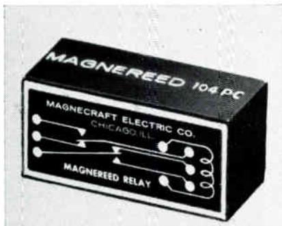
The class 104 encapsulated dry-reed assemblies have preadjusted gold contacts hermetically sealed in inert gas. The spdt units operate in 1msec. and release in 1msec. Contacts are rated 3va @ 0.25a. Life is 10 million cycles. Magnecraft Electric Co., 5575 N. Lynch, Chicago, Ill.
