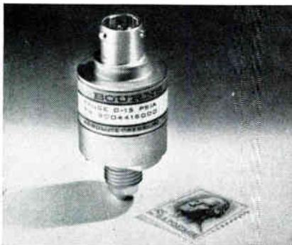
Model 441 operates over pressure ranges of 0-5 to 0-450 psia. Flex-pivot construction virtually eliminates mechanical friction and enables resolution of 0.5%. Other features include ultra-reliable potentiometric elements; hermetic seal construction; and optional LOX-clear compatibility in all pressure ranges. Bourns, Inc., 1200 Columbia Ave., Riverside, Calif.
