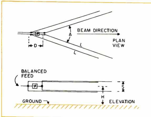
Fig. 3: Basic single-unit horizontal rhombic antenna.
