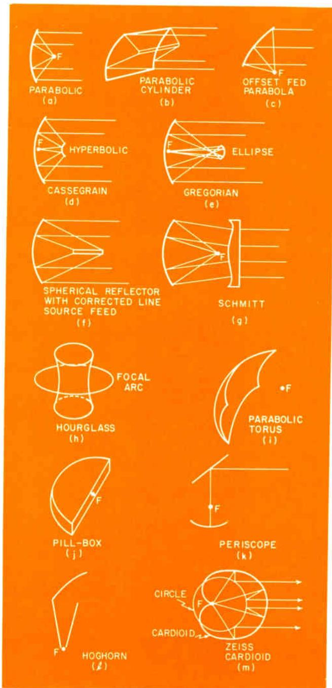
Fig. 1: Some of the possible antenna reflector forms.
