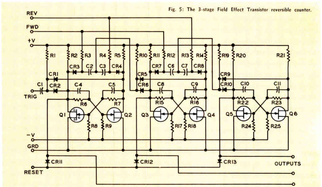
Fig. 5: The 3-stage Field Effect Transistor reversible counter.
