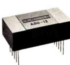
**Differential Amplifier—ADO-12** DC Voltage Gain = 30,000. Voltage Drift =  $3\mu V/^\circ C$  (max.). Differential Voltage = 5V (max.). Gain Bandwidth Product = 1.6Mc (min.). Full compliance with MIL-D-16400 and MIL-E-5400. (Specify part number ADO-12M for 12V/ $\mu$ sec slewing rate.) Dimensions:  $1'' \times 1\frac{1}{4}'' \times 1\frac{1}{2}''$ . Price: \$450.
