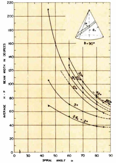
Fig. 8: Typical half-power beamwidths for conical
