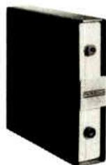
**Operational Amplifier—ADO-7** Photo-resistor chopper stabilized operational amplifier. DC gain over  $4 \times 10^7$  (min). Gain bandwidth product = 1 mc (min). Output =  $\pm 100V$ . Drift  $< 1\mu V/^\circ C$ . Maximum Load Current = 10mA to ground at  $\pm 100V$ . Short Circuit Proof. Slewing rate  $> 10V/\mu sec$ . No chopper drive required. Low noise. Dimensions:  $4\frac{3}{4}'' \times 1\frac{1}{4}'' \times 5''$ . Prices: 1-4, \$195; 5-9, \$182; 10-24, \$172; 25-99, \$164.
