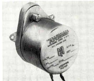
Series 44600 rotation is unidirectional, either clockwise or counterclockwise, as required. The rotor shaft rotates in discrete 15° steps, and at rates up to 4800 steps/min. Positive magnetic detenting occurs at each of 24 angular rotor positions. Stepping action is obtained by applying dc pulses alternately to 2 stator coils. Operating voltage is 27vdc ±10° in standard models. The A. W. Haydon Co., 232 N. Elm St., Waterbury, Conn.
