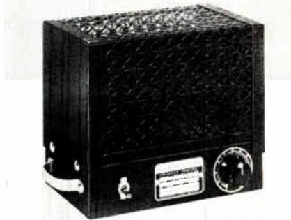
The Change-A-Cycle device uses a principle entirely different from conventional motor-generator devices. The ac input (from 25 to 400 cps) is first rectified to dc. It is then filtered and fed to a rotary dc to ac converter which, in turn, produces either 50 or 60 cps current. Standard units operate from single phase input and deliver single phase output. Units are available with up to 2kw outputs. Carter Motor Co., 2760A W. George St., Chicago, Ill.
