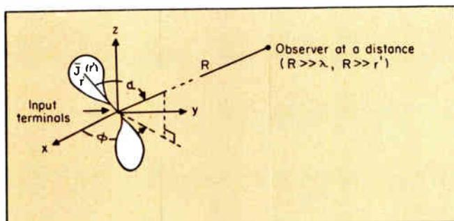
Fig. 2: Receiving ant. in field of elliptically polarized wave.
