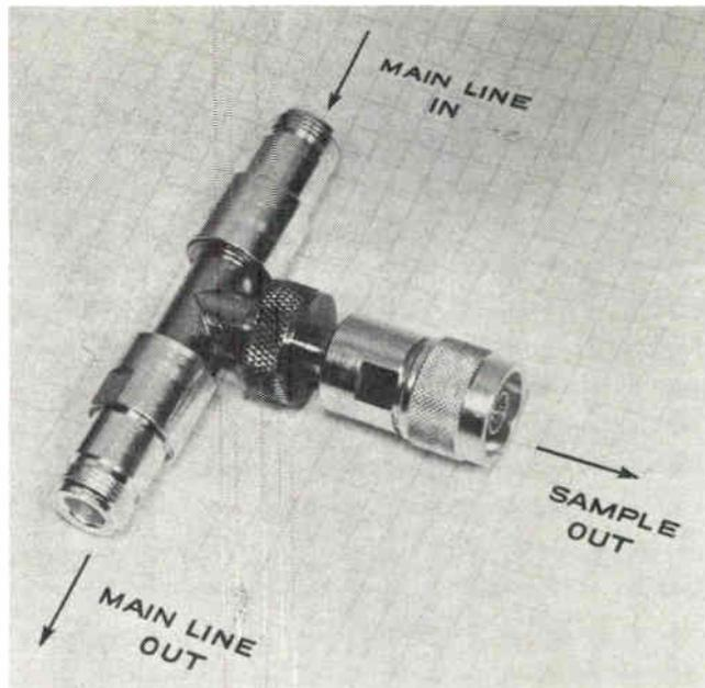
For freq. sampling and power monitoring, TSS-1 has N male and female connectors for attachment to main line or off line.
