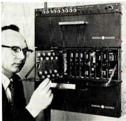
U. S. General Services Administration now using this solid state command terminal in Federal Telecommunications System in Boston area. Designed by General Electric, it provides switching, signalling, and audio amplification for two-way communication manual or direct-dial radiotelephones and landlines.
