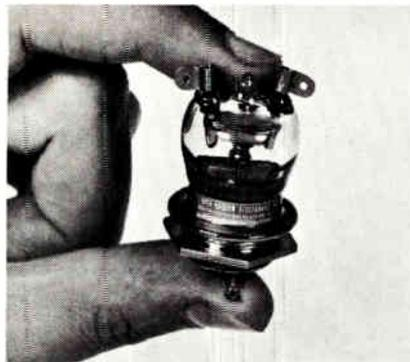
Stubby 1 3/4 in. vacuum relay switches 15 kvdc. Mfd. by High Vacuum Electronics
