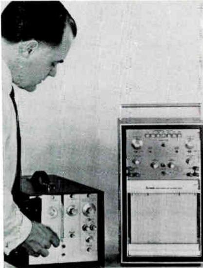
Full-floating, 500  $\mu$ v. level, high-voltage dc preamplifier that accepts microvolt level signals up to 1000v off-ground on low-level channel, or a potential difference up to 1000v dc. on high level has been developed by Brush Instruments, Clevite Corp. Amplifier, recorder and system monitored are all protected by current limiters and over-voltage devices. Unit insures noise-free operation.
