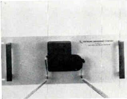
The EECO 5000 Photoblock Readers can control any automated punched tape programmed system. Typical uses include automatic test equipment, ground support systems, machine tool control, and manufacturing process control. Each signal output is capable of switching up to 100ma from either plus or minus logic levels, or from relay loads depending upon output option selected. The unit has no clutch, brake or pinch rollers. Electronic Engineering Co. of Calif., 1601 W. Chestnut Ave., Santa Ana, Calif.
