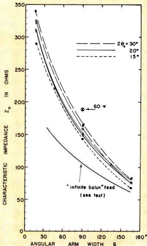
Fig. 10: The input impedance of the conical spiral antenna is mainly a function of the angular arm width.
