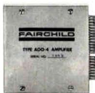
**Operational Amplifier—A00-4** Solid state, chopper stabilized. DC gain over  $5 \times 10^6$ . Gain Bandwidth Product=2 megacycles. Output =  $\pm 20$ V @ 2mA;  $\pm 10$ V @ 7mA. Drift less than 10 $\mu$ V/ $^{\circ}$ C. from -20 $^{\circ}$ C. to +85 $^{\circ}$ C. Plug-in case 4" x 5" x 1". P.C. edge connector. No chopper drive required. Prices: 1-4, \$92; 5-9, \$86; 10-24, \$81; 25-99, \$77.
