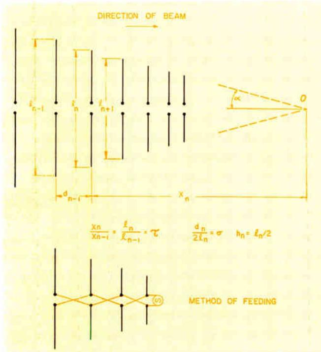
Fig. 1: A schematic of the LP antenna, with symbols used.
