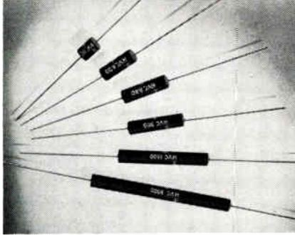
These high voltage cartridge type silicon rectifiers have avalanche characteristics which provide built-in protection against transient overvoltages. Dc ma range from 250 to 50, depending on the voltage. Max. forward voltage drop at rated current ranges from 4v. for the smaller units to 50vdc for the largest type. Sarkes Tarzian Inc., Semiconductor Div., 415 College Ave., Bloomington, Ind.
