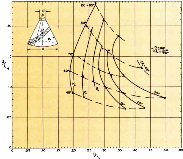
Fig. 7: The factors determining log-spiral antenna frequency ranges.
