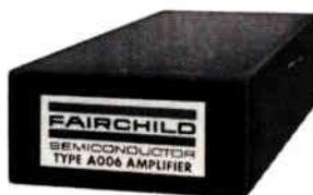
**Operational Amplifier—A00-6** Photo chopper stabilized. DC gain over  $10^7$ . Gain Bandwidth Product = 1 megacycle. Output =  $\pm 25$ V @ 5mA. Drift less than 0.5 $\mu$ V/ $^{\circ}$ C. from 0 $^{\circ}$ C. to +55 $^{\circ}$ C. Long term drift 1 $\mu$ V per week. Plug-in case, precision connector; 1 $\frac{1}{2}$ " x 3" x 6". No chopper drive required. Prices: 1-4, \$230; 5-9, \$215; 10-24, \$203; 25-99, \$192.
