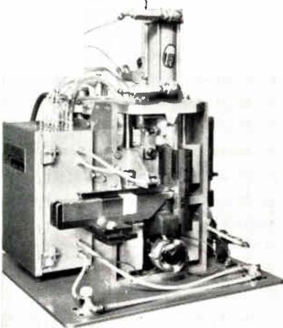
Model PCR-20 Automatic Coil Retainer Inserting Machine allows 1 operator to insert the coil retainer, stamp identifying numbers, secure the leads, and perform the final forming of the end turns at rates of up to 400 fields/hr. Designed for both machine wound and hand inserted fields, it handles stack dia. up to 6 in. and stack heights up to 3 1/2 in. The standard machine uses preformed coil retainer material. Possis Machine Corp., 825 Rhode Island Ave. So., Minneapolis, Minn.
