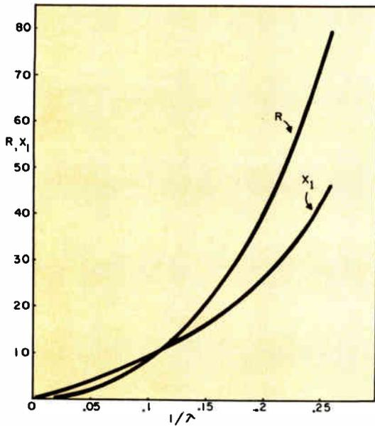
Fig. 3 (left): R and X<sub>1</sub> of a linear antenna.
