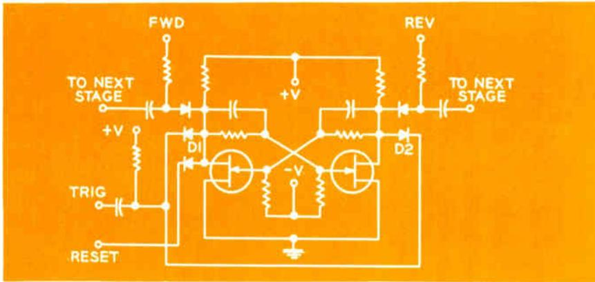
Fig. 4: Typical schematic for the logic diagram shown in Fig. 3.
