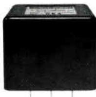
**Differential Amplifier—ADF-1** Drift=1 $\mu$ V/ $^{\circ}$ C. from 0 $^{\circ}$ C. to +60 $^{\circ}$ C. Noise less than 5 $\mu$ V/p-p. Common mode rejection=90 db @ 60 cps; 100 db @ DC. Fixed gain=1000. Size = 1 $1\frac{1}{2}$ " x 1 $1\frac{1}{2}$ " x 1 $\frac{1}{2}$ ". Output=20V/p-p @ 1mA. Pre-aged—100 hour operational test. Prices: 1-4, \$190; 5-9, \$177; 10-24, \$167; 25-99, \$160.
