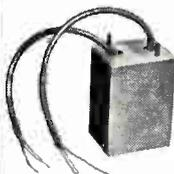
Magnetic shielded plus electrostatic shield for voltage isolation of 2x10<sup>4</sup>. Primary 200K C.T. to within 0.1%. Secondary 50K.
