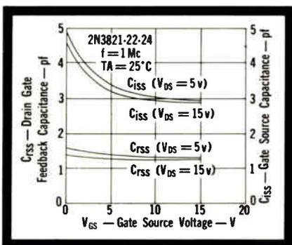
Figure 2. Important capacitance curves for 2N3821, 22, 24 transistors
