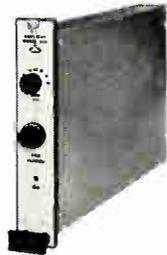
**Model 885-235 Differential Amplifier** to drive data systems, long lines and galvanometers.
