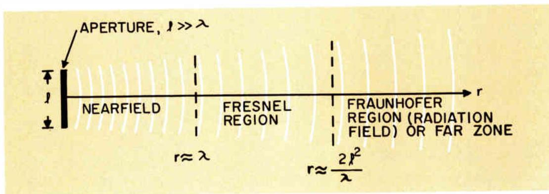
Fig. 4: Fields from a large aperture antenna.
