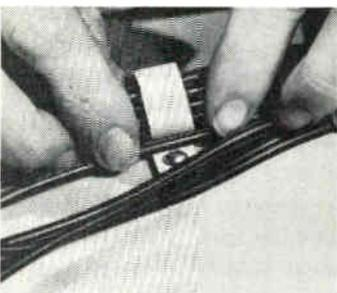
Ideal for supporting long runs of cable in point-to-point wiring. This clamp, TC70 series is available in 5 sizes to accommodate bundles from 1/4" to 1 1/2" in diameter. Wire bundles are quickly snapped into place after the clamps have been mounted in position. These clamps are not only recommended for permanent wiring, but also as a handy device for temporary wiring and bread boarding.
