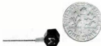
Model 2222 piezoelectric accelerometer is 0.25 in. hex x 0.20 in. high. Its light weight, 0.5 gram, permits measurement of the motion of circuit boards, components, airframe skin and other lightweight structures with negligible loading effects from its own mass. This transducer is adhesive mounted and it is optimized for operation with both charge and voltage amplifiers. Endeveco Corp., 801 S. Arroyo Pkwy., Pasadena, Calif.
