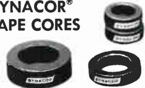
Square loop tape cores manufactured with high permeability alloys, designed for use in critical non-linear magnetic components. Applications in magnetic amplifiers, saturable reactors, d-c to d-c and d-c to a-c converters and specialty transformers.
