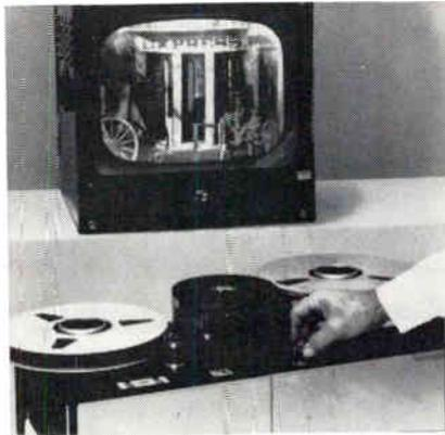
Precision Instrument PI-4V TV recorder features StopScan and VariScan, single controls which allow playback at stop-motion, or slow motion at any speed up to original recorded speed. First 23 of the 75-lb devices have gone to the Air Force for instructor training.
