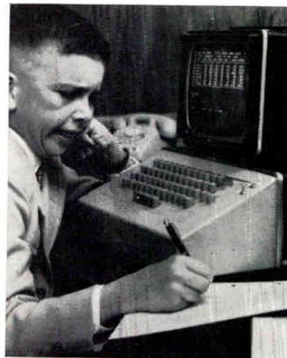
No cowboys and Indians here. Ten-year-old Wayne Burner tries hand at operating new General Electric Datanet—760 Keyboard Display Terminal. Device will display data stored in GE-235 computer systems. Device also allows changing and updating of data in the computer from the unit's keyboard.
