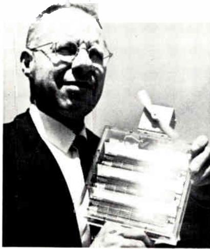
Reflected sun from V-ridge concentrators matches glitter of spinning prop powered by solar energy. Jack Tallent, Boeing Company aerospace engineer, holds small section of concentrating solar cell unit of several V-ridge concentrators, which are thin aluminum panels with solar cells in valleys and highly reflective aluminum on 60°-slopes to bounce extra sunlight onto cells. This unit, being developed for spacecraft, generates 2 watts.
