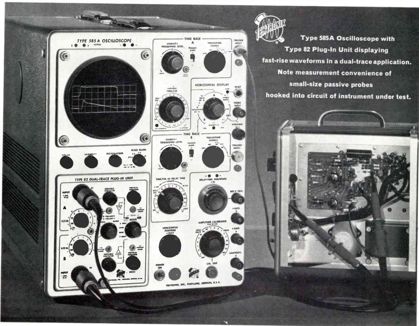
**Type 585A Oscilloscope with Type 82 Plug-In Unit displaying fast-rise waveforms in a dual-trace application. Note measurement convenience of small-size passive probes hooked into circuit of instrument under test.**
