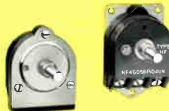
Provides higher voltage and wattage ratings for industrial and commercial electronic equipment. Quiet, stepless control. Life exceeds 100,000 complete cycles of operation on accelerated tests with less than 10% resistance change. Rated 5 watts at 40°C and 3 watts at 70°C, with a maximum of 750 volts.
