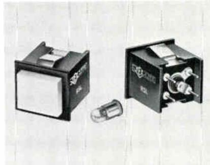
The Tec-Lite Rectangular Switch Lite, RSL Series, provide a choice of 14 different lens colors. Lenses can be hot stamped with legends in 4 different type sizes. Three available options include: Model 1, SPST normally open switch and indicator; Model 2, 2 normally open switches, DPST, and no indicator; and Model 3, an indicator only. The switch is rated 100ma at 120vac, non-inductive. Transistor Electronics Corp., Box 6191, Minneapolis, Minn.
