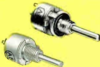
Type G potentiometers are miniature controls with solid molded resistance element. Only  $\frac{1}{2}$ " in diameter. Quiet, stepless operation. Rated  $\frac{1}{2}$  watt at 70°C. Values to 5 megohms. Type L are similar to Type G but rated  $\frac{1}{2}$  watt at 100°C. Can be used at 150°C with "no load."
