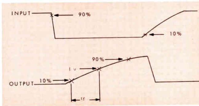
Fig. 7 (above): Some ICs pose complications to time measuring.
