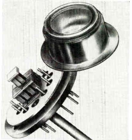
Model 094447 is a 2-stage cascade thermoelectric unit. It is capable of achieving a zero load temp. differential of 85°C. Carrying a 15mw heat load, this cooler will maintain the cold plate junction at -58°C in a vacuum of 10<sup>-6</sup> Torr with a +27°C heat sink temp. Cooler performance including vacuum level is guaranteed for 1 year. A 4w. heat sink is required, while input power is 3.5a. @ 1.1-vdc. Borg-Warner Thermoelectrics, Wolf & Algonquin Rds., Des Plaines, Ill. 60018.
