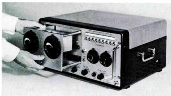
or production operations. Now, with one instrument and several, interchangeable plug-in oscillators, an engineer can cover a frequency range from audio to 3000 mc.
