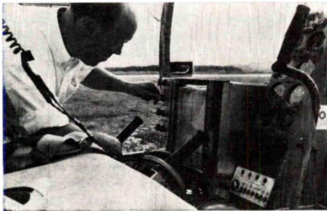
Four-channel recorder, highly portable, easily installed in aircraft, used to record air pollution over metropolitan New York. The recorder, made by Baldwin-Lima-Hamilton Electronics, is adjusted by Alex Proudfit, head of Sign-X Labs., firm making air sample tests.
