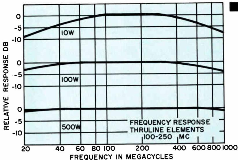
Fig. 3: Typical sensitivity response curves for r-f wattmeters.
