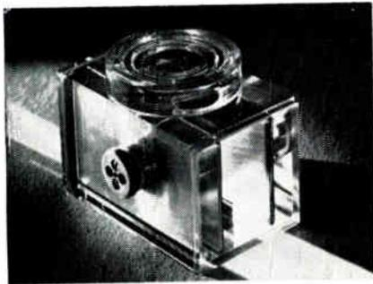
In this Kerr cell the windows are flat to a quarter wavelength and are low-reflection coated for 6943Å. The device is hermetically sealed and filled with hyper pure nitrobenzene. This eliminates space charge effects, produces an extremely uniform electric field, and creates a uniform and complete closure. Electrode separation or aperture width is 0.8 in. and aperture height is 1.5 in. Kappa Scientific Corp., 5785 Thornwood Ave., Goleta, Calif.
