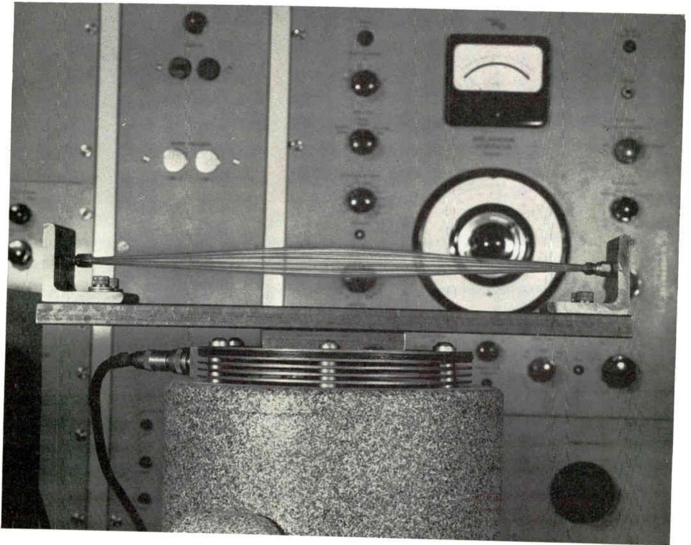
**This miniature coaxial cable of ours was vibrated at resonance 7 hours before the sheath cracked. The best competitive cable lasted 55 minutes.**
