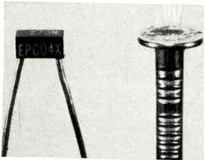
The Nailhead™ is part of the Neolythic™ capacitor series. They are designed for miniature and subminiature electronic packaging in filters, coupling, phase shifting, and most commercial, industrial, and military general-purpose digital circuitry. The capacitors are available in radial-lead epoxy-encased rectangulars, as well as axial-lead round tubular configurations. Electron Products, div. of Marshall Industries, 1960 Walker Ave., Monrovia, Calif.
