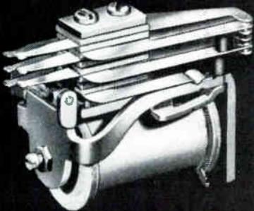
**CLASS Z RELAY.** Small and lightweight, but designed for service where flexibility is most important. Provides adequate coil volume to permit slugging for long operate and release timing. Four types for DC, one for AC, and two with snap-action contacts.
