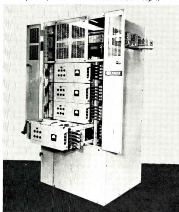
Fig. 2: This modular case group can supply 100 hp screwdown motor for forward and reverse operation, double operation, 300% load. It uses the drawers in Fig. 1.
