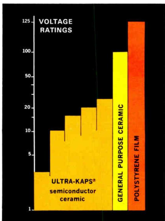
Check the chart for the type and voltage rating you need. Centralab offers the most practical approach to a bypass or coupling application. For 3 to 25 volt ratings the Ultra-Kap<sup>®</sup> semiconductor type of ceramic capacitor provides the maximum capacitance per unit volume at low cost. The 25-volt-rated types have high insulation resistance permitting their use in many new circuits.
