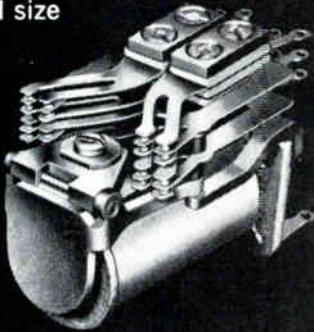
**CLASS E RELAY.** A lightweight space-saver with most of the features of the Class B. Life exceeds 200 million operations. Industry's widest terminal options: taper pin, integral socket, conventional solder, taper-tab, solderless wrap and printed circuit terminals.
