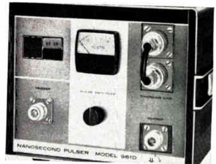
Model 961 provides high-voltage nsec. pulses for R&D, engineering and calibration uses. Amplitudes are adjustable from 0 to 3kv. Repetition rate is at 1 cps, line freq., or pushbutton actuated. The primary use is for simulation of scintillations from nuclear events by driving nsec. light sources. Other uses include photosynthesis timing, impedance measurements, multiplier phototube testing. Huggins Laboratories, 999 E. Arques Ave., Sunnyvale, Calif.
