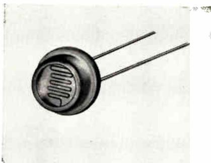
Type NSL-364C cadmium selenide photoconductive cells have chopping freqs. up to 2kc. Very low applied voltage operation is possible since the photocells have a linear voltage-current characteristic. Illuminated by a neon lamp, typical photocell resistance is 5K $\Omega$ , and dark resistance is 50 megohms minimum. Higher resistance types are also available. National Semiconductors Ltd., 2150 Ward St., Montreal 9, Canada.
