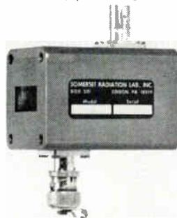
Model X430 Switch/Modulator/Voltage-Controlled Attenuator has its switching diodes connected in series, instead of the usual parallel. This allows a choice of either polarity grounded biasing or straight through bias drive in an ungrounded system. Min. attenuation of 3db or less is realized from 8.5 to 9.5gc with a total diode current of 150ma. Modulation freq. are dc to 500mc. Modulation is 99% from 8.2 to 10.5gc. Somerset Radiation Laboratory, Inc., Box 201, Edison, Pa. 18919.
