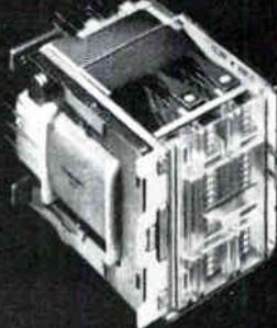
**CLASS W RELAY.** 17, 34 or 51 form C contact-spring combinations. Features low loss insulation, high insulation resistance. Extremely low inter-spring capacitance. Life in excess of one billion operations. Gold contacts available for low-level switching.
