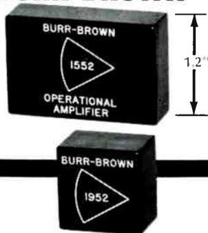
These new general purpose dc operational amplifiers employ matched junction FETs in the balanced input stage to achieve high input resistance and unusually low drift. Designed for  $\pm 10$  volt service, units have an operating temperature range of  $-40$  to  $+85^\circ\text{C}$ . Model 1552 is supplied in a modular  $1.8'' \times 1.2'' \times 0.6''$  package. Model 1952, designed for high density applications, is  $1.0'' \times 1.0'' \times 0.7''$ . Units are priced at \$145 and \$165.
