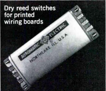
**PRINTED CIRCUIT CORREEDS.\*** Strong, moisture-resistant, compact. Unstressed contact leads provide firm, positive connections. Glass-filled plastic bobbins prevent moisture absorption. Low profiles and magnetic shielding permit high density within standard PC terminal spacing (multiples of 0.200 inches). Available with 1, 2, 3 and 5 capsules and magnetic latching. Contact forms A, B, & C.
