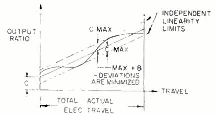
Independent linearity limits are shown with the output ratio vs. total elec. travel.
