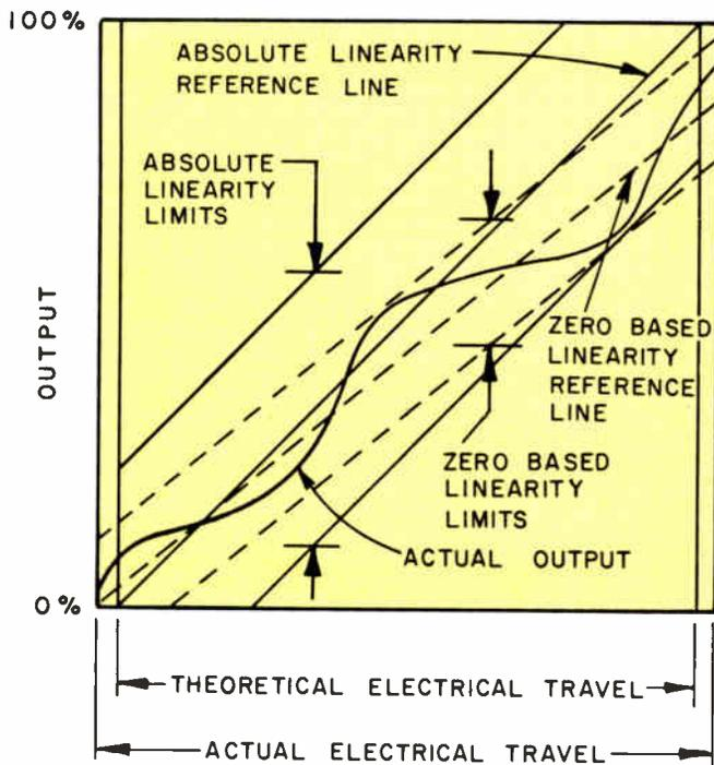
Fig. 2: Comparison between absolute and zero-based linearity.
