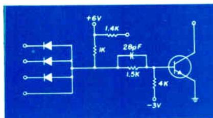
Circuit schematic, UC-1001B NAND/NOR Gate.
