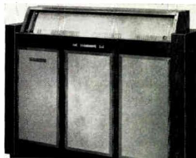
Model 750 is a high-speed, alpha-numeric data printer. It combines the speed and reliability of a line printer with the ease of operation, flexibility and low cost of a serial entry printer. Printing speed is 75 char./sec. Uses include on- or off-line operation with tab card, punched tape, and magnetic tape devices. It accommodates roll paper as wide as 50 in. and all standard sizes of fan-fold paper. The Bristol Co., Waterbury, Conn. 06720.
