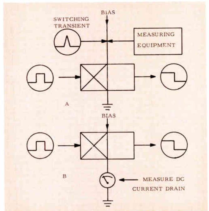
Fig. 9 (right): It is vital that compound dynamic and static measurements be made. Tester must be able to do both.
