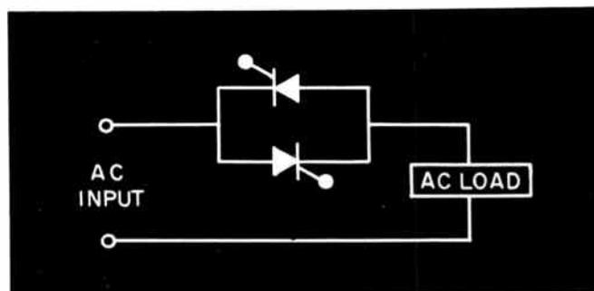
Fig. 9: A basic inverse parallel connection—ac output.
