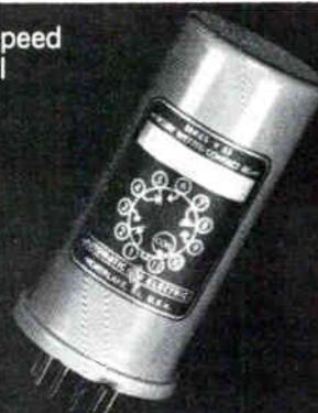
**CLASS V MERCURY-WETTED RELAY.** For computers, data processing and control equipment. Up to 200 operations per second. No contact erosion, no bounce. Over 1 billion operations without change, maintenance or adjustment. Can be operated within 30° of vertical. Polarized and nonpolarized versions. 1 pole to 4 pole double throw contact forms.
