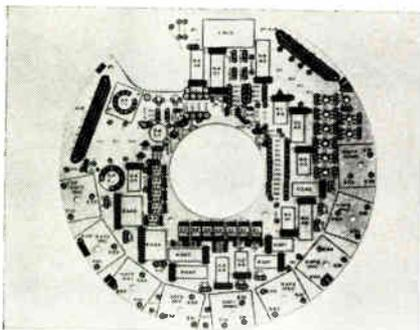
Two grades of ultrathin copper-clad laminated plastics are available for multilayer etched circuits. GEC-500 E, with base material, meets the specs. for NEMA grade G-10 laminate; and Fireban 600 E, a flame-retardant grade with base material, meets the specs. for NEMA grades G-10 and FR-4. Prepreg (B-stage) insulating sheets of the corresponding base laminates can be furnished. Taylor Corp., Valley Forge, Pa. 19481.
