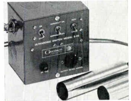
Model S-82 consists of a transmitter, receiver and control unit. The transmitter contains an 82kc piezoelectric transducer. Transmitter power is supplied by the control unit or by battery if separation of the 2 units is desired. The control unit converts 60 cps, 110v. to low voltages for the transistorized transmitter, receiver, relay driver and switching circuits. Electronic Components Div., Genisco Technology Corp., 6320 W. Arizona Circle, Los Angeles, Calif.
