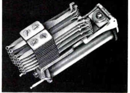
CLASS B RELAY. Finest quality telephone-type. Provides hundreds of millions of operations under all mounting and service conditions — with unfailing contact reliability. Combines sensitivity, contact stability, and circuit adaptability. Bifurcated twin-contacts. Long or short armatures for wide range of practical timing. Also for quiet AC operation.
