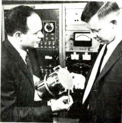
Robert Speiser (left) Electro-Optical Systems, Inc., and James Wolters, NASA Lewis Research Center, examine electron bombardment engine of type that just completed extended endurance test over 2,610 hours in space simulation tests. The run gives second-generation thruster "measurable status" as a propulsion source.
