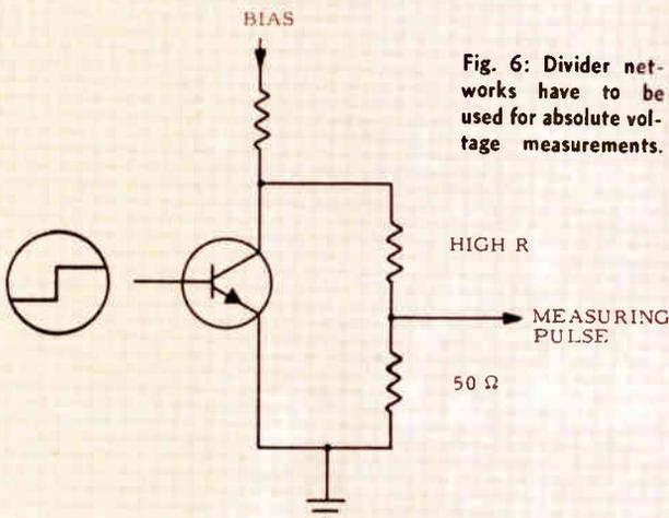
Fig. 6: Divider networks have to be used for absolute voltage measurements.
