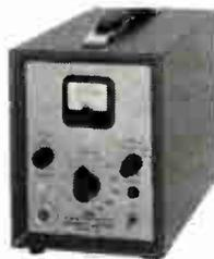
**Model 121Z Nanovoltmeter** provides  $0.1 \mu\text{V}$  full scale bridge balance detector or thermocouple indicator for standards and calibration work, in the field and in laboratories.
