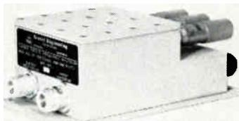
The Model 90600 tunable solid-state freq. multiplier is useful in L-Band and S-Band. The passive unit accepts input signals from 150 to 300mc and delivers typically 1/2 to 1w. output power between 900mc and 2.4gc. A multiplier diode type of unit, it is compact and weighs less than 3 lbs. Output filtering holds undesired harmonics and spurious freq. oscillations down more than 30db, typically 50db or more. Resdel Engineering Corp., 990 S. Fair Oaks Ave., Pasadena, Calif.
