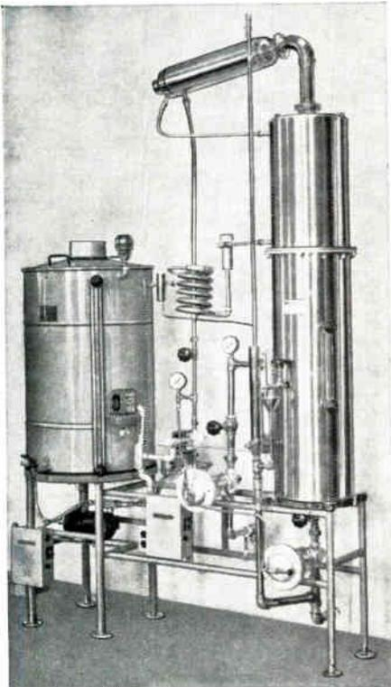
This NEW Still produces better quality distilled water than any other Still including triple distillation types. Special patented high purity features insures water of 0.1 ppm or less — ten times purer than ordinary distilled water.
