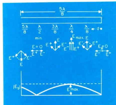
Fig. 4: Standing-wave diagram for voltage on a transmission line.
