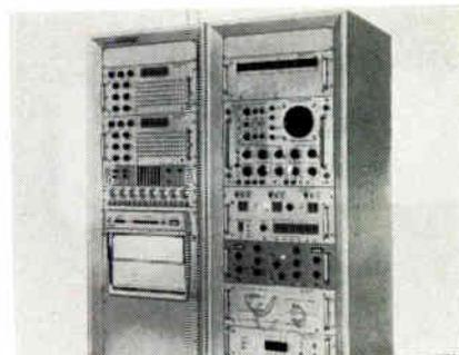
Model TRC-138 PCM ground station decommutates, synchronizes and reconstructs signals in the presence of noise, freq. drift and signal fadeout. It provides max. versatility for accommodation of both present and future requirements with performance within 1db of the theoretical optimum and bit synchronization to -10db. Decommutated channels may be prime, subcommutated or supercommutated data. The Roback Corp., Dept. 1526, Huntingdon Valley, Pa.
