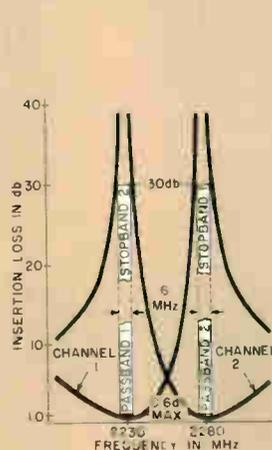
WITH TWO REJECTION CAVITIES PER CHANNEL
