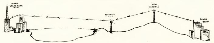
Artist's sketch showing relay points in WBKB's South-Bend-Chicago radio relay. Towers boost signal above earth's curvature.
