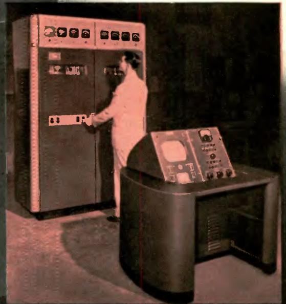
RCA's 500-watt TV transmitter is as easy to operate and tune as a standard broadcast transmitter. Controls for each unit are all within handy reach.
