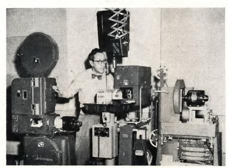
HAROLD HADDEN (above), supervisor of projection, talks into an overhead intercom as he gets set to operate the 35mm RCA cold light projector. Also grouped around the multiplexer is a 2 x 2 glass slide projector and a 16mm machine. Mr. Hadden (right), checks the Grey Telop which takes opaque slides, transparencies, ticker tape, scroll and a clock. The instrument can perform superimpositions and cross fades.
