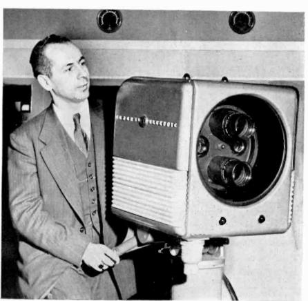
General Electric's new lightweight television camera has two sets of turretmounted lenses, and is equipped with finger-tip controls. A silent electric hydraulic system, foot-operated, gives flexibility of elevation controls. Lenses are focused by twisting the rotating grip on the right handle, as illustrated.
