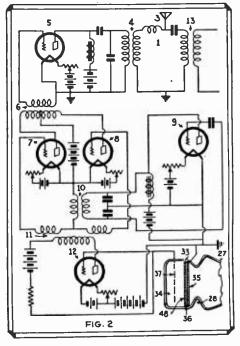
Zworykin's plan for using cathode ray tube as a transmitter—48 is photo-electric layer.
