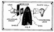
Fig. 4—Complete optical line-up in a "television camera"—which picks up image illuminated by artificial or natural light.
