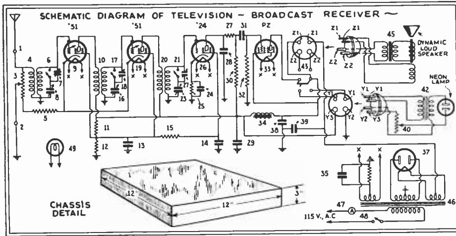
Wiring diagram for the combination broadcast and television receiver. To receive television waves the midget condenser short-circuiting switches 6, 17 and 21 are opened, reducing the tuning capacity for the shorter waves, by placing two condensers in series across each inductance as shown.
