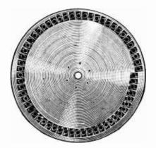
Appearance of finished See-All lens disc of the type used in their crater-tube projector. Each lens can be adjusted separately.
