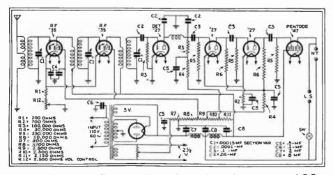
Complete circuit of the Pioneer television receiver, which employs two stages of R.F., detector and three A.F. stages.
