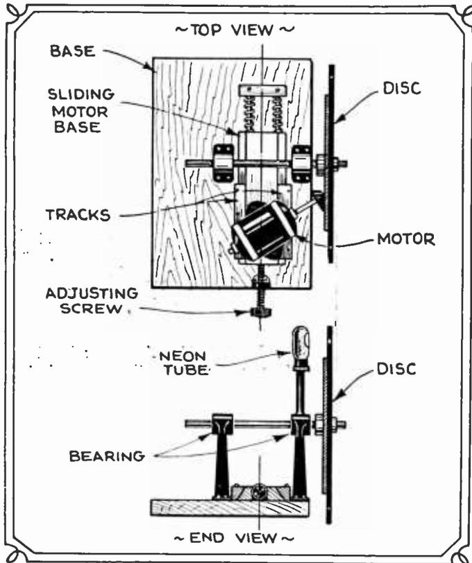
One of the simplest yet best scanning motor drives of the friction type, which has been used very successfully by many television experimenters. It was first suggested by Mr. C. F. Jenkins.
