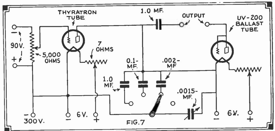
Complete hook-up of thyatron oscillator, using a UV 200 as a ballast tube.
