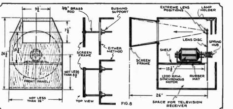
Side and front views of lens disc projector mounted in cabinet. This machine produces a brilliant image 10 by 12 inches. Special "framing" means are provided.
