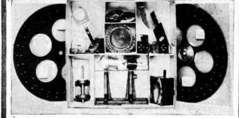
At the left we see the neat appearance and fine workmanship employed in making one of the European television scanner kits. These kits can be fitted with scanning discs containing different number of holes. Note the neon tube which is supplied as a part of the kit, also the lens mounting. Some kits contain the parts for the receiving set as well. The phonic wheel parts are also included.
