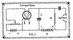
Fig. 1—Simplified diagram of thyratron oscillator.
