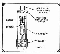
Arrangement of the electrodes in the Western Electric Co. cathode ray oscillograph tube.
