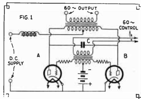
Diagram showing the connections for thyatron inverter.
