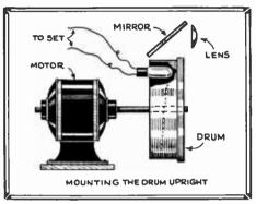
Mounting of drum scanner on motor shaft; the light rays from the neon tube are reflected by the mirror to the lens.
