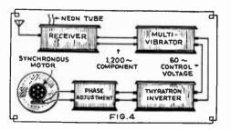
Here we have the complete line-up of the new apparatus here described for maintaining positive synchronism of the receiving scanner.
