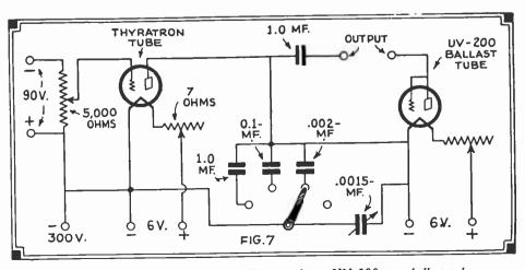
Complete hook-up of thuratron oscillator, using a UV 200 as a ballast tube.
