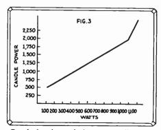
Graph showing ratio between candle-power and watts (power input) to the oscillator, a linear relation holding good over almost the entire range.
