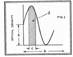
If the length of the scanning aperture is "C", the value of the light passing through the scanning aperture (hole) will be proportional to the shaded area "d".
