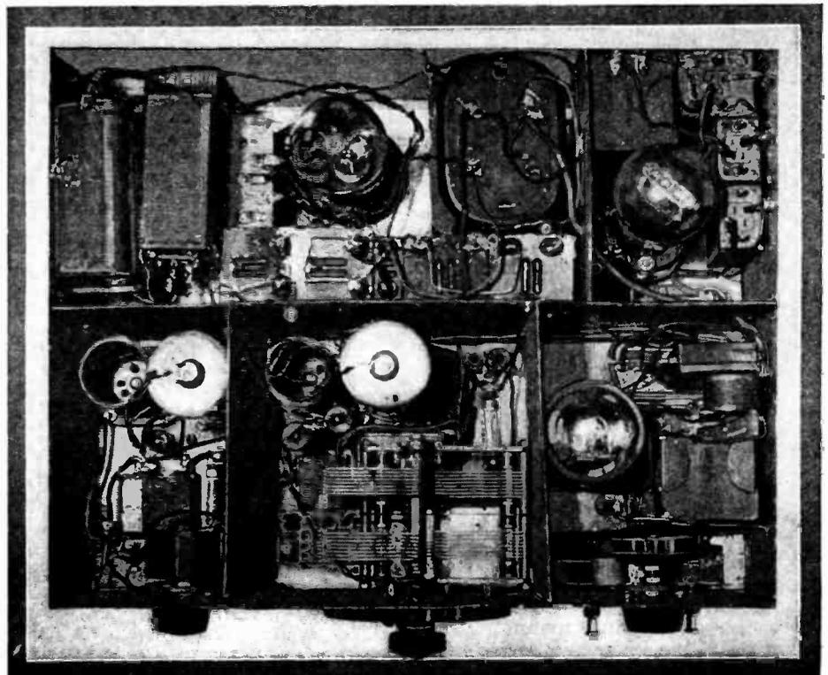
At Last! The Loftin-White amplifier adapted to television reception in this unusual receiver, which uses pentode output tube. Coil winding and other data included. Set works a Crater tube.
