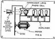
Arrangement of lenses in "direct pick-up" camera.
