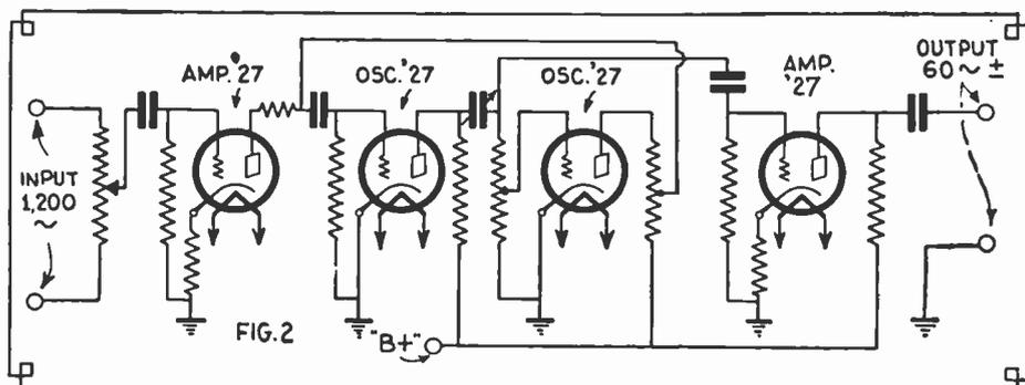
Diagram above shows connections of tubes, resistors and condensers in the multi-vibrator and amplifier circuits, used in establishing synchronization.
