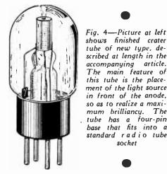
The hole in the cathode is about .07" in diameter and about  $\frac{1}{4}"$  deep—the ratio of width to depth being about 8 to 1. Under these conditions full advantage of the theoretical possibilities may be taken and the true point-source obtained.
