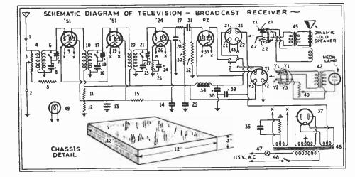
Wiring diagram for the combination broadcast and television receiver. To receive television waves the midget condenser short-circuiting switches 6, 17 and 21 are opened, reducing the tuning capacity for the shorter waves, by placing two condensers in series across each inductance as shown.
