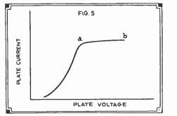
Fig. 5-Saturation curve of ballast tube.
