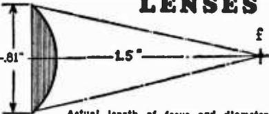
Actual length of focus and diameter for mounting in 20"-24" lens disc
