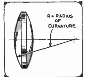
Right—The radius of curvature of a lens is important in television optics.
