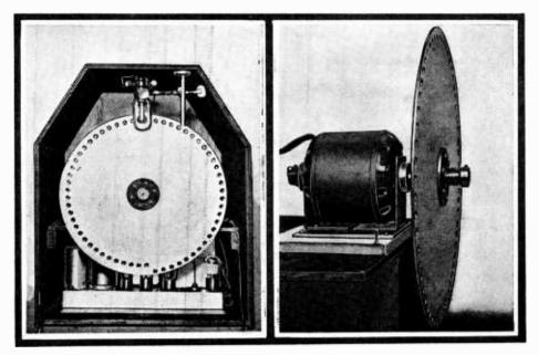
Rear view of lens disc and crater tube at left; and at right, close-up of Baldor synchronous motor and lens disc, with Baldor spring coupling.
