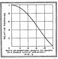
Curve showing relative response compared with the ratio of aperture length to the length of a single cyclic variation.
