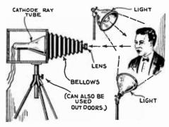
Image of subject, illuminated by lights as shown, is picked up by lens of camera and focused onto photo-sensitive end of the special cathode ray tube.
