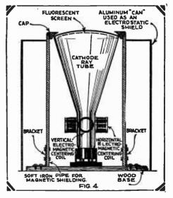
How cathode ray tube is shielded with iron and aluminum cans.
