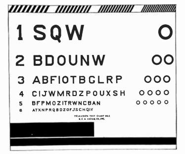
Fig. 1-Black and white chart, which has been found very useful in checking up fidelity in transmission.
