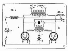
Diagram showing the connections for thuratron inverter.
