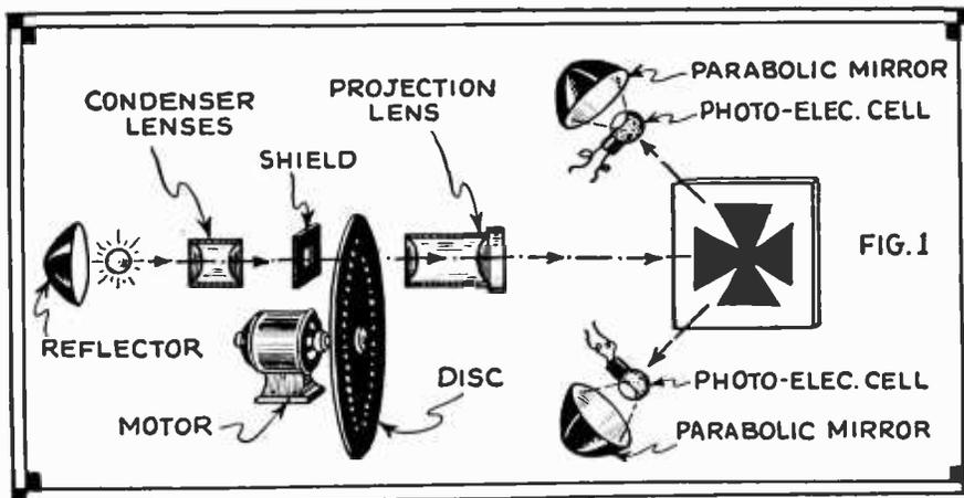
Fig. 1—Optical system used in the "flying spot" television image pick-up arrangement. The light ray passes out through the scanning disc and lens on to the subject, the reflected light rays being picked up by the photo-cells.
