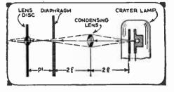
Above—How con-densing leas im-proves efficiency by focussing light upon the dia-phragm opening.
