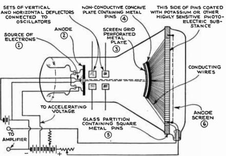
Fig. 4—The Lora "transmitting" cathode ray tube scanner. A photo-electric layer of pins are affected by the image, which is focused on to the anode screen by a camera.
