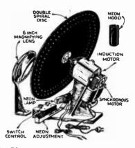
The Pioneer scanner, fitted with accelerating and synchronous motors. The image is viewed through the lens at the left.
