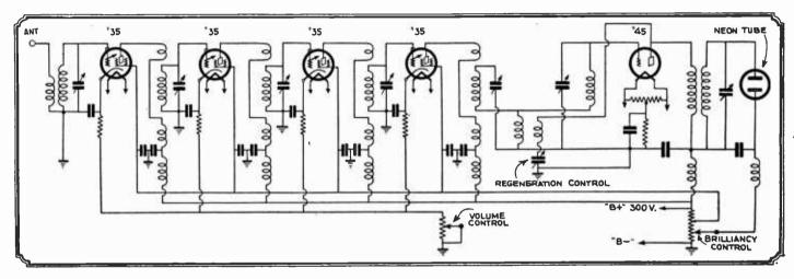
Hook-up of four screen-grid and power amplifier stages to neon tube. The input stages are the same as those employed for normal operation using a detector. One of the features of this circuit is the elimination of the distortion caused by the detector.
