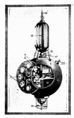
The Hartmann sub-sea television camera which is provided with a scanner 9, and lens 6, together with a second lens 7, prism 11 and movie camera 12. The electric motor 13 and propeller 14, help to pull the device down to the desired depth in the water.
