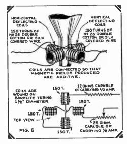
Size and position of magnetic deflecting coils used for centering the image on cathode tube screen.
