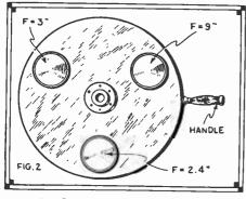
Fig. 2-Several lenses mounted in turret head, so as to make any one available in-stantly for use on image "pick-up".
