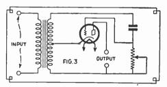
Circuit diagram is given above as used for making phase adjustment by thyratron control.
