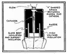
Cross-section of improved crater tube perfected by the author, in which the glow is brought out in front of the anode cylinder. Fig. 3.
