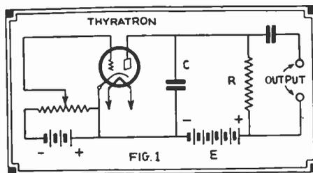
Fig. 1—Simplified diagram of thyatron oscillator.
