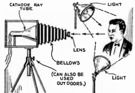
Image of subject, illuminated by lights as shown, is picked up by lens of camera and focused onto photo-sensitive end of the special cathode ray tube.
