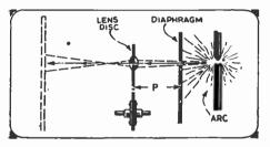
Use of restricting diaphragm between spot source of light and lens disc; the distance "P" is important, as explained in the text.
