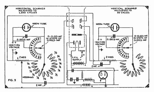
Fig. 9—How the 1.200- and the 20-cycle "saw-tooth" oscillators, also the signal amplifier are connected to a Von Ardenne (General Radio Co.) cathode ray oscillograph tube.
