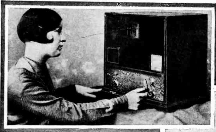
The television kits here shown are of the Telehor (German) design and manufacture, and illustrate the kind of apparatus European television fans are "looking in" with. Girl above is tuning one of the kits assembled into a cabinet.
