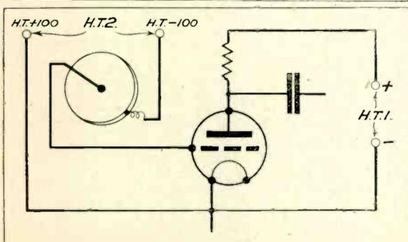
(Above) Method of coupling cell to first stage amplifier. (Below) An alternative method, which is more sensitive but requires two H.T. batteries; no grid leak is used.
