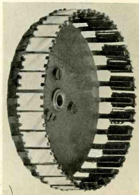
*The completed drum with mirrors in position.*
