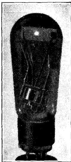
Micromesh Tunograph, a visual tuning indicator functioning on the principle of the cathode-ray oscillograph.
