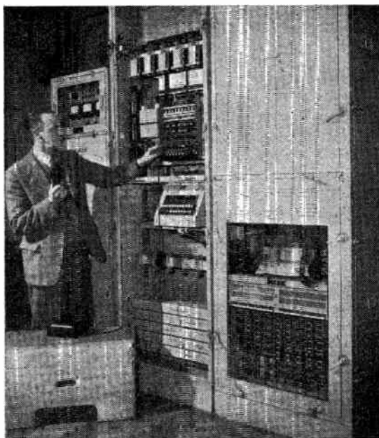
The magnetic drum director at the Lee Green exchange showing the actual drum in the right-hand cabinet.
