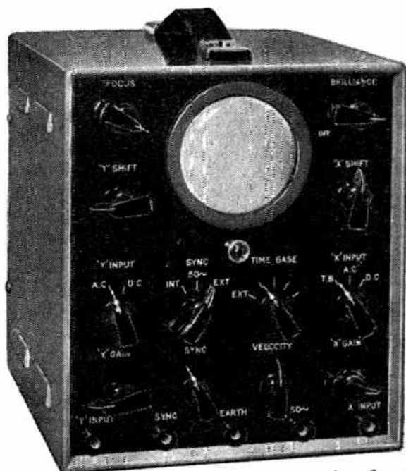
Model 2300. Light-weight Portable. B/W D.C. to 2.5Mc/s Sensitivity 50mV/cm. C.R. Tube 3in. diam. Dims.: 7½x4½x 7½ins.
