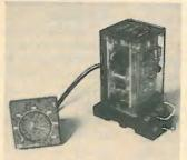
Operating over the range  $-200^{\circ}$ C to  $+1600^{\circ}$ C, the CAL 6101 electronic temperature controller from Controls and Automation can switch a 3kW resistive load (at 14A, 220V 50Hz). This range is covered by nine versions of the controller, each of which comprises two separate sections, the plug-in control section and a remote bezel and dial giving, according to the makers, greater flexibility in mounting. The dial potentiometer is connected to the controller by a single flexible
