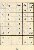
**Fig. 2** (a) An n pulse recirculating shift register, (b) truth table. Although t.t.l. and c.m.o.s. can be used in this and other circuits, all of the diagrams are shown using the positive edge of the clock pulse.
