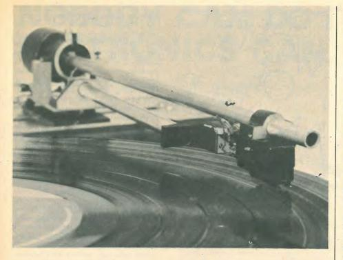
First constructional methods are not necessarily the best. Dual-purpose light slit with cue-bar to raise pickup arm (above) could be simplified; and author found simplifications could be made to the hinged platform, pivot pillars and gymbal, shown right and below (improvements in part 2).
