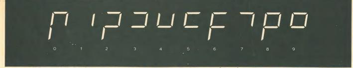
Fig. 3. Displays of the decimals 0 to 9 with both the C and D segments omitted. There are still ten distinct patterns and no confusion between the decimals.
