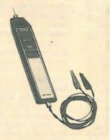
as is the DP-50. The DP-50 digital probe is a 50MHz instrument which displays logic activity as three l.e.d. indicators to indicate pulse presence and high/low logic states. An unusual feature is a "memory freeze" which stores pulse display. The DP-50 has a  $2M\Omega$  input impedance, is fully protected from overload and detects pulses to within 10ns. Distributed by Empire Exporters, Inc, Plainview New York, USA. WW 303
