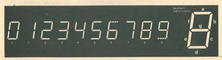
Fig. 1. Seven-segment displays of the decimals 0 to 9. Segment A on decimal 6 and segment D on decimal 9 are normally included.
