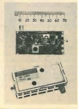
low content of undesirable mixing products. Colour subcarrier and sound sub-carrier beat product is -55dB with respect to carrier, resulting, according to Astec, in interferencefreè pictures. The modulator measures 71  $\times$  37  $\times$  20mm and current consumption is 9mA with a recommended supply of 5V  $\pm$ 10%. Astec Europe Ltd, 4A Sheet St, Windsor, Berks. WW 311
