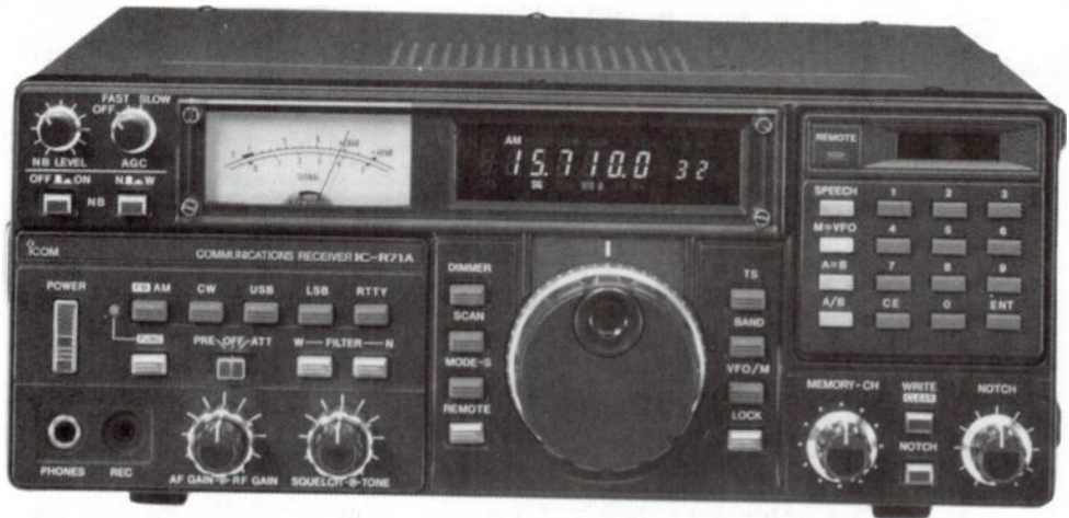
3-4 A superb receiver with memories, dial and keyboard tuning, and remote-control capabilities. (courtesy of Icom Inc.)
