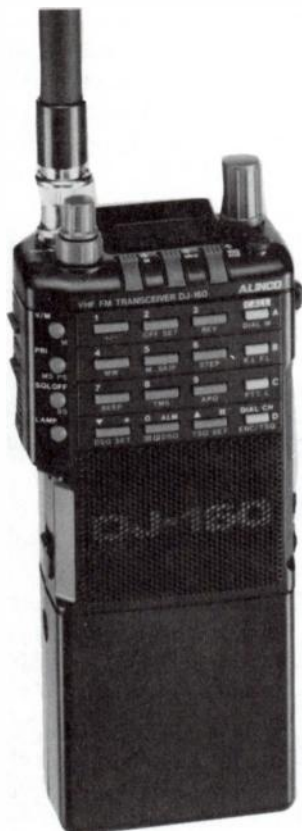
9-9 The Alinco DJ-160 is a VHF FM transceiver that is made specifically for using repeaters.
