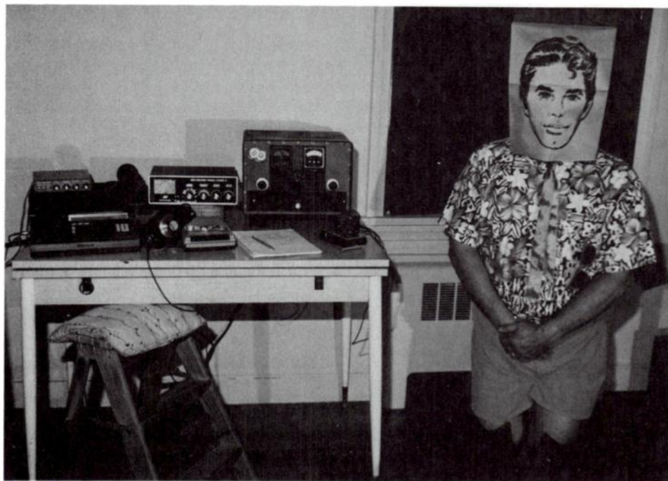
8-1 H.V. Short in the backup studios of RFM. The shack contains a receiver, a limiter/compressor, a cassette player, an antenna tuner, and a Johnson Viking Challenger transmitter from the 1950s.
