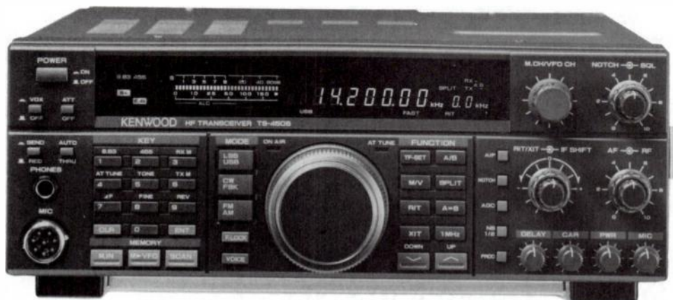
9-3 The Kenwood TS-450S HF transceiver has an electronic LED S-meter to the left of the digital readout. (courtesy of Kenwood).
