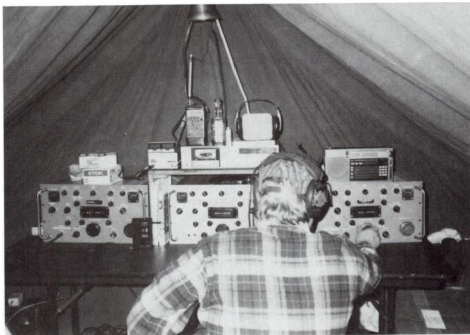
3-1 Three military-surplus R-390A receivers from the 1960s. Compare them to the size of the Sony ICF-2010 (standing on the right-hand R-390A) and to the Sony Pro-80 (standing in the center, above the cassette deck).
