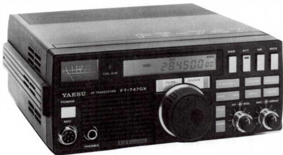
9-7 The uncomplicated Yaesu FT-747GX transceiver, which (like all modern transceivers) can be used in either LSB or USB modes (courtesy of Yaesu).
