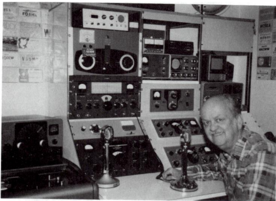
9-5 Bud Enoch, KE6DN, dressed up his old equipment with a sleek homemade console. The rack-style console was constructed from one-inch steel tubing and was mounted on casters for easy access to the back. (courtesy of Electric Radio ).
