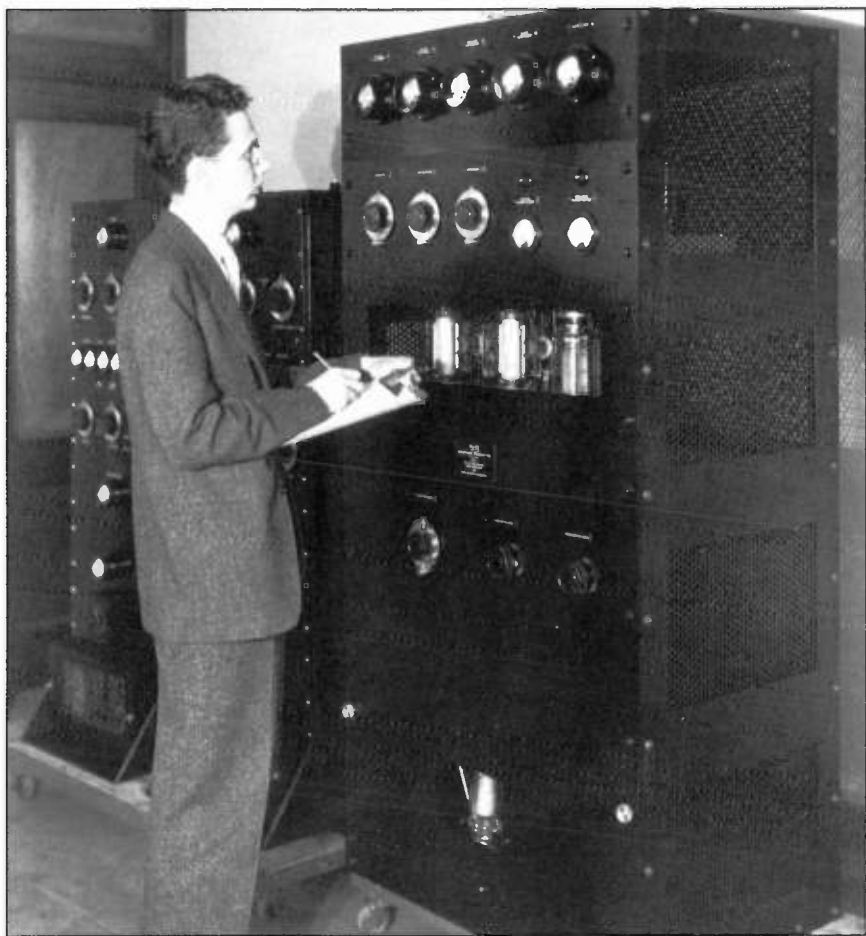
Arthur Collins with the Byrd Antarctic Expedition Transmitters. The 1,000-watt 20B is the large unit on the right.
