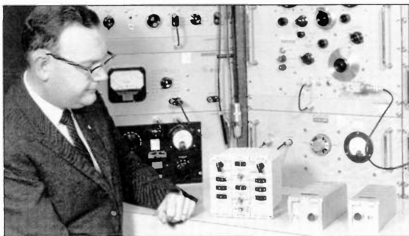
The Collins-built voice communication equipment for the two-man Gemini spacecraft.
