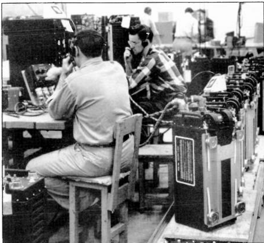
Technicians testing aircraft AN-ARC-27 UHF transceivers, radios which helped restore Collins to profitability after World War II
