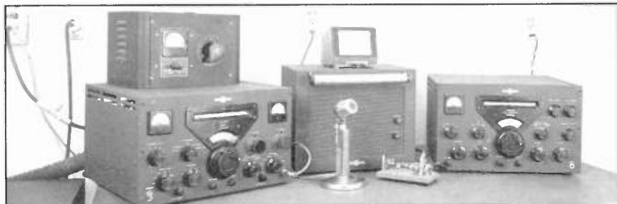
The KWS-1 transmitter, left, and 75A-4 receiver, the first Collins amateur single side-band radios.
