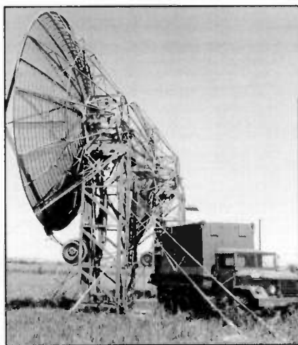
One of several types of portable scatter communication systems, used by the Army in VietNam.
