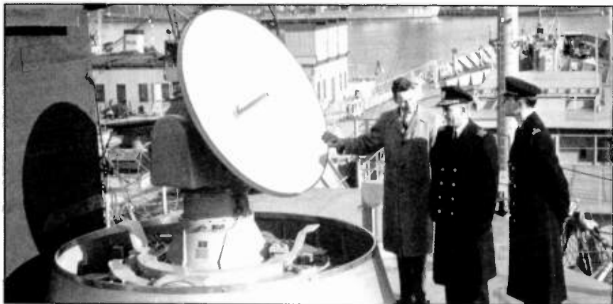
Navy officials inspect a shipboard installation of the Collins Radio Sextant, a major development in navigation capability in the 1950s.
