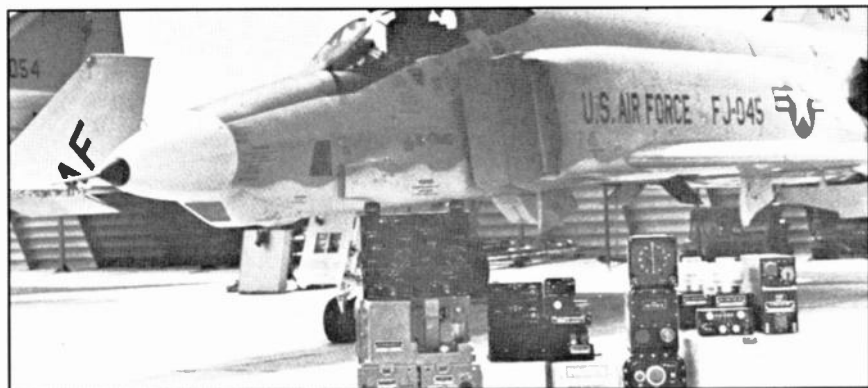
Collins equipment for the Air Force F-4 Phantom aircraft, including CNL system, high frequency radio and horizontal situation indicator.
