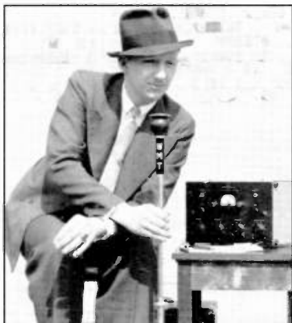
Clair Miller, one of Arthur's first employees, demonstrating a 12X portable amplifier used for radio broadcasts from field locations.
