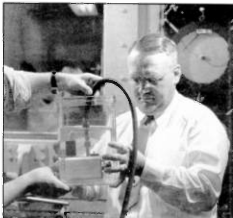
Ted Hunter testing Permeability Tuned Oscillator: At right, Mel Doelz and the Mechanical Filter:
