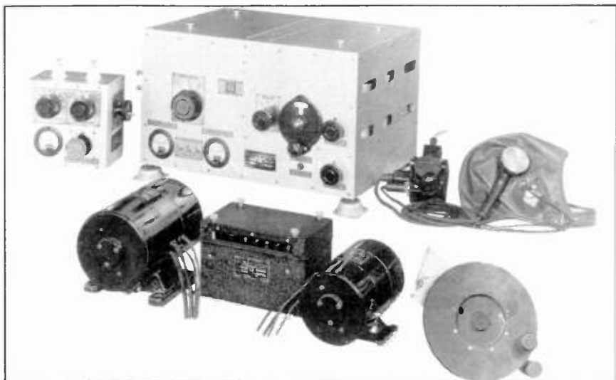
Aircraft communication equipment for the air force of Colombia, part of the first large order of airborne gear designed and built by Collins about 1935.
