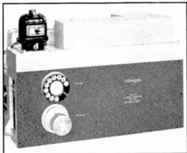
Above, first aircraft transmitter with a Collins Autotune, built for Braniff Airways. At right, patent for the Collins Course Indicator.
