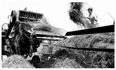
Steam threshing in early 1970s. Robert Hale pitches grain bundle into the slat-belt feeder of the 36 inch Minneapolis grain separator. Machine is belt driven by steam engine 60-75 feet away, thus the long drive belt.
